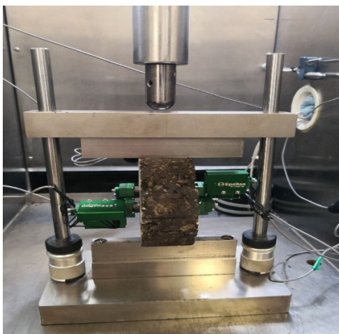
Figure 2-4 IDT test setup
