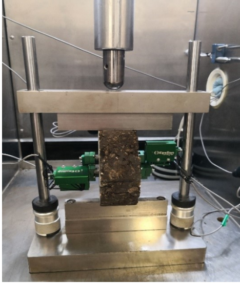
Figure 4-5 Creep compliance and strength test setup
