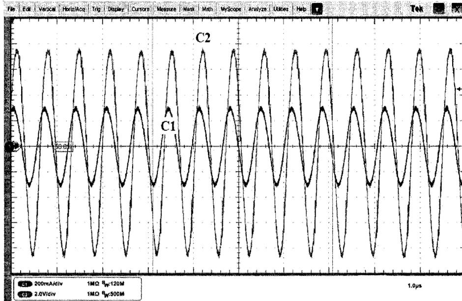
**Figure 3.3: Sample measurement showing voltage (C2) and current (C1) signal**
