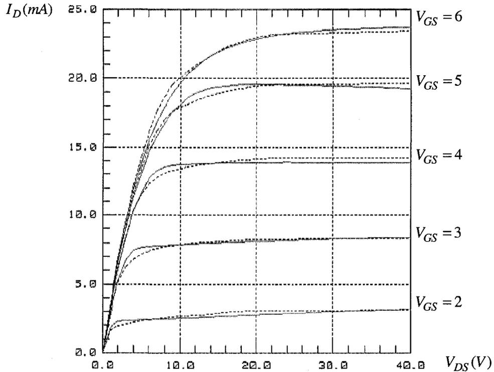
**Figure 4.24:** Plots of drain current ( $I_D$ ) versus drain-to-source ( $v_{DS}$ ) voltage for NDH16GC LDMOS: measured (solid line) versus simulated (dotted line) curves at different gate-to-source voltage ( $v_{GS}$ ), provided by Dalsa Semiconductor Inc. in [38]
