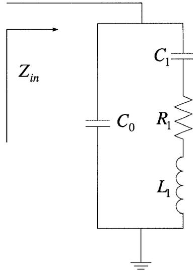
**Figure 2.3: Van Dyke's model for a piezoelectric element at resonance**
