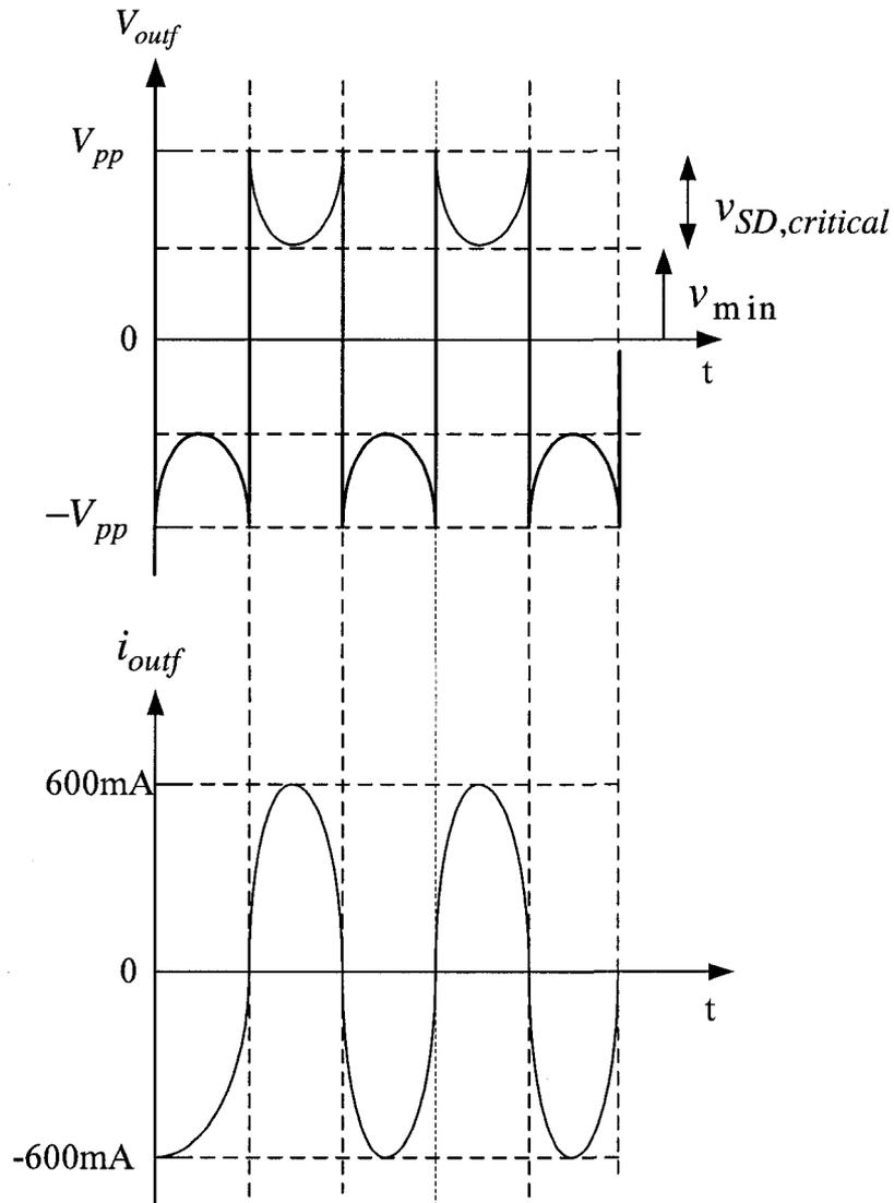
**Figure 4.26:** Expected output voltages and currents at  $V_{outf}$  node of the pulse-modulated signal generator circuit
