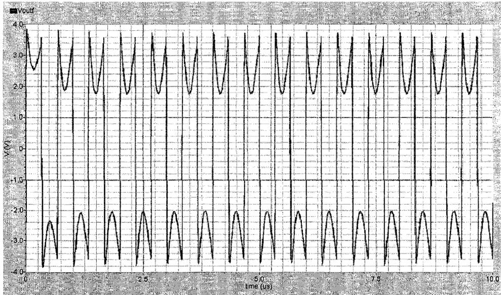
*Figure 4.30: Simulated waveform showing 1.50MHz voltage at Voutf*
