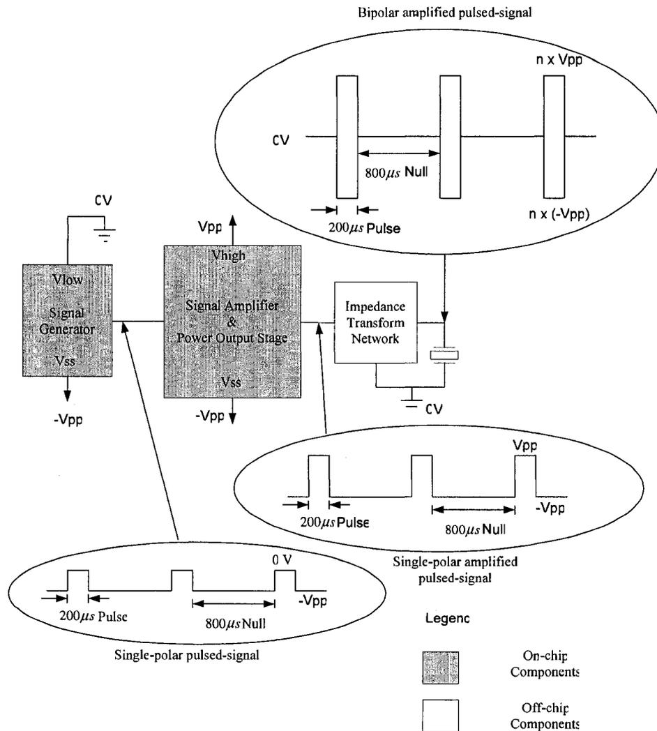
**Figure 4.8: Mechanism for the generation of bipolar pulse-modulated signal from single-polar pulsed signal**
