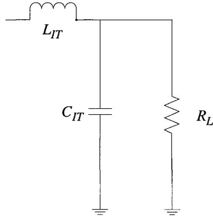
**Figure 4.3: An L-match consisting of an inductor  $L_{IT}$  and a capacitor  $C_{IT}$  connected to a load resistor  $R_L$**
