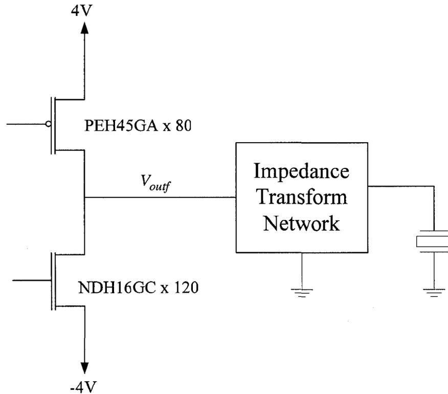
**Figure 4.27: Final design of power output stage**
