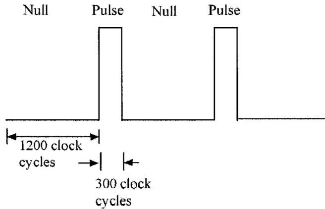
**Figure 4.11: Pulse characteristics diagram**
