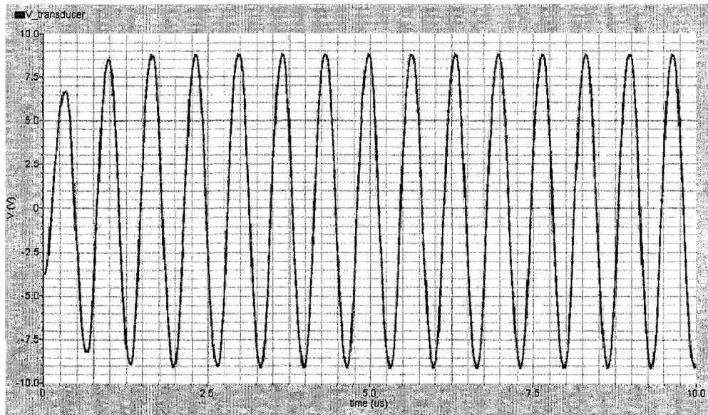
*Figure 4.31: Simulated waveform showing 1.50MHz voltage across the transducer*
