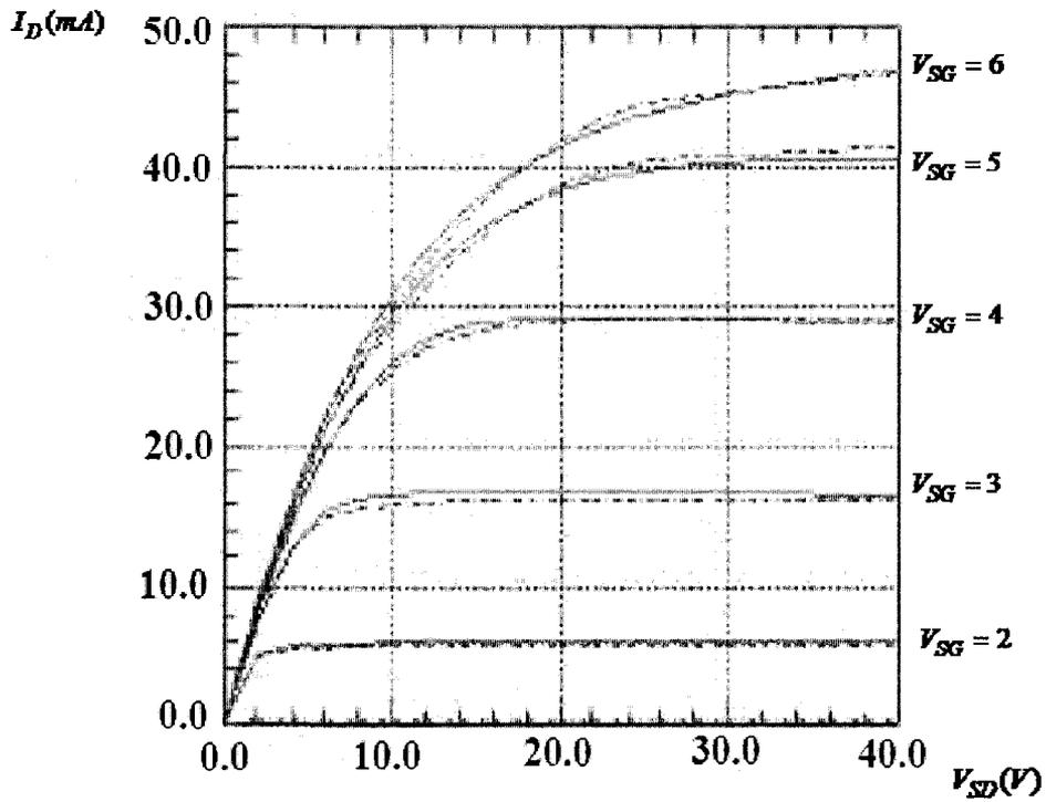
Figure 4.23: Plots of drain current ( $I_D$ ) versus source-to-drain voltage ( $v_{SD}$ ) for PEH45GA EDMOS: measured (solid line) versus simulated (dotted line) curves at different source-to-gate voltage ( $v_{SG}$ ), provided by Dalsa Semiconductor Inc. in [38]
