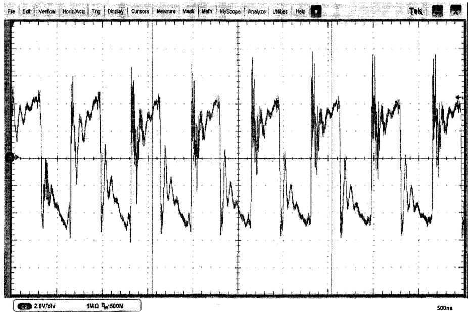
*Figure 4.38: Voltage waveform at the Voutf pin of the pulse-modulated signal integrated circuit*
