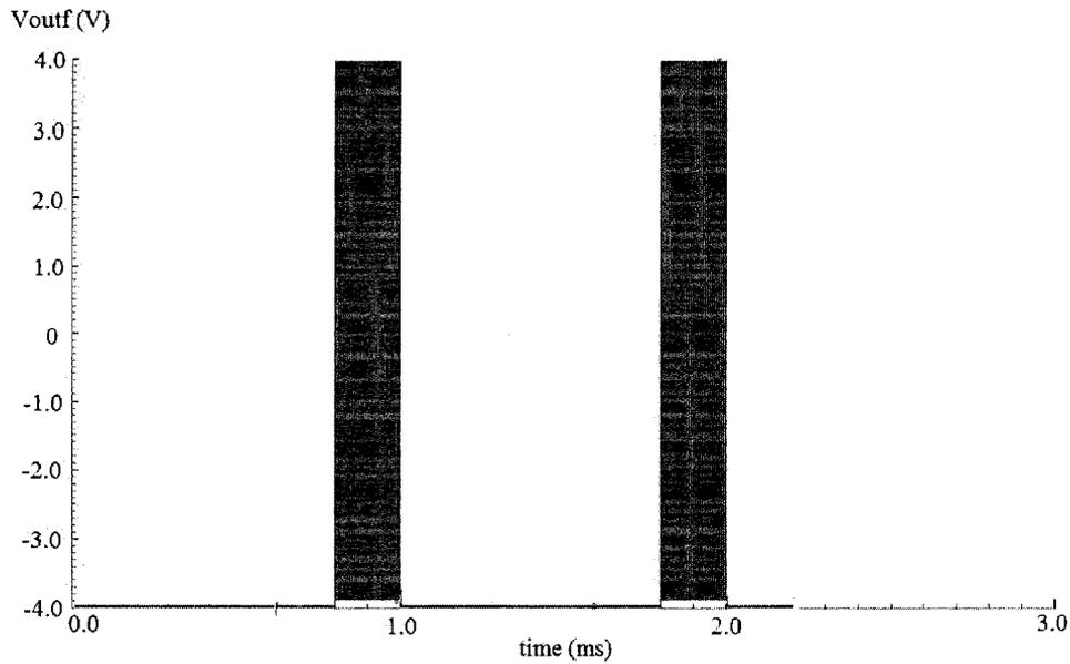
**Figure 4.29:** Simulated output pulses, each  $200\mu\text{s}$  wide and separated by  $800\mu\text{s}$
