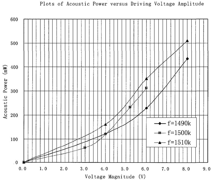
**Figure 3.8: Plots of acoustic power as a function of driving voltage magnitude**
