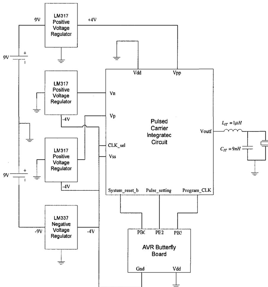
**Figure 4.35: Circuit diagram of board-level circuit**
