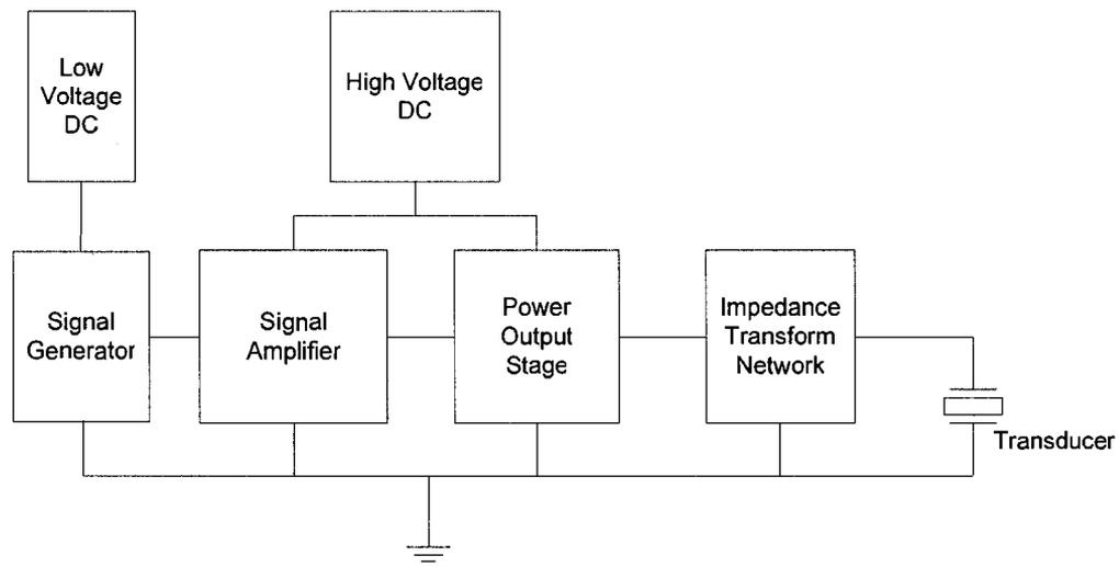
**Figure 2.5: System block diagram of a typical ultrasound generator**
