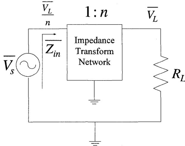
**Figure 4.2: Conceptual representation of the input impedance of an impedance transform network driven by a voltage source  $V_s$**
