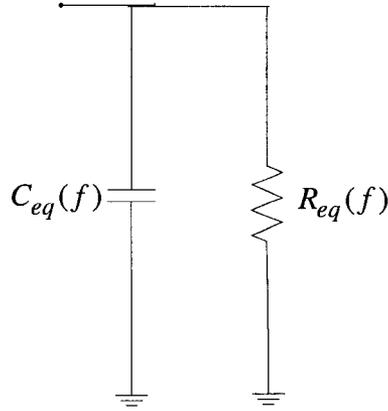
**Figure 3.10: Proposed narrow-bandwidth circuit model**
