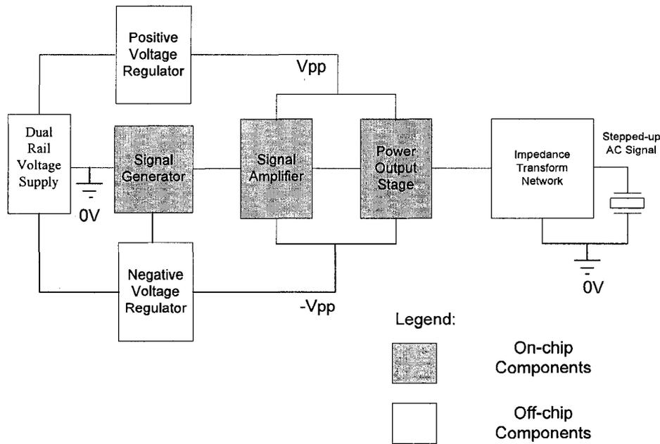
**Figure 4.7: Proposed architecture for LIPUS generator showing the scope of chip-level integration**
