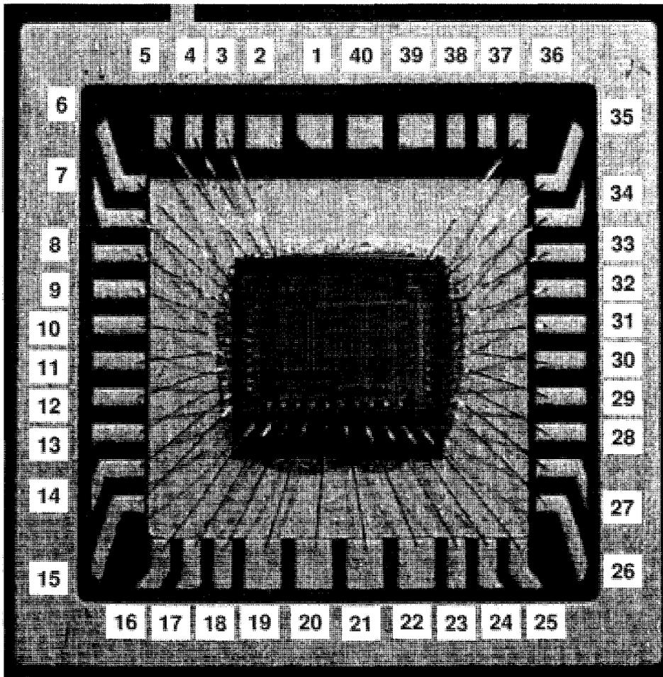
*Figure B.1: Bonding diagram*
