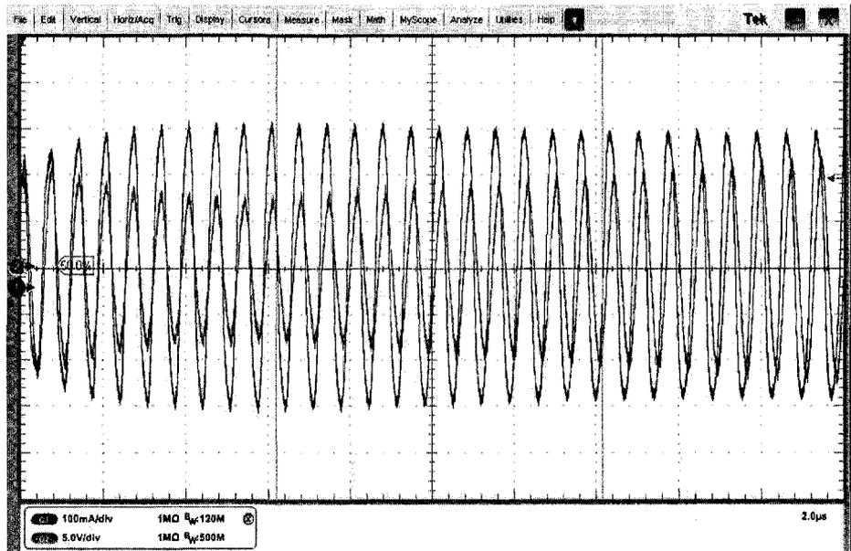
**Figure 4.40: 1.5MHz voltage (smaller waveform) and current (larger waveform) signals**
