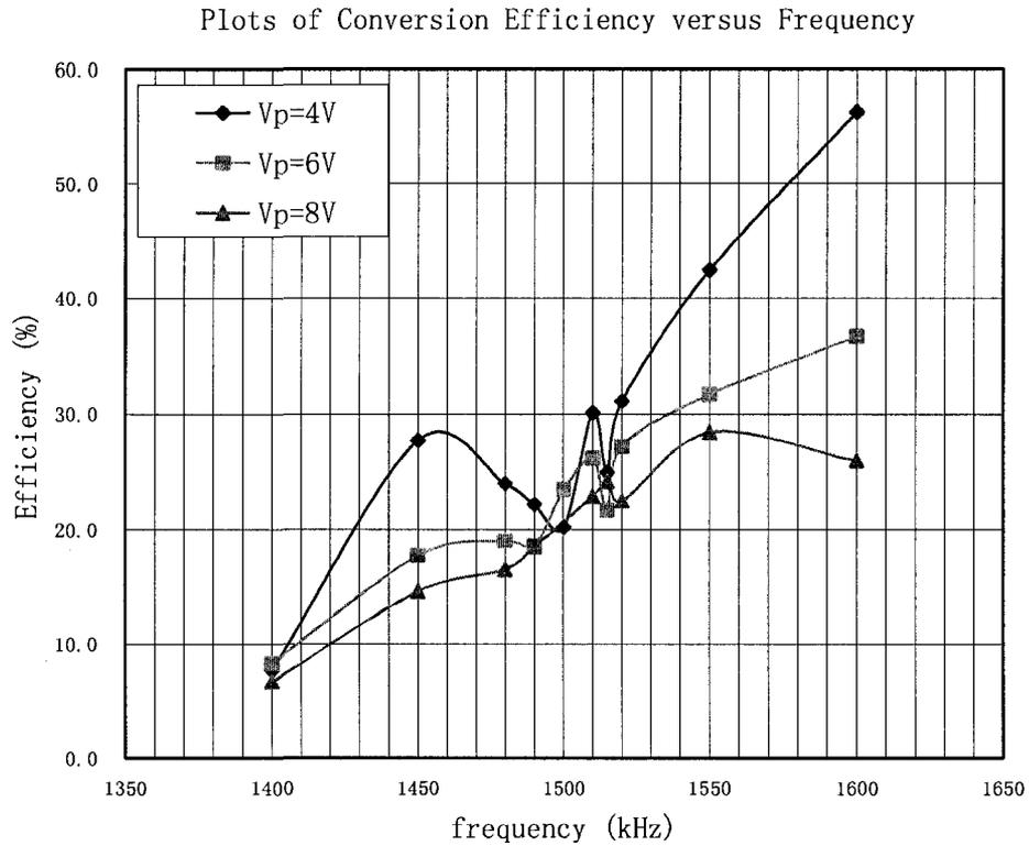
**Figure 3.7: Power efficiency plot for voltage amplitudes of 4V, 6V and 8V**
