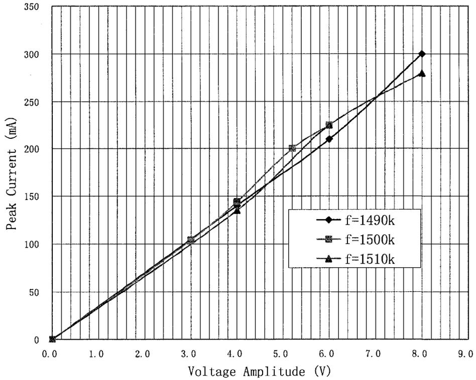
**Figure 3.9: Peak current versus driving voltage amplitude curves at  $f = 1490\text{kHz}$ ,  $f = 1500\text{kHz}$  and  $f = 1510\text{kHz}$  respectively**
