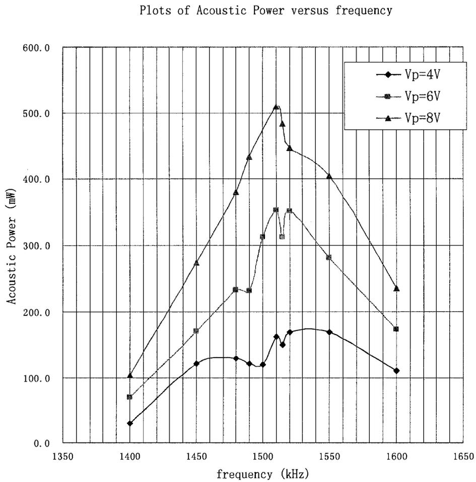
**Figure 3.6: Plots of acoustic power versus frequency for driving voltage of amplitudes 4V, 6V and 8V**
