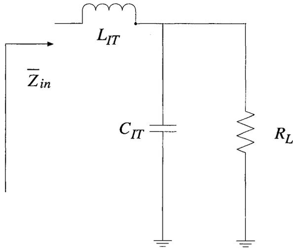
**Figure A.1:** An L-match network consisting of  $C_{IT}$  and  $L_{IT}$  for load  $R_L$
