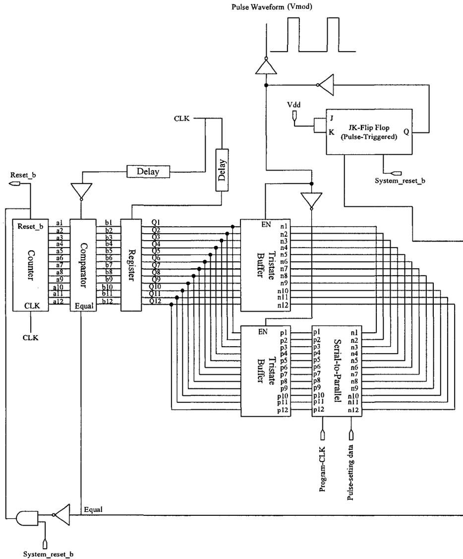
Figure 4.14: Pulse generator circuitry
