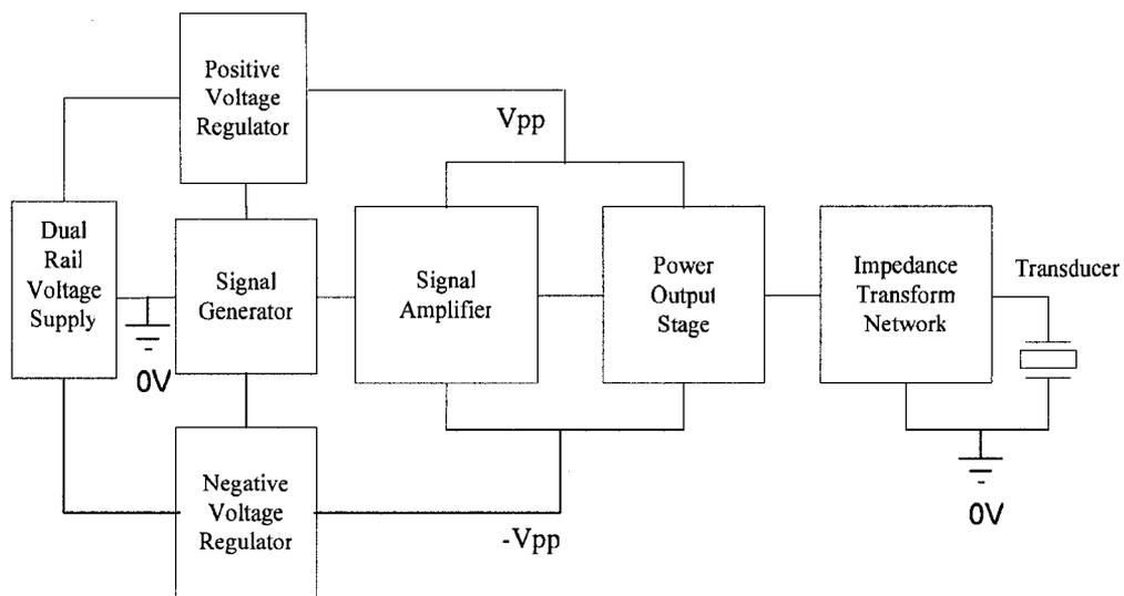
*Figure 4.1: Proposed architecture for LIPUS generator*
