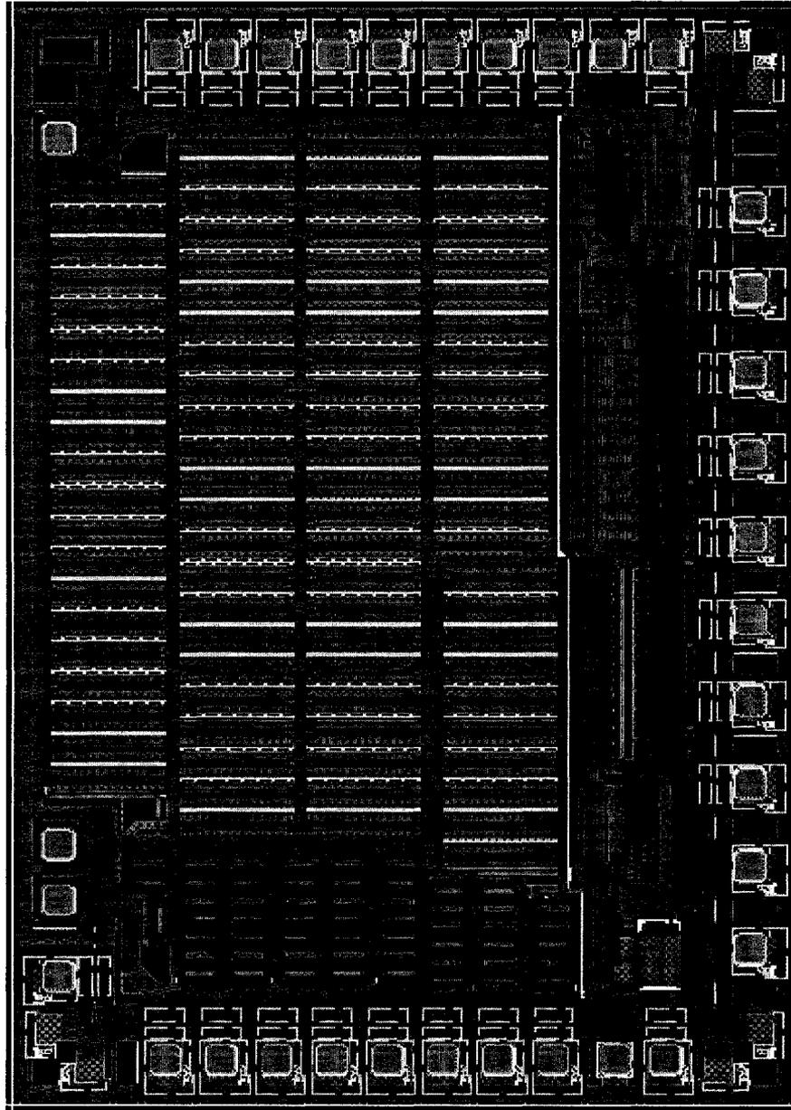
*Figure 4.33: Pulse-modulated signal generator integrated circuit layout*
