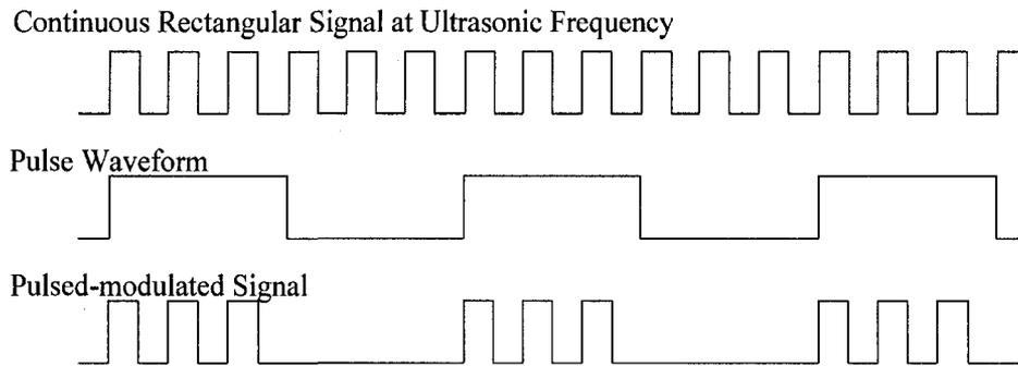
**Figure 4.10: Illustration of pulse-modulated signal waveform Generation**
