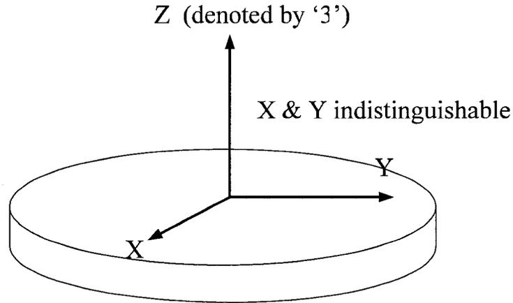
*Figure 2.1: Designation of axes for a thin ceramic piezoelectric disc*
