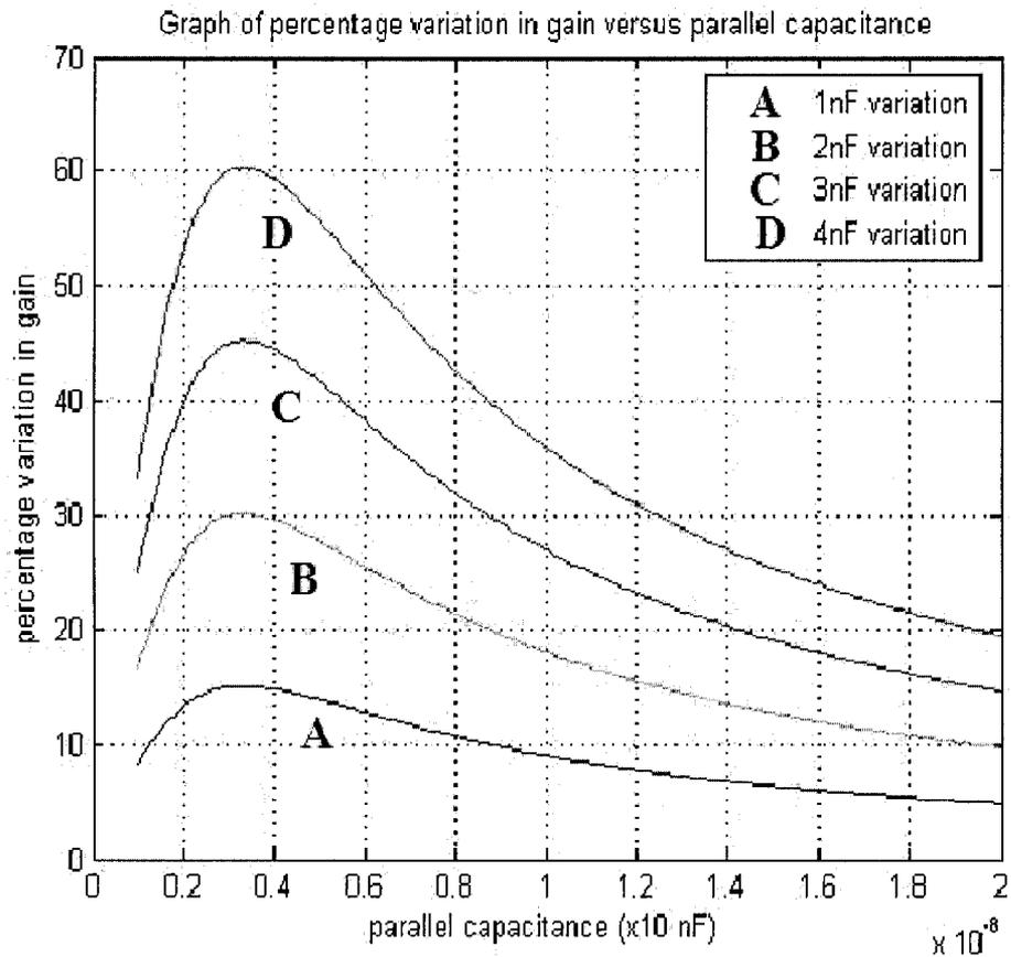
**Figure 4.5:** Curves illustrating percentage variation in gain due to variation in capacitance
