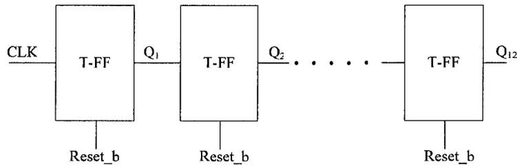
**Figure 4.15: Gate-level counter implementation using a cascade of 12 T-flip flops**
