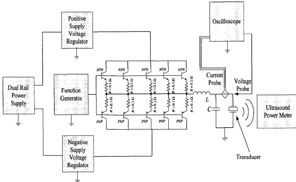
**Figure 3.1:** Schematic diagram of the proposed setup for transducer characterization
