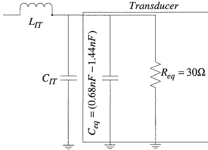
**Figure 4.4: L-match circuit for impedance transformation**
