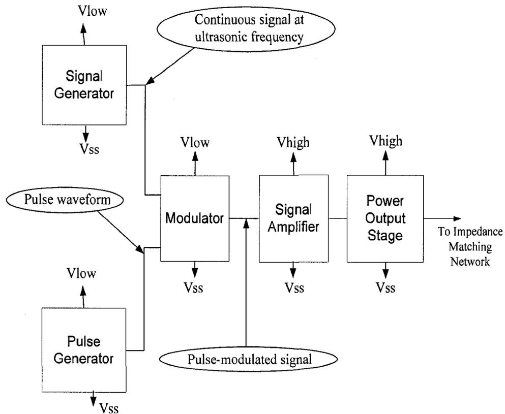
**Figure 4.9: Proposed single-polar pulse-modulated signal generator architecture**
