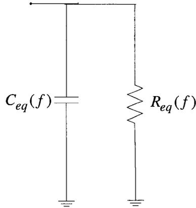
**Figure 3.10: Proposed narrow-bandwidth circuit model**
