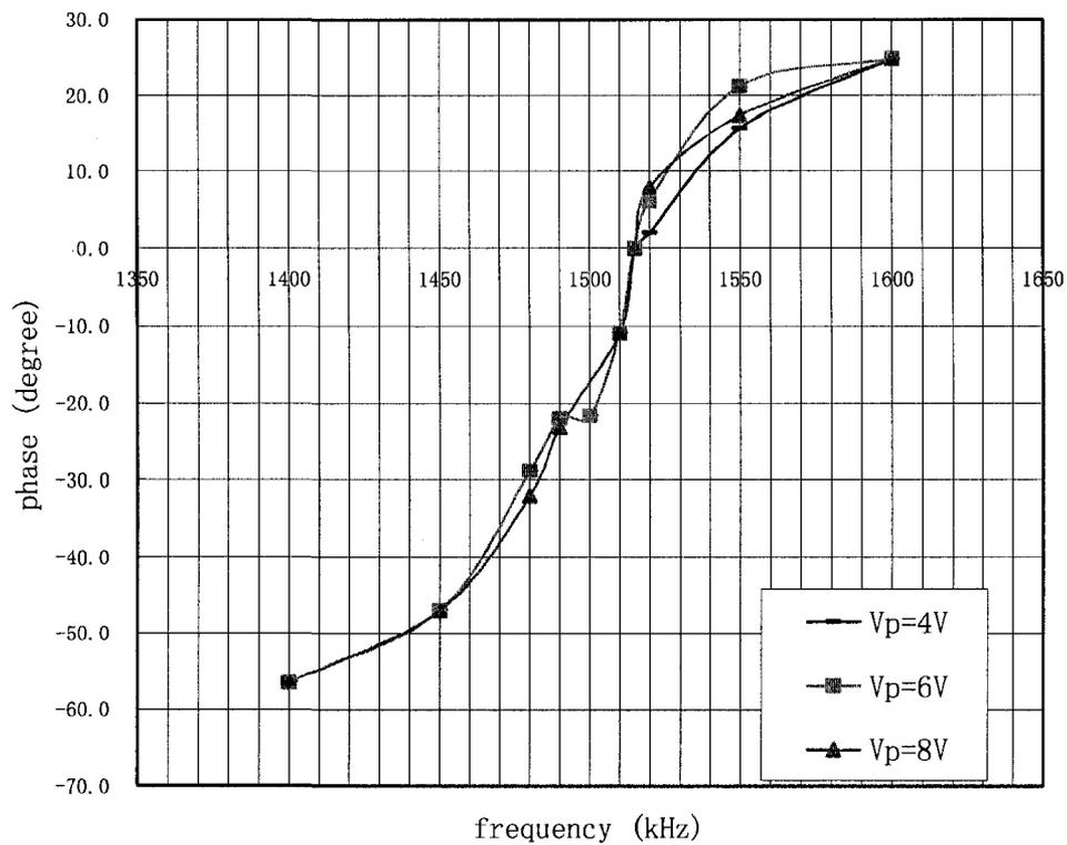
**Figure 3.5: Plots of impedance phase as a function of frequency for voltage signals of amplitudes 4V, 6V and 8V**
