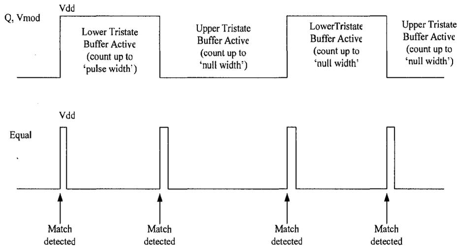
**Figure 4.17: Illustration of pulse-generation mechanism showing waveforms on nodes labeled 'Equal', 'Q', and 'Vmod'**
