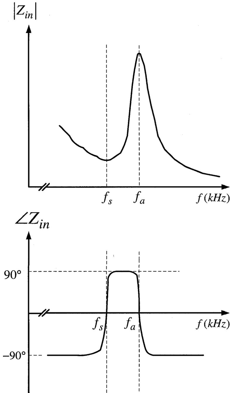
*Figure 2.4 (top) Impedance magnitude and (bottom) impedance phase of a piezoelectric transducer*
