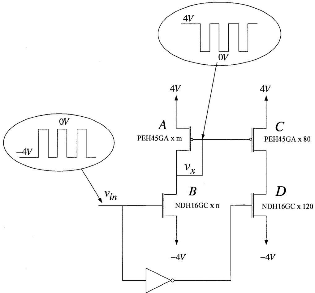
**Figure 4.28: Illustration of  $v_x$  in level-shifter circuit**
