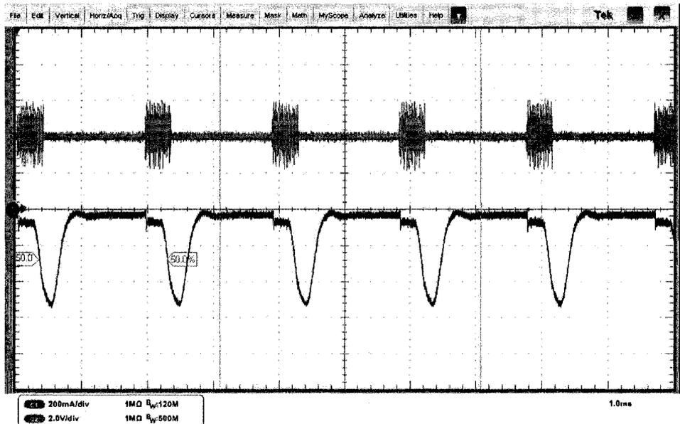
**Figure 4.41:** Current into circuit measured at the output of the negative voltage regulator (bottom waveform) and supply voltage at the output of the positive
