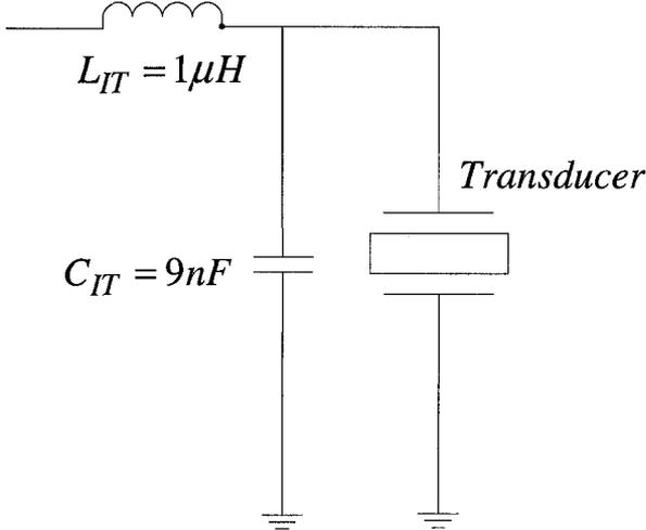
**Figure 4.6:** *L-match circuit for voltage gain of three*
