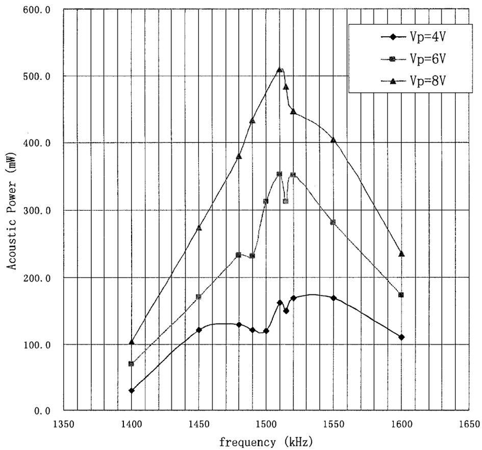
**Figure 3.6: Plots of acoustic power versus frequency for driving voltage of amplitudes 4V, 6V and 8V**
