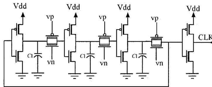
**Figure 4.13: Ring Oscillator Circuit**
