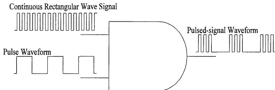
**Figure 4.19: Modulation with an AND gate**
