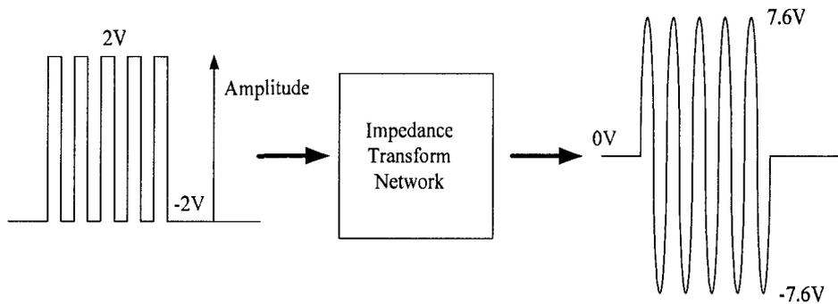
**Figure 4.22: Single-polar rectangular waveform to bipolar sinusoidal waveform conversion**
