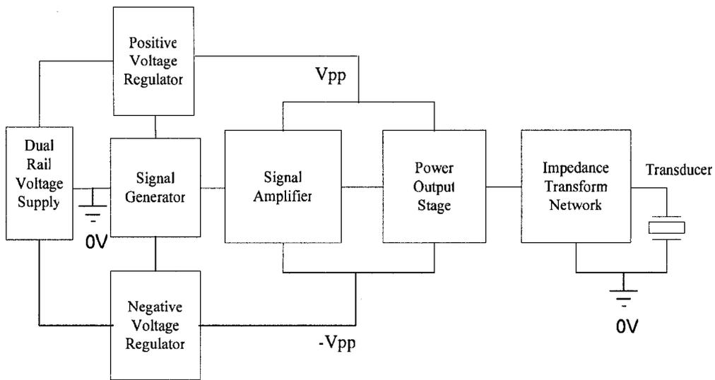
*Figure 4.1: Proposed architecture for LIPUS generator*
