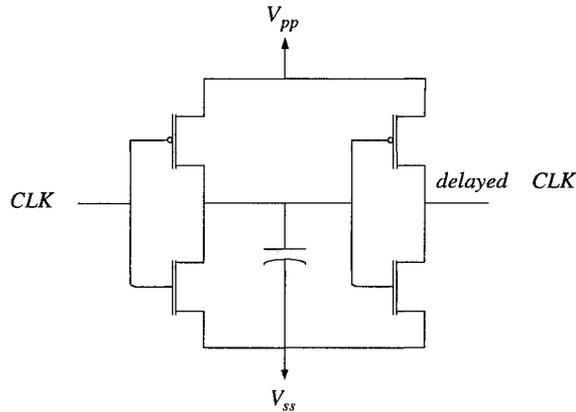
**Figure 4.18: Circuit realization of delay block**
