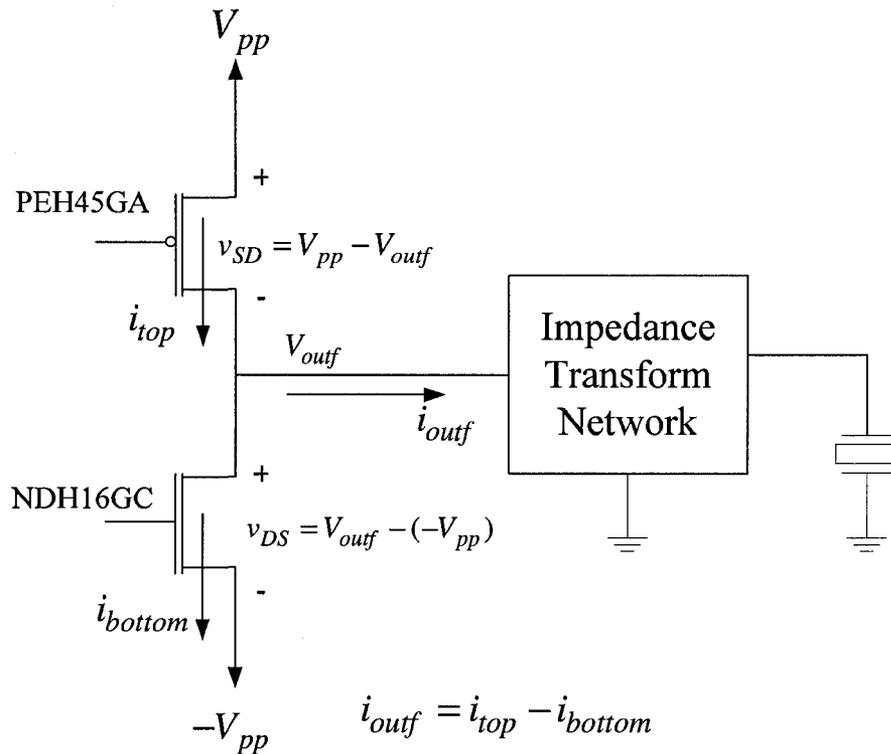
**Figure 4.25: Illustration of currents and voltages in the power output stage**
