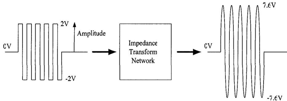
**Figure 4.21: Bipolar rectangular waveform to bipolar sinusoidal waveform conversion**
