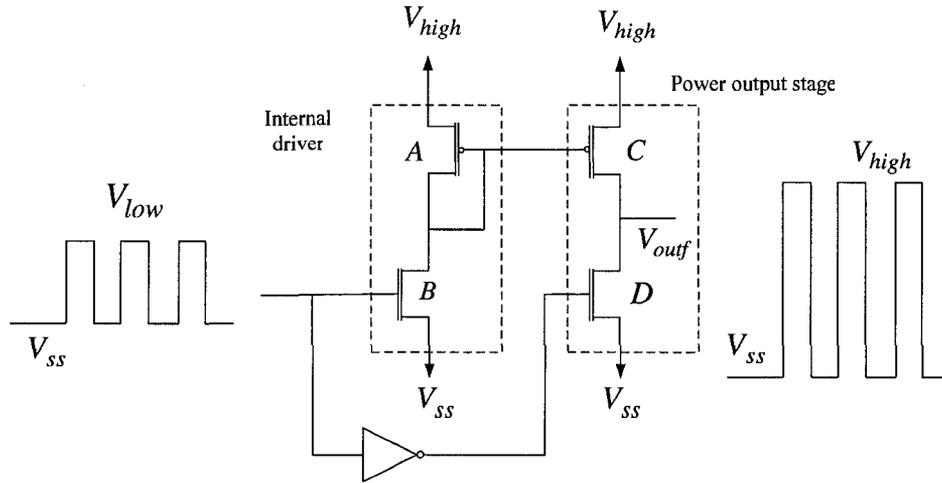
**Figure 4.20: Level-shifter Circuit**
