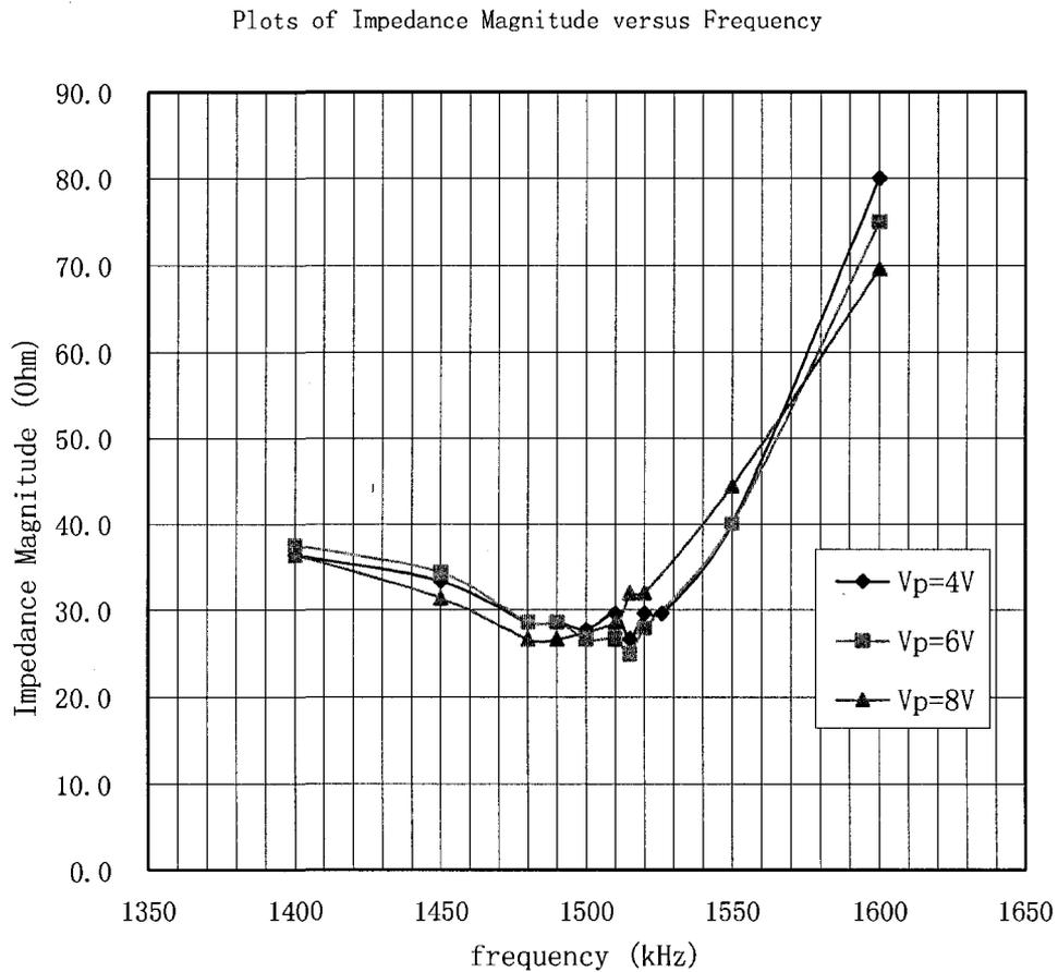
**Figure 3.4:** Plots of impedance magnitude as a function of frequency for voltage signals of amplitudes 4V, 6V and 8V
