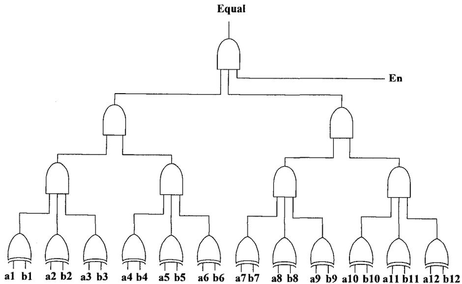
**Figure 4.16: Gate-level implementation of comparator**
