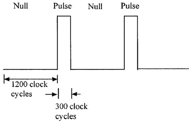
**Figure 4.11: Pulse characteristics diagram**
