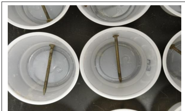
Figure 7: Red brown iron oxidation of the post experiment experimental group.
