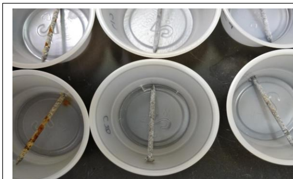
Figure 6: White oxidation characterized as white rust from the galvanized coating of the zinc.
