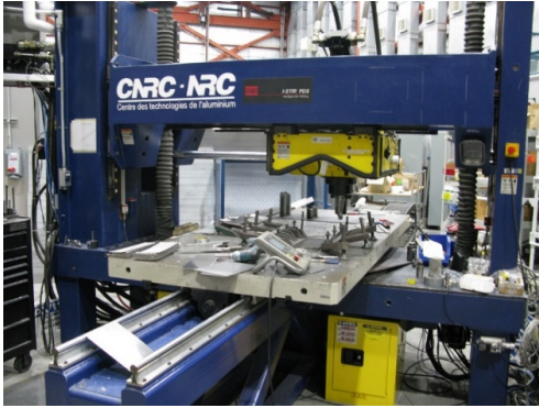
Figure 3. MTS I-Stir PDS system used for welding, NRC Saguenay
