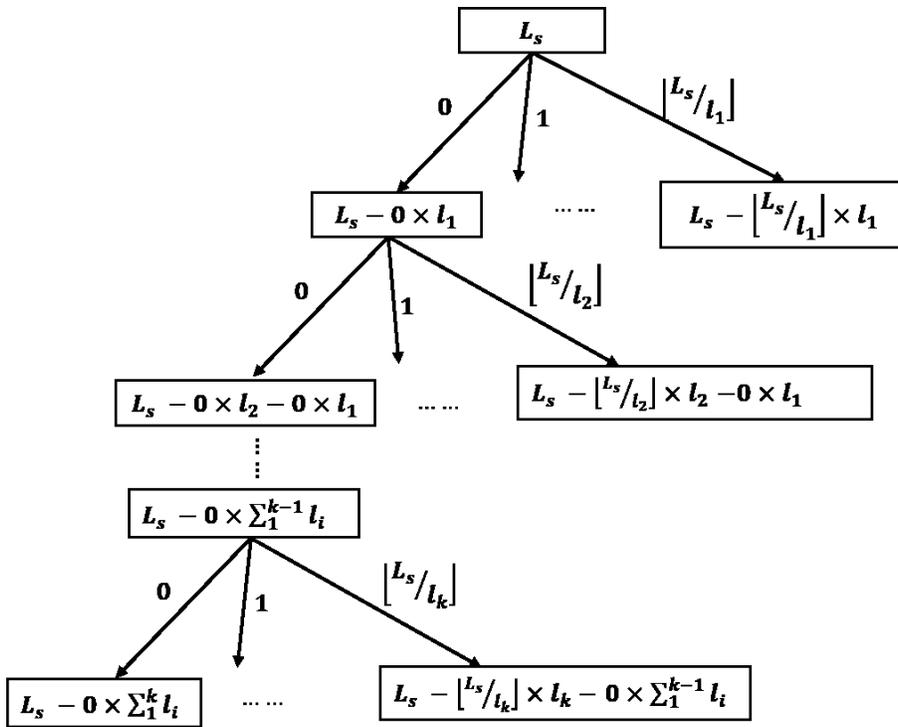
Figure 3-24: Tree structure for generating possible cutting scenarios
