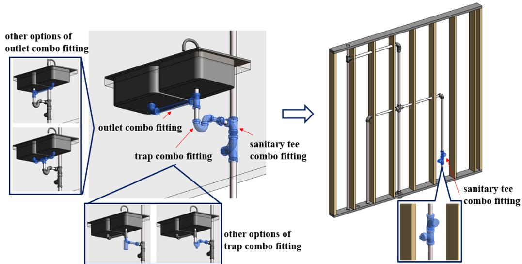
Figure 3-11: Combo fitting design for a kitchen sink with double basins
