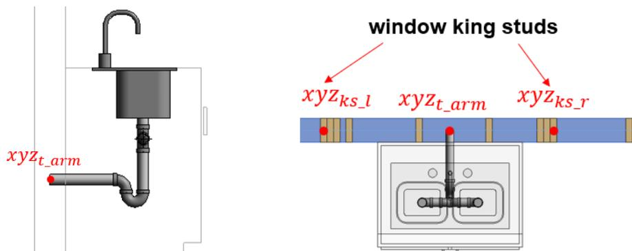
(a) Section view of kitchen sink drainage pipe design
