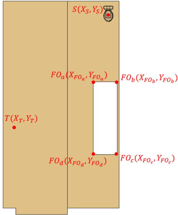
Figure 3-20: Start and terminal points and vertices points of a floor opening
