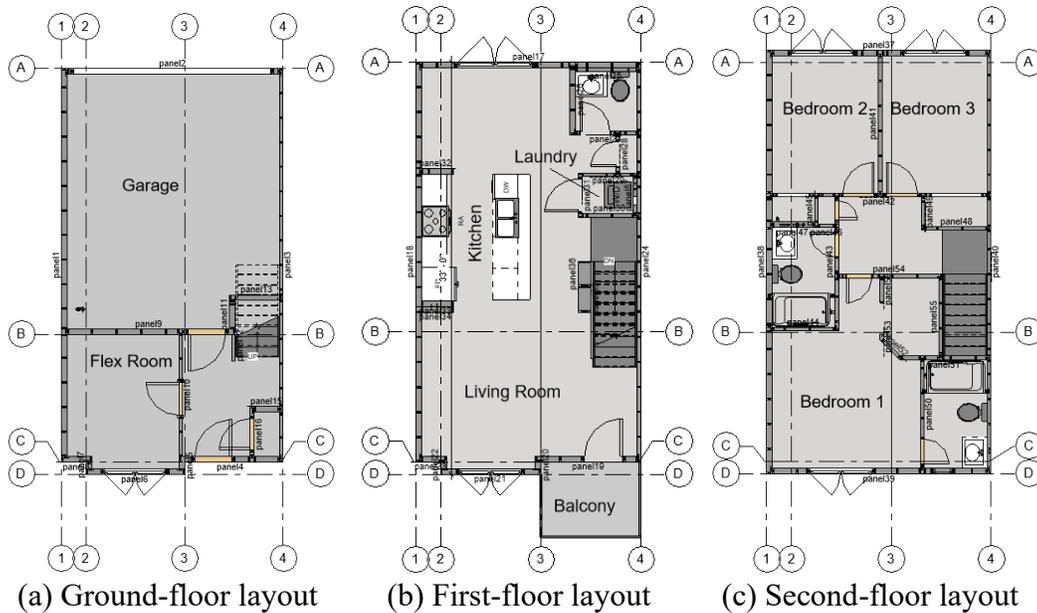
Figure 4-2: Sample model of floor layouts in one unit building
