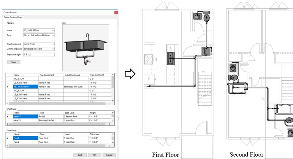
Figure 4-10: Drainage pipe generation
