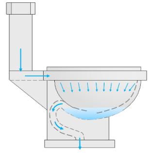
(b) Elevation view of water closet's integrated trap
