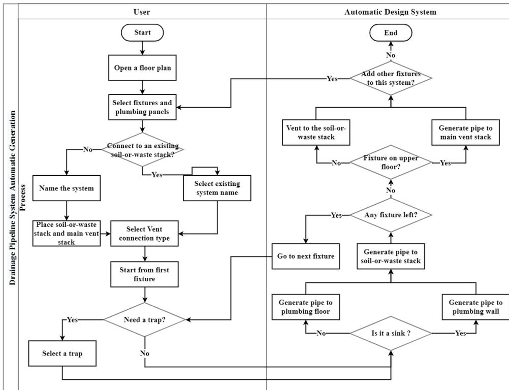
Figure 4-4: Cross-functional flowchart of automated design system
