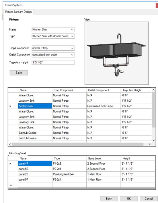
Figure 4-7: Windows Form for fixture drainage pipe design
