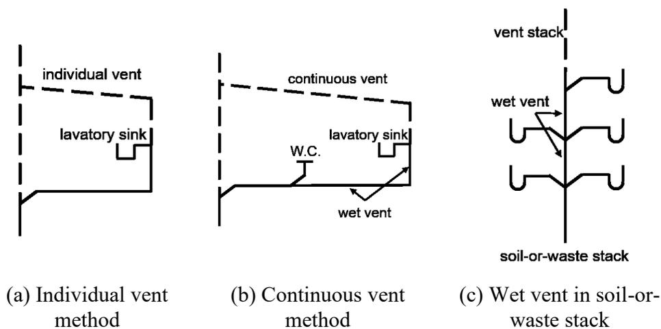
Figure 3-5: Methods of venting a plumbing fixture
