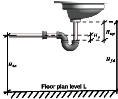
Figure 3-18: Fixture outlet and trap arm height relationship
