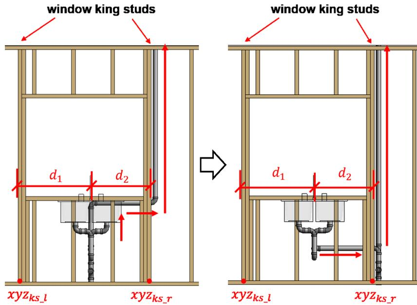
Figure 3-16: Vent pipe design for window opening in the wall
