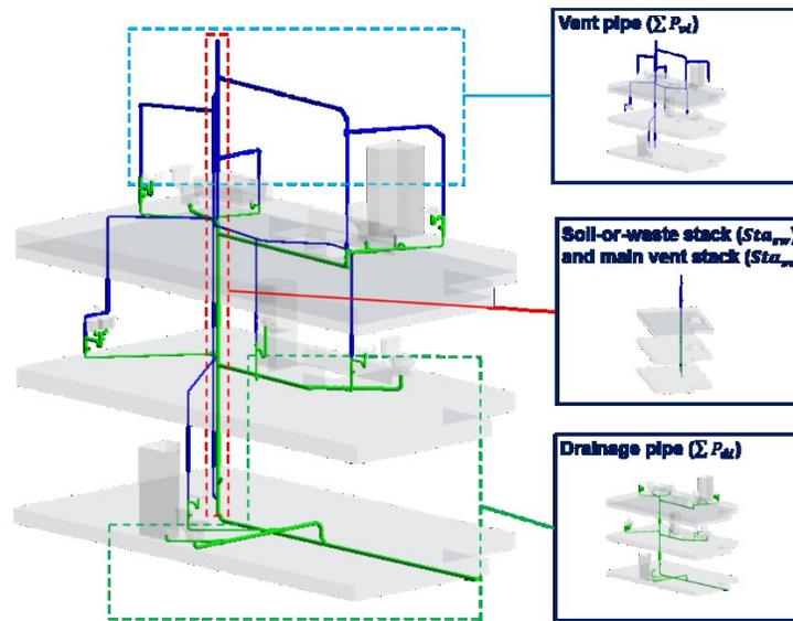
Figure 3-2: Drainage system (DS) 3D view
