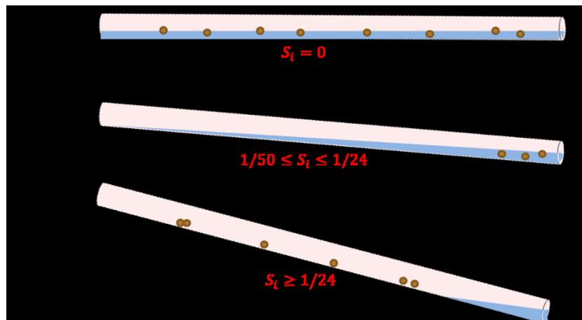
Figure 3-4: Effect of pipe slope on drainage
