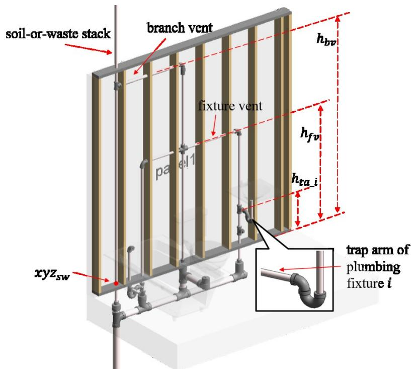
Figure 3-13: One fixture to one vent design option
