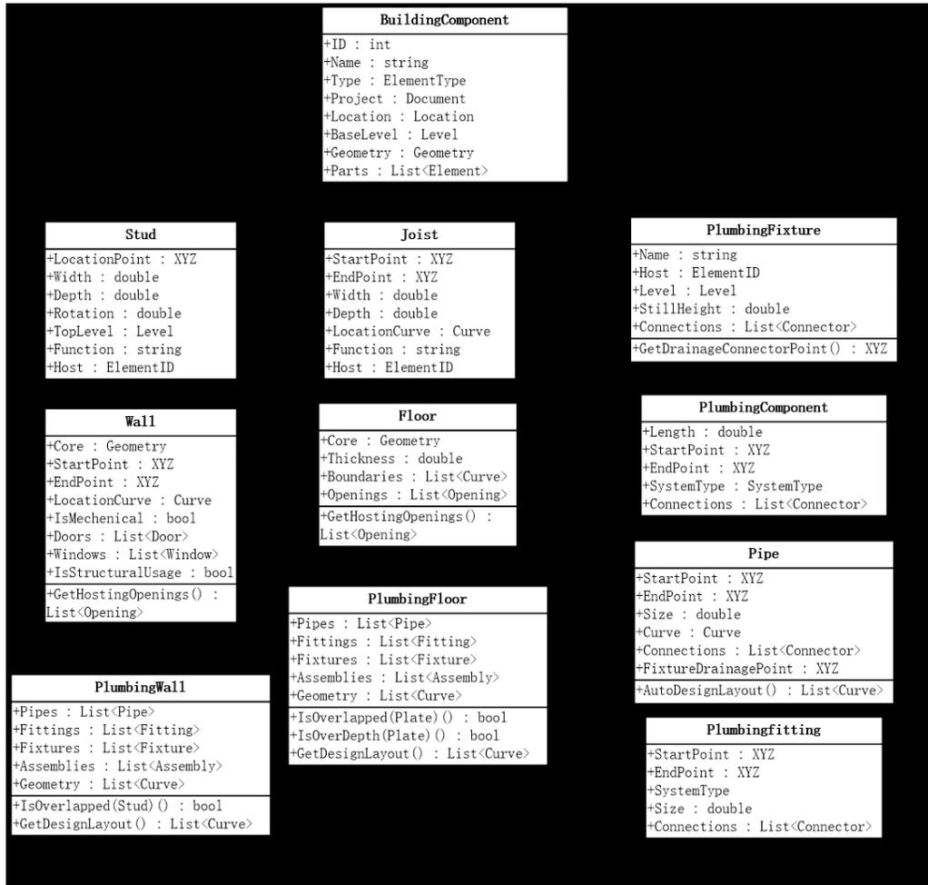
Figure 4-5: Excerpt of BIM information for drainage system design using UML
