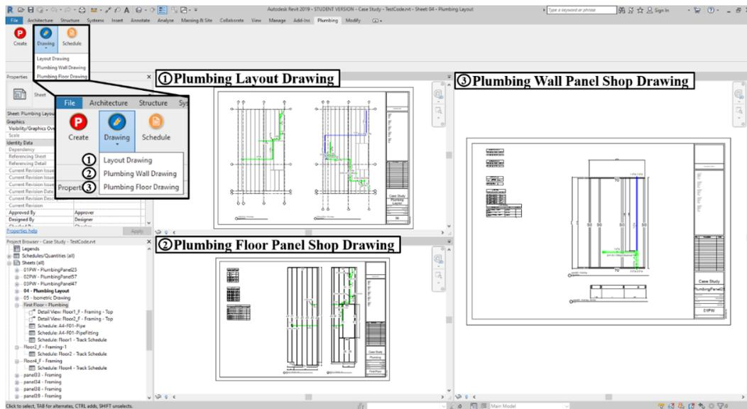
Figure 4-8: Shop drawing samples for drainage system in Revit
