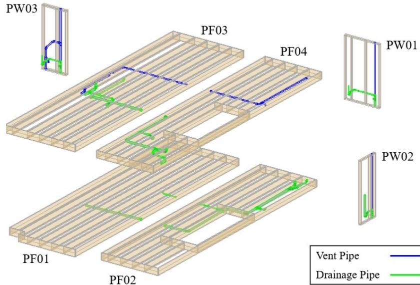
Figure 4-11: Panelized drainage system for one unit building
