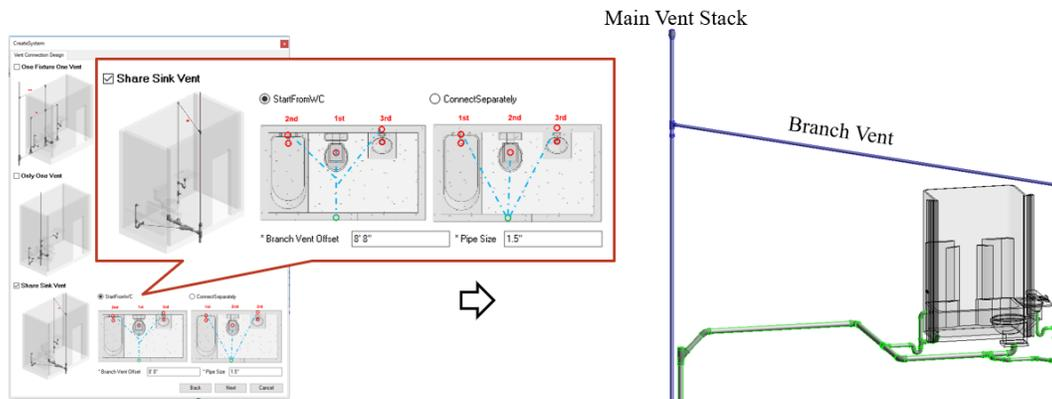
Figure 4-9: Vent pipe design example for a bathroom on the second floor
