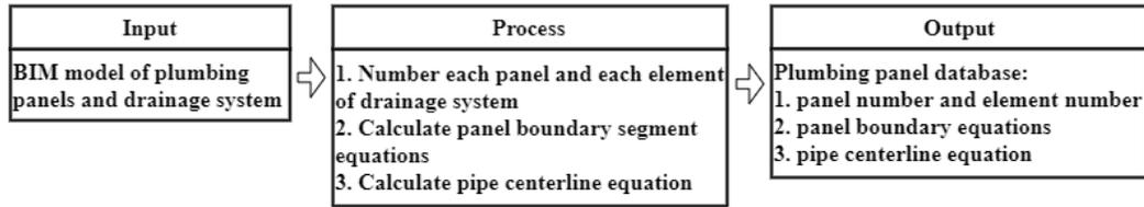
Figure 3-22: Flowchart of establishing database of plumbing panels
