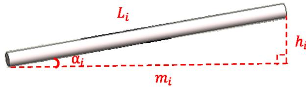
Figure 3-3: Pipe slope ( $S_i$ ) calculation
