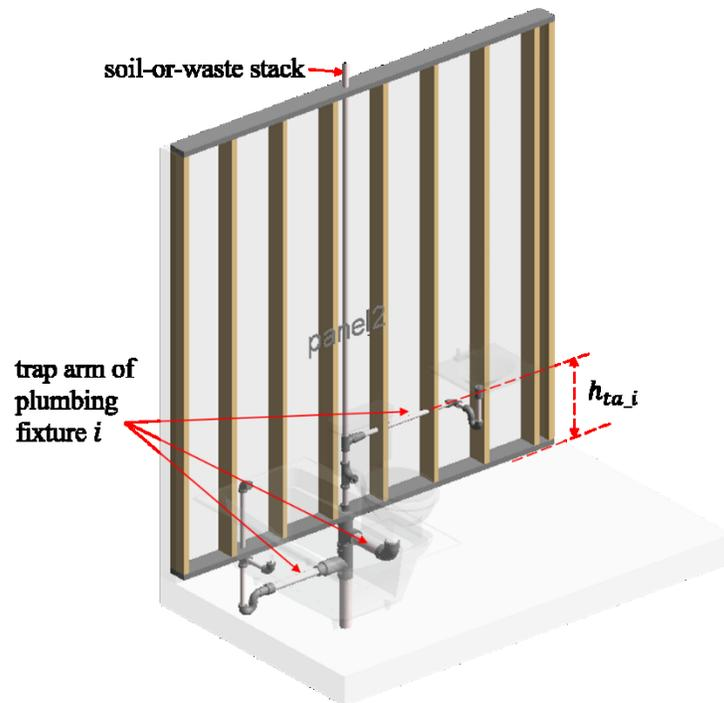
Figure 3-14: All fixtures to one vent design option
