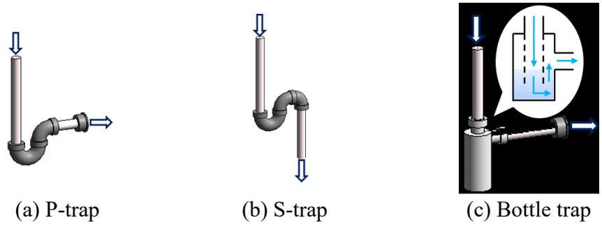
Figure 3-7: P-trap, S-trap and bottle trap examples
