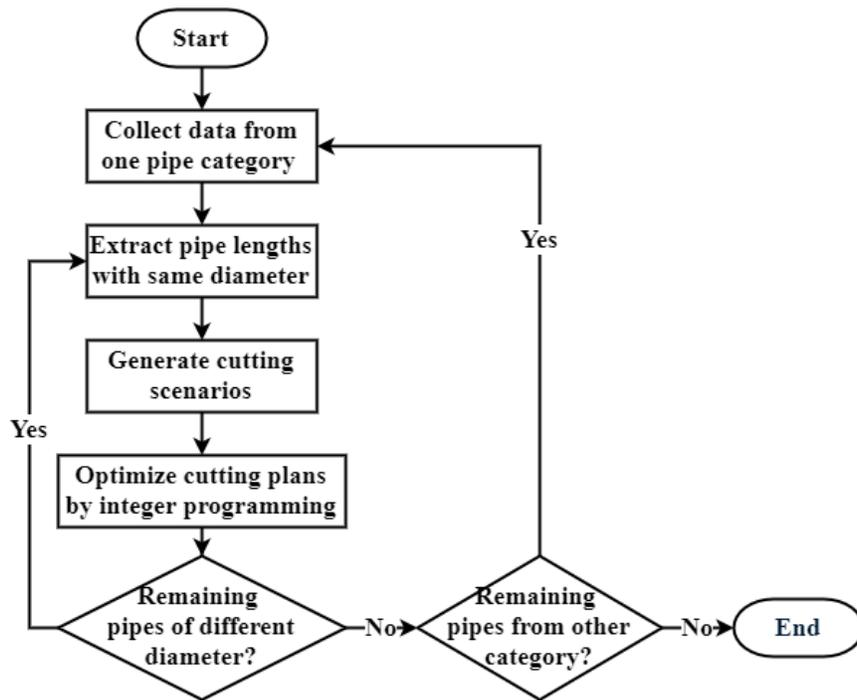
Figure 3-23: Cutting optimization process
