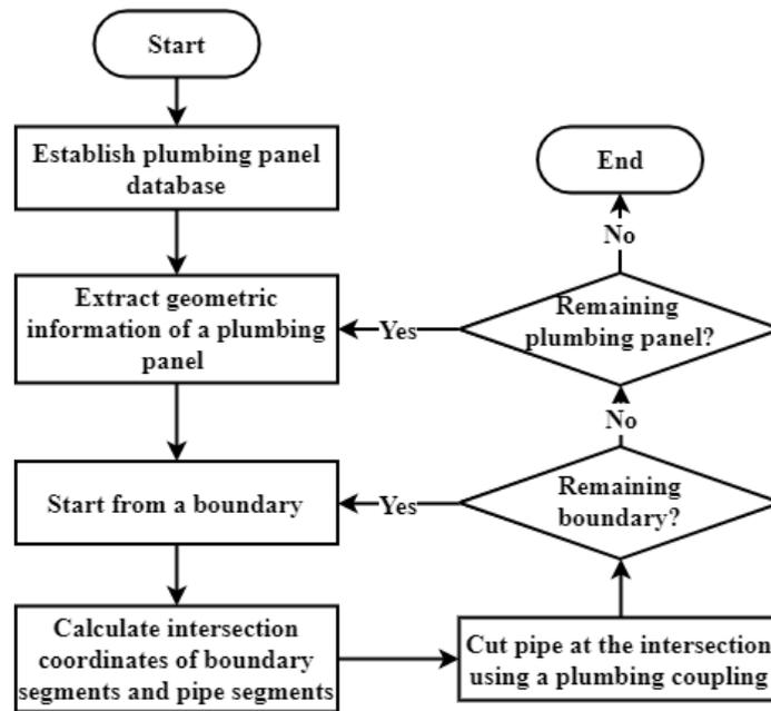
Figure 3-21: Flowchart of drainage system panelization planning algorithm
