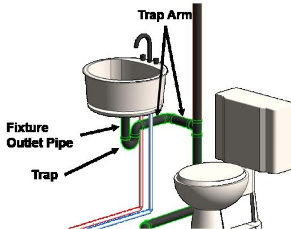
Figure 3-6: An example of a lavatory sink drain
