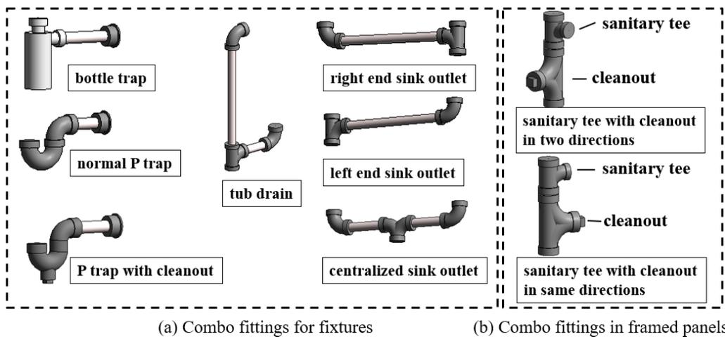
Figure 3-10: 3D view of combo fittings
