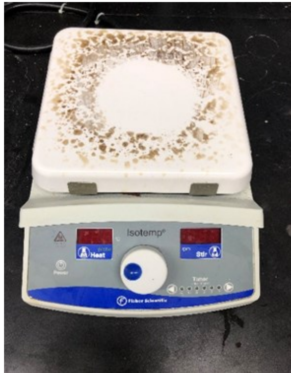
Figure 3.8: Magnetic Stirrer for Preparing Smaller Samples of Polymers
