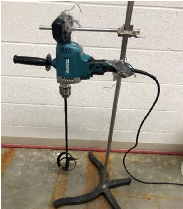
Figure 3.6: Overhead Mixer for Preparing Polymer Sample
