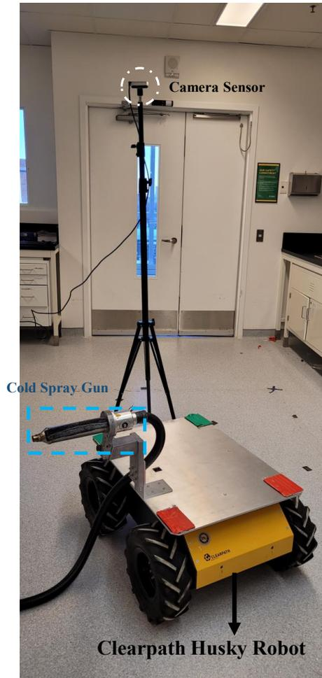
Figure 2.2: System setup including the Husky Robot made by Clearpath, cold spray gun, and camera sensor are shown. The goal is to estimate the position (two-dimensional) and orientation (one-dimensional) pose of the mobile robot.
