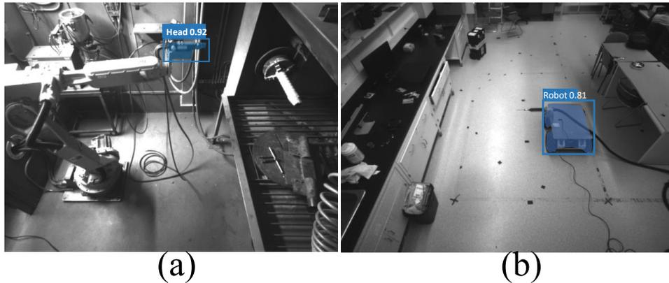
Figure 2.5: Accurately detecting the bounding boxes for the robots using OrientMask. The pixel contents of each bounding box are labeled using the segmentation framework, providing rich information on the 2D position of the target object in the image.
