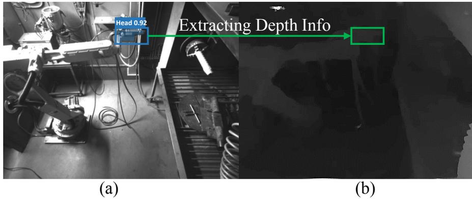
Figure 2.8: Extracting disparity info from the disparity image. This is done by applying the binary mask from the instance segmentation module to the depth image.
