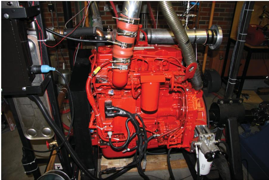
Figure 3.3: Cummins 4-cylinder QSB4.5 (Tier 3) Diesel Engine
