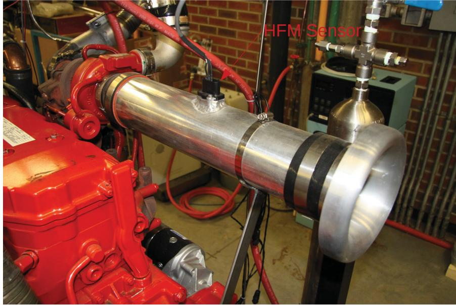
Figure 3.4: Custom air intake with HFM sensor
