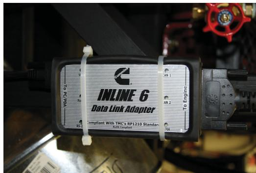
Figure 3.11: INLINE 6 Data Link Adapter from Cummins
