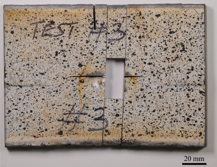
Figure 3 Photo showing sample 3 cut-off for fracture analysis.
