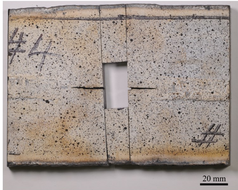
Figure 5 Photo showing sample 4 cut-off for fracture analysis.
