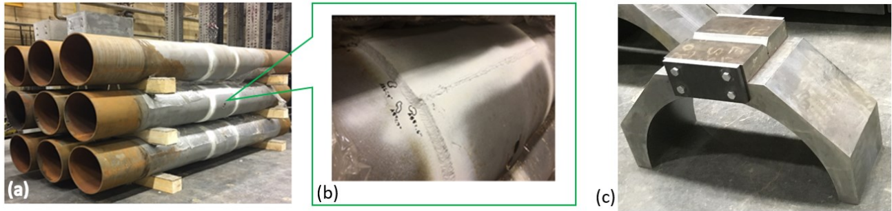
Figure 4-1 Photographs of: (a) Pipe specimens, (b) Sleeved girth weld and (c) Pipe cradle.
