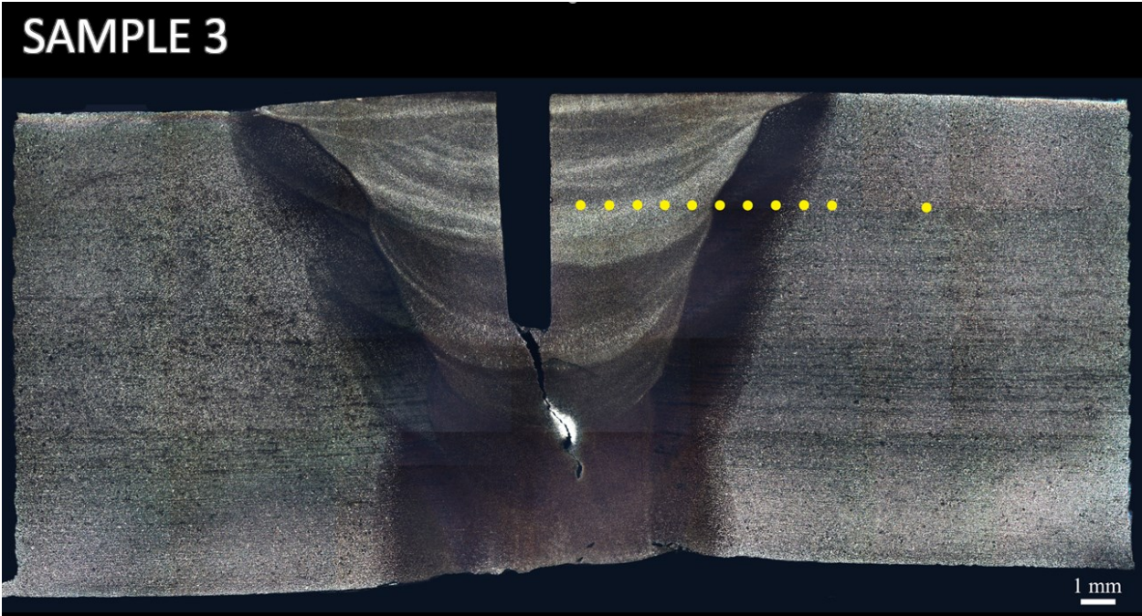
Figure 24 Sample 3 showing the approximate locations of indentations
