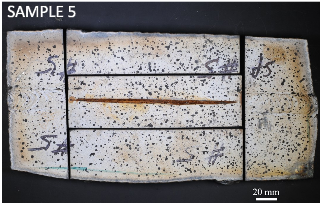
Figure 7 Photo showing sample 5 cut-off for fracture analysis.
