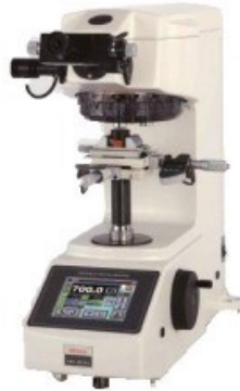
Figure 20 The Mitutoyo Micro Vickers hardness indenter
