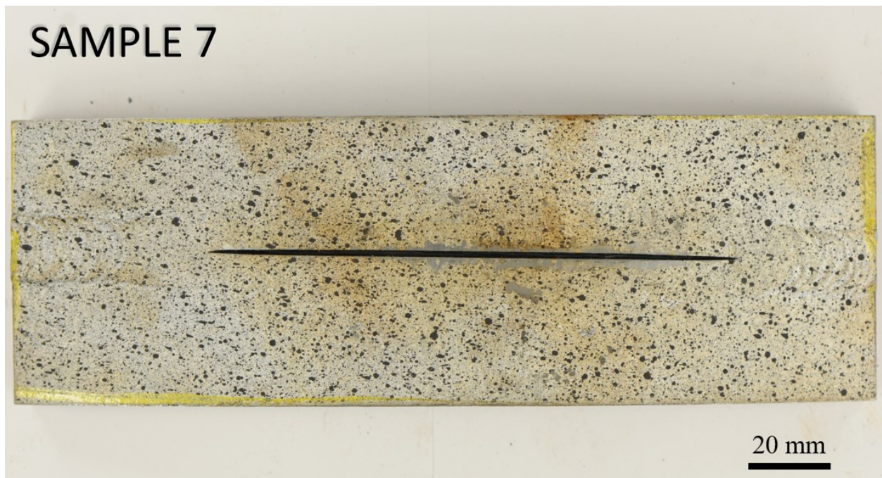
Figure 12 Photo showing sample 7 cut-off for fracture analysis.
