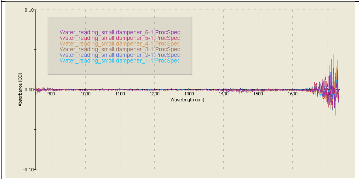
Figure 4-17 Improvement in the variation of the baseline of fully developed flow
