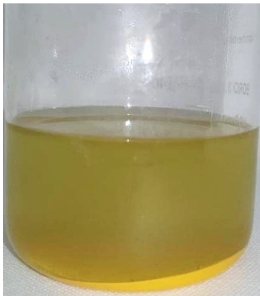
Figure 4. 7 Yellow \text{H}_2\text{WO}_4 precipitates with extended thermal decomposition duration to 2 more hours.
