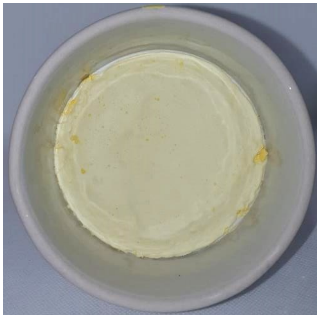
Figure 3. 8 Yellow \text{H}_2\text{WO}_4 precipitates contamination in the resulting \text{CaSO}_4 filter cake obtained from the 2-step method.
