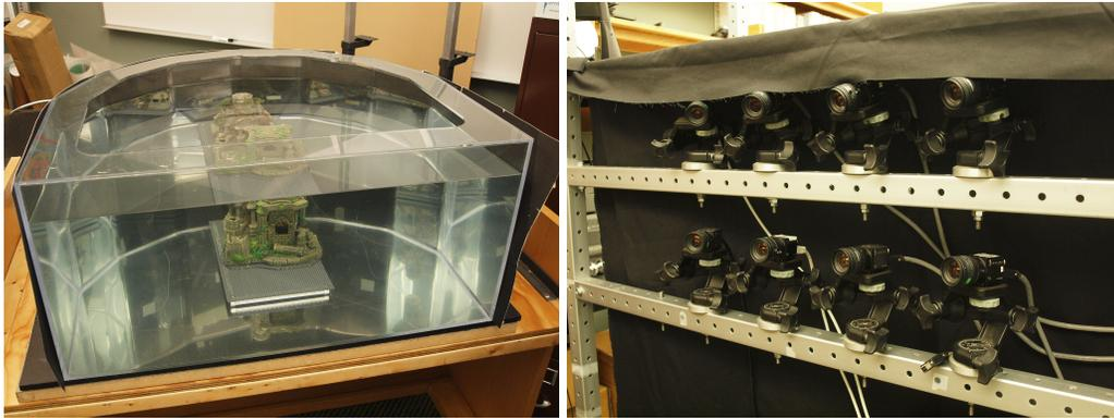
Figure 5.19: Experimental setup for our real data experiments. (Left) The scene set up inside an acrylic water tank. (Right) The camera array.
