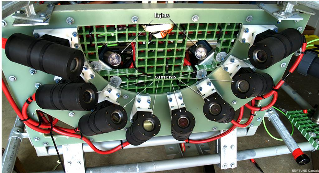
Figure 1.1: The underwater camera array deployed by Ocean Networks Canada under the NEPTUNE program [3].
