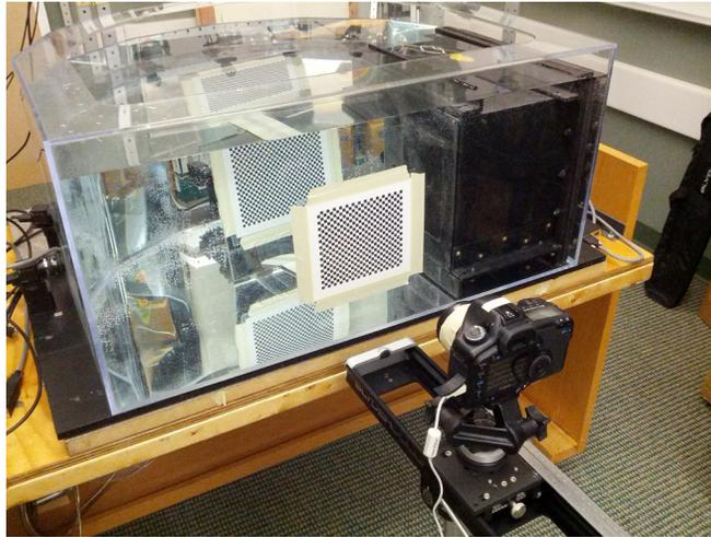
Figure 4.7: Experimental setup, showing the calibration device and a checkerboard inside the tank, a checkerboard affixed to the tank surface, and the camera mounted on a SliderDolly translation rail.
