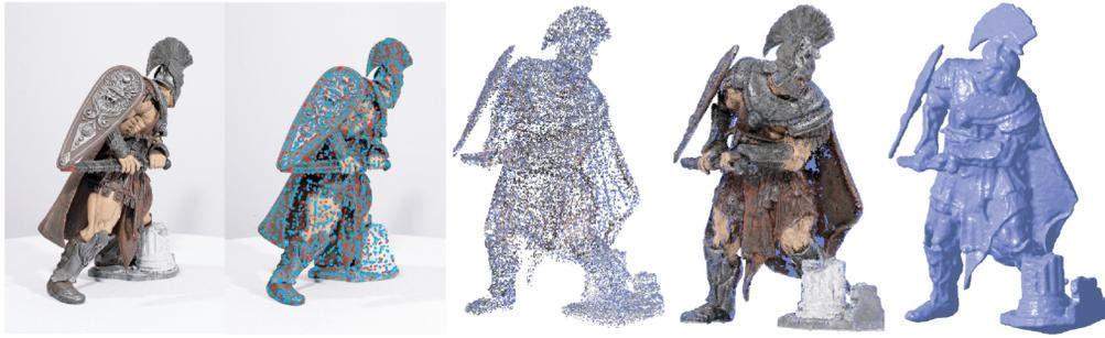
Figure 2.4: Example 3D reconstruction with PMVS2. Left to right: an example input image, detected features, initial patches, final patches after expansion and filtering, mesh model. Source: [18]
