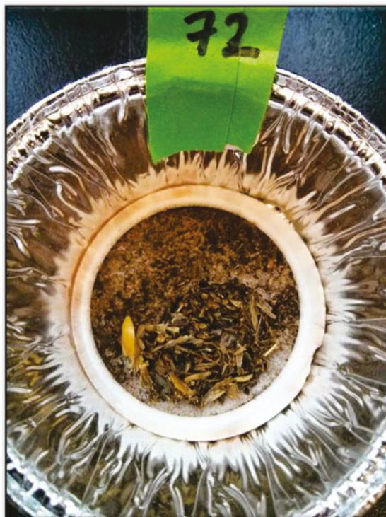
Photo 23. LF recovery from Lethbridge wheat-fallow 2 mm roller mill soil
