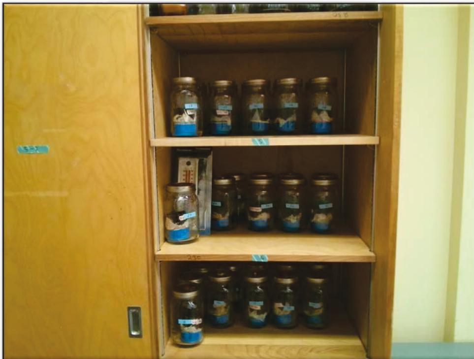
**Photo 11. Closet used to house the incubation chambers during the experiment**
