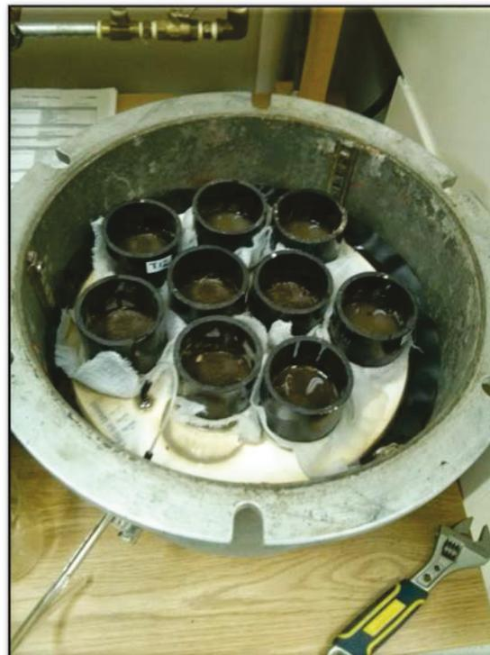
**Photo 8. Saturated soil cores before pressure extraction**
