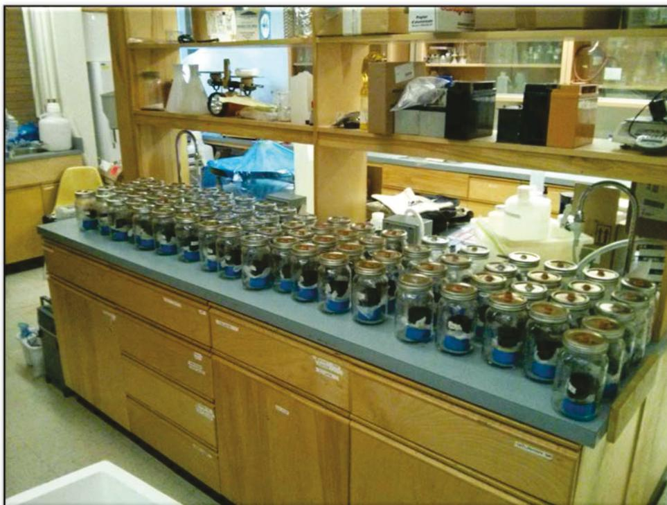
**Photo 9. Prepared incubation chambers with soil samples**
