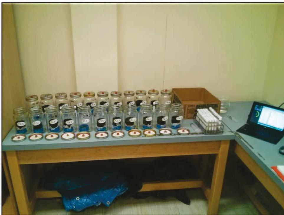
**Photo 10. Headspace sampling event. Front row equilibrating with ambient atmosphere**
