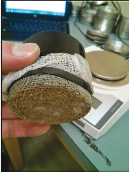
**Photo 17. Soil sample holder with intact cheesecloth at the of incubation**
