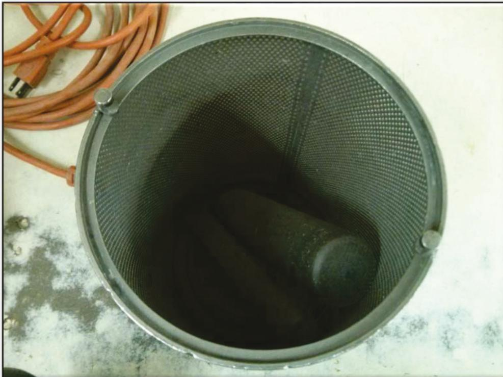
**Photo 2. Single drum of 2 mm roller mill showing internal rollers**
