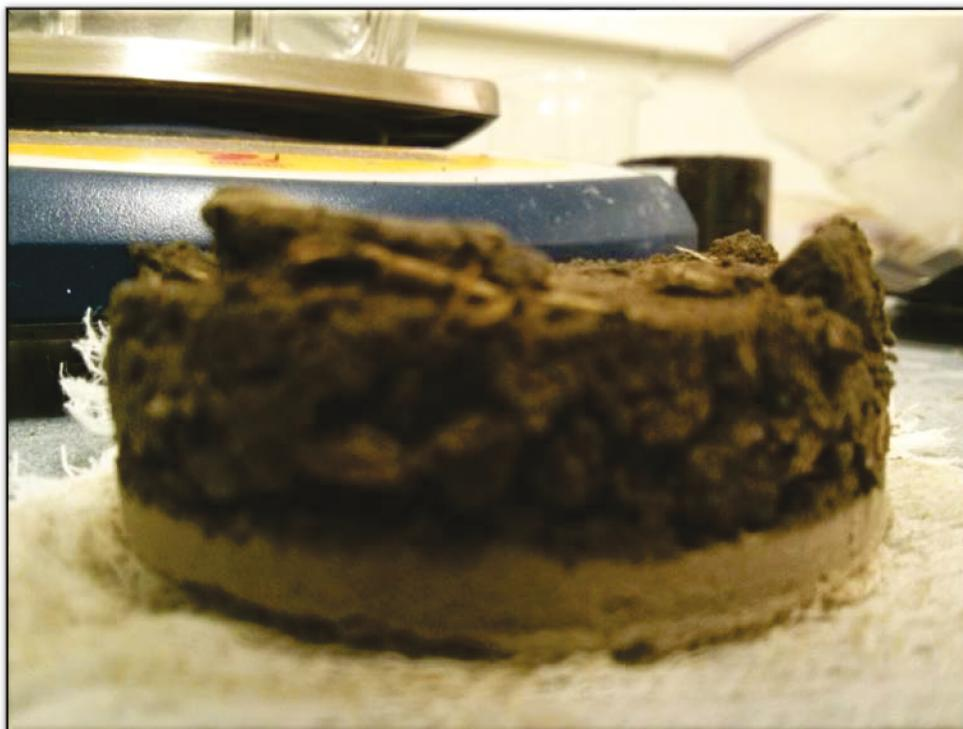
**Photo 12. Intact soil sample after incubation**
