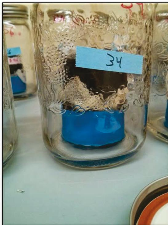
Photo 13. Soil sample holder inside incubation chamber
