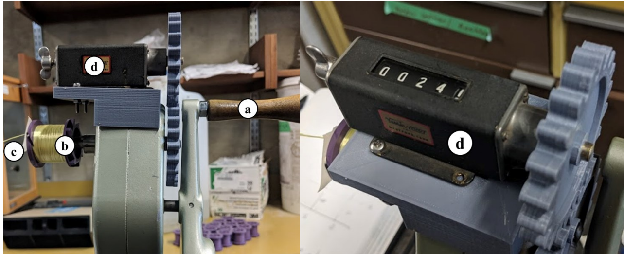
Figure 3-4: Images of custom twist counter. The handle (a) is rotated to turn the braider bobbin (b) and twist the yarn (c) about its axis. The analog counter (d) records the number of turns of the braider bobbin.
