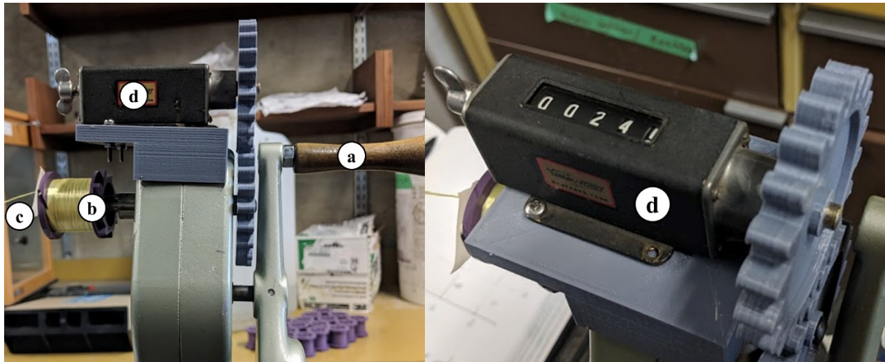
Figure 6-2: Images of custom twist winder. The handle (a) is rotated to turn the braider bobbin (b) and twist the yarn (c) about its axis. The analog counter (d) records the number of turns of the braider bobbin.
