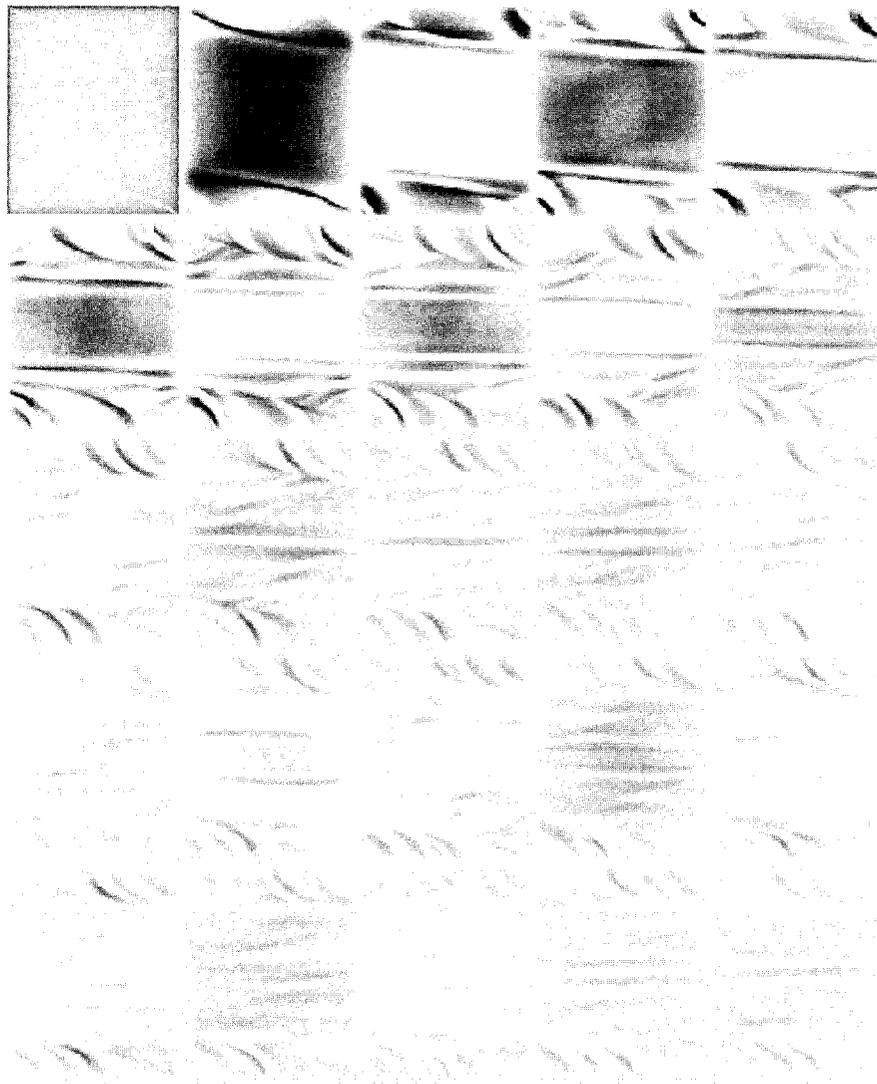
**Figure 4.13** Simulated FMR in a 4 micron square in a 45 Gauss DC field. Time scan at the center of the sample and spatial scans. First out of plane spatial scan frame is taken at  $t=33$  ps. Each additional frame 120 ps later. Initial state ( $t=0$  s) subtracted from all frames
