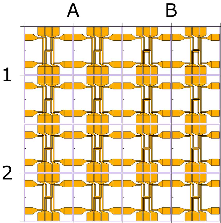
FIGURE 4.2: The full photomask design for the first generation of chips. The 18 mm square chips are tiled with  $500 \mu\text{m}$  spaces between chips. The variants of the design are distributed as shown in table 4.1.
