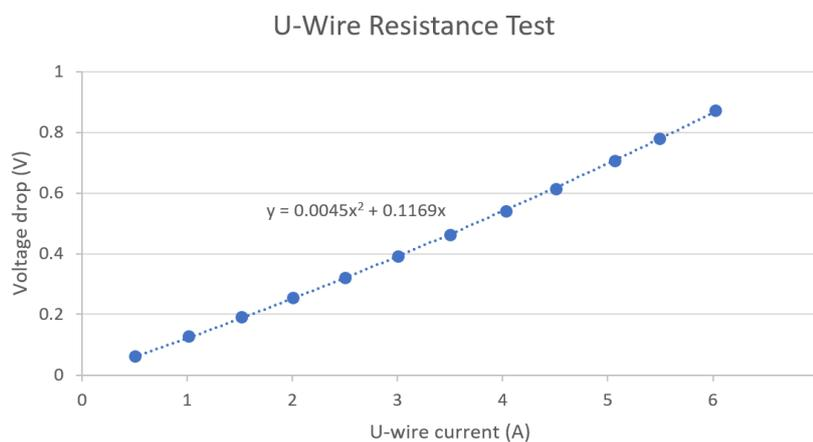
FIGURE 4.10: The results of the U-wire resistance test. The behavior appears linear, and thus ohmic, for all tested current values.
