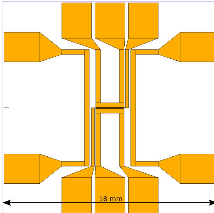
FIGURE 4.1: The original photomask design for a single chip. The trap geometry is identical to that described in figure 3.3. The solid structures correspond to opaque regions of the mask, which in turn correspond to metal coated regions on the final chip.
