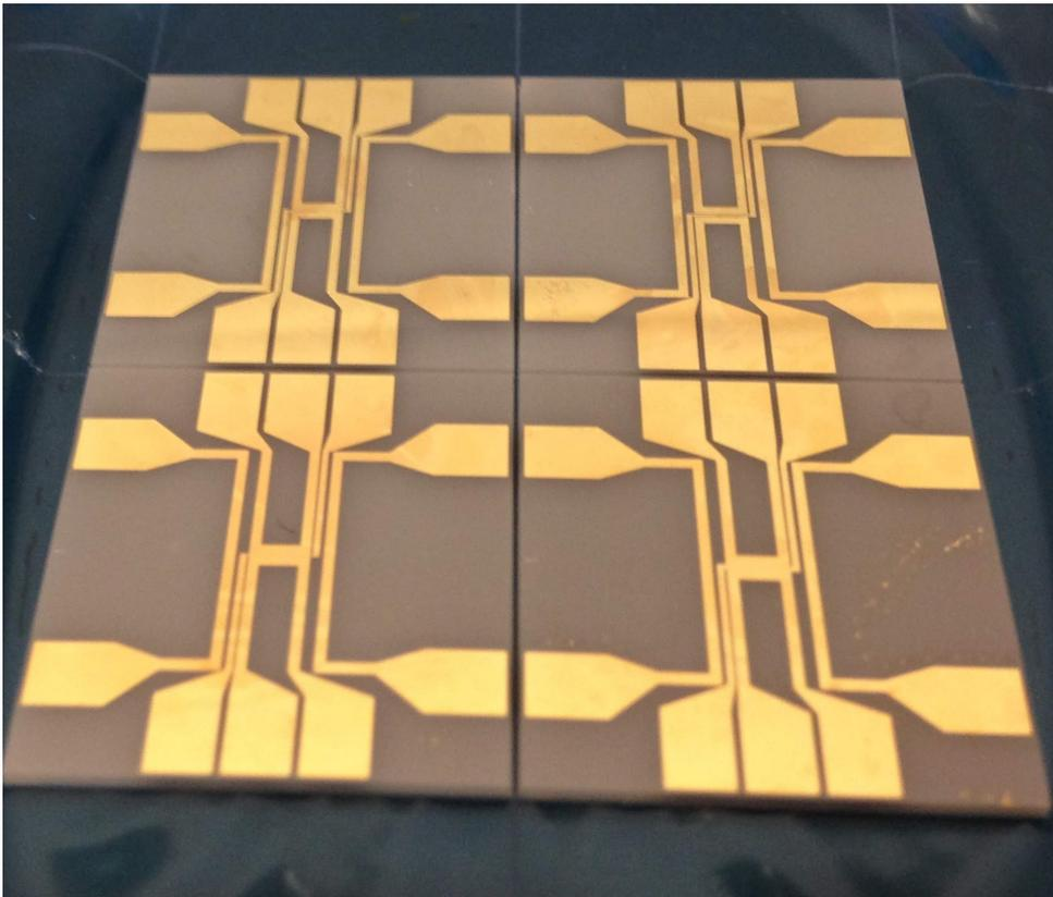
FIGURE 4.3: Pictured here are four first generation atom chips fabricated from a single substrate. Included are each of the four variants corresponding to the center four chips in figure 4.2.
