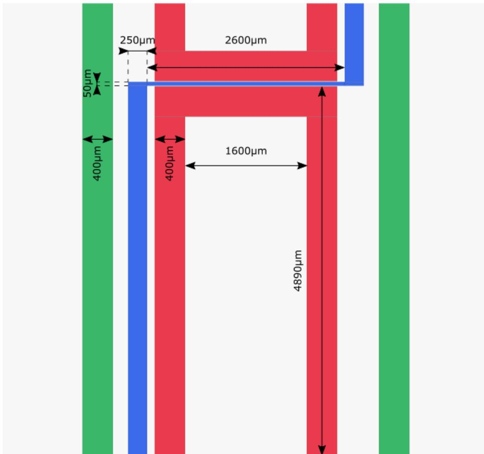
FIGURE 3.3: Schematic of our initial trap design. The Z wire (blue) serves as the main trapping wire. The two U wires (red) produce the required vertical bias field. The Ioffe wires (green) supply additional bias to eliminate the zero-field crossing.
