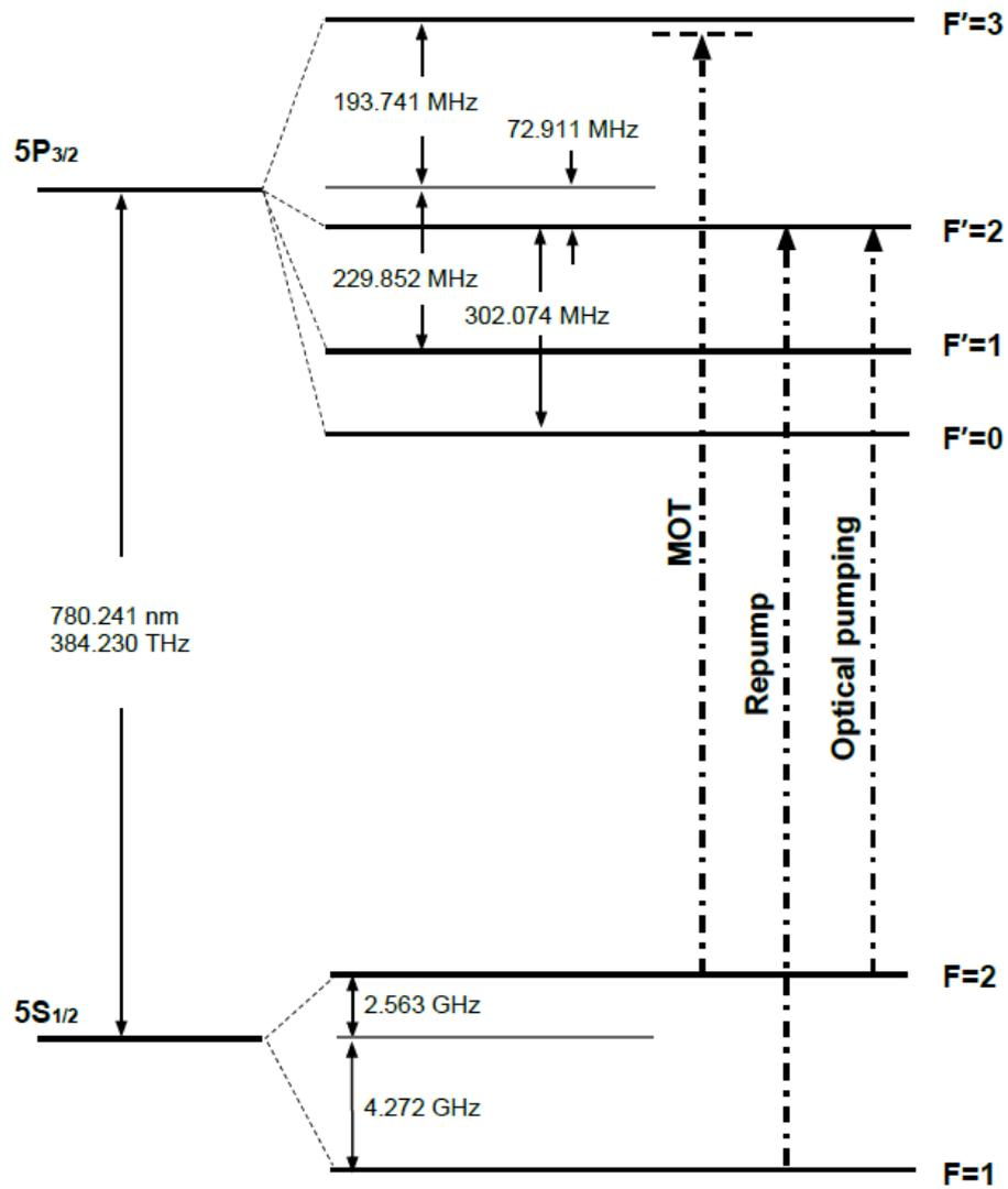
FIGURE 2.2: Hyperfine structure of the D2 line transitions of rubidium-87. Adapted from [17].
