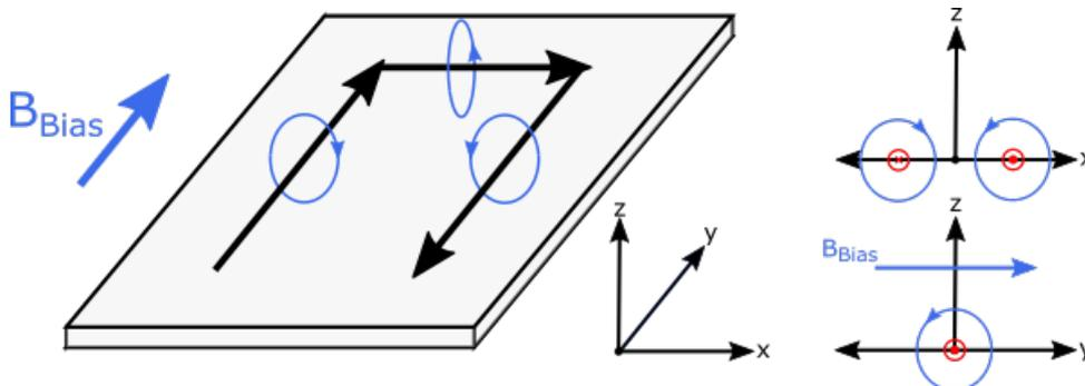
FIGURE 3.1: Example U-trap wire configuration. Current direction indicated by black arrows. A zero point in the magnetic field amplitude is achieved through the summation of the four component fields (blue).
