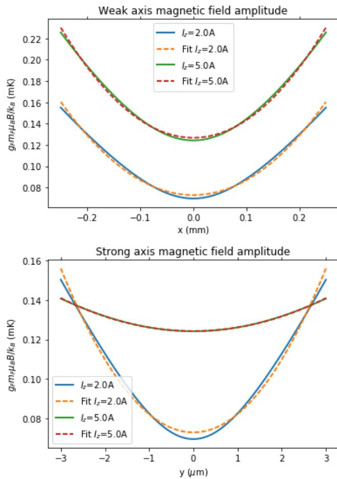
FIGURE 3.6: Quadratic fits to the simulated magnetic fields for trap frequency calculation. For visual clarity only the 2 A and 5 A cases are shown.
