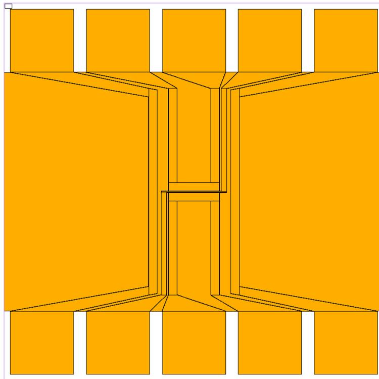
FIGURE 4.6: The second generation atom chip design. The entire surface is covered in metal with a  $10\ \mu\text{m}$  gap around the wire segments. Additionally, the contact pads are evenly distributed along opposite ends of the chip and have been increased in size to 3 mm squares.
