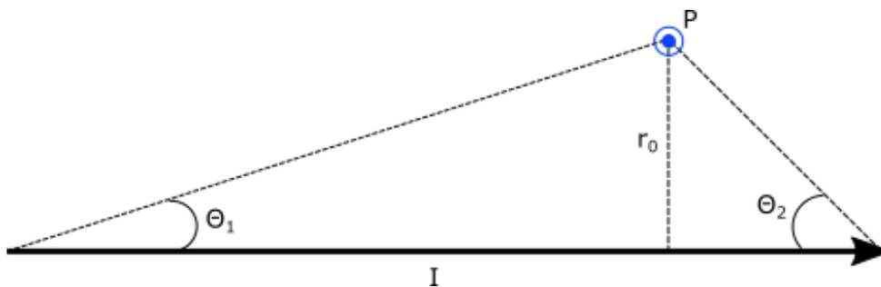
FIGURE 3.4: The geometry specified in equation 3.6 to calculate the magnetic field at point P for a given current  $I$  using the infinitely thin, finite length wire approximation.
