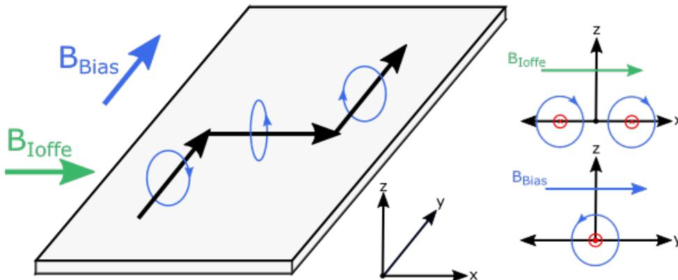
FIGURE 3.2: Example Z-trap wire configuration. Current direction indicated by black arrows. A minimum in the magnetic field amplitude is achieved through the summation of the four component fields (blue). An optional Ioffe field (green) can be applied to guarantee the absence of a zero crossing in the  $x$  component.
