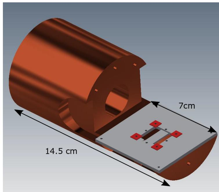
FIGURE 2.4: The simplified chip mount created by Daniel To. The central platform has been reduced from a complex sliding platform to a simple removable plate. The chip would be mounted over the hole in the center platform with the electrical connections supplied by wires running through the large circular opening in the main block of the mount.
