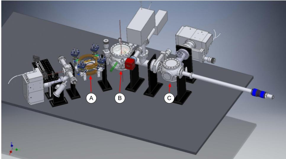
FIGURE 2.1: Schematic of hybrid system apparatus. Highlighted are the preparation region (A), the science chamber (B), the loading chamber (C). The entirety of the vacuum chamber system has been constructed with the exception of the loading arm extending from the loading chamber.
