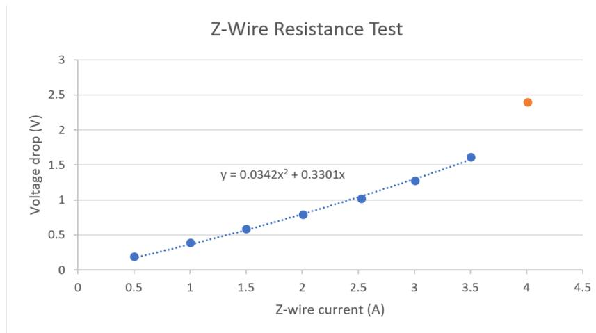
FIGURE 4.9: The results of the Z-wire resistance test. The behavior appears linear and is thus consistent with ohmic behavior. At 4 A of current (orange) the chip lost contact with the heat sink and the silver epoxy began to burn, destroying the chip.
