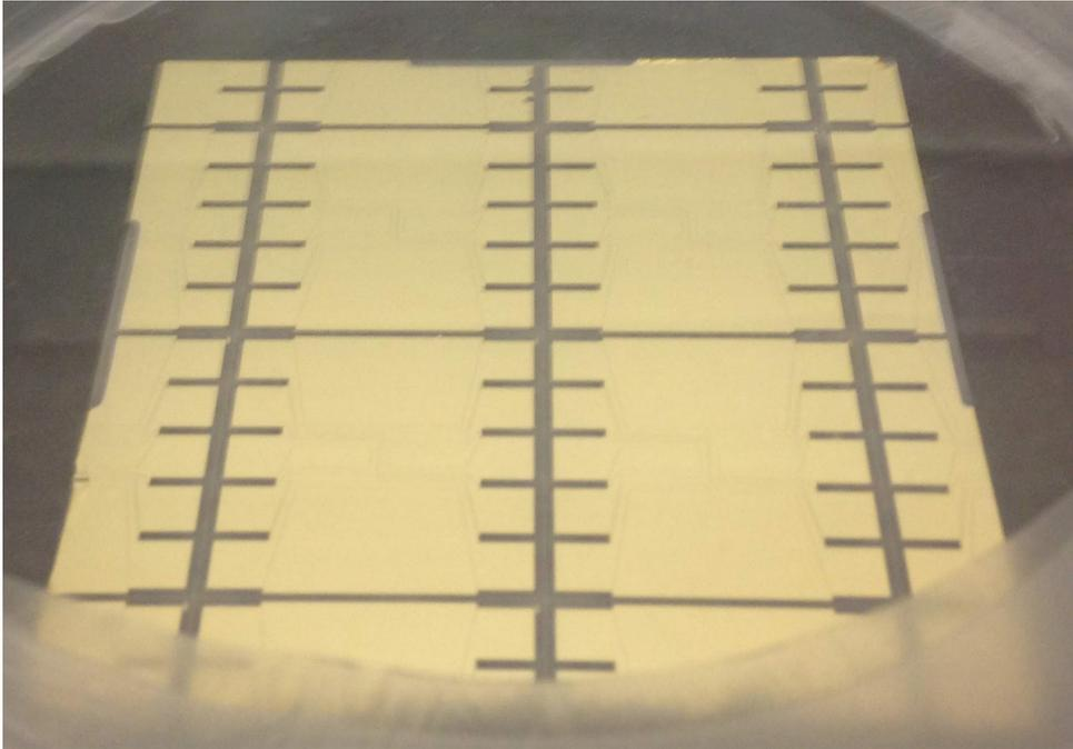
FIGURE 4.7: Pictured here is the partially completed second generation atom chips. The substrate includes four variants in the chip design and has undergone all stages of the fabrication up to the completion of the lift-off process.
