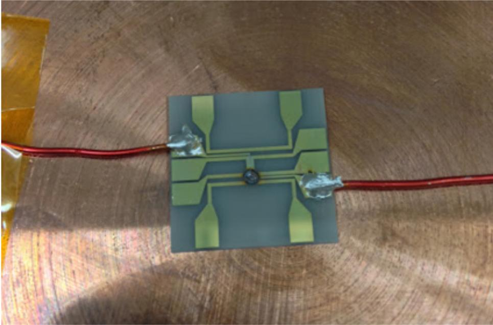
FIGURE 4.8: Pictured here is the damaged chip from the absolute current limit test of the Z-wire. The burned area is visible slightly below the center of the chip.
