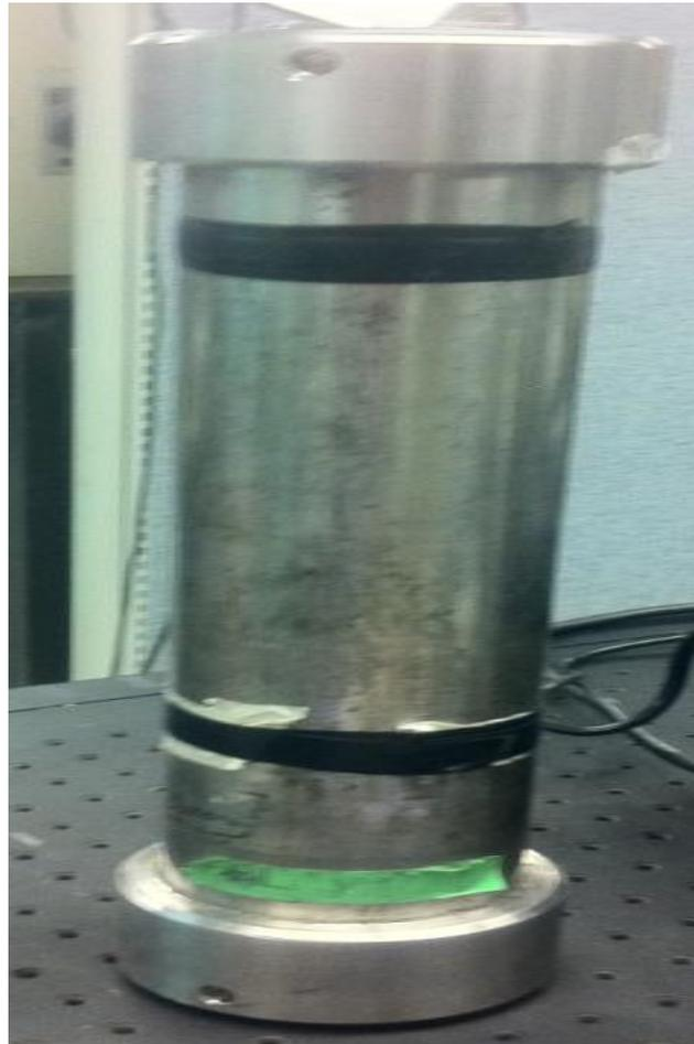
Figure 5.11 High pressure cell
