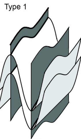
Figure 18. Type 1 fold interference pattern.
