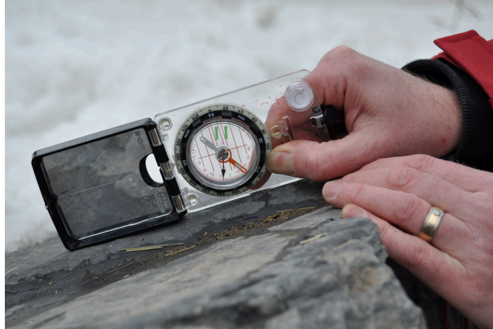
Figure 2: Compass-clinometer used to measure an inclination – in this case the dip of a bedding plane.
