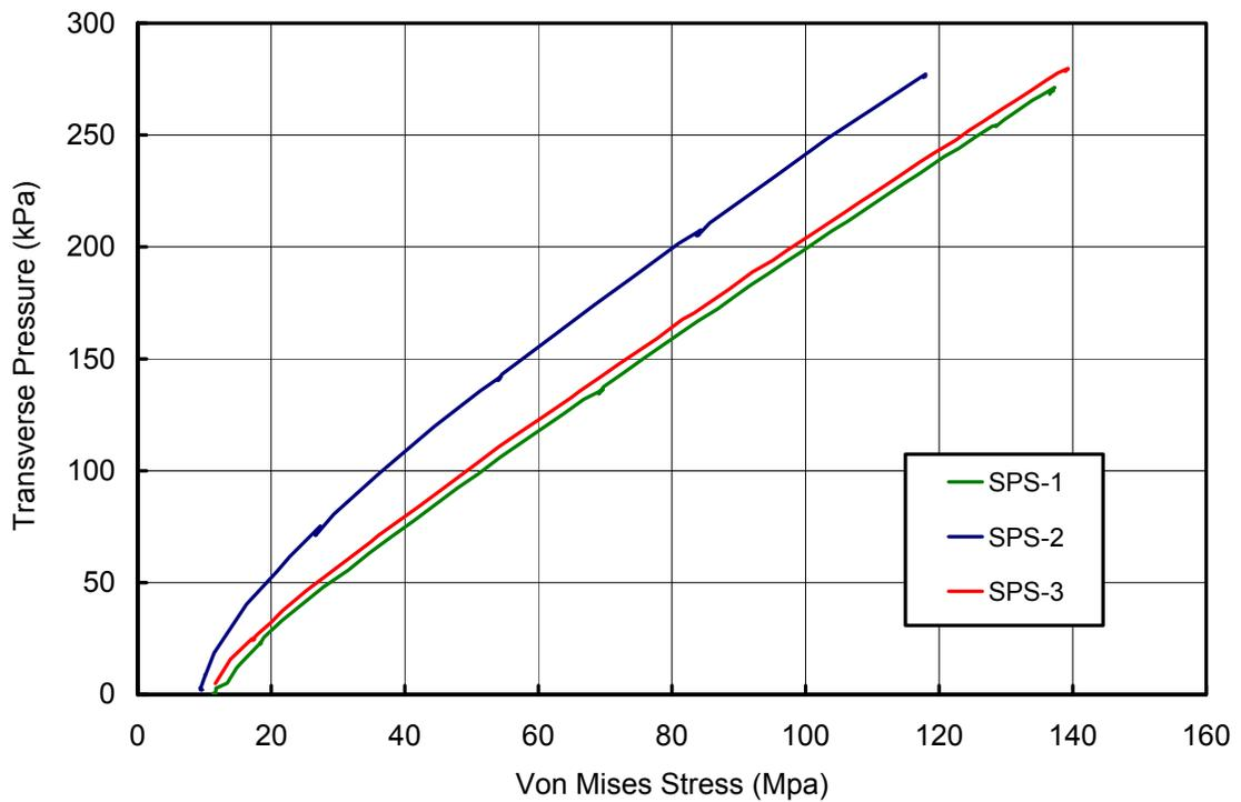
Figure 4.10: Transverse Pressure versus Average Panel Midpoint von Mises Stress
