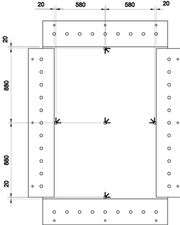
Figure 3.31: Strain Rosette Layout
