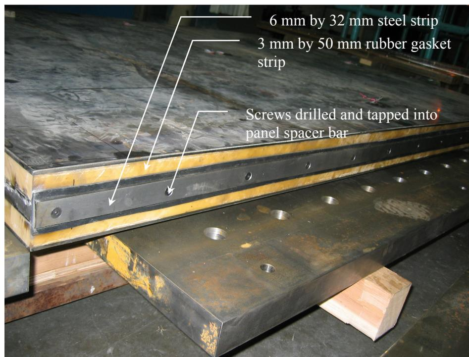
**Figure 4.20: Extra Neoprene Edge Gasket and Steel Retaining Strip added to SPS-3 Specimen Set**
