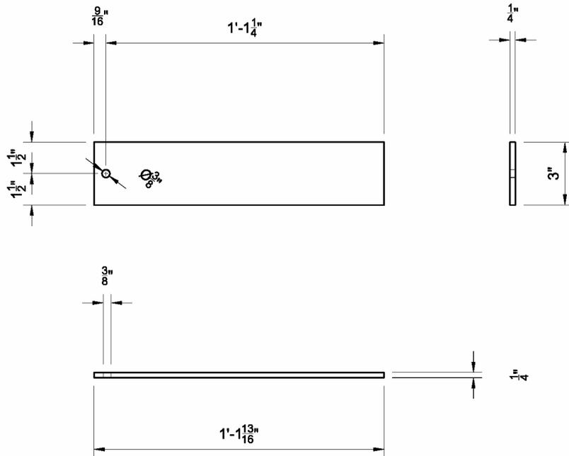
**Figure A10: Outer Bearing Plate for Roller Bearing Assemblies (20 Pieces Required) – Fabrication Drawing with Imperial Units**
