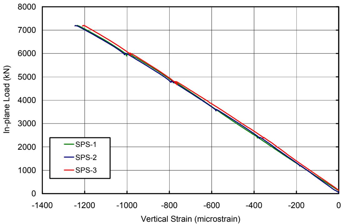
**Figure 4.2: In-plane Load versus Average Vertical Panel Strain for Axial Load of 7200 kN and No Lateral Pressure**
