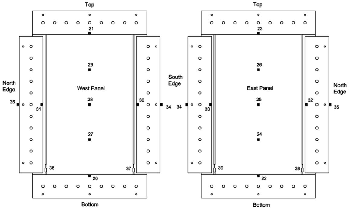
**Figure 3.35: Channel Numbers Corresponding to LVDT Positions**
