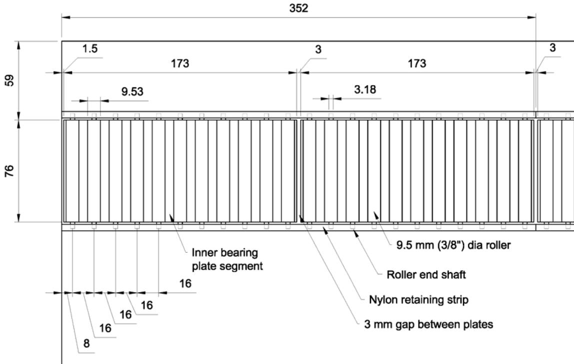
Figure 3.17: Plan View of Portion of Roller Bearing Assembly
