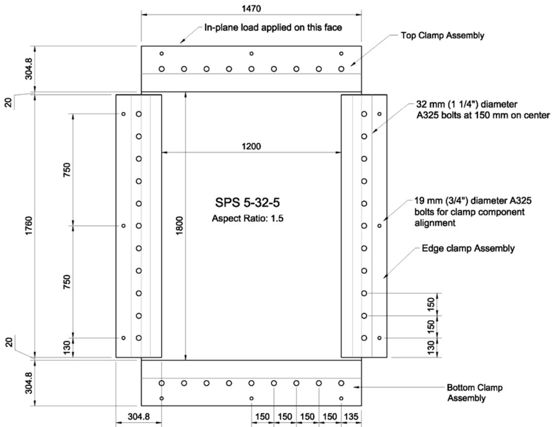
Figure 3.9: Plan View of Test Frame
