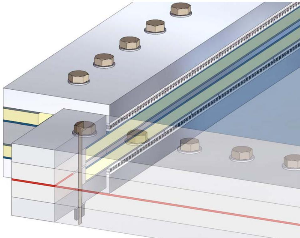
**Figure 3.19: Rendered Cutaway View of Portion of Roller Bearing Assembly**
