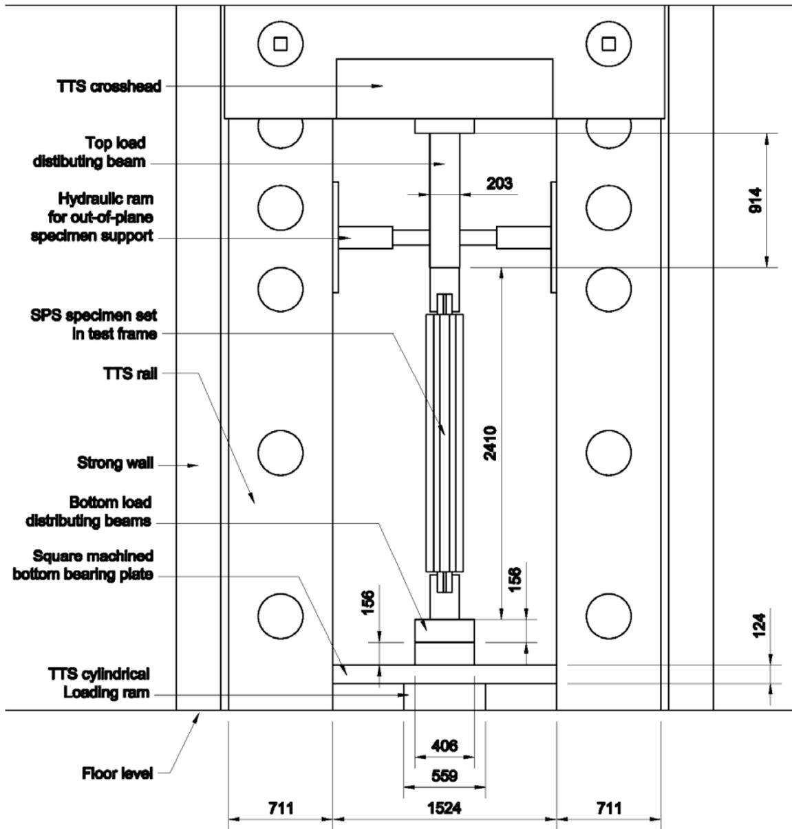
Figure 3.26: Specimen Mounted in the Testing Machine – Front View
