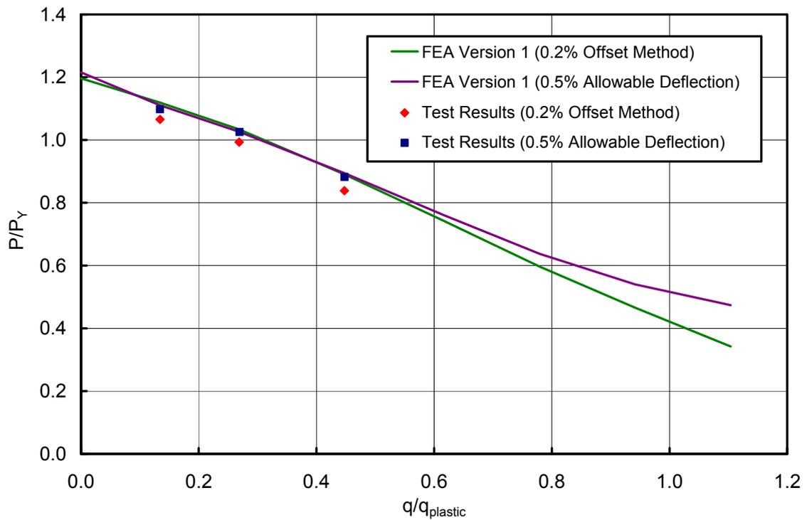
Figure 5.12: Interaction Diagram - FEA Version 1 and Test Results
