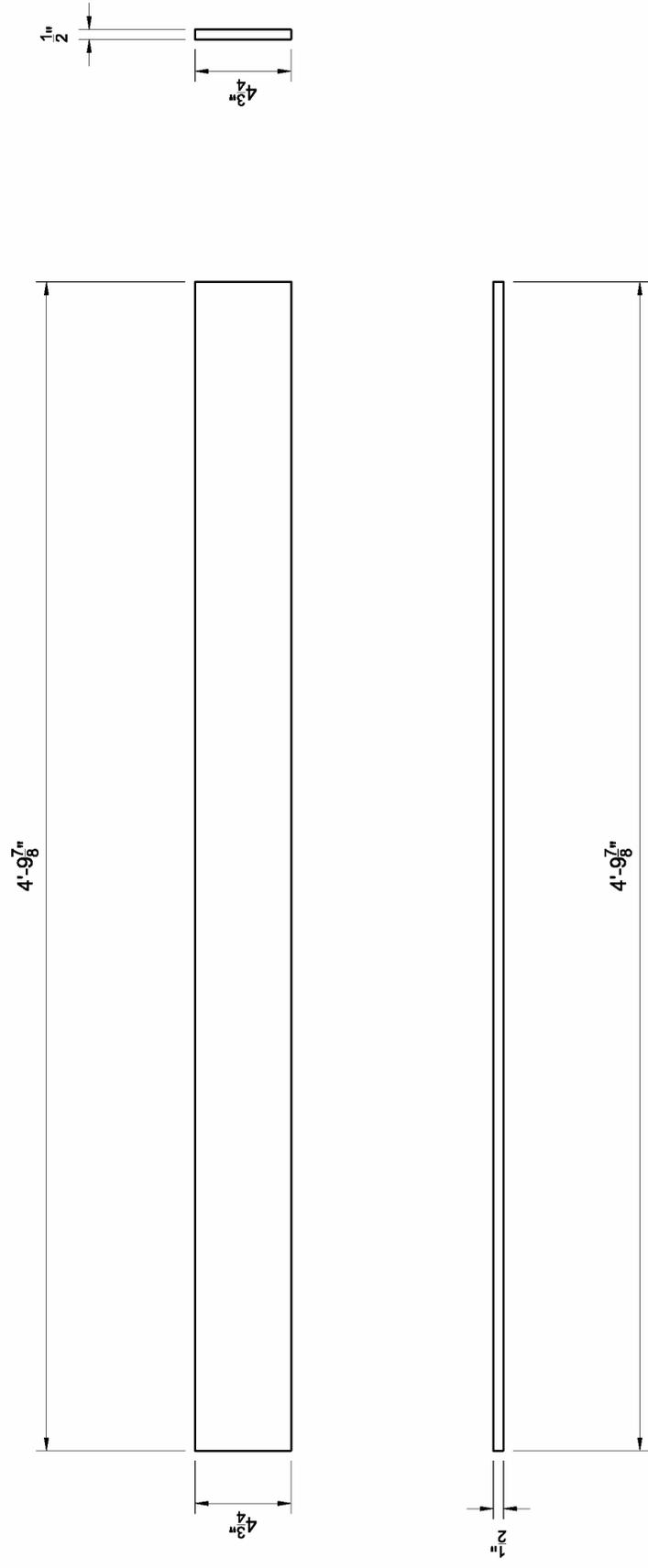
Figure A5: Top Panel Spacer Bar (2 Pieces Required per Specimen Set) – Fabrication Drawing with Imperial Units
