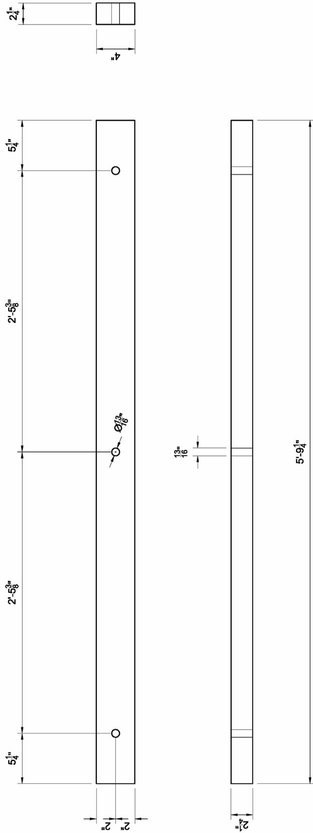
Figure A4: Edge Clamp Spacer Bar (2 Pieces Required) – Fabrication Drawing with Imperial Units
