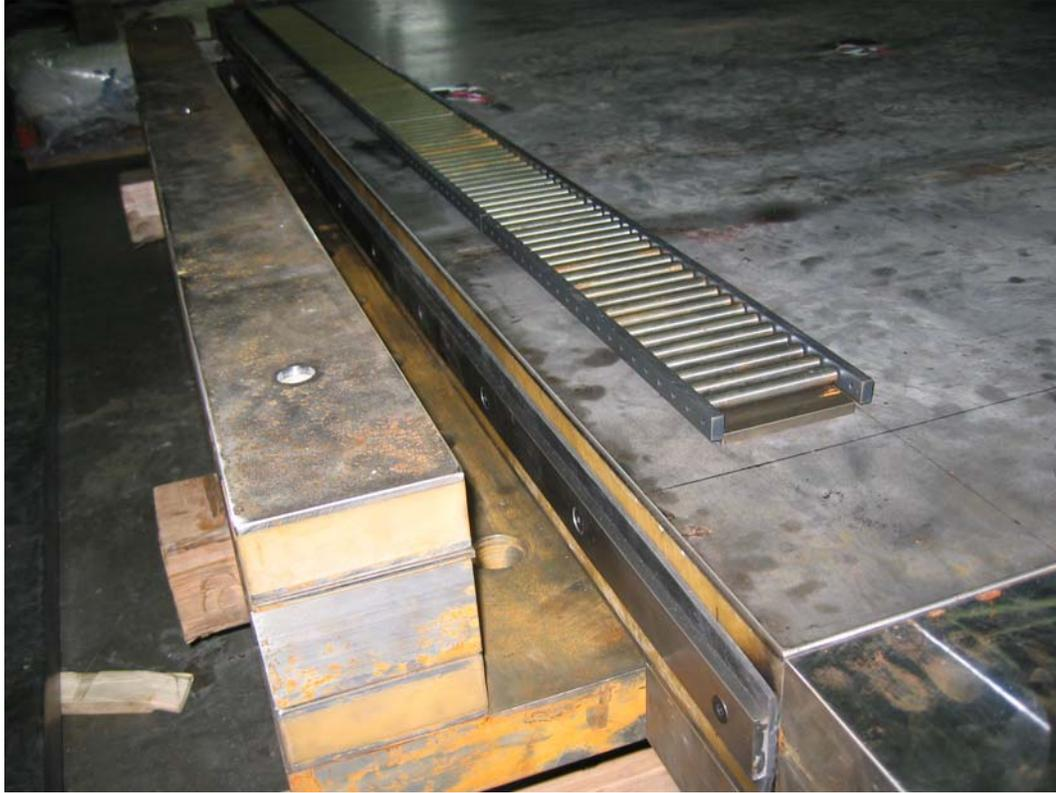
**Figure 3.20: Roller Strip – Outer Bearing Plates Removed**
