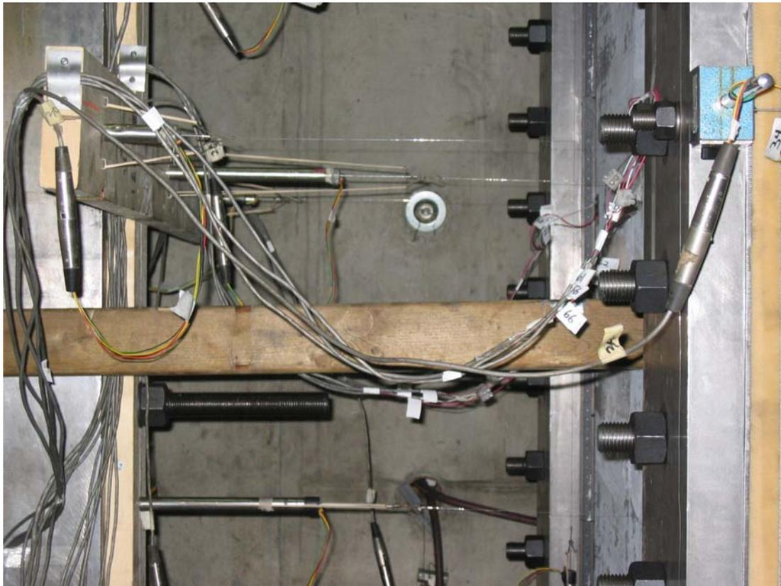
**Figure 3.36: Typical Out-of-plane LVDT Setup**
