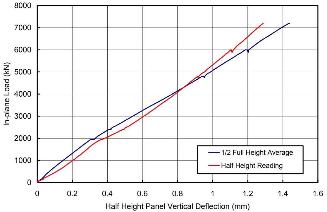
Figure 4.30: Half-height In-plane Deflection of SPS-1
