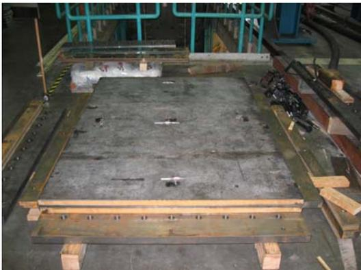
(e) SPS Specimen Set (Assembly Sequence Shown in Figure 3.19) Placed on Top and Bottom Clamp Bars and Roller Bearing Strips
