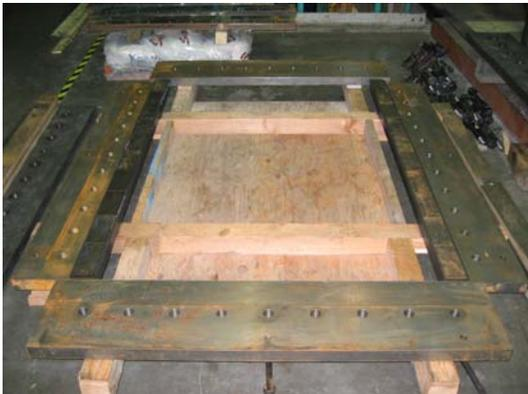
(c) Inner Bearing Plates Placed on Each Strip of Roller Bearings
