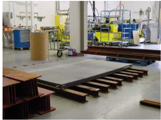
(d): Top Steel Plate Positioned on Perimeter Bar – Sand Blasted Face Down
