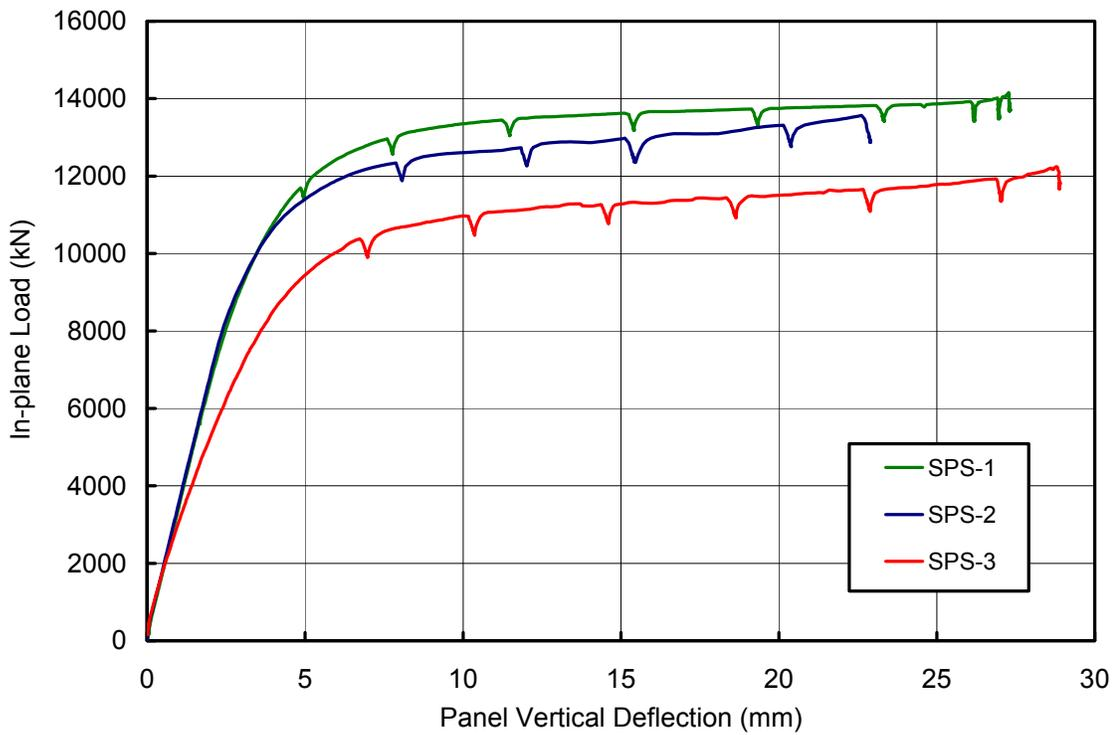
Figure 4.22: In-plane Load versus In-plane Deflection for All Three Tests
