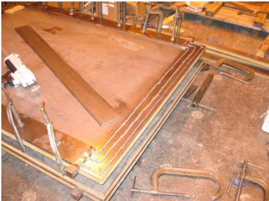
(i) Three Glue Beads for Top Spacer Bar Component
