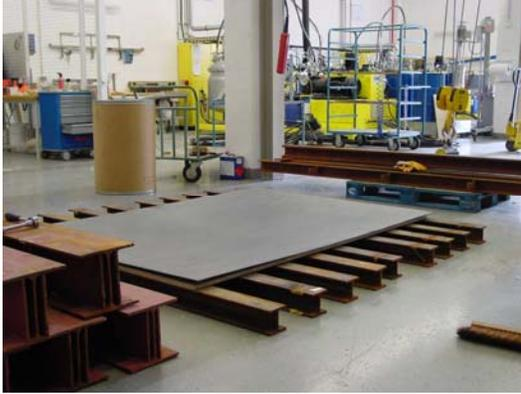
(a): Bottom Steel Plate on Out-of-plane Restraint Beams – Sand Blasted Face Up
