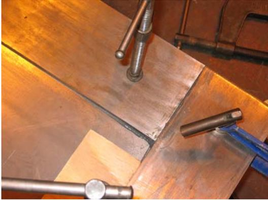
(g) Close-up of Typical Butt Joint Between Top / Bottom and Edge Spacer Bars
