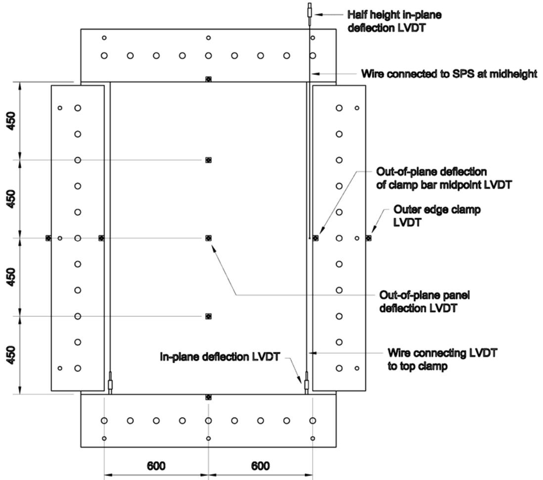
Figure 3.34: LVDT Layout on Specimen Set
