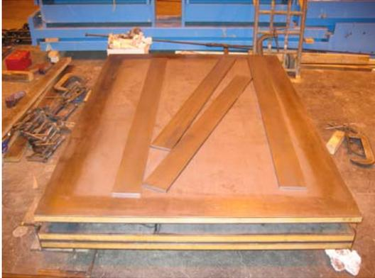
(a) First SPS Panel with Spacer Bar Components
