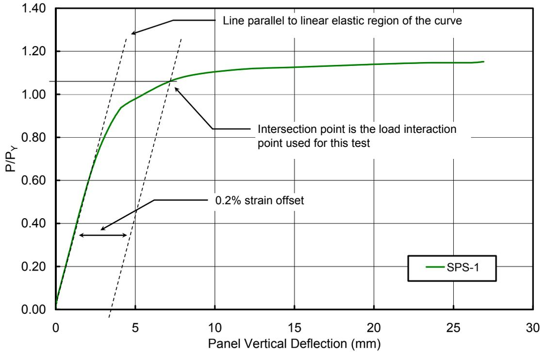
**Figure 5.9: Determination of Interaction Point using 0.2% Strain Offset Method – SPS-1**
