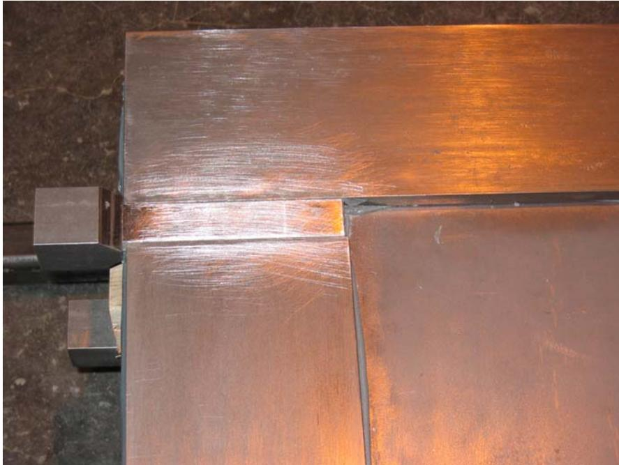
Figure 3.8: Water Inlet Spacer Insert
