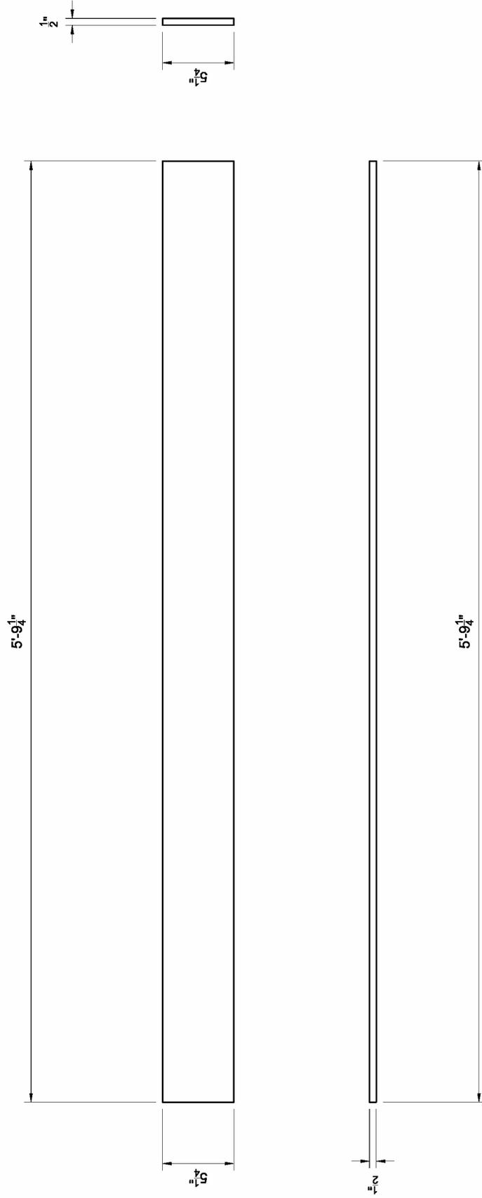
Figure A6: Edge Panel Spacer Bar (2 Pieces Required per Specimen Set) – Fabrication Drawing with Imperial Units
