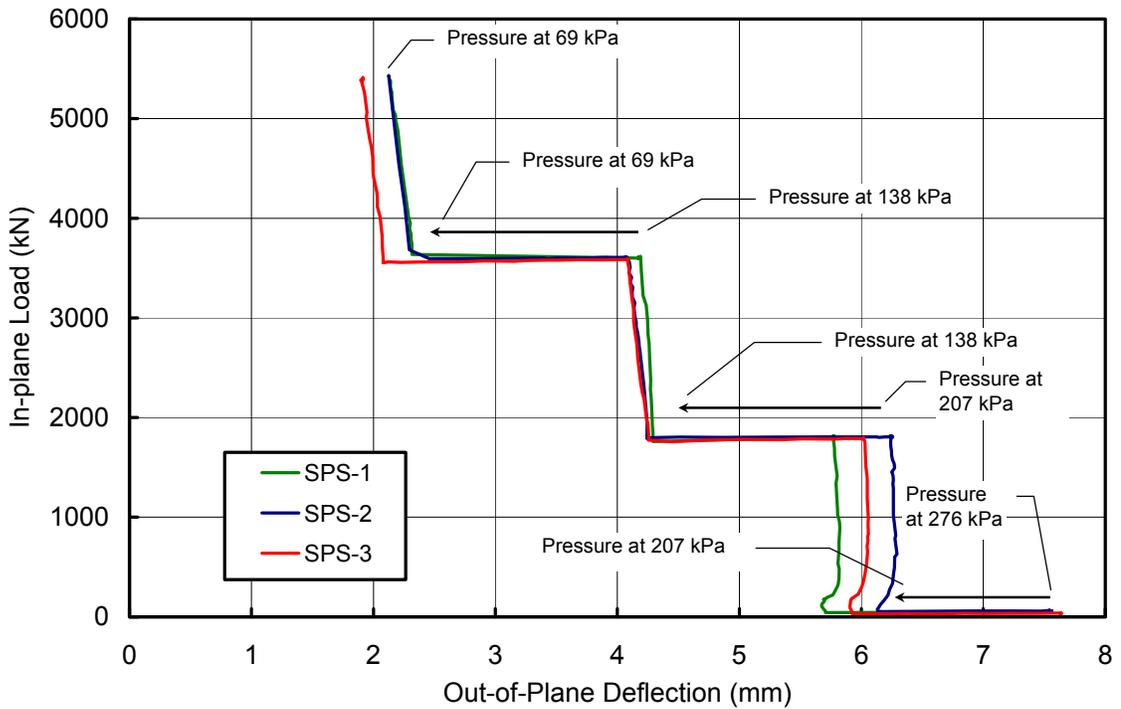
Figure 4.12: In-plane Load versus Panel Midpoint Out-of-plane Deflection
