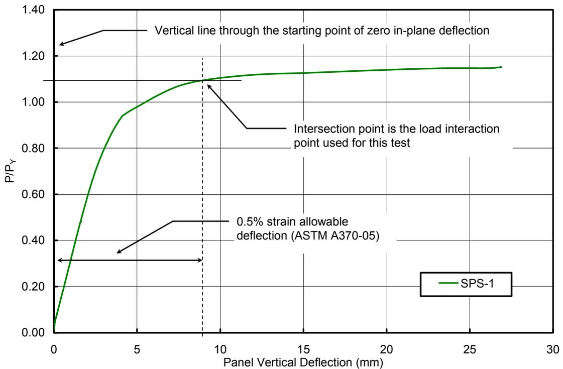
**Figure 5.10: Determination of Interaction Point using 0.5% Allowable Deflection Method – SPS-1**
