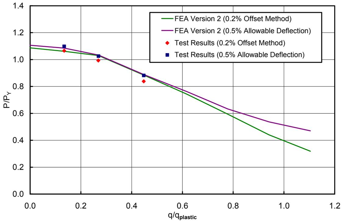
Figure 5.14: Interaction Diagram - FEA Version 2 and Test Results
