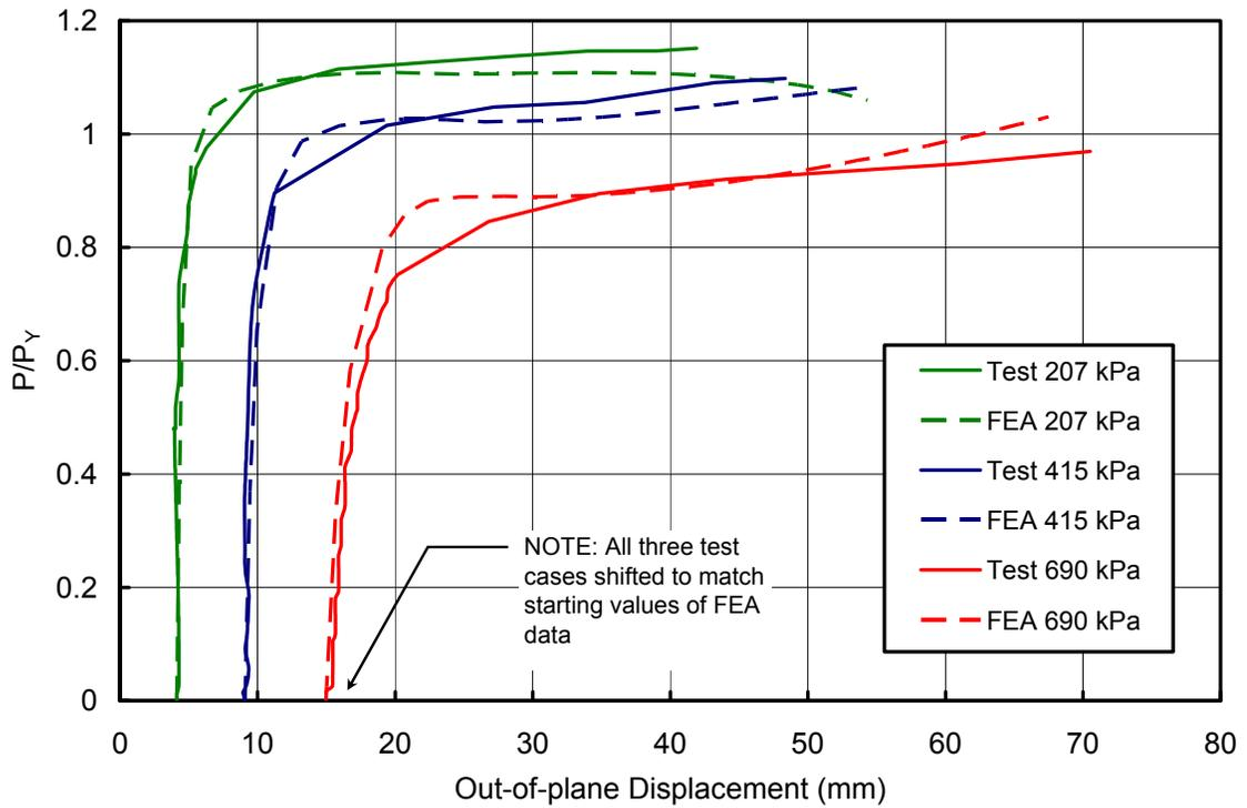
Figure 5.5: In-plane Load versus Out-of-plane Deflection at Panel Quarter Point – FEA versus Test
