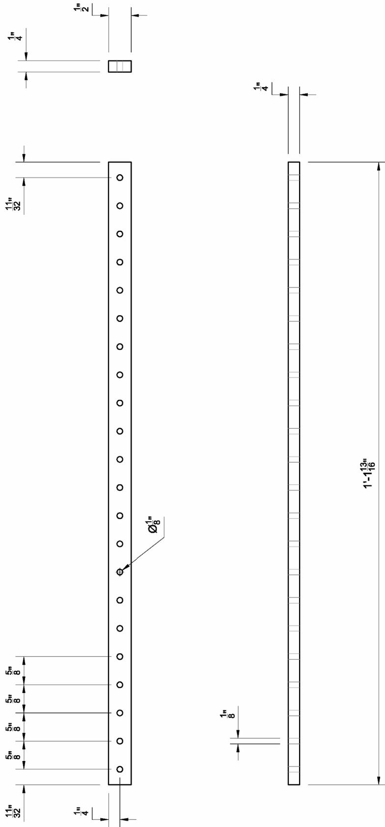
Figure A8: Nylon Retaining Strip for Roller Bearing Assemblies (40 Pieces Required) – Fabrication Drawing with Imperial Units
