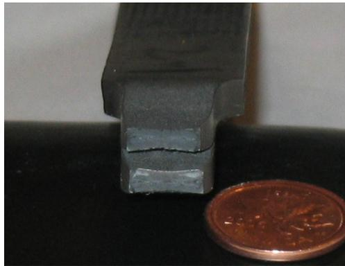
**Figure 3.41: Failed Section of Typical Tension Coupon**
