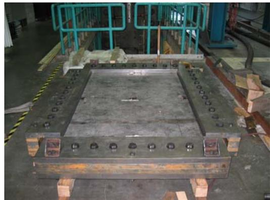
(l) Rectangular Ring of 1-1/4 in Diameter Bolts Inserted and Tightened all Around Frame
