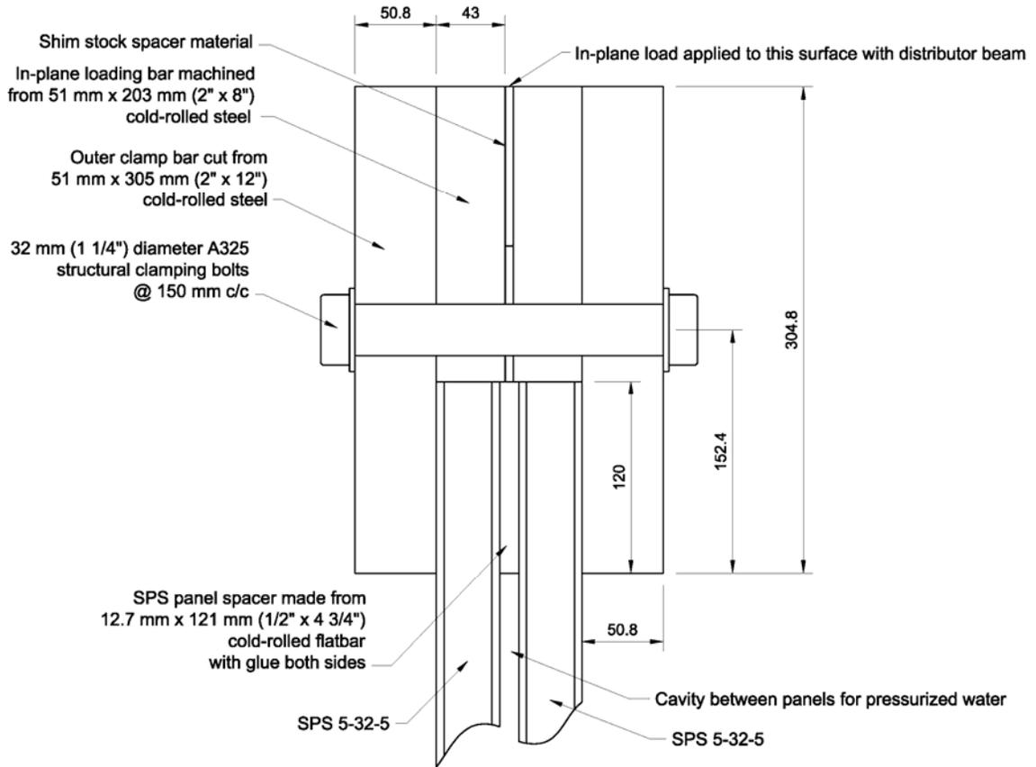
Figure 3.12: Top Clamp Section
