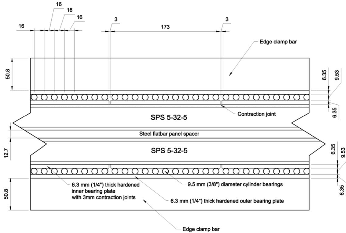
**Figure 3.18: Section of Portion of Roller Bearing Assembly**
