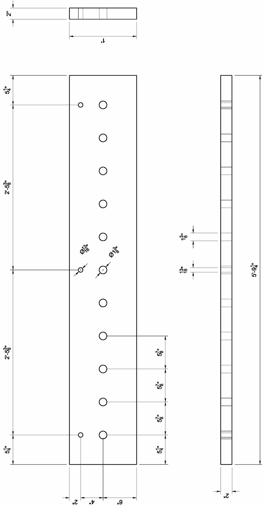
Figure A3: Edge Clamp Outer Bar (4 Pieces Required) – Fabrication Drawing with Imperial Units
