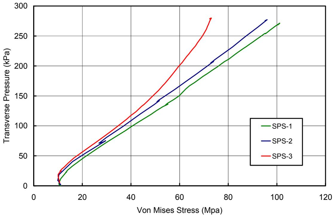
Figure 4.9: Transverse Pressure versus Average Panel Edge von Mises Stress
