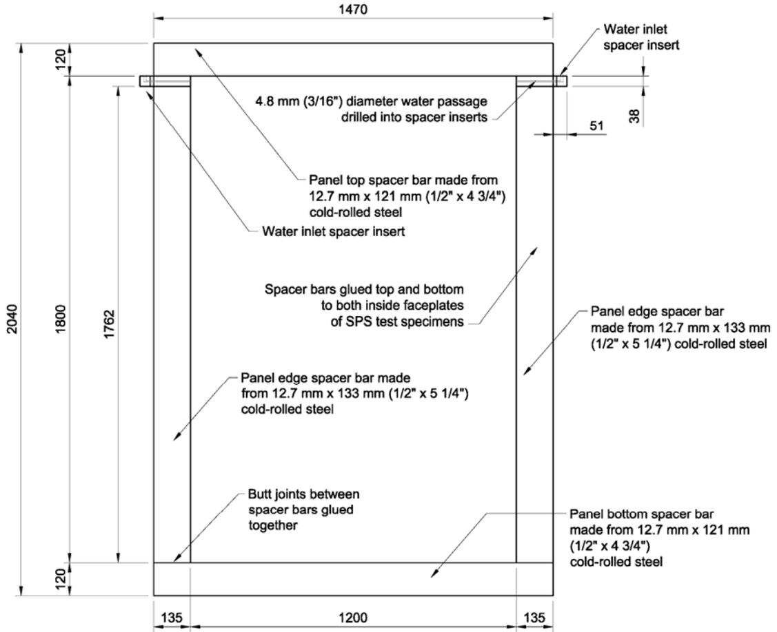
**Figure 3.6: Panel Spacer Bar Layout**
