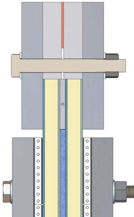
Figure 3.13: Rendered Top Clamp Section
