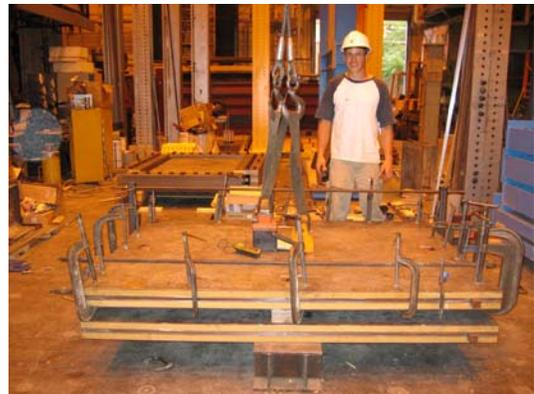
(l) Second SPS Panel Lowered into Position with Crane and Clamped Until Cure
