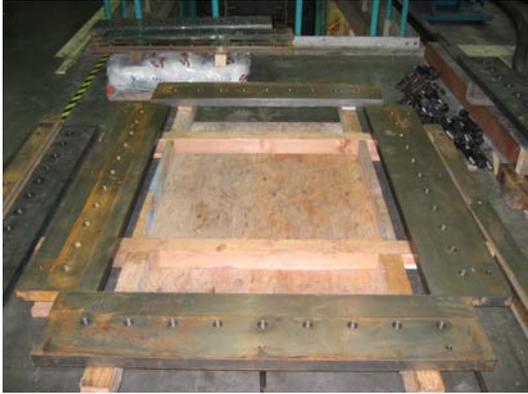
(a) Four Outer Clamp Bars Placed on Wood Assembly Platform
