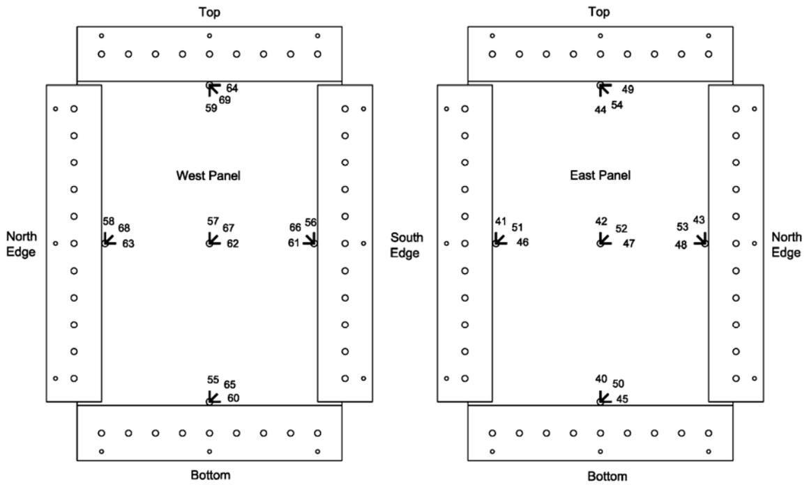
Figure 3.32: Channel Numbers Corresponding to Strain Rosette Components
