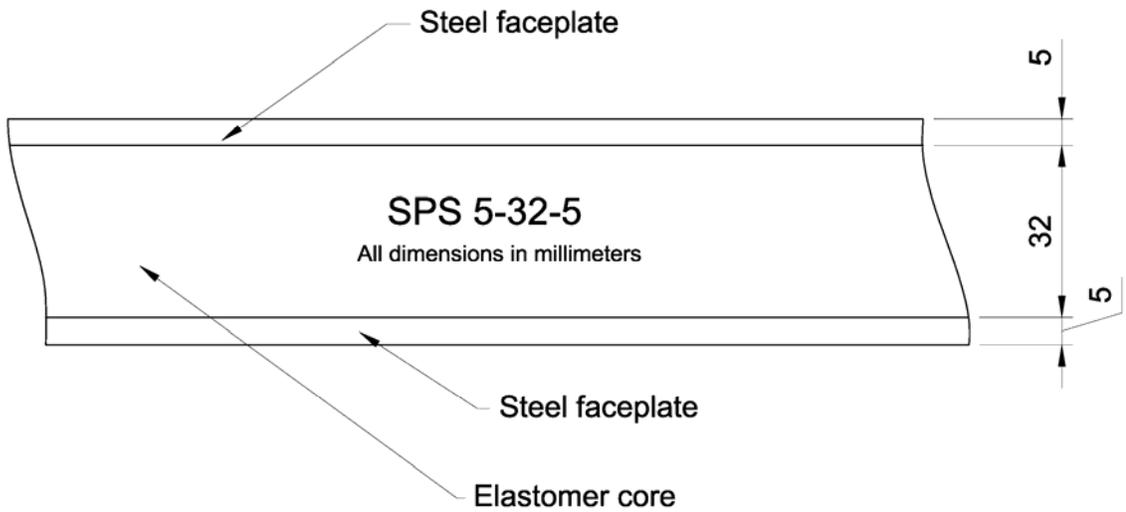
Figure 3.2: SPS Specimen Section
