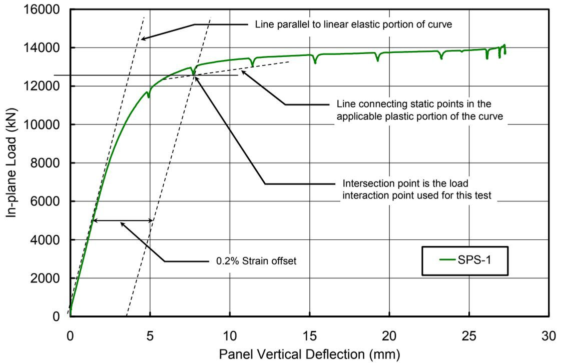
Figure 4.26: Interaction Point from In-plane Load versus In-plane Deflection Curve for SPS-1 Test
