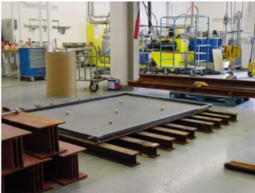
(c): Elastomer Spacer Blocks Placed at Intervals on Plate Mid Region
