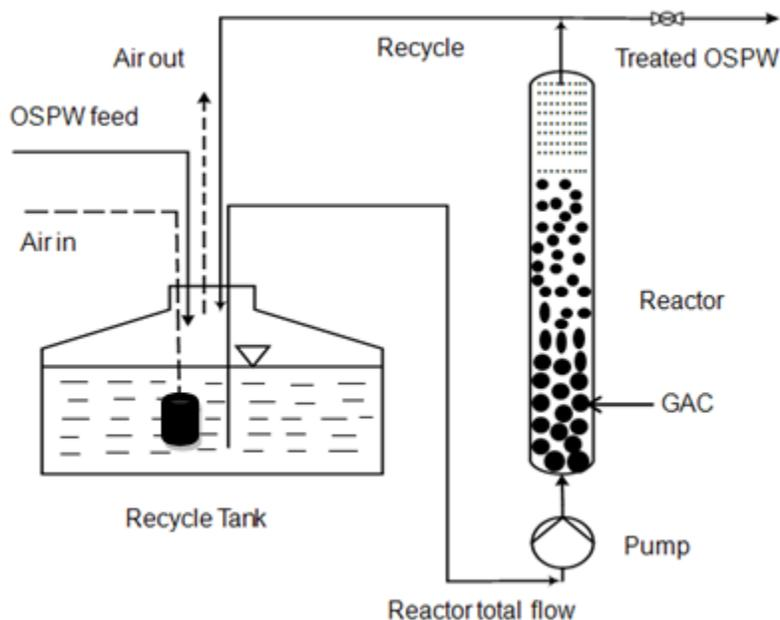
**Figure 3.1.** Schematic diagram of the experimental set-up.
