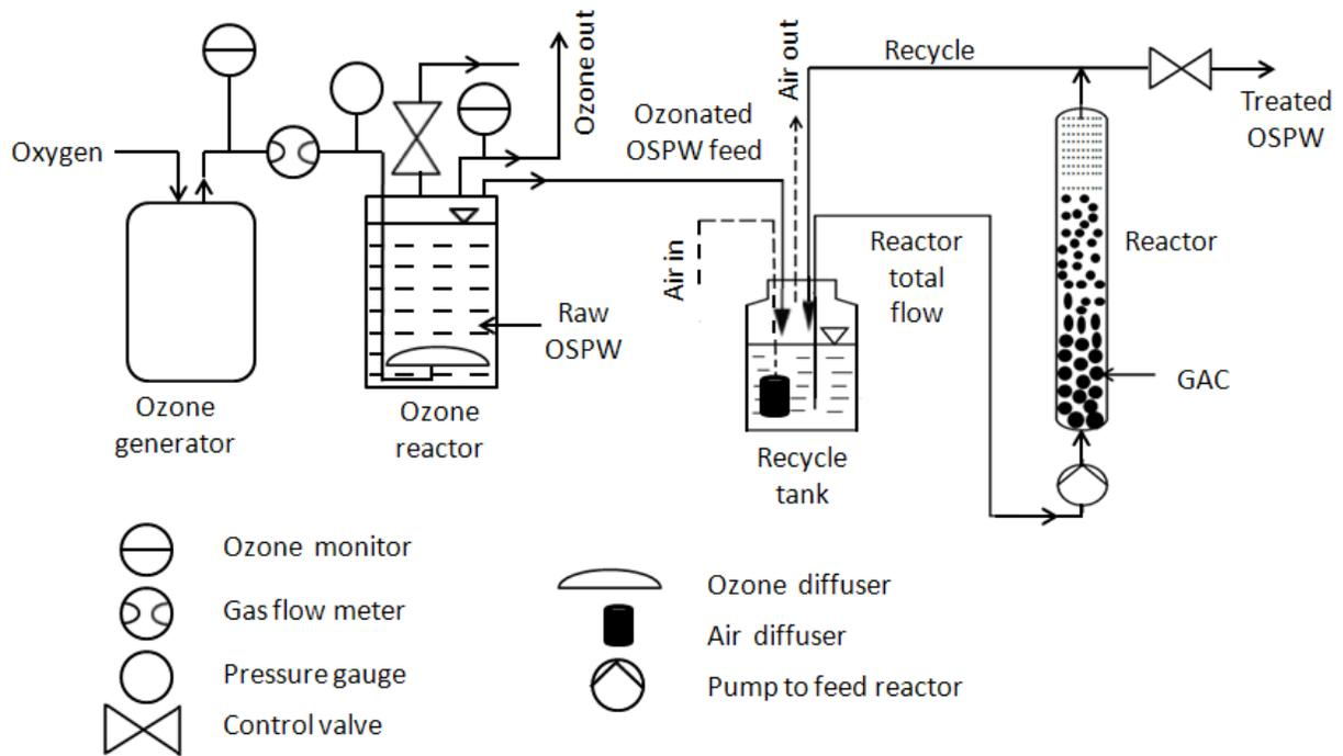
**Figure 4.1.** Schematic of combined ozonation and GAC-FBBR system.
