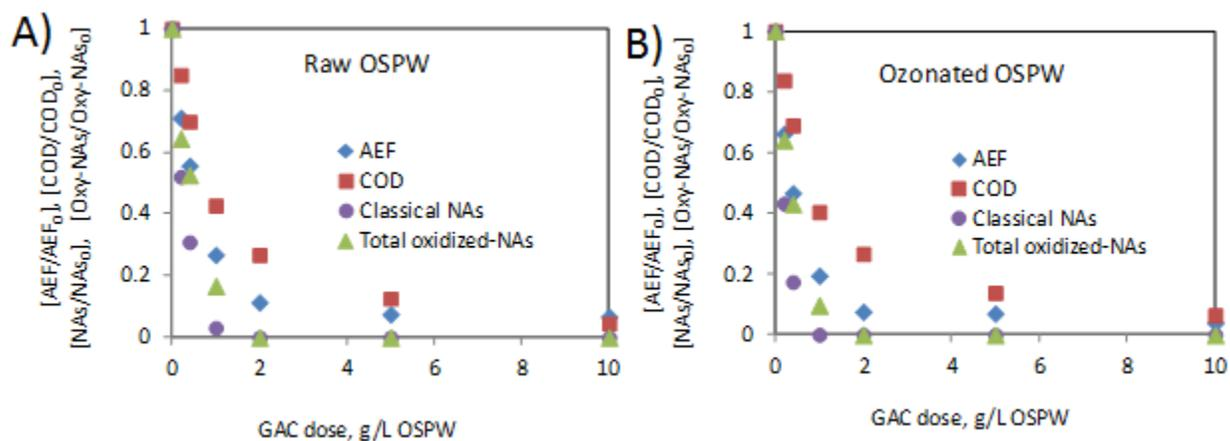
**Figure D1.** Relative removal of AEF, COD, classical-NAs and oxidized-NAs from both raw and ozonated OSPW after preliminary GAC treatment (Raw OSPW:  $AEF_0 = 67.48$  mg/L,  $COD_0 = 214$  mg/L,  $Classical\ NAs_0 = 17.43$  mg/L,  $Total\ oxy\ NAs_0 = 27.58$  mg/L; Ozonated OSPW:  $AEF_0 = 53.05$  mg/L,  $COD_0 = 222$  mg/L,  $Classical\ NAs_0 = 12.59$  mg/L,  $Total\ oxy-NAs_0 = 27.26$  mg/L).
