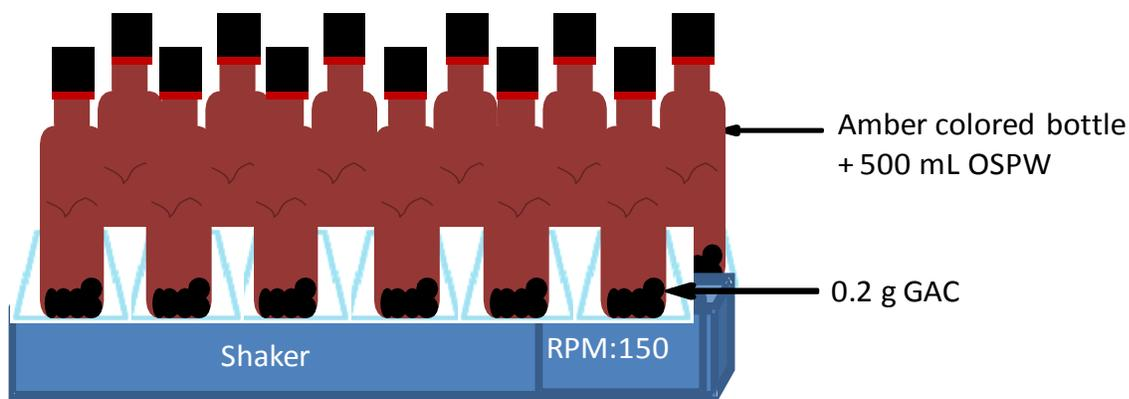
**Figure 5.1.** Experimental set up for carrying out GAC adsorption, biodegradation and combined treatment mechanisms.
