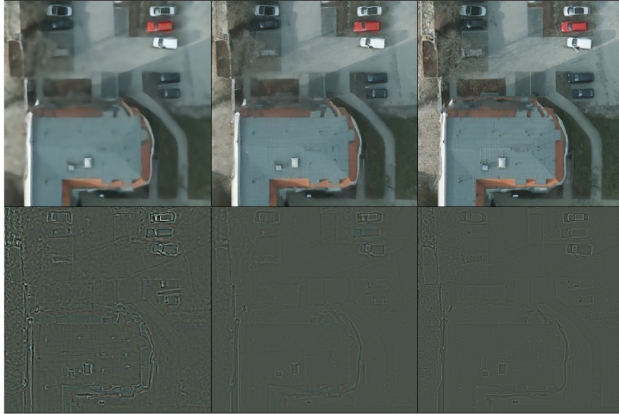
(a) Final SR image and enhanced edge with L_{img\_cst} loss (b) Final SR image and enhanced edge with L_{img\_cst} and L_{edge\_cst} losses (c) Ground truth HR image with extracted edge
