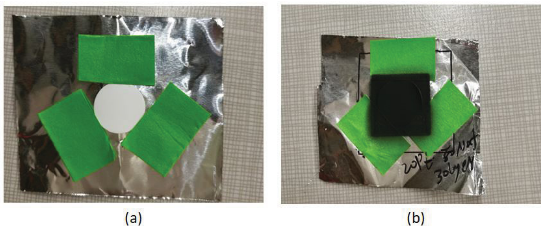
Figure 3.4: Pictures of: (a) PTFE filter fixed on aluminum foil, (b) Catalyst printed on PTFE filter
