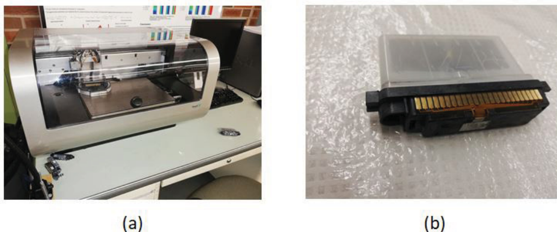
Figure 3.3: Images of: (a) Dimatix 2831 inkjet printer, (b) Printer cartridge
