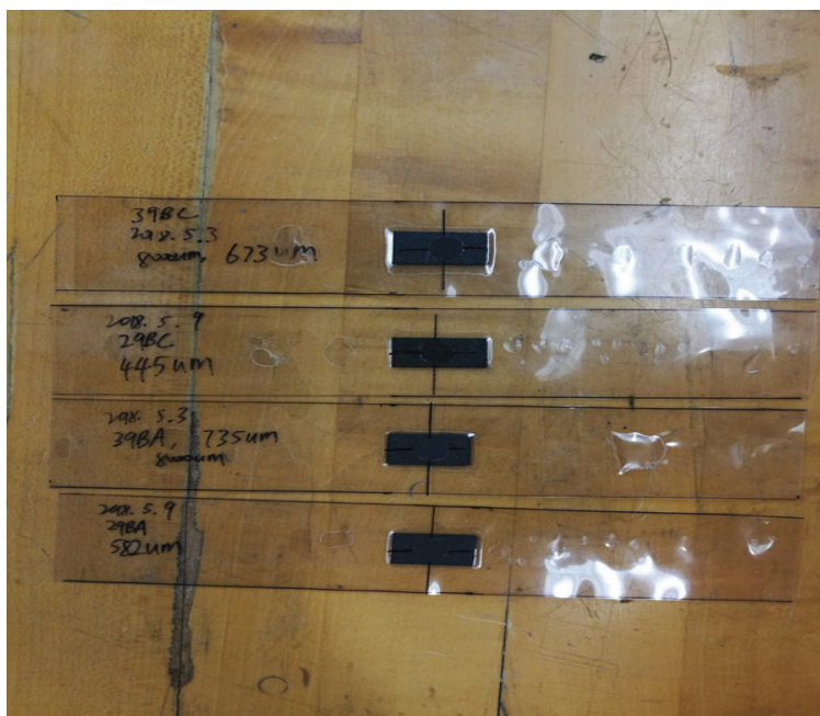
Figure 3.2: Prepared GDL samples
