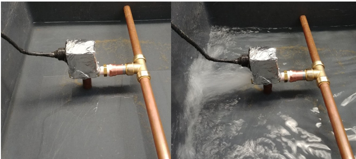
Figure 4.18: Large leak source (electrically-actuated valve)
