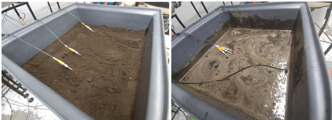
Figure 4.14: Dry black loam and at saturation point
