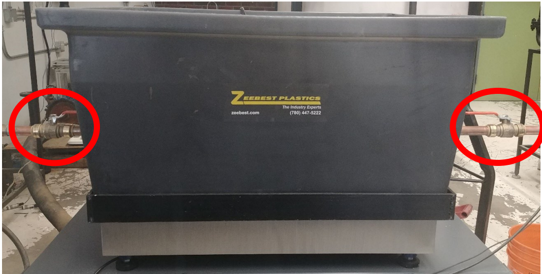
Figure 4.16: On-off valves to create an abrupt alteration of the flow
