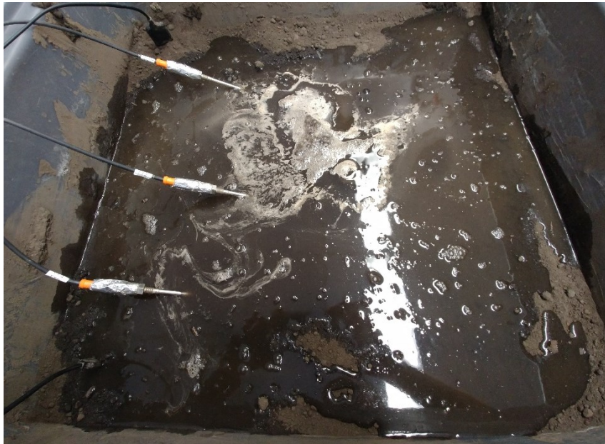
Figure 5.50: Water-soil flow at minute 20 of starting leak (2:55 pm) (Test9 – Round 2)
