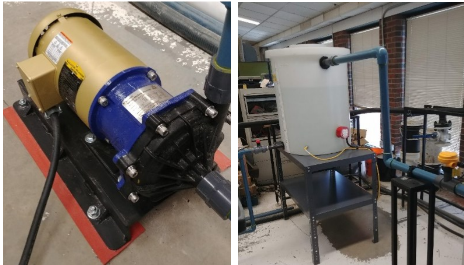
Figure 4.12: Centrifugal pump and reservoir
