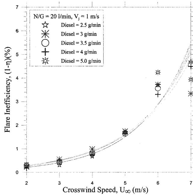
**Figure 4.16: Effects of mass flow rates of diesel on the inefficiency of the flares with low jet exit velocity in crosswinds**
