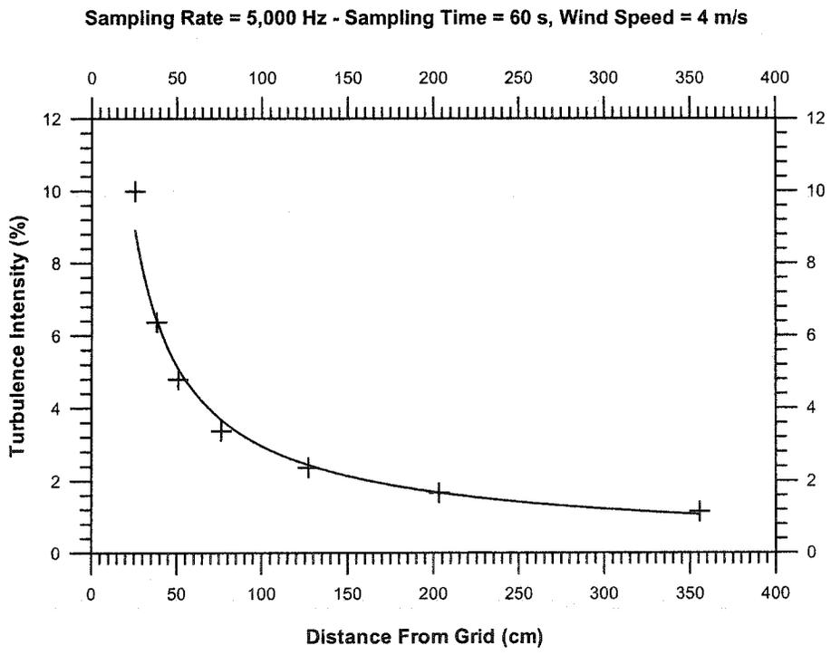
**Figure 3.10: Turbulence intensity decay behind the grid with 25.4 mm square holes**
