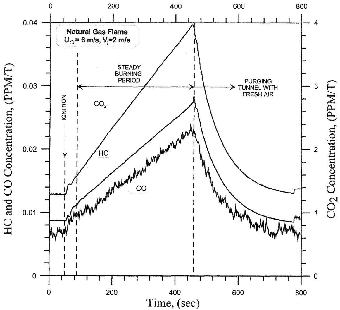
**Figure B.3: Ratio of concentrations of major carbon containing species divided by temperature during an experiment in tunnel**
