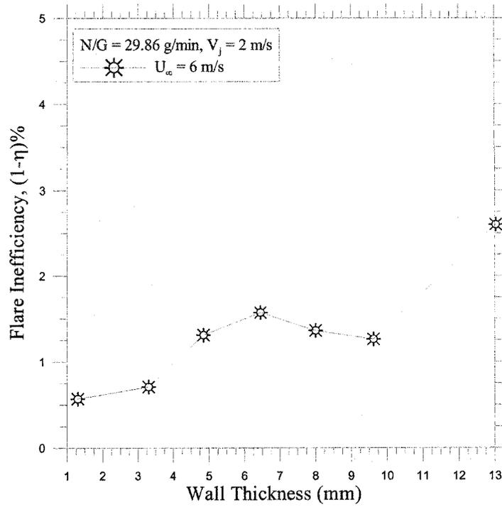
**Figure 5.15: Effects of varying wall thickness on the inefficiency of high jet exit velocity flare at 6 m/s**
