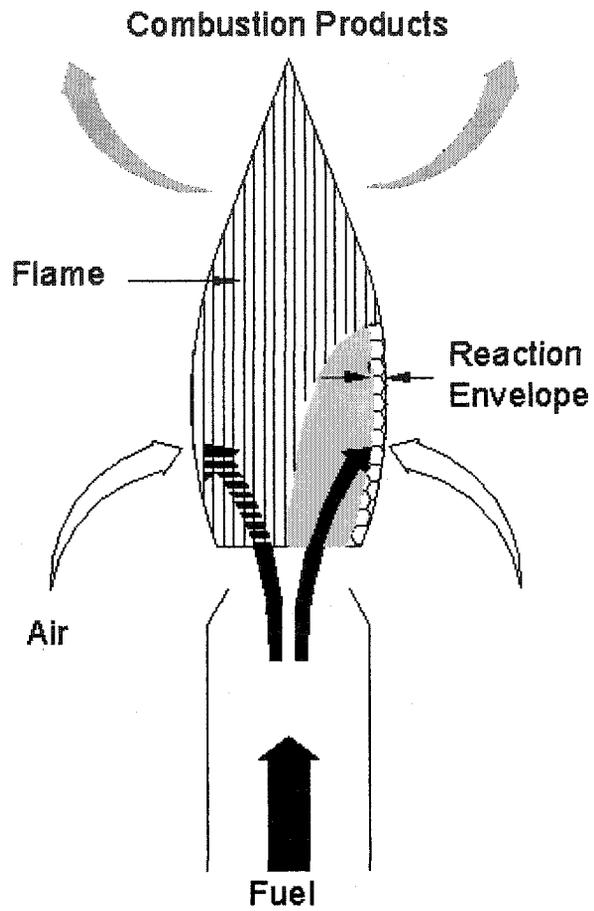
Figure 2.3: Combustion of gaseous fuel in diffusion flame (Edwards, 1974)
