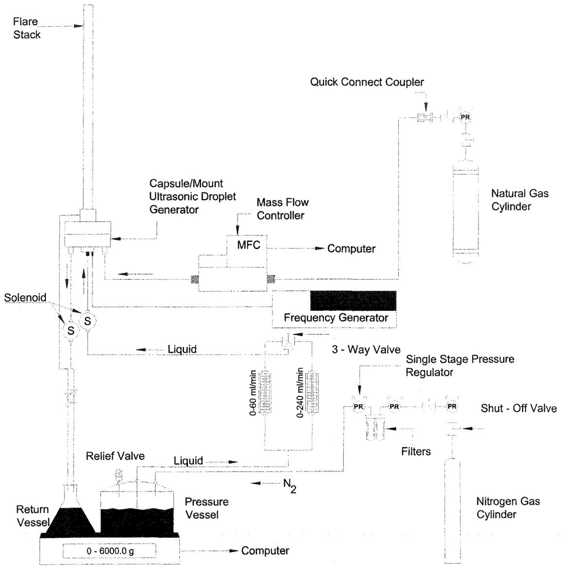
**Figure 3.5: Liquid supply system and mass flow rate of the liquid exiting the flare stack (Kosiuk, 2000)**
