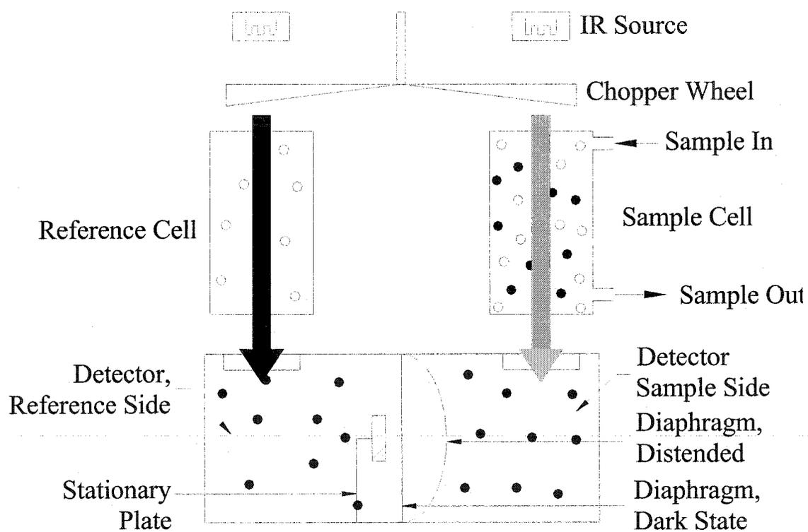
**Figure A.6: Non-dispersive Infrared Analyzer**
