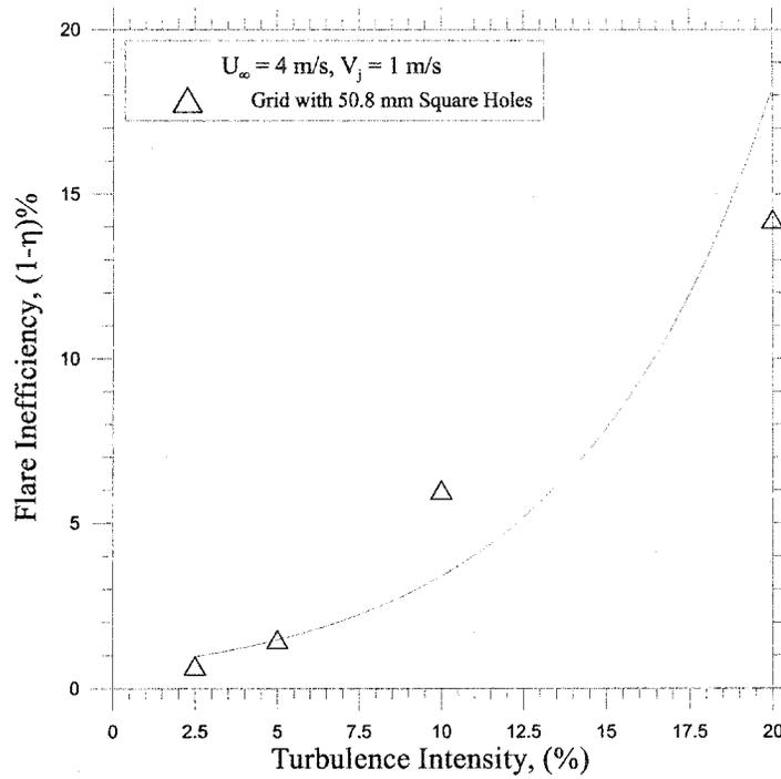
**Figure 5.1: Inefficiency of the flares having low flare gas flow rate subjected to varying turbulence intensities generated by the grid with 50.8 mm square holes**
