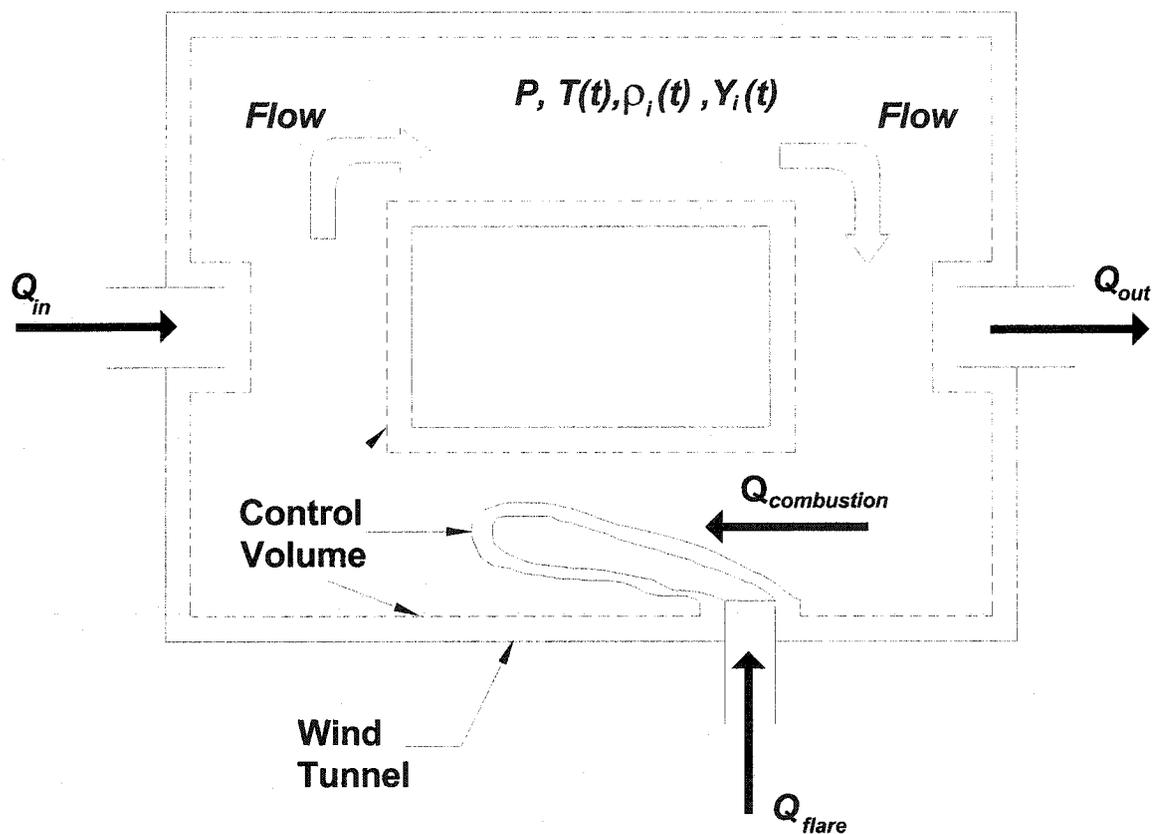
Figure B.1: A model for wind tunnel as constant pressure enclosure (Johnson *et.al.*, 2001)
