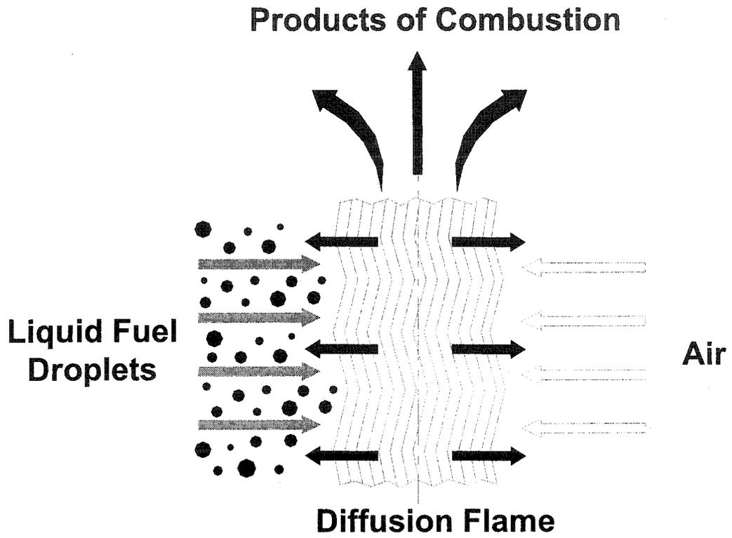
**Figure 2.5: Combustion of liquid fuel droplet**
