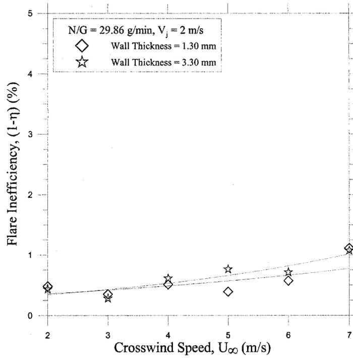
**Figure 5.11: Effects of increased wall thickness on the inefficiency of the flares having high flare gas flow rates and jet exit velocity in crosswind**
