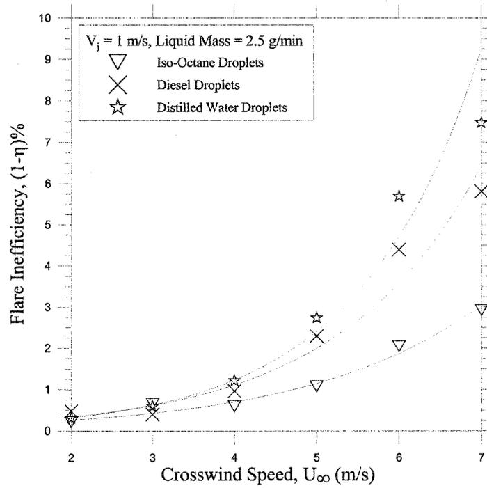
**Figure 4.24: Effects of iso-octane, diesel, and distilled water droplets on the inefficiency of the flares of low jet exit velocities in crosswinds**
