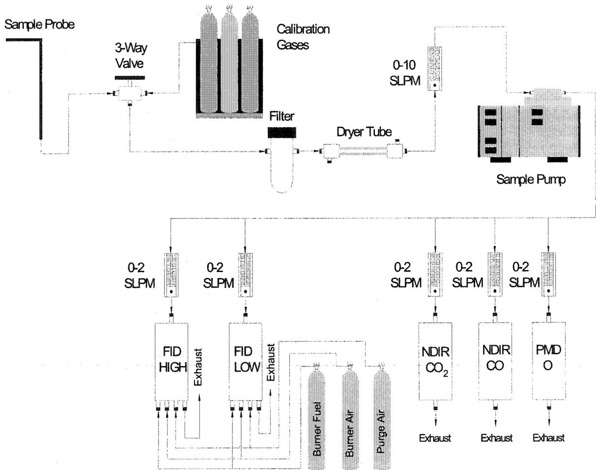
**Figure A.4: Schematic of gas sampling system**
