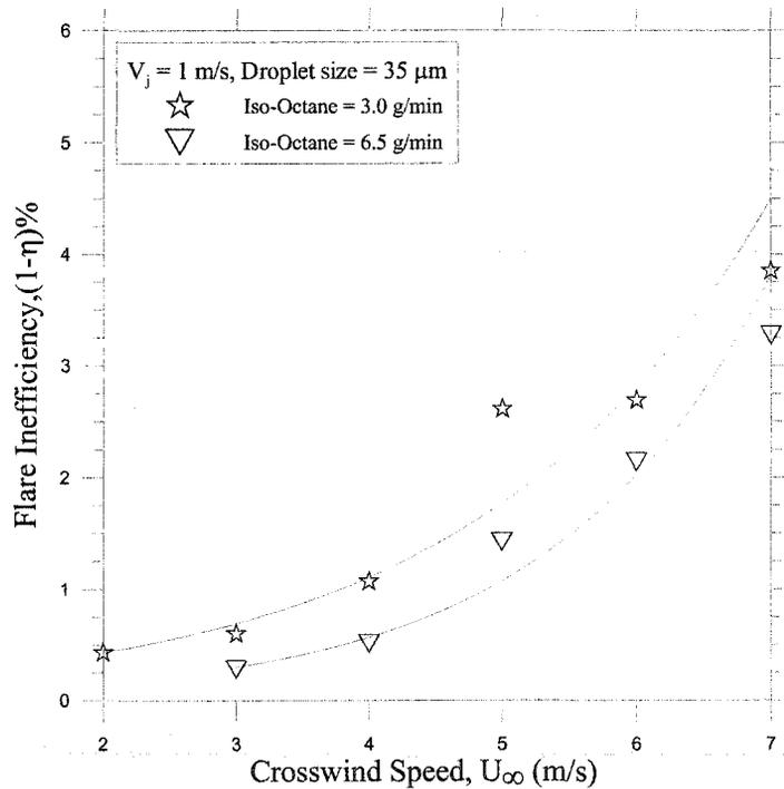
**Figure 4.9: Effects of the mass flow rate of iso-octane on the flare inefficiency having same size of the droplets in the flare stream**
