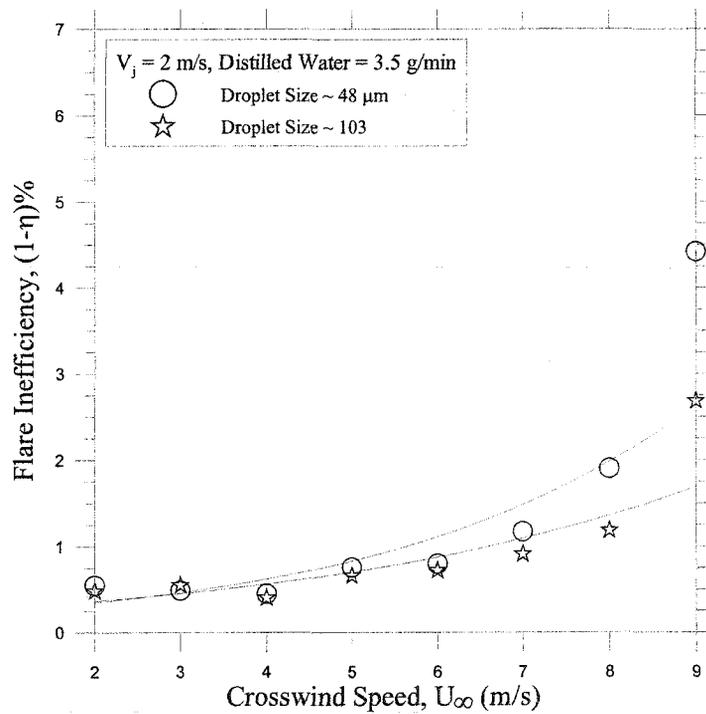
**Figure 4.21: Inefficiency analysis of the flares with higher jet exit velocity having two different sizes of water droplets in the flare stream**
