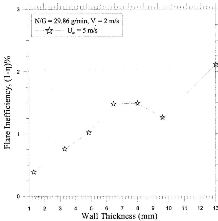
**Figure 5.14: Effects of varying wall thickness on the inefficiency of high jet exit velocity flare at 5 m/s**
