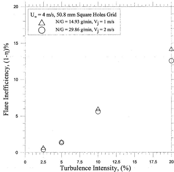
**Figure 5.4: Comparison of the inefficiencies of the flares with high and low flow rates of the flare gas under the same turbulent crosswind conditions**
