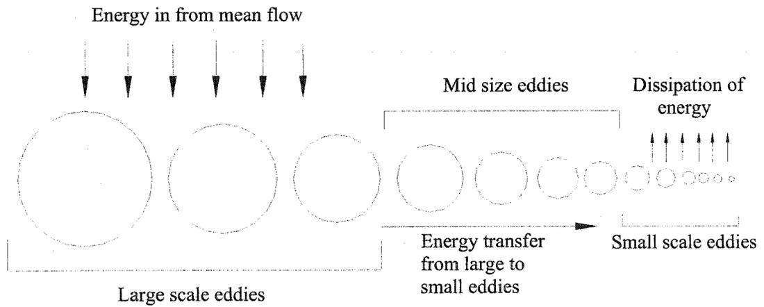
**Figure 5.2: Eddies generated in turbulent flow**
