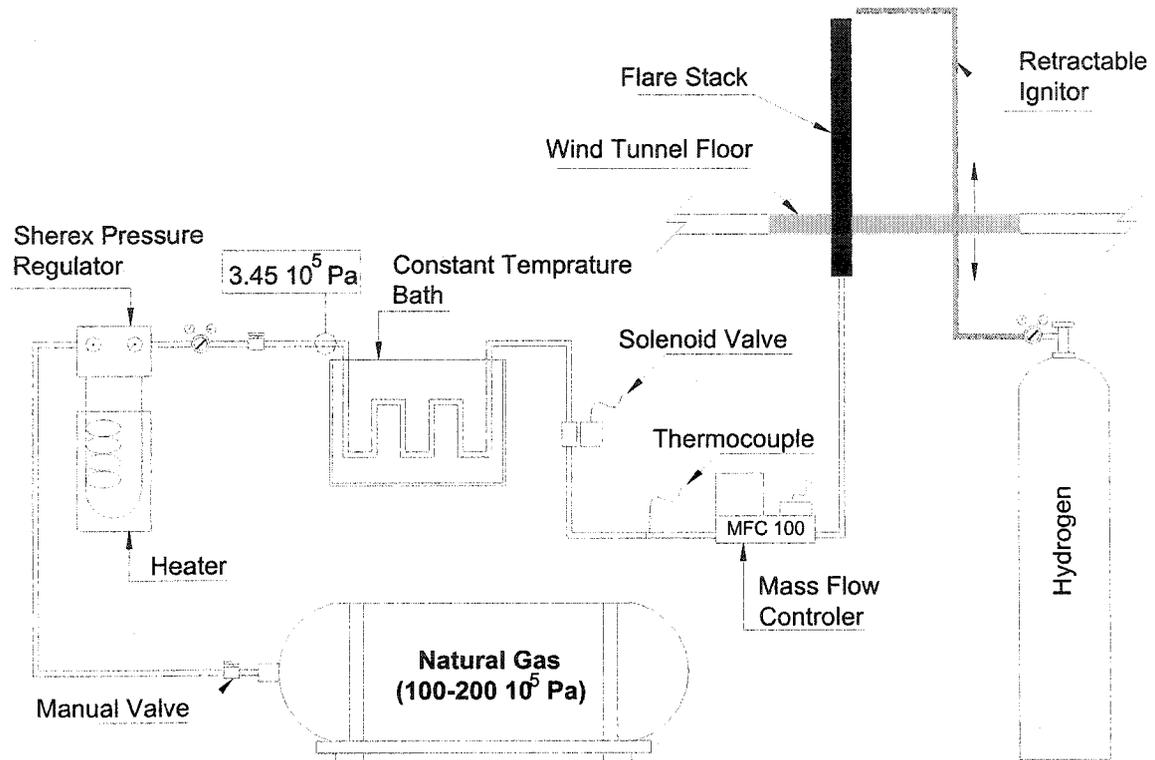
**Figure A.3: Schematic of natural gas supply system**
