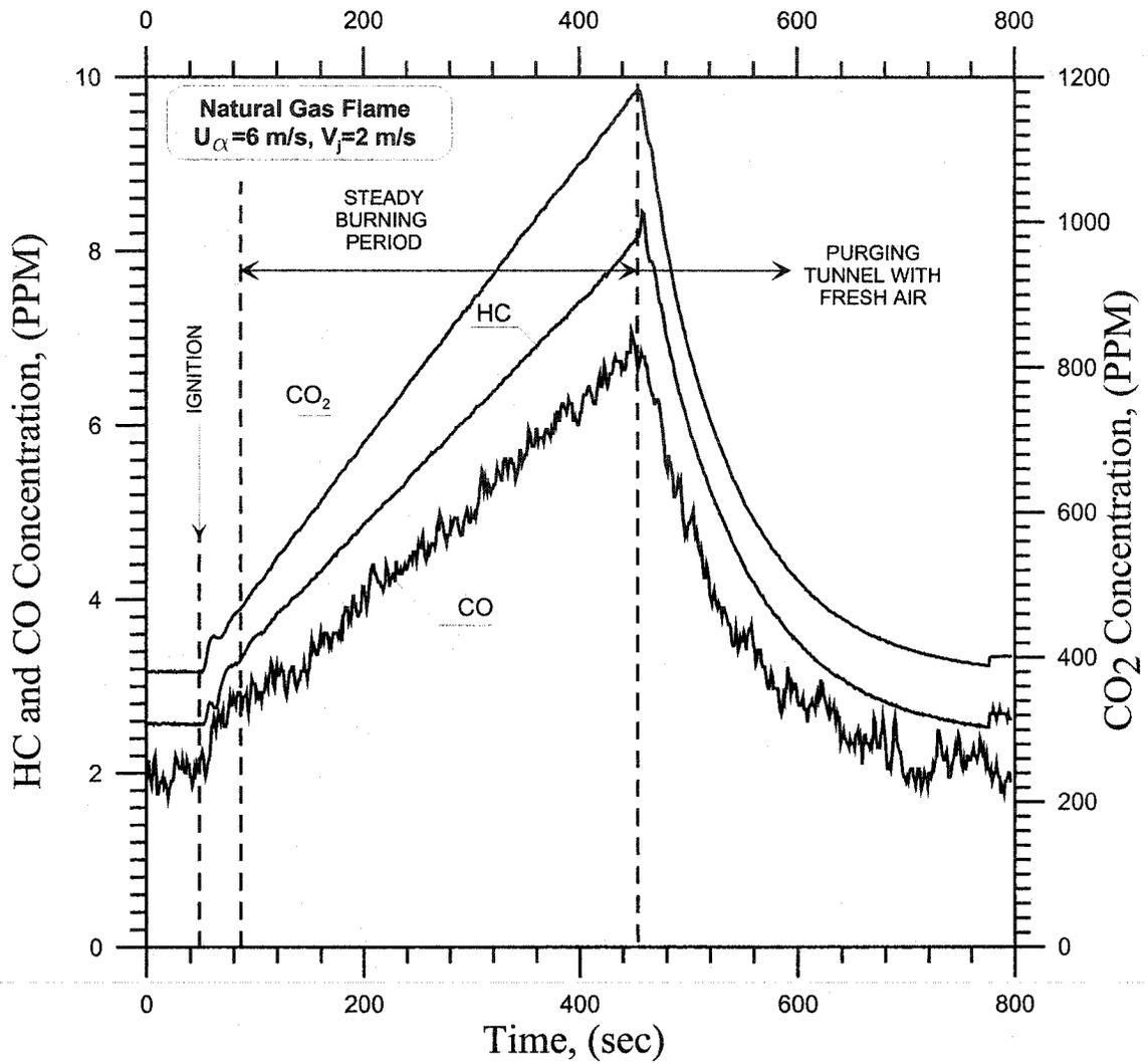
**Figure B.2: Time trace of concentrations of CO<sub>2</sub>, HC and CO during an experiment in the closed-loop wind tunnel**
