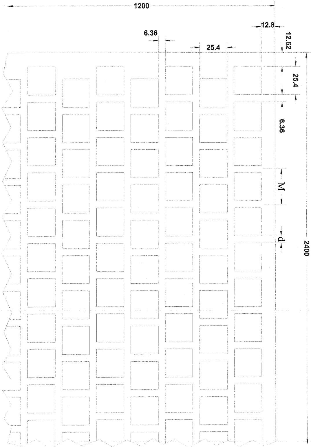
**Figure 3.7: 4 x 8 m and 1.6 mm thick grid with 25.4 mm square holes
