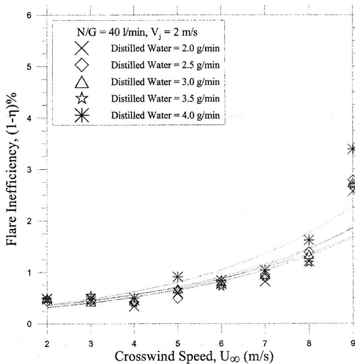
**Figure 4.23: Inefficiency of the flares having high jet exit velocity with varying flow rates of distilled water using 48 kHz droplets generator**
