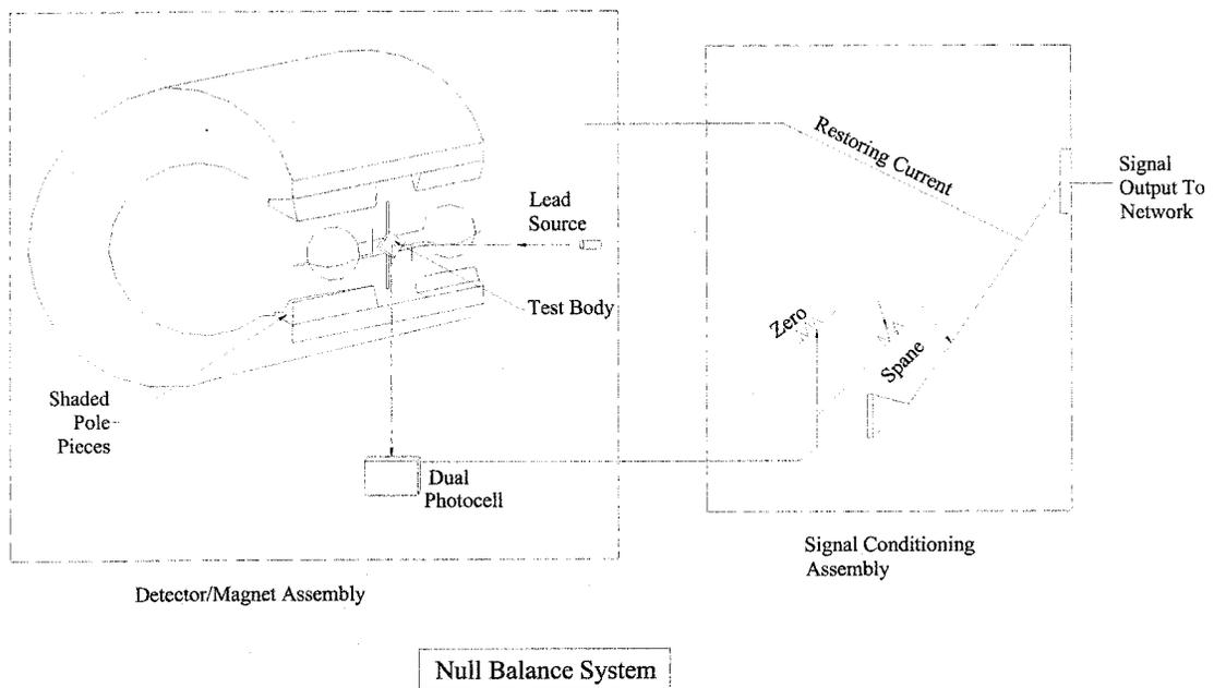
**Figure A.7: Paramagnetic Detector Technology**
