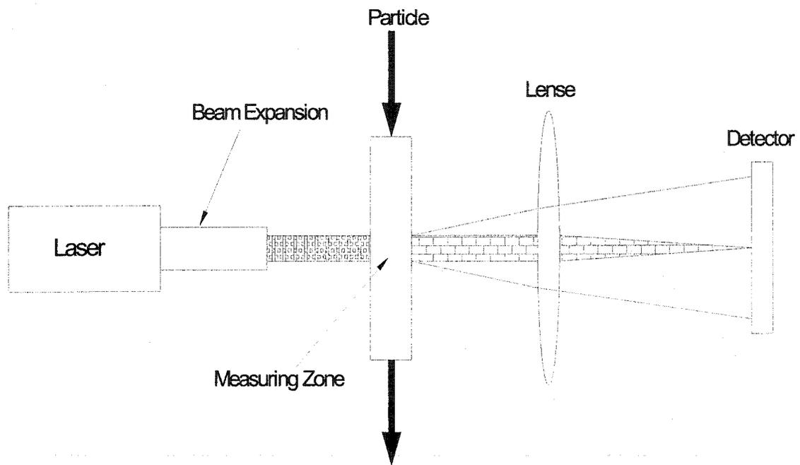
**Figure D.1: Optical setup for the measurement of diffraction patterns (Puckhaber and Röthele, 1999)**
