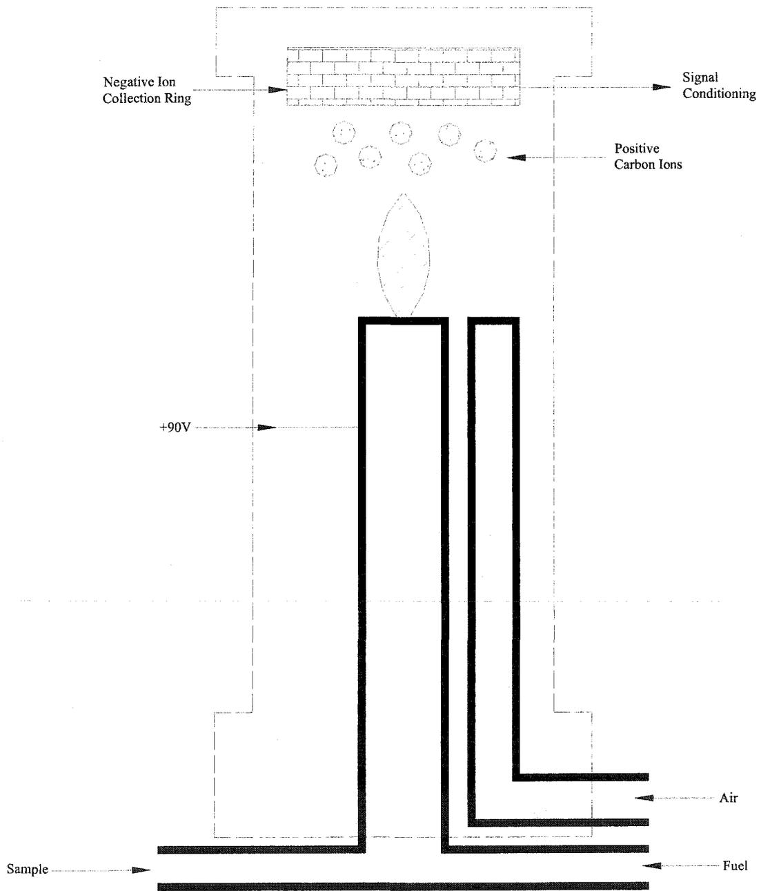
**Figure A.5: The Flame Ionization Technology**
