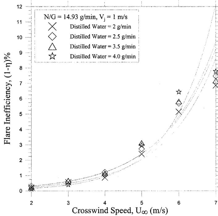
**Figure 4.22: Inefficiency of the flares having low jet exit velocity with varying flow rates of distilled water using 18 kHz droplet generator**
