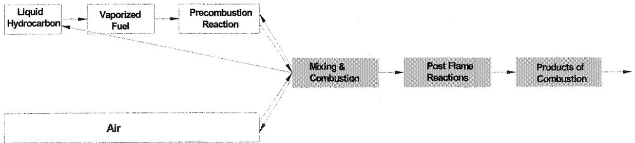
Figure 2.4: Combustion of liquid fuel in diffusion flame
