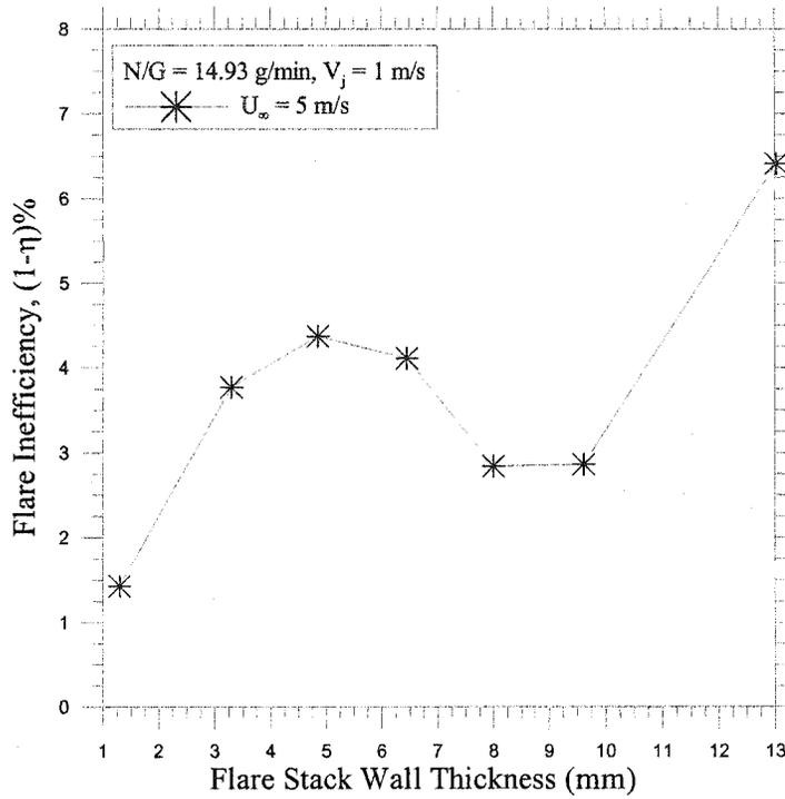
**Figure 5.13: Effects of varying wall thickness on the inefficiency of low jet exit velocity flare at 5 m/s**
