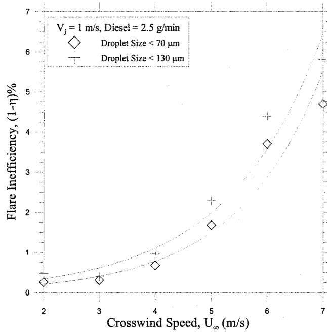
**Figure 4.14: Effects of the diesel droplet size on the inefficiency of the flares with low flare gas exit velocity**
