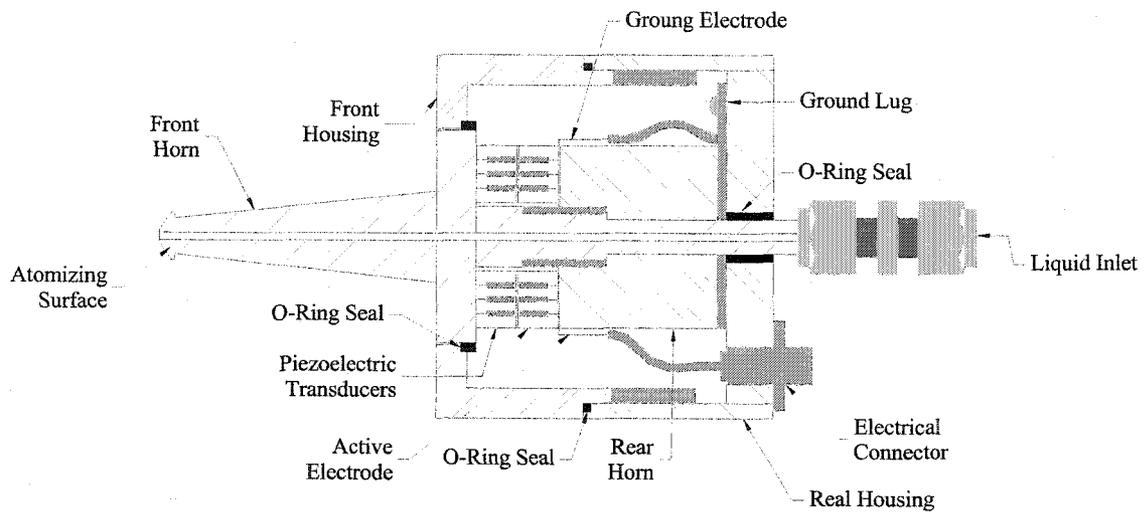
**Figure C: Ultrasonic atomizing droplets generator**
