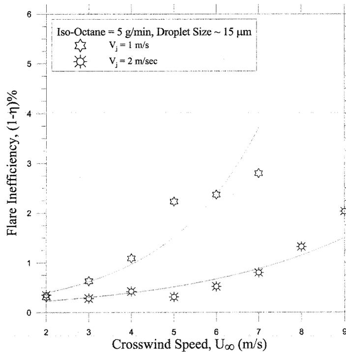
**Figure 4.5: Inefficiency analysis of the flares with different flow rates of flare gas and same droplets size and flow rates of iso-octane**
