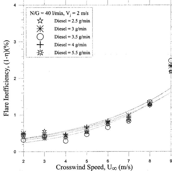
**Figure 4.17: Effects of higher jet exit velocity and mass flow rates of diesel on the inefficiency of the flares in crosswinds**
