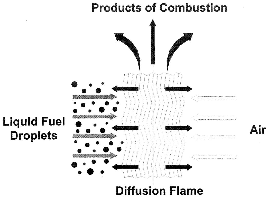
**Figure 2.5: Combustion of liquid fuel droplet**
