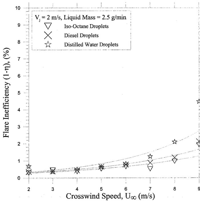
**Figure 4.25: Effects of iso-octane, diesel, and distilled water droplets on the inefficiency of the flares of high jet exit velocities in crosswinds**
