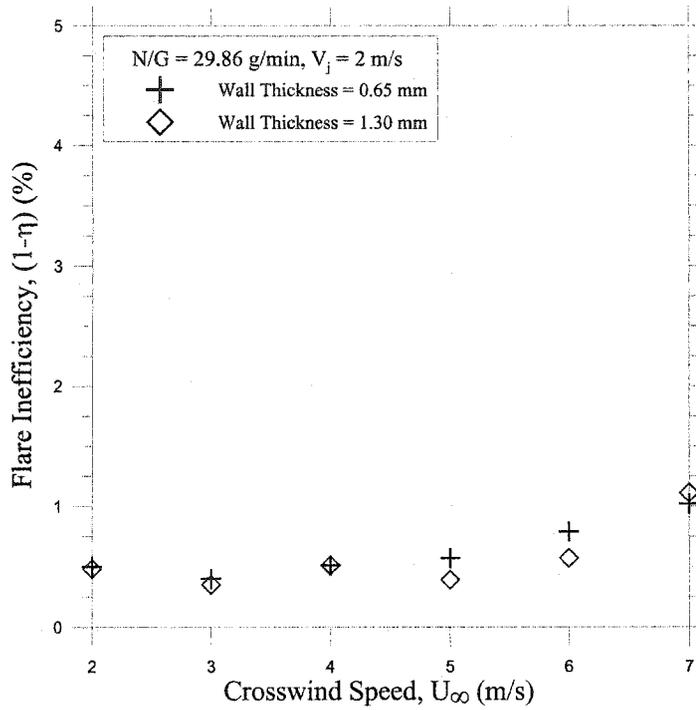
**Figure 5.9: Effects of decreased wall thickness on the inefficiency of the flares having high flare gas flow rates and jet exit velocity in crosswind**
