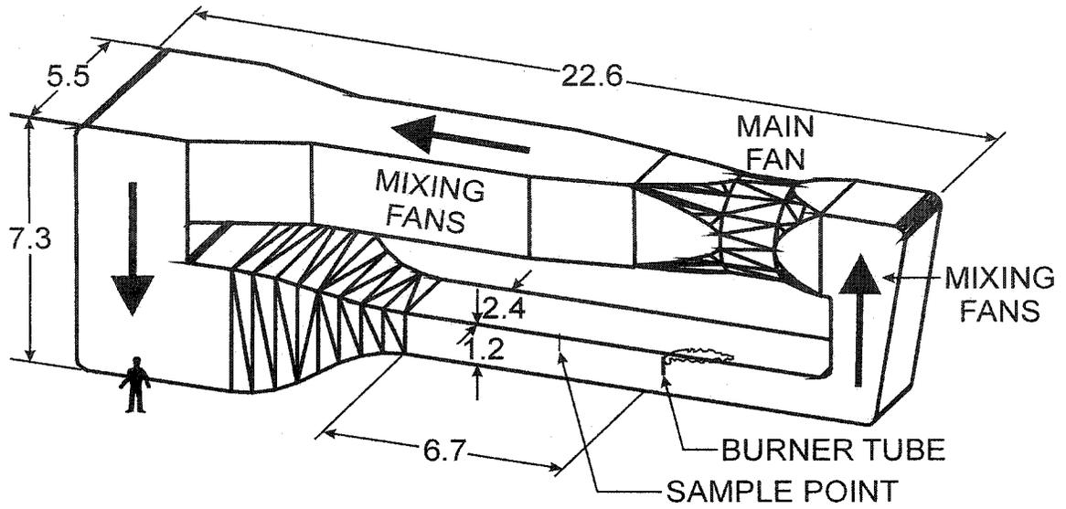
**Figure A.1: Schematic of a closed-loop combustion wind tunnel
