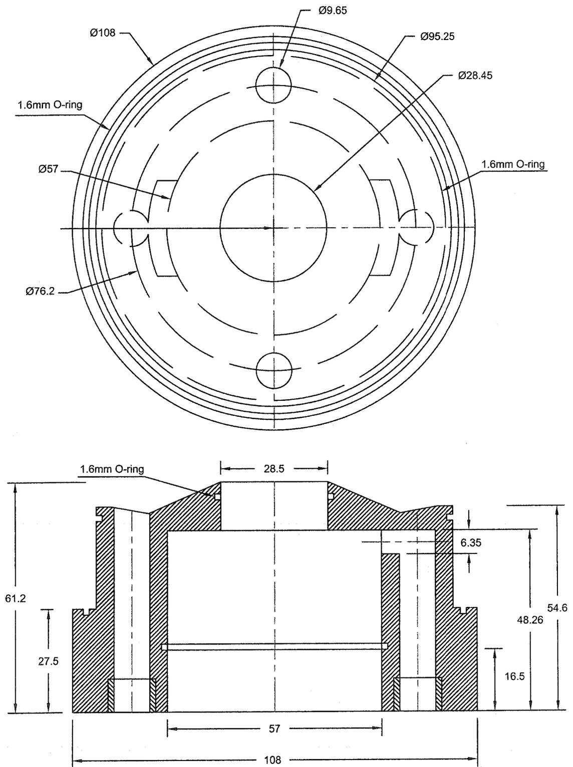
**Figure 3.2: Capsule for 48 kHz ultrasonic droplets generator
