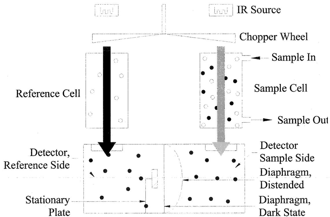
**Figure A.6: Non-dispersive Infrared Analyzer**
