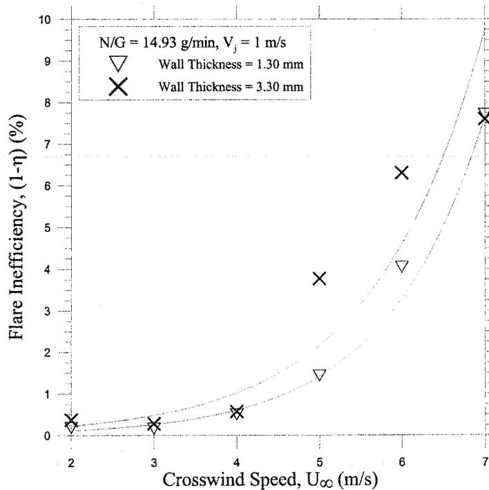
**Figure 5.10: Effects of increased wall thickness on the inefficiency of the flares having low flare gas flow rates and jet exit velocity in crosswind**
