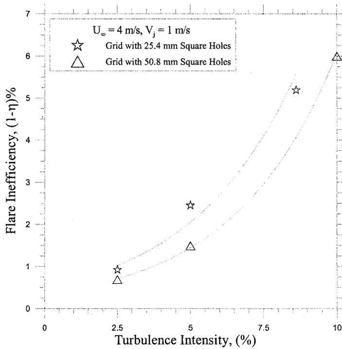
**Figure 5.5: Inefficiency of the flares having low flare gas flow rate subjected to varying turbulence intensities generated by the grid with 25.4 mm square holes**
