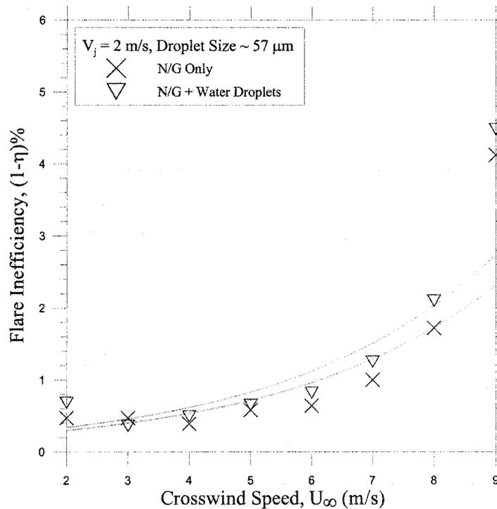
**Figure 4.19: Effects of distilled water droplets on the inefficiency of the flare with high flare gas exit velocity in crosswind**
