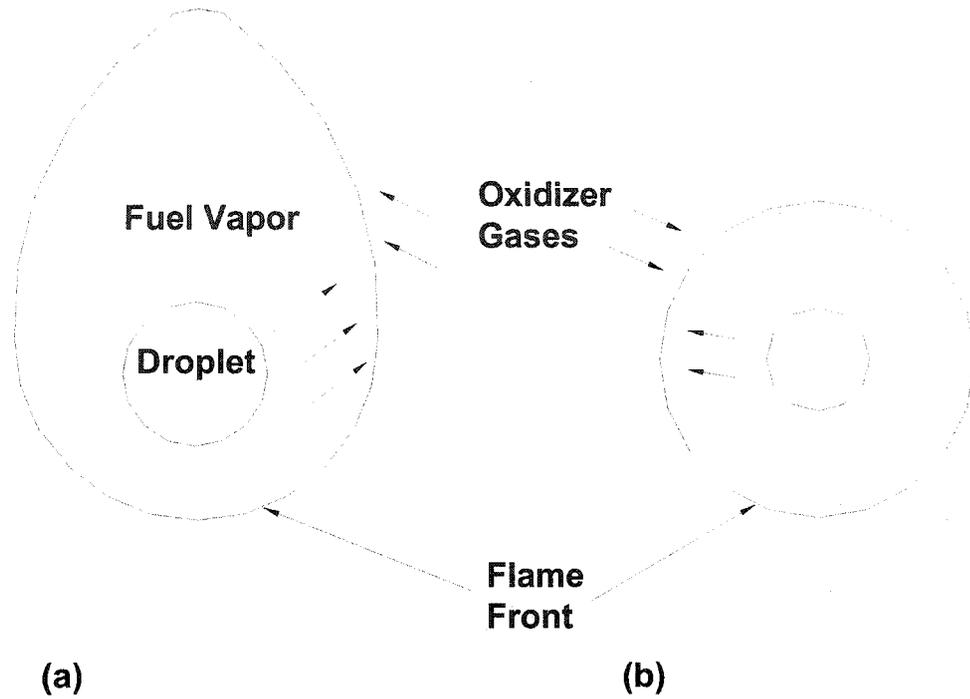
Figure 2.7: Shapes of diffusion flames surrounding a burning spherical fuel droplet
