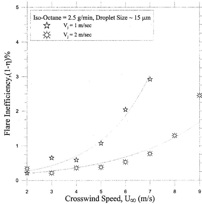
**Figure 4.4: Effects of the flare gas exit velocities on the flare inefficiency having same sizes of droplets and mass flow rates of iso-octane**
