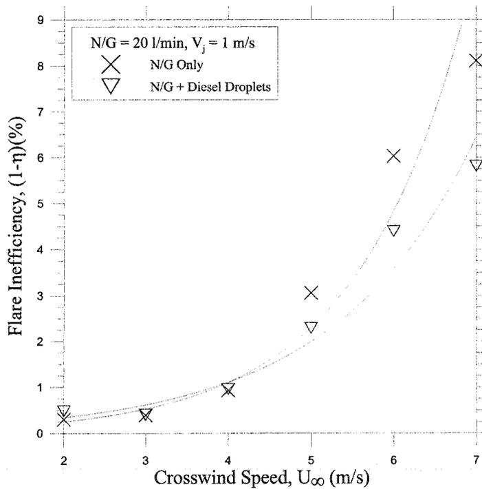
**Figure 4.13: Effects of diesel droplets on the inefficiency of the flares in crosswind**
