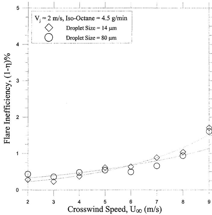
**Figure 4.8: Effects of iso-octane droplets size on the inefficiency of the flares with higher jet exit velocity in crosswind**
