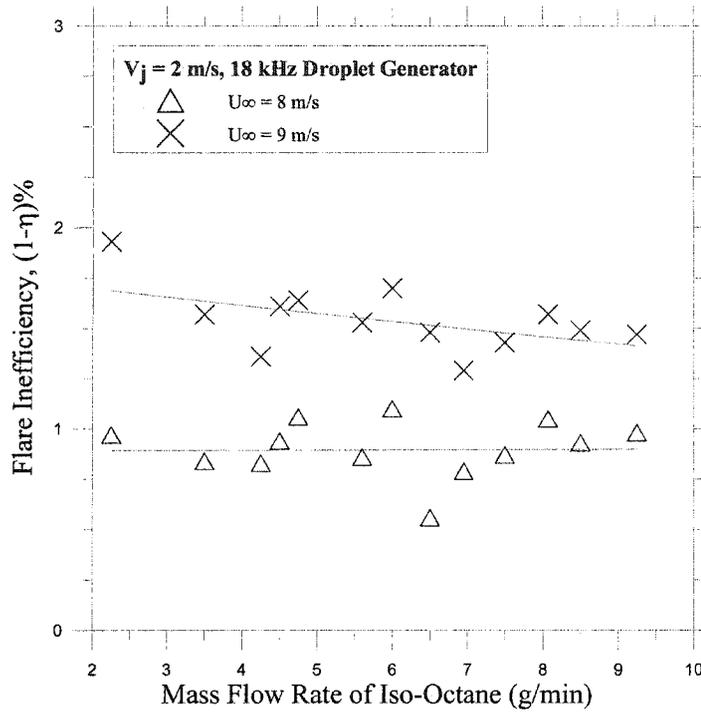
**Figure 4.12: Flare inefficiency as a function of mass flow rate of iso-octane with higher jet exit velocity using 18 kHz droplets generator**
