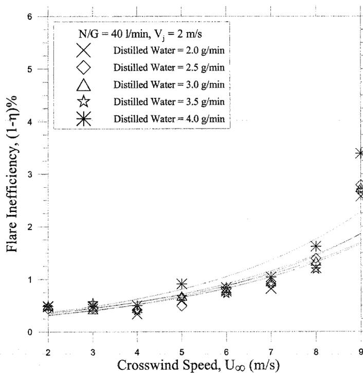
**Figure 4.23: Inefficiency of the flares having high jet exit velocity with varying flow rates of distilled water using 48 kHz droplets generator**
