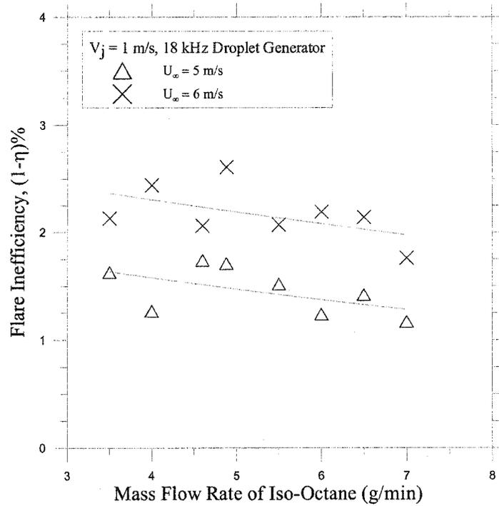
**Figure 4.10: Flare inefficiency as a function of mass flow rate of iso-octane using 18 kHz ultrasonic droplets generator**
