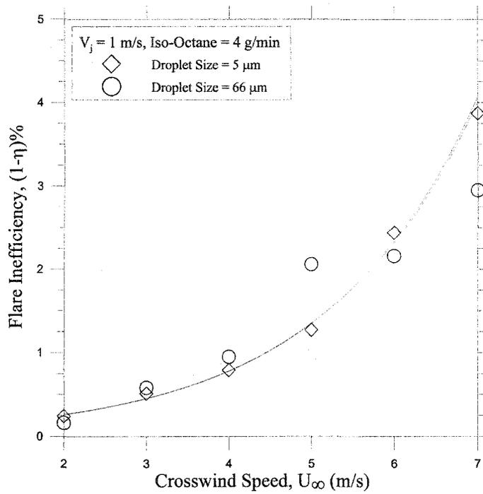
**Figure 4.6: Effects of iso-octane droplet size on the inefficiency of the flares with low flare gas exit velocity in crosswind**
