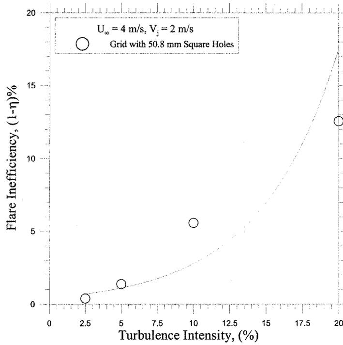
**Figure 5.3: Inefficiency of the flares having high flare gas flow rate subjected to varying turbulence intensities generated by the grid with 50.8 mm square holes**
