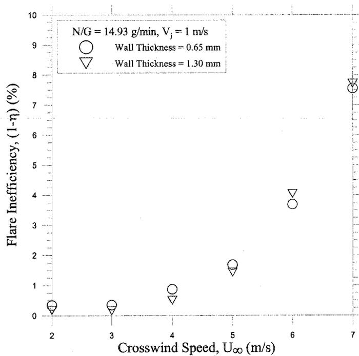
**Figure 5.8: Effects of decreased wall thickness on the inefficiency of the flares having low flare gas flow rates and jet exit velocity in crosswind**
