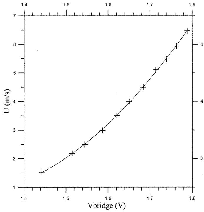
**Figure 3.9: Hotwire anemometer calibration curve**
