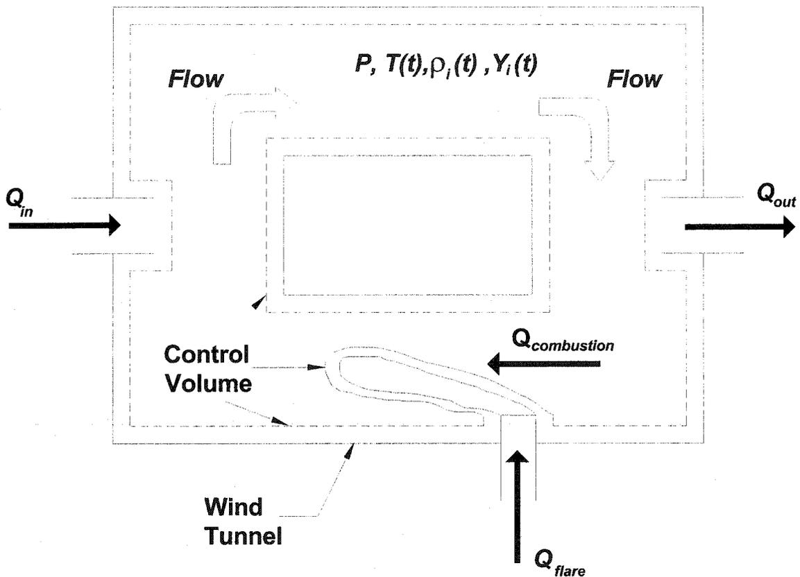
Figure B.1: A model for wind tunnel as constant pressure enclosure (Johnson *et.al.*, 2001)
