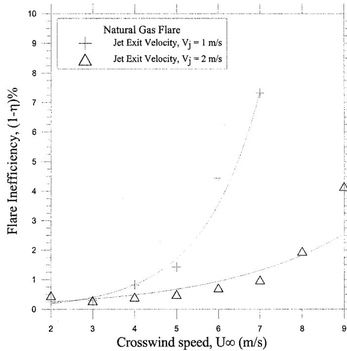
**Figure 4.2: Effects of crosswinds and flare gas exit velocity on the inefficiency of the flares**
