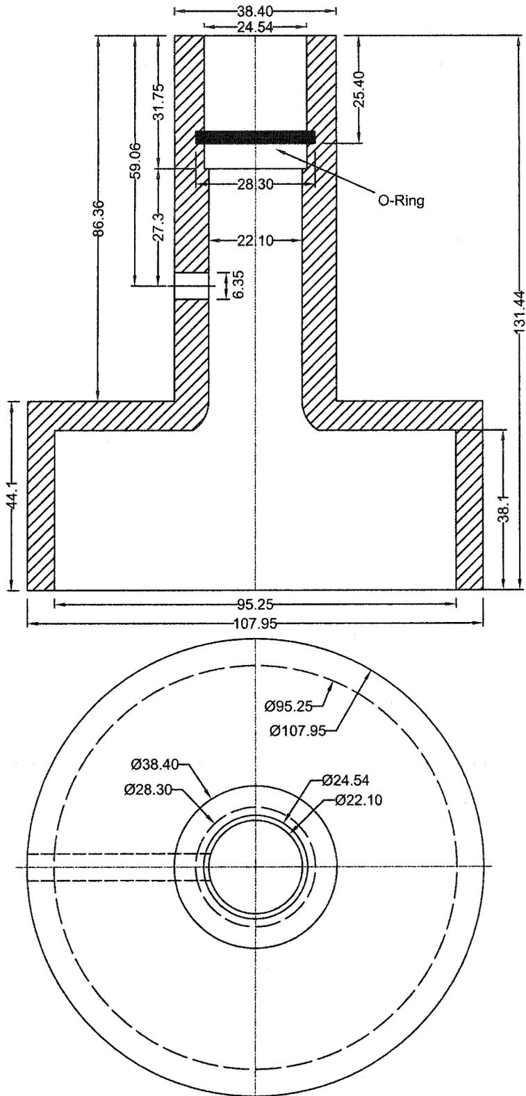
**Figure 3.3: Cap for holding the flare stack
