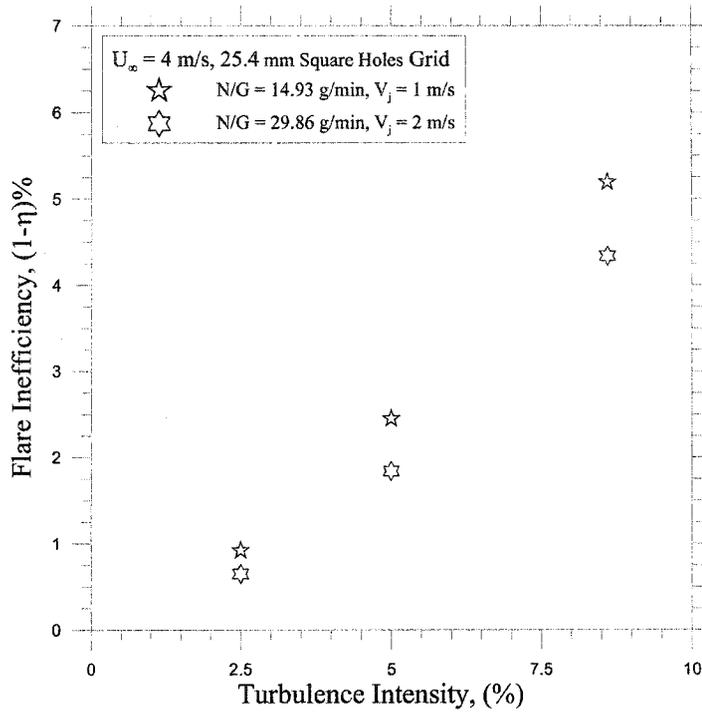
**Figure 5.7: Inefficiency comparison of the flares with two different flare gas flow rates subjected to the same turbulent crosswind conditions**
