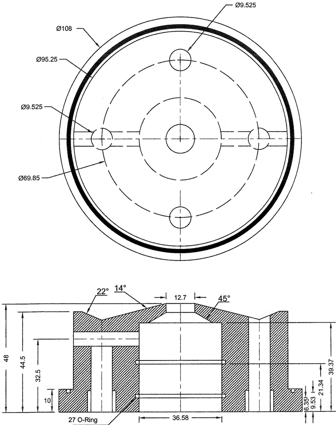
**Figure3.1: Capsule for 18 kHz ultrasonic droplets generator**
