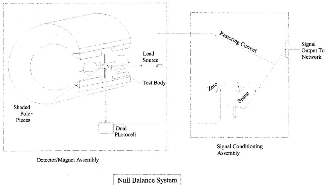
**Figure A.7: Paramagnetic Detector Technology**
