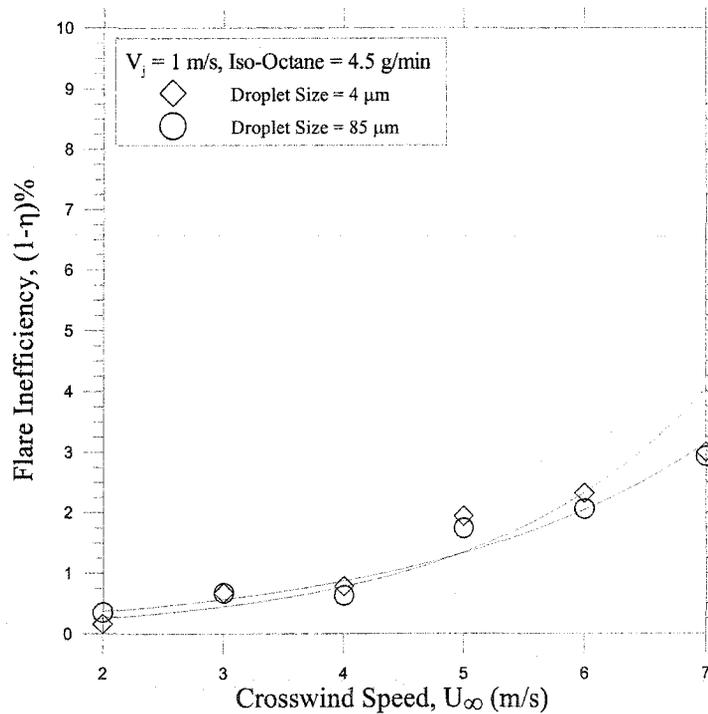
**Figure 4.7: Effects of iso-octane droplets size on the flare inefficiency with low jet exit velocity in crosswind**
