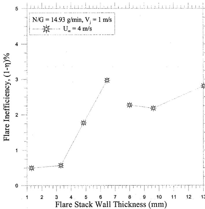
**Figure 5.12: Effects of varying wall thickness on the inefficiency of low jet exit velocity flare at 4 m/s**
