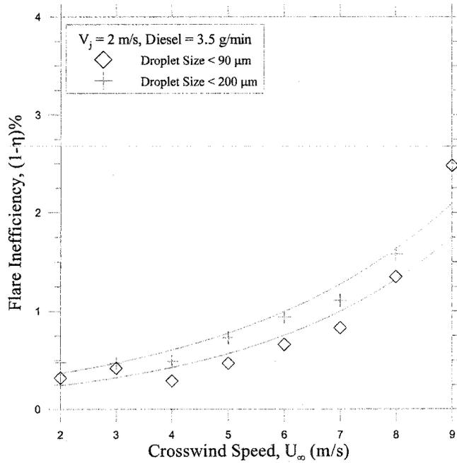
**Figure 4.15: Effects of the diesel droplet size on the inefficiency of the flares with higher flare gas exit velocity**
