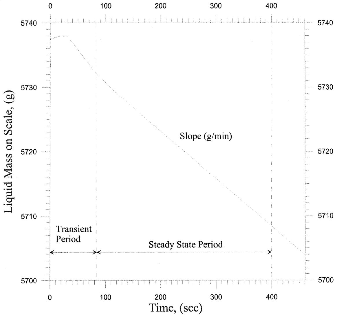
**Figure 3.6: Time trace of liquid mass flow rate**
