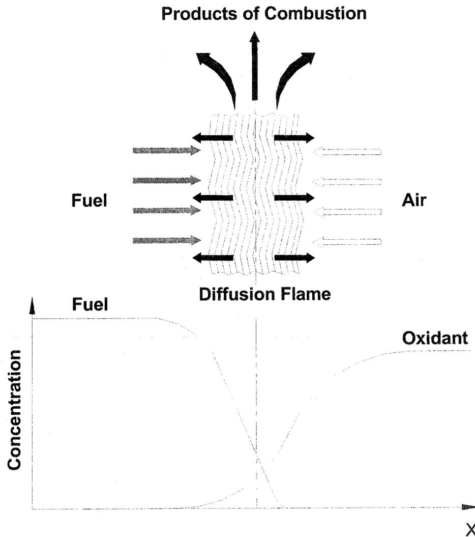
Figure 2.2: Diffusion of fuel and oxidant to a flame
