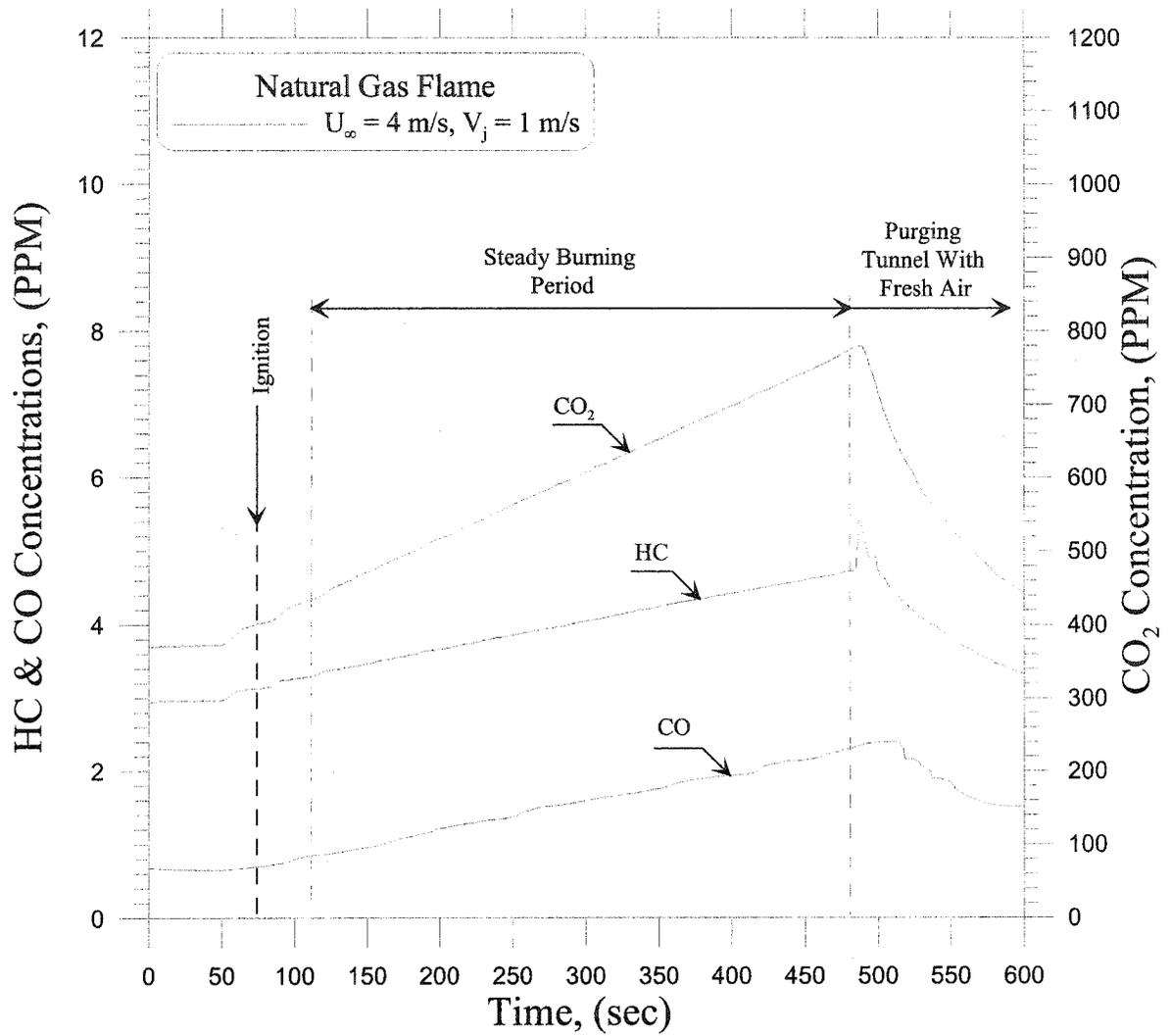
**Figure 4.1: Time trace of the concentrations of major carbon-containing species during a typical test in the wind tunnel**
