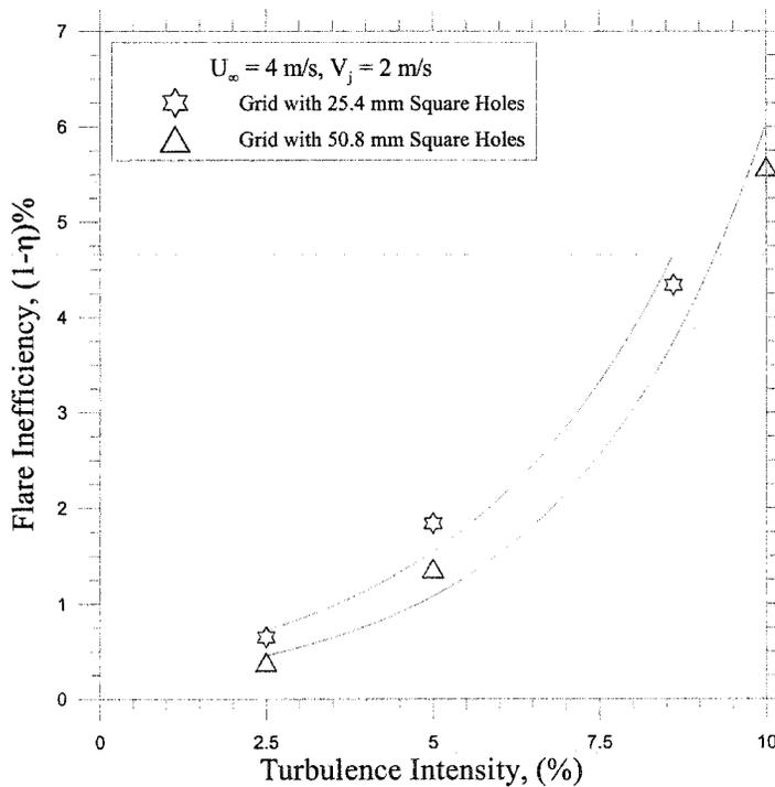
**Figure 5.6: Inefficiency of the flares having high flare gas flow rate subjected to varying turbulence intensities generated by the grid with 25.4 mm square holes**
