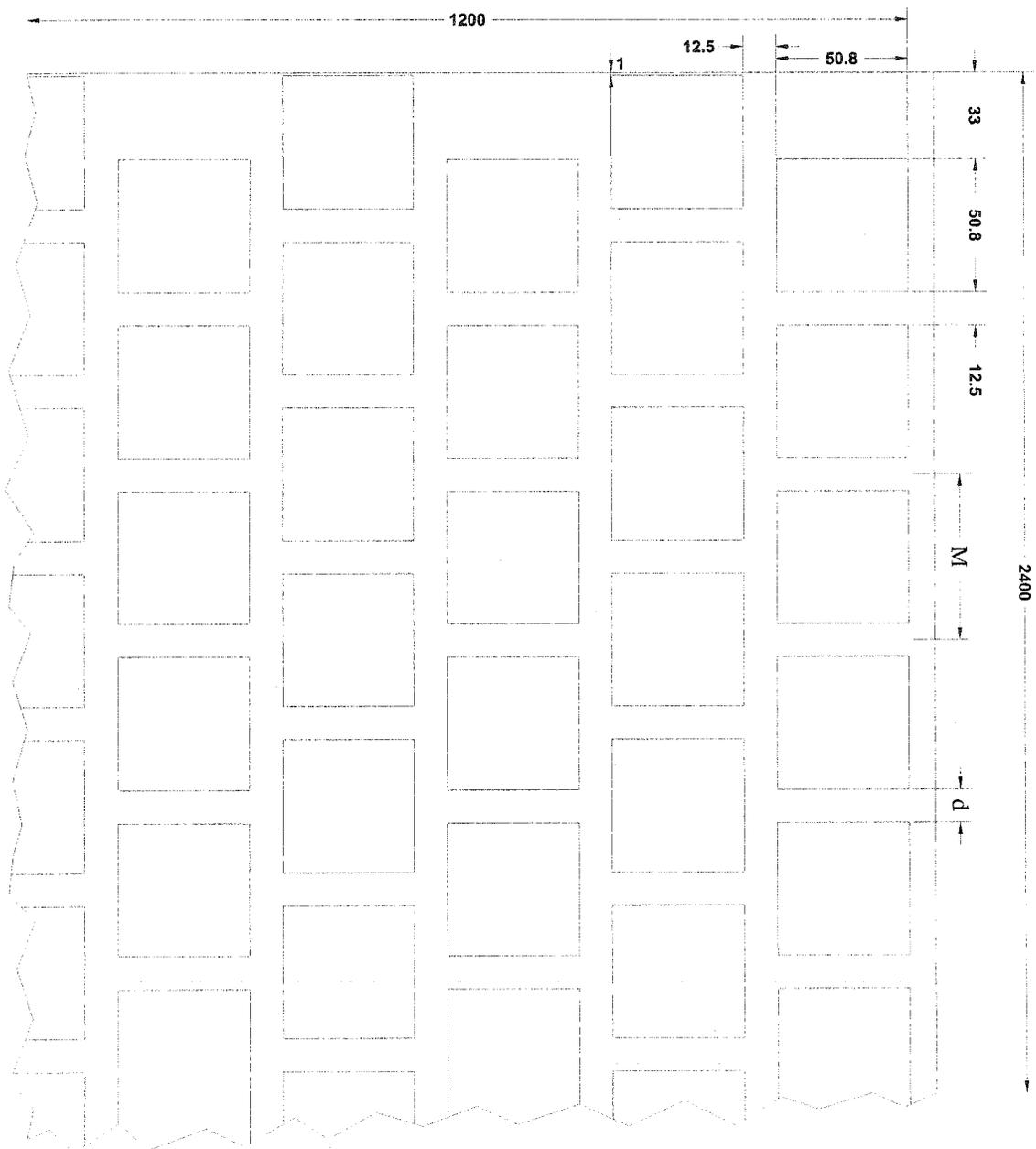
**Figure 3.8: 4 x 8 m and 1.6 mm thick grid with 50.8 mm square holes
