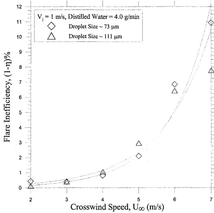
Figure 4.20: Effects of water droplet size on the flare inefficiency in crosswind
