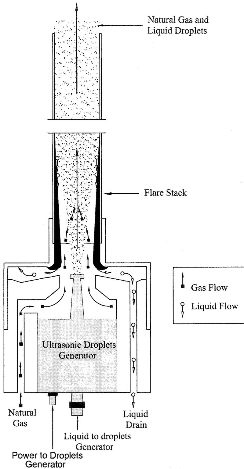
**Figure 3.4: Droplets generation and their introduction into the flare stream (Kostuik, 2000)**
