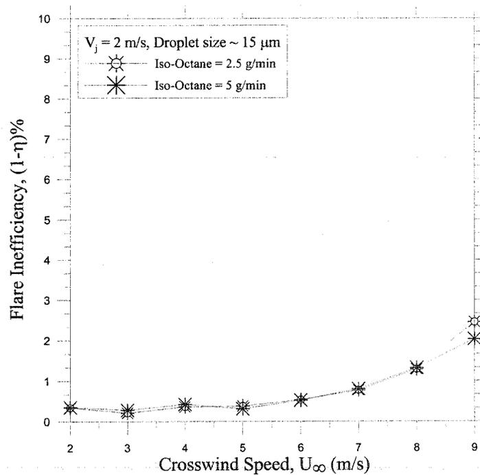
**Figure 4.11: Effects of the mass flow rates of natural gas and iso-octane on the flare inefficiency with the same size of droplets in the flare stream**
