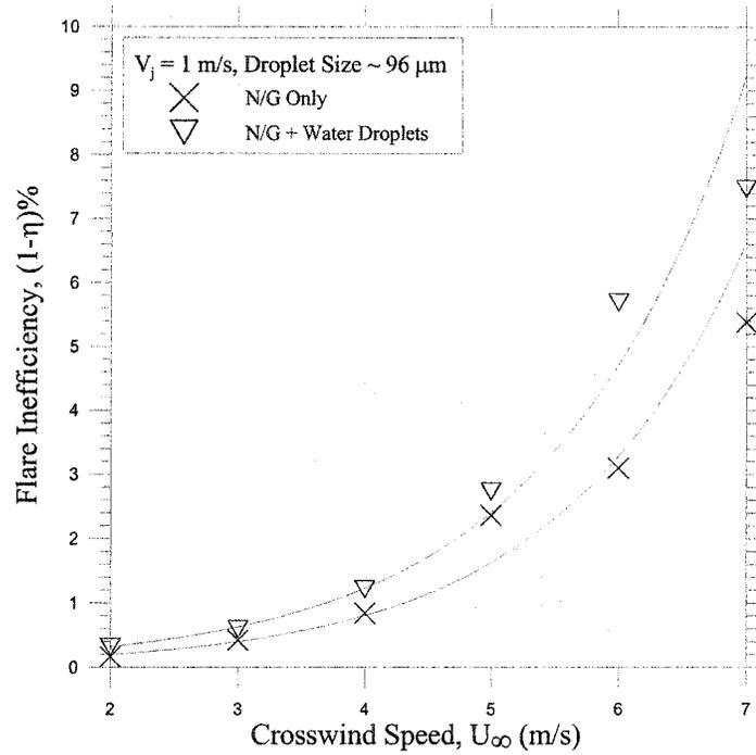
**Figure 4.18: Effects of distilled water droplets on the inefficiency of the flare with low flare gas exit velocity in crosswind**
