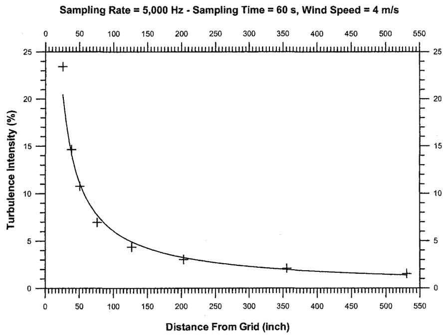
**Figure 3.11: Turbulence intensity decay behind the gird with 50.8 mm square holes**
