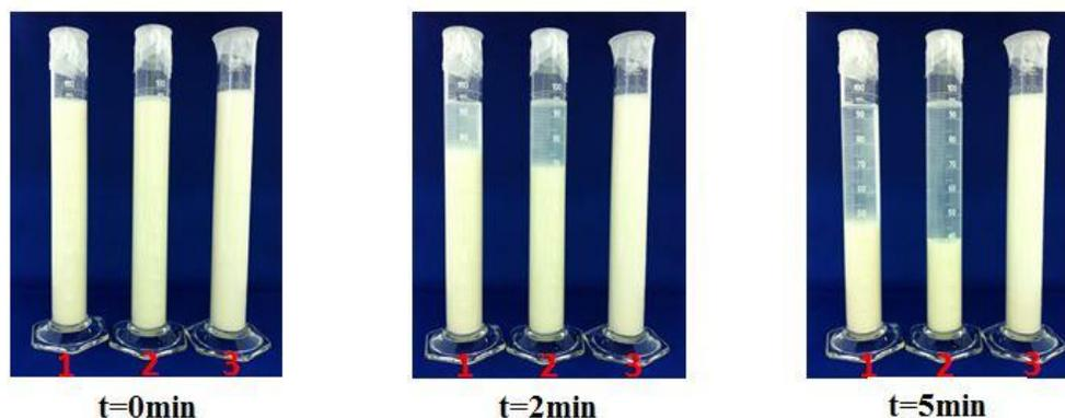
**Figure 0.8** Real-time pictures for the settling of 2 wt% kaolinite suspensions at pH=3.4 for t=0, 2 and 5 minutes. Note: samples 1, 2 and 3 contain 0, 0.05 wt% and 0.40 wt% of PCE respectively
