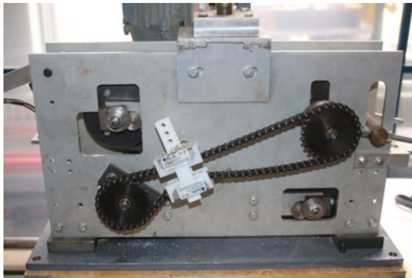
Figure 3-3 Image of caterpillar puller that moves the mandrel through as the preform is braided on it
