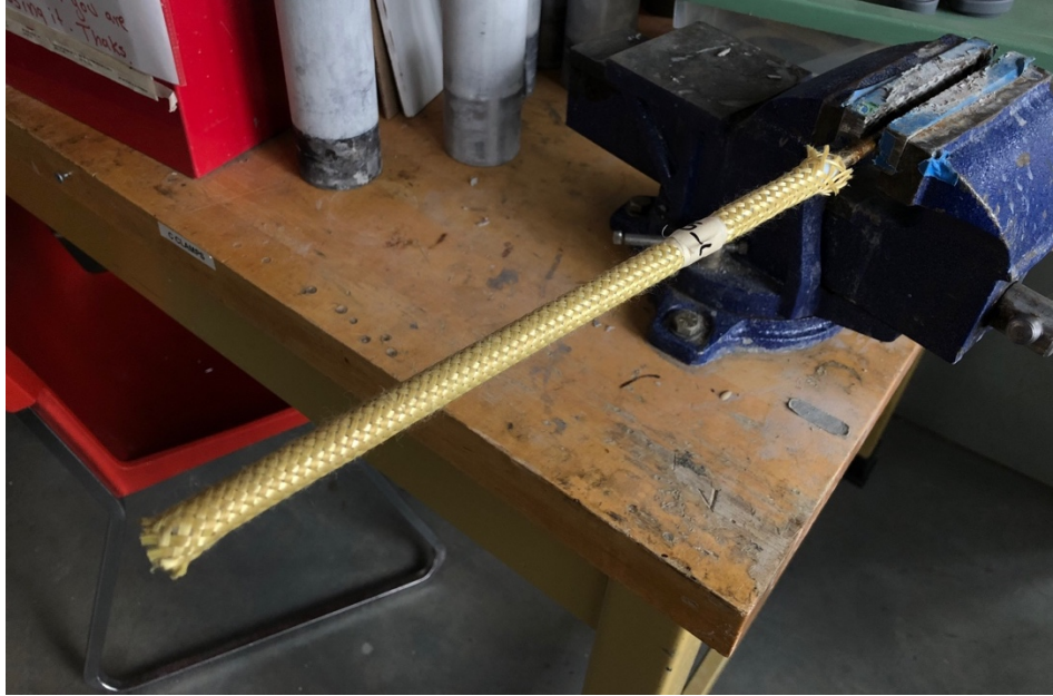
Figure 3-6 Image of a preform socked onto the clamped Teflon-shell/steel-core curing mandrels
