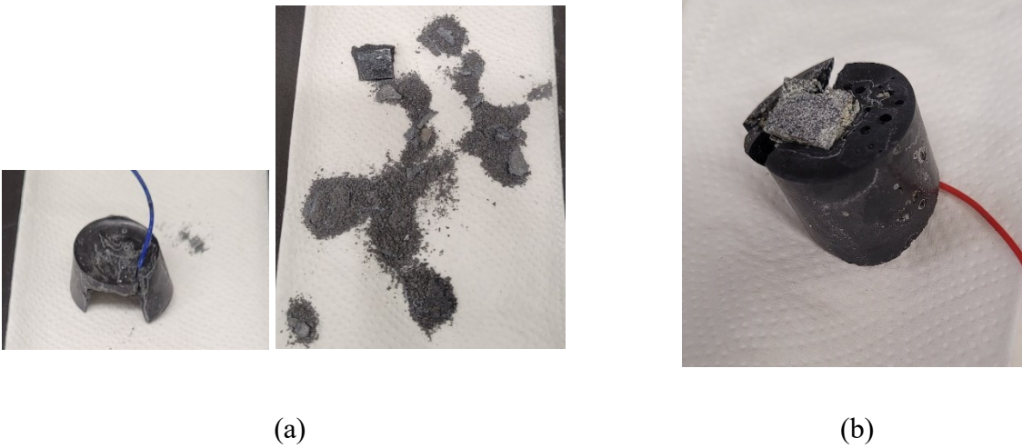
Figure 4.14. Corroded samples in 0.59 M KCl at 90 °C: (a) Complete dissolution of DA18 (sample dropped off the mold) and (b) Severe corrosion of DA25 sample showing part of the samples dropped off the surface.
