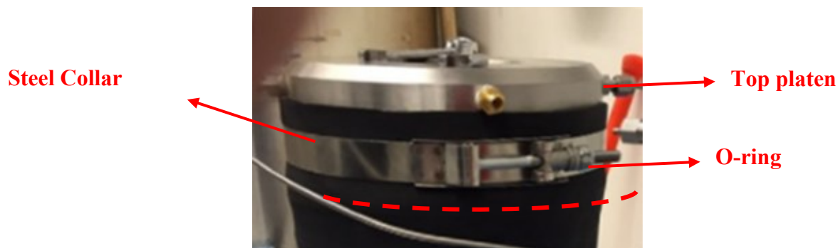
Figure B.8: Top Platen Installation
