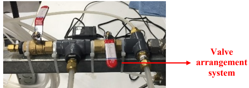
Figure B.13: Valve Arrangement System
