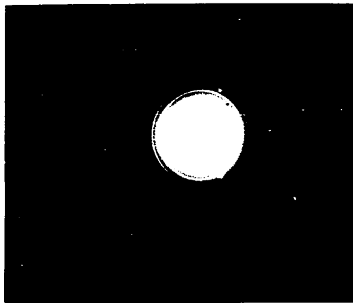
FIGURE 50. Precipitate in pyrolytic graphite-titanium alloy with [110] zone planes perpendicular to graphite basal planes.
