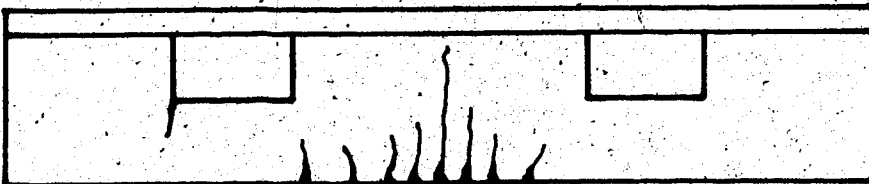
Flexural failure at midspan
