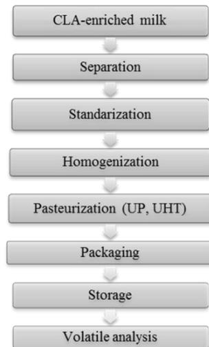
Figure 4.1. General overview of the protocol used for conventional thermal treatments of milk (UP and UHT).
