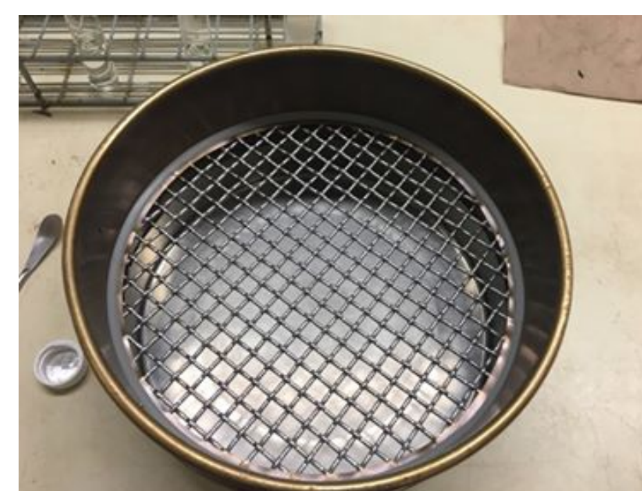
Figure 4: The 8mm sieve used to sieve our soil samples.
