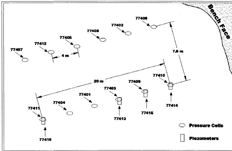
Figure 154: Survey locations for ground sensors
