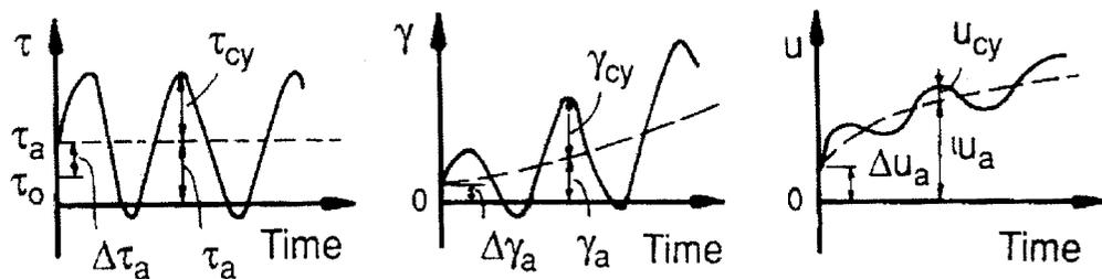
Figure 66: Shear stress, shear strain and pore pressure during cyclic loading (after Anderson, 1988)
