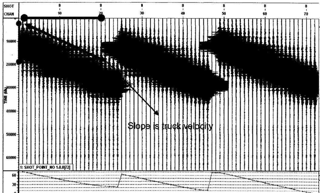
Figure 28: Truck velocity from passive data
