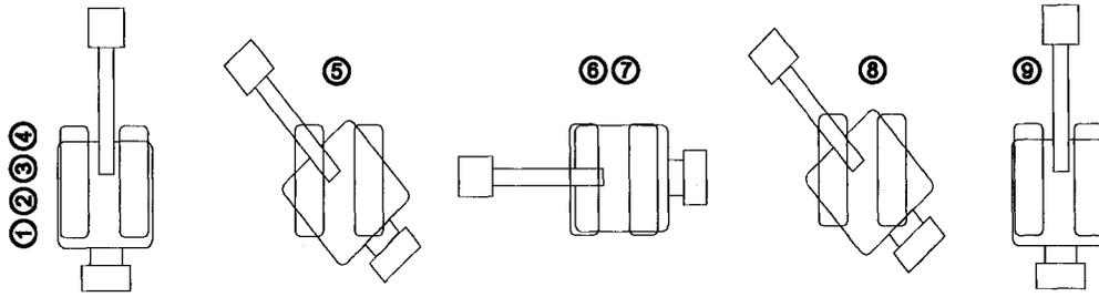
Figure 4: Shovel duty cycle (after Joseph et al. 2003)
