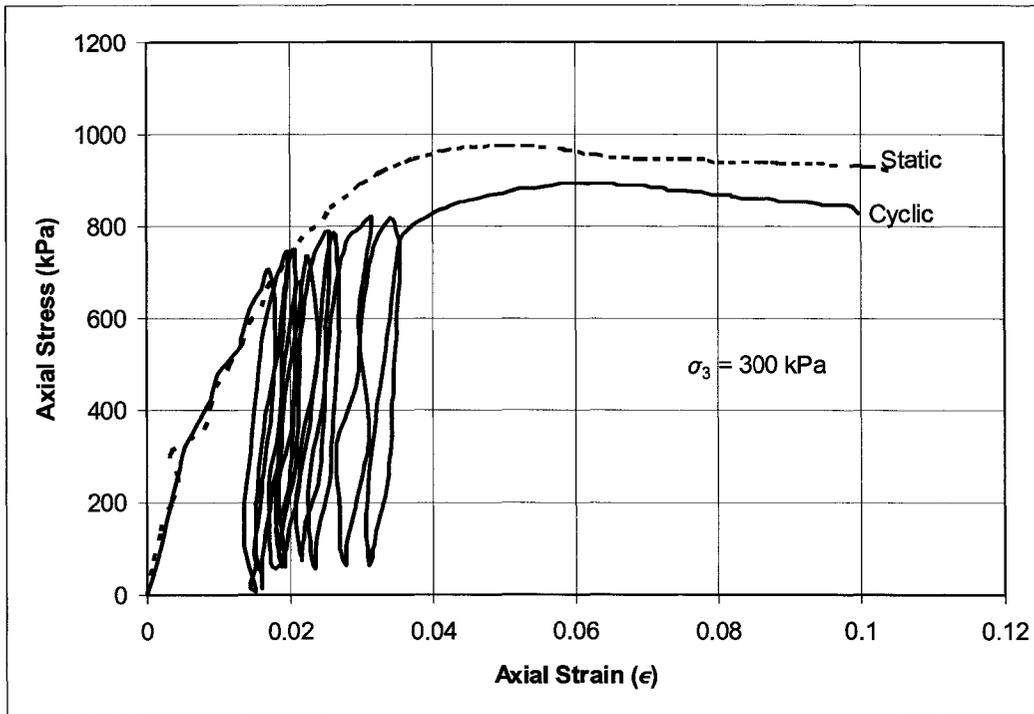
Figure 82: Cyclic and conventional stress-strain curve comparison for 300 kPa confining pressure
