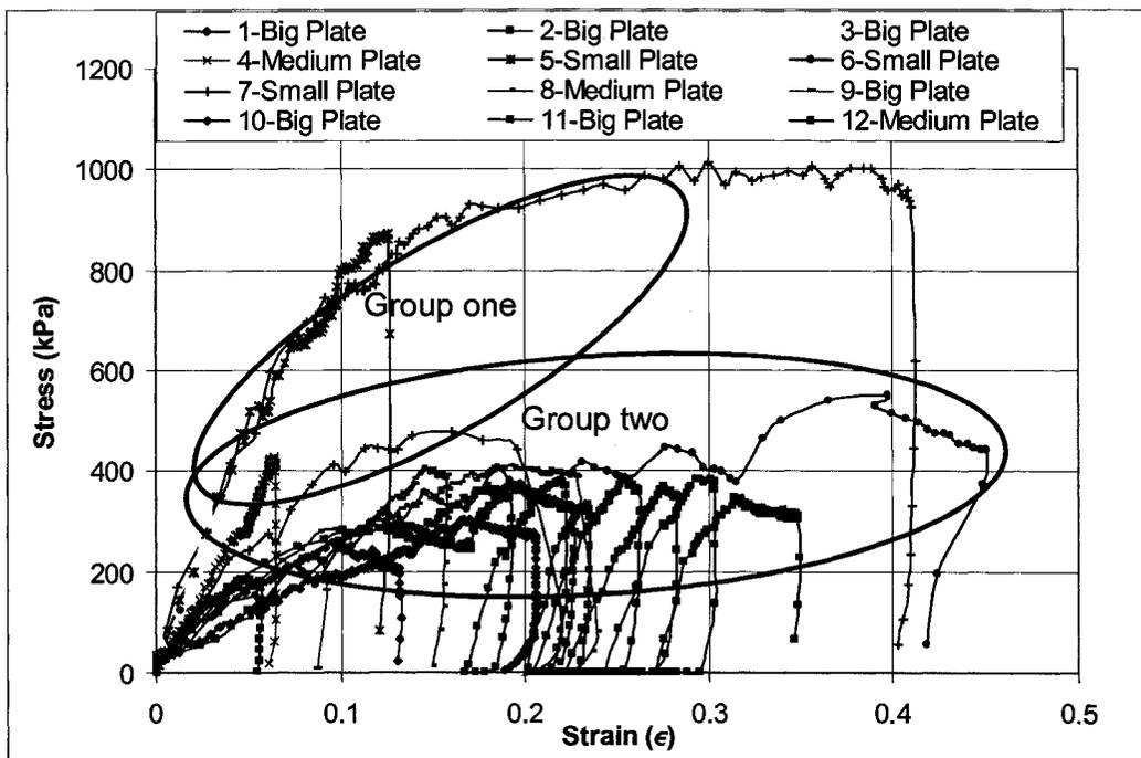
Figure 91: All cyclic plate load test
