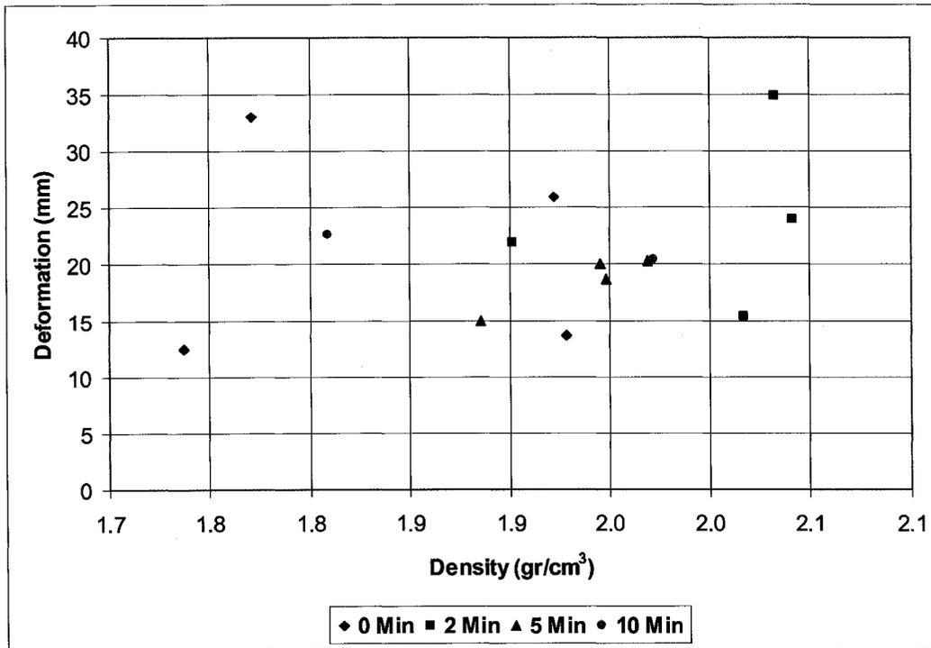
Figure 138: Initial density versus initial loading deformation
