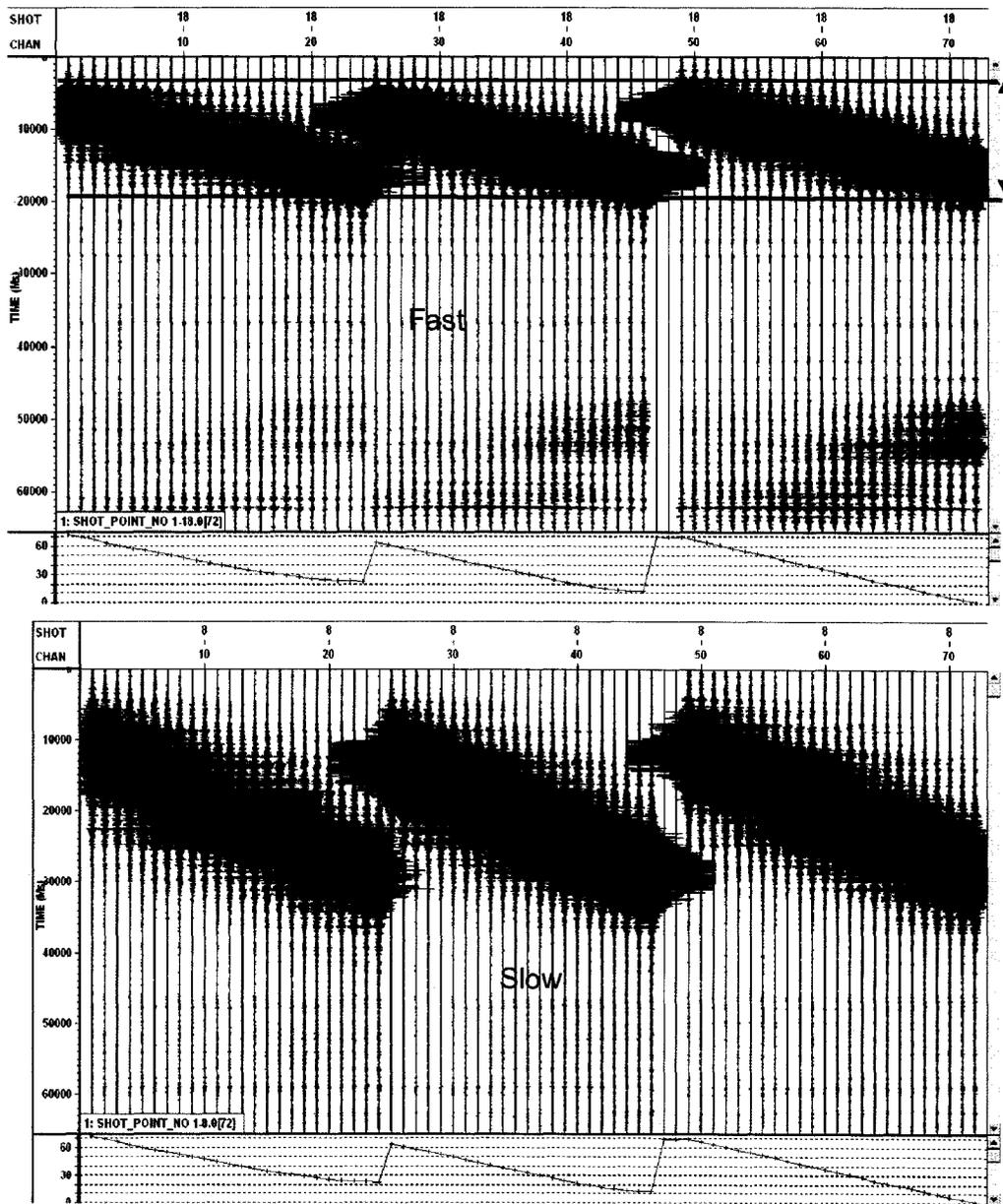
Figure 30: Slow truck velocity vs. fast truck velocity
