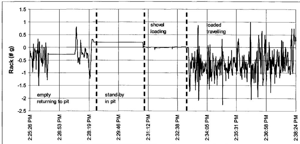
Figure 13: The calculated rack of an ultra-class truck (after Joseph 2003)
