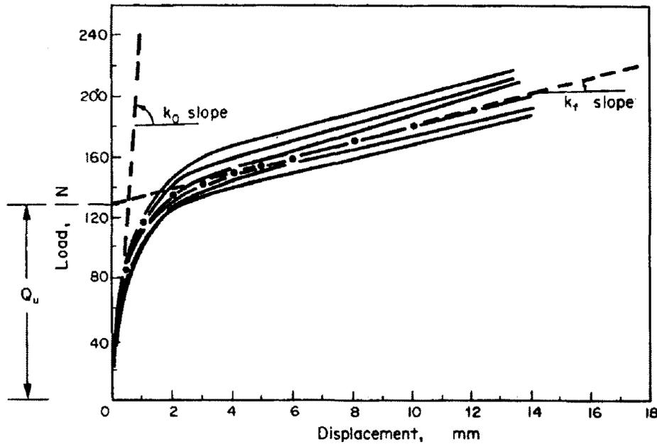
Figure 67: Change of the stiffness during cyclic loading (after Butterfield and Georgiadis 1980)
