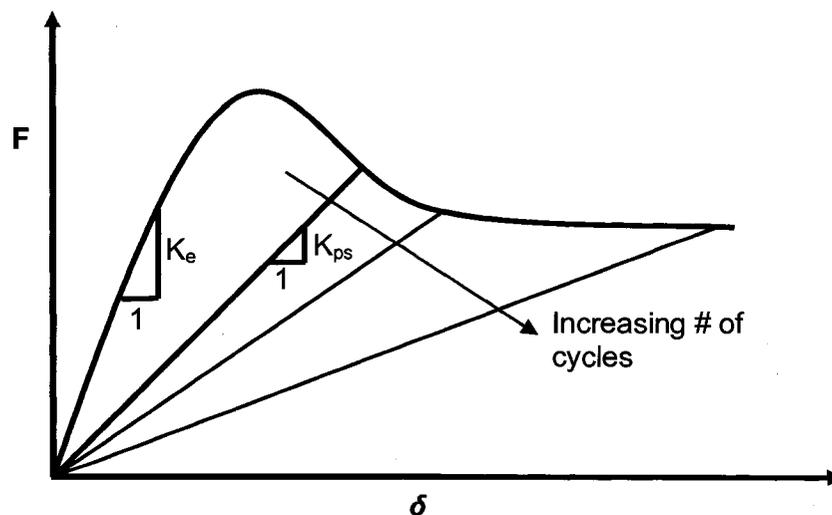
Figure 7: Oil sand stiffness change under cyclic loading (after Joseph 2003)
