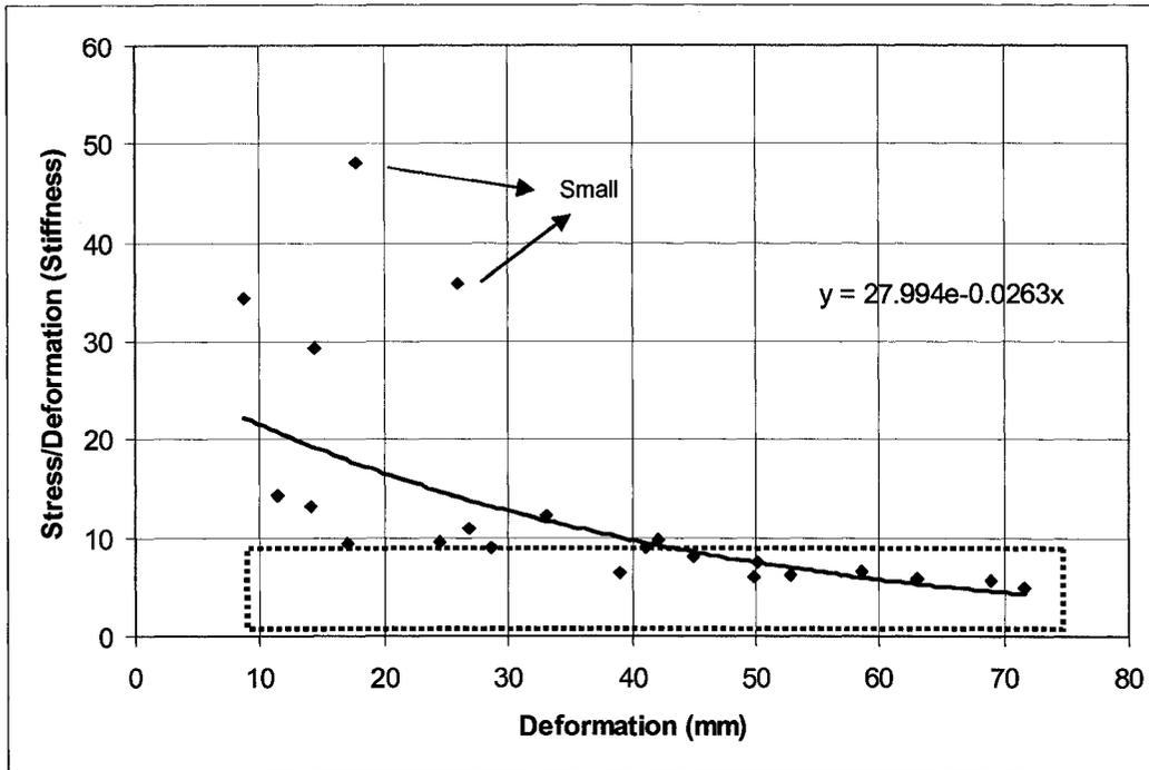
Figure 90: Changing stiffness during loading for oil sand
