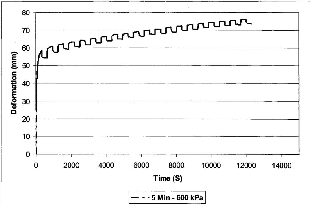
Figure 152: Deformation vs. Time for 600 kPa and 5 Min test
