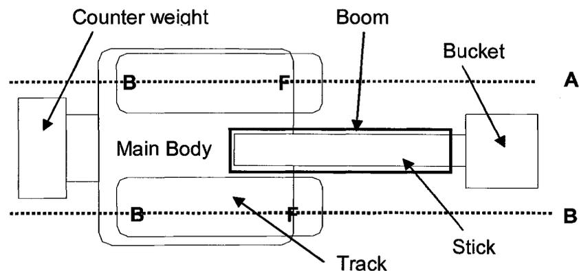
Figure 163: Sections of calculated stress for an ultra-class shovel
