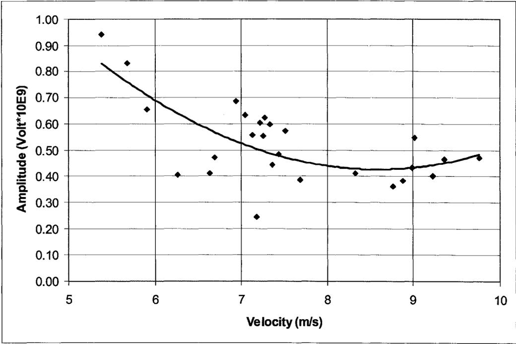
Figure 42: Unloaded truck velocity vs. sum of amplitude for day 3
