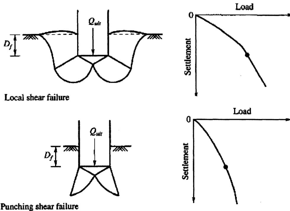
Figure 127: Bearing capacity failure (after Vesic 1963)
