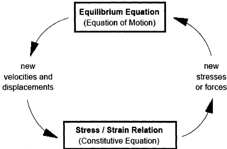
Figure 94: General calculation sequence in FLAC (after FLAC 2002)
