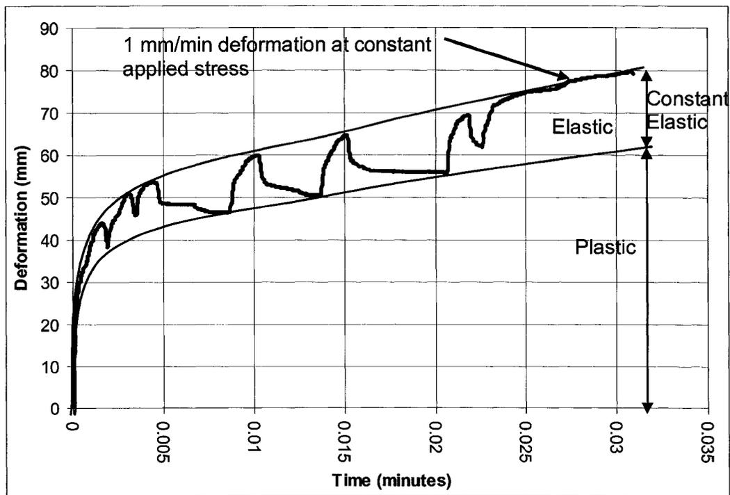
Figure 93: Plastic and elastic deformation components
