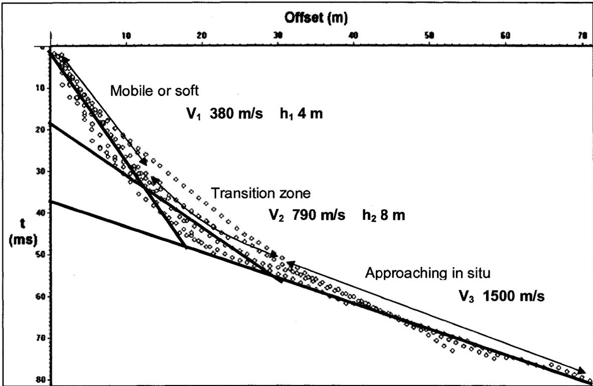
Figure 2: Ground condition and corresponding velocity profile (after Welz 2001)
