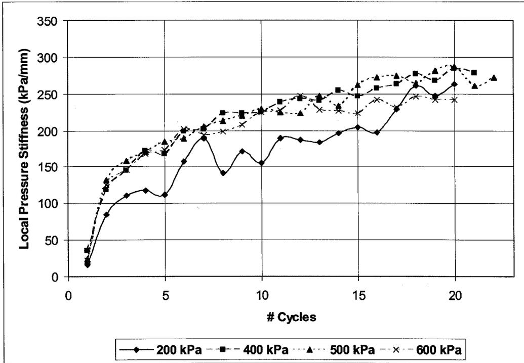
Figure 144: Local pressure stiffness during cycles for 2-min. duration cycles
