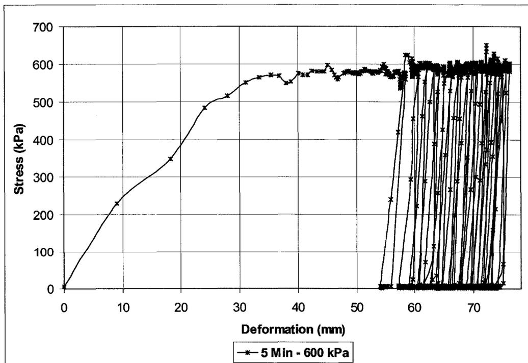
Figure 151: Stress Vs. deformation curve for 600 kPa and 5 Min test
