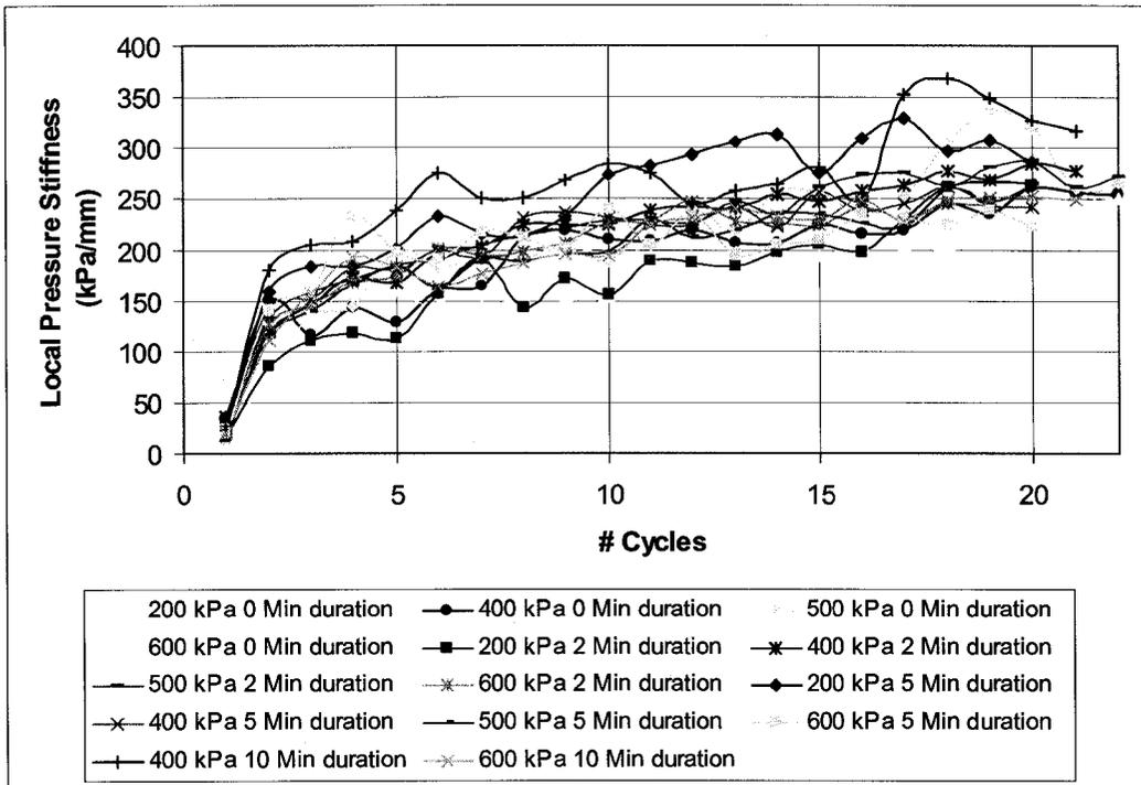
Figure 145: Local pressure stiffness during cycles for 0-10 min. duration cycles
