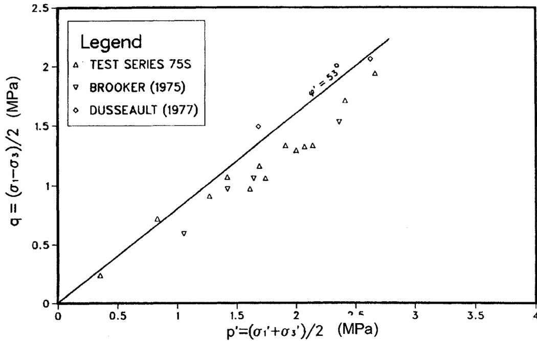
Figure 58: Ultimate shear strength of oil sand in undrained triaxial (after Plewes 1987)
