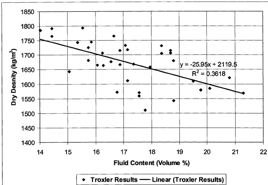
Figure 118: Troxler dry bulk density results vs. fluid content
