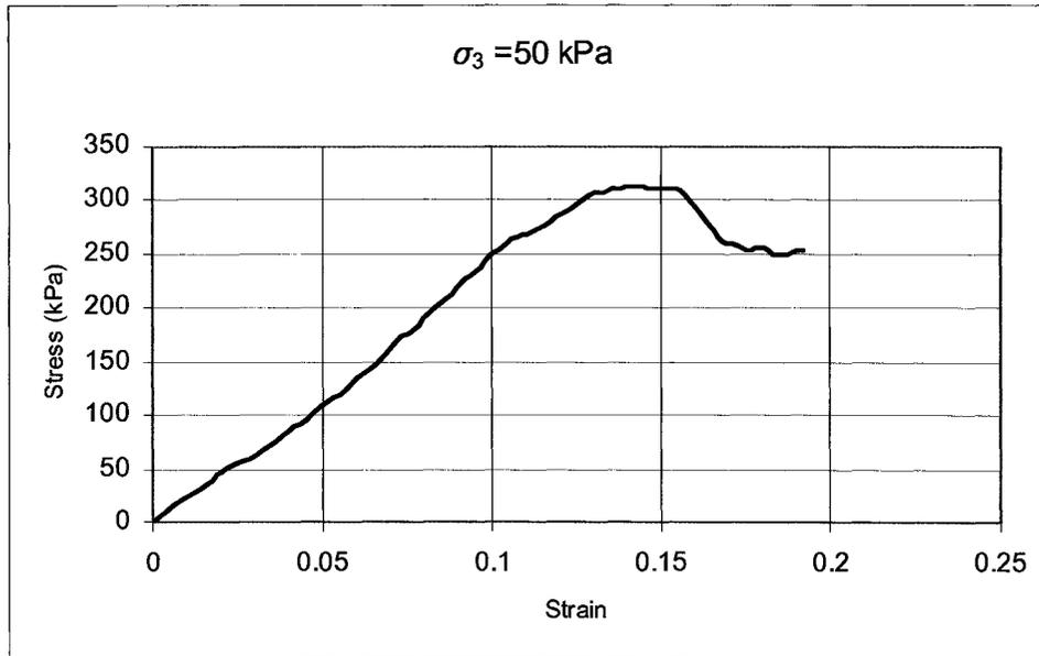
Stress-strain curve for %11 oil sand
