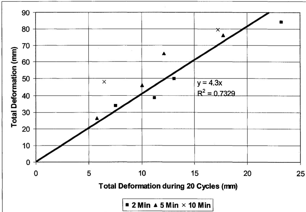
Figure 142: Total deformation versus deformation in 20 cycles for 2-10 min. (on removing the instantaneous 0-min data)
