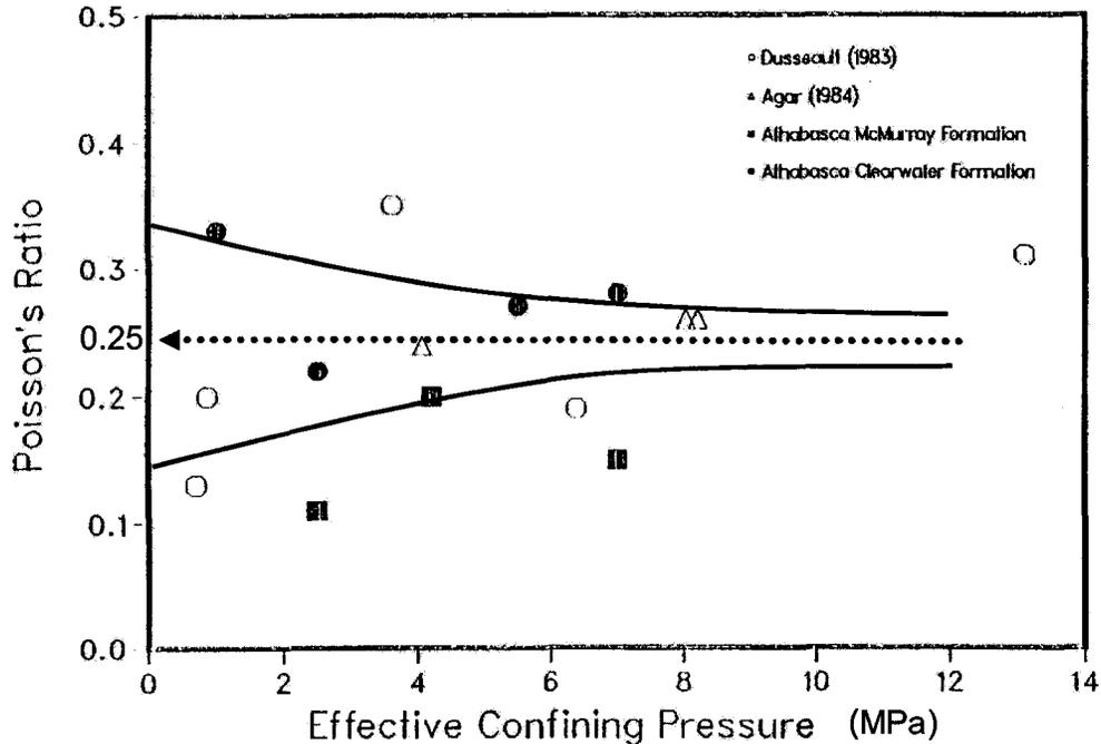
Figure 60: Change of Poisson's ratio with confining pressure (after Kosar 1989)
