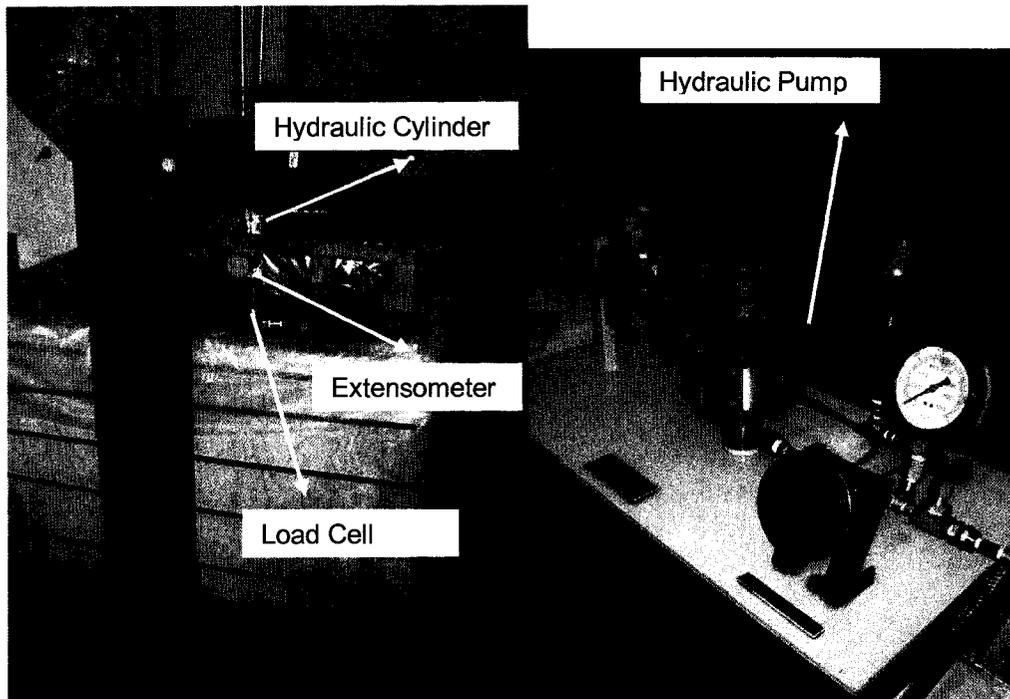
Figure 121: Plate load laboratory test set-up
