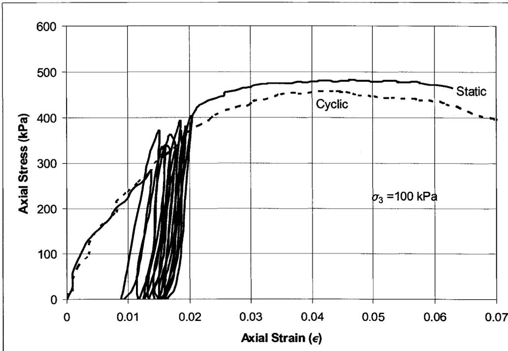
Figure 81: Cyclic and conventional stress-strain curve comparison for 100 kPa confining pressure
