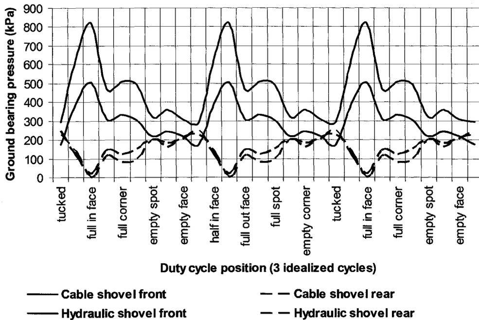
Figure 5: Cyclic ground pressure under shovel (after Joseph 2002)
