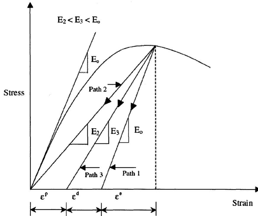
Figure 73: Path 1 ideal plastic deformation, path 2 perfectly brittle material and path 3 combination of plasticity and damage (after Al-Shayea 2003)
