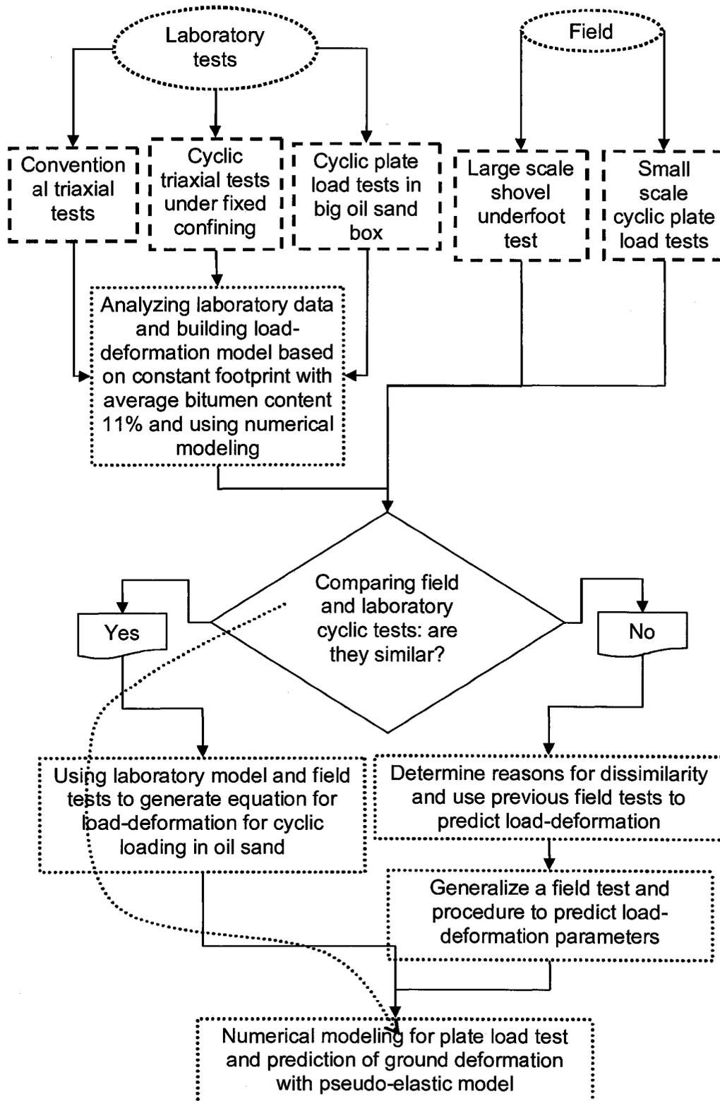
Figure 8: Flow chart of methodology and tests
