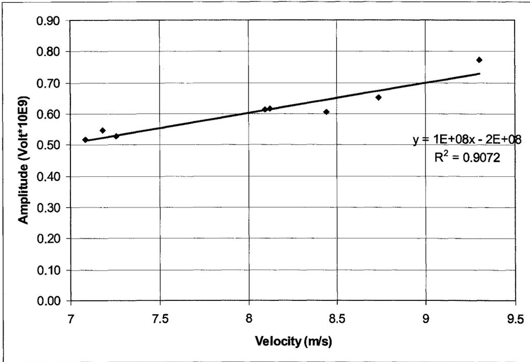
Figure 39: Sum of the amplitude vs. truck velocity for an unloaded truck day 1
