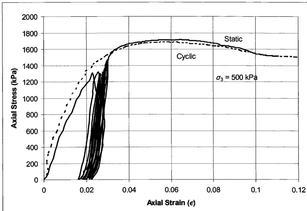
Figure 83: Cyclic and conventional stress-strain curve comparison for 500 kPa confining pressure
