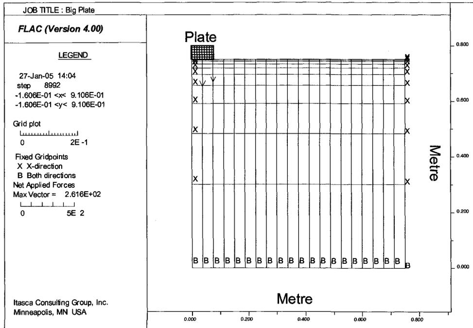
Figure 96: Boundary condition and applied load
