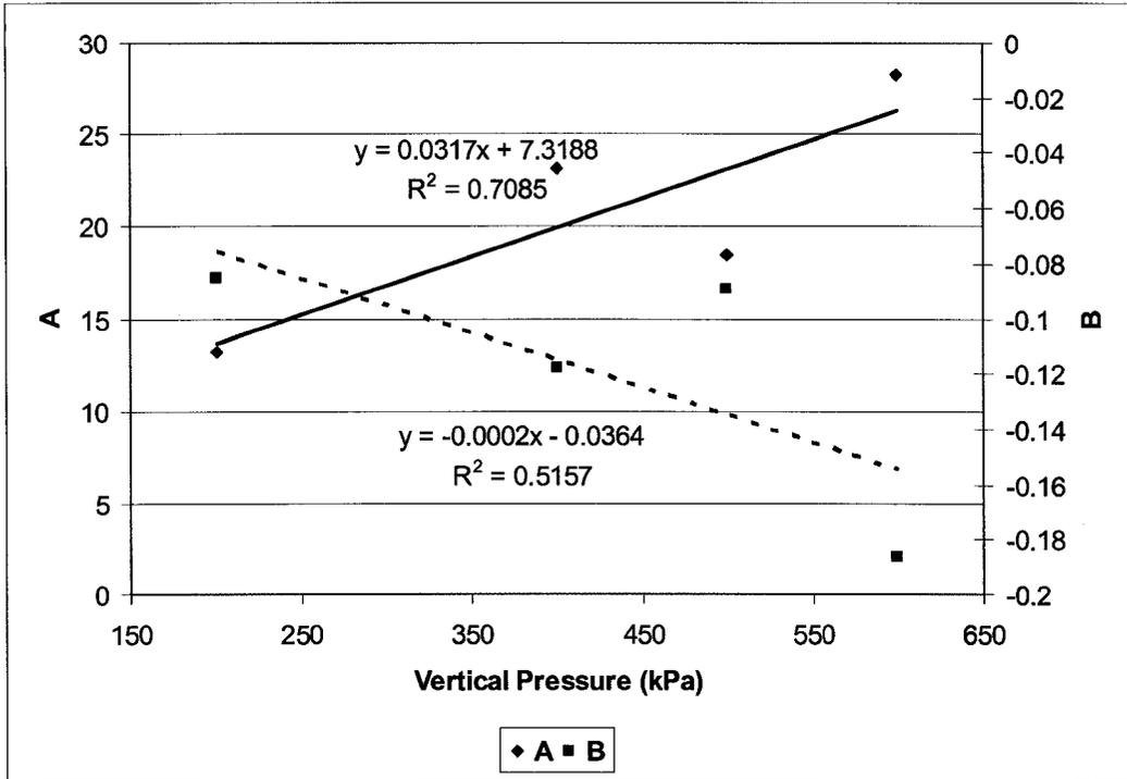
Figure 149: Coefficient factors for different vertical pressure level
