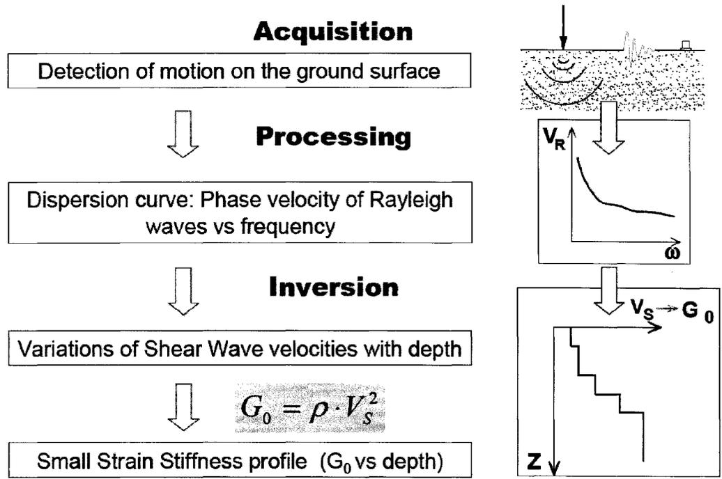
Figure 48: Sequence of obtaining Shear Wave velocities (from Matthews et al. 2000)
