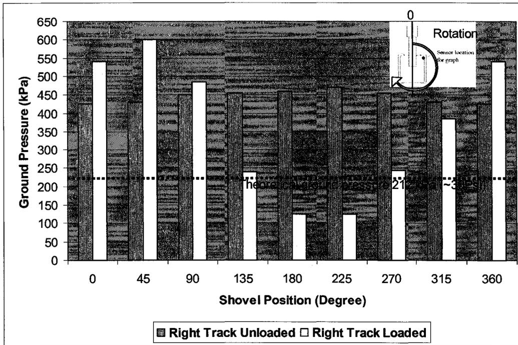
Figure 162: Ground pressures recorded at hold position
