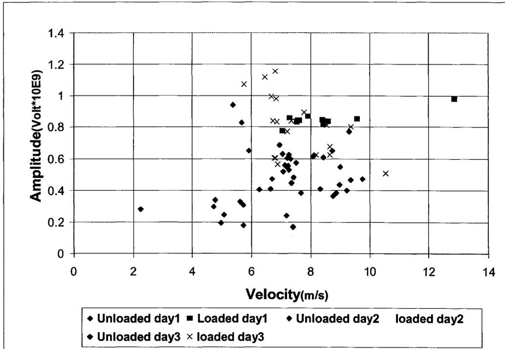
Figure 44: Loaded and unload trucks velocity vs. sum of amplitude for the 3 days
