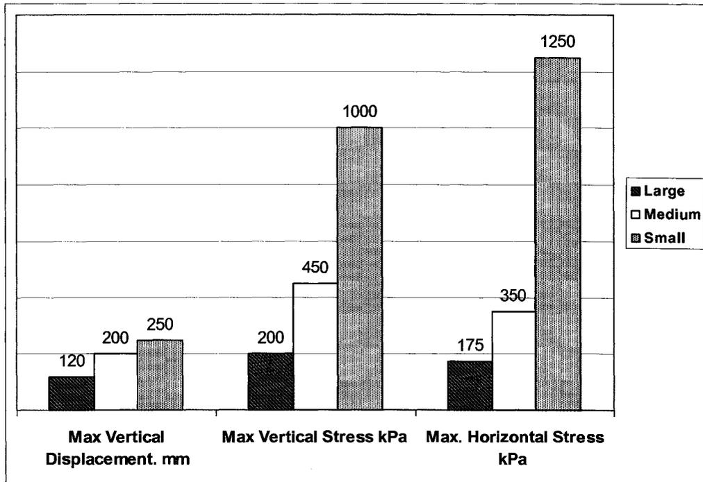
Figure 103: Summary of FLAC modeling for deformation and stresses
