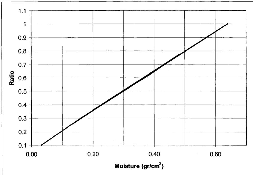
Figure 114: Moisture calibration curve for MC-1 densometer
