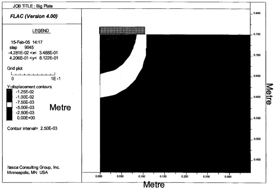
Figure 100: Vertical deformation under large plate
