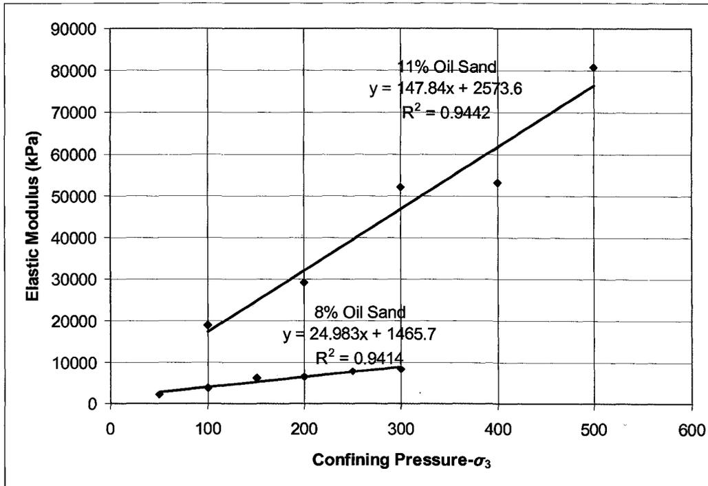
Figure 97: Elastic modulus change with confining pressure for 8 and 11% oil sand
