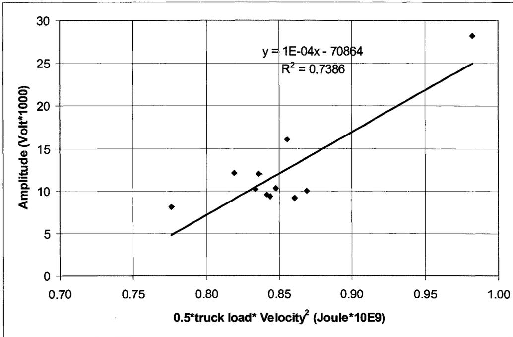
Figure 38: Kinematics energy vs. amplitude for load trucks
