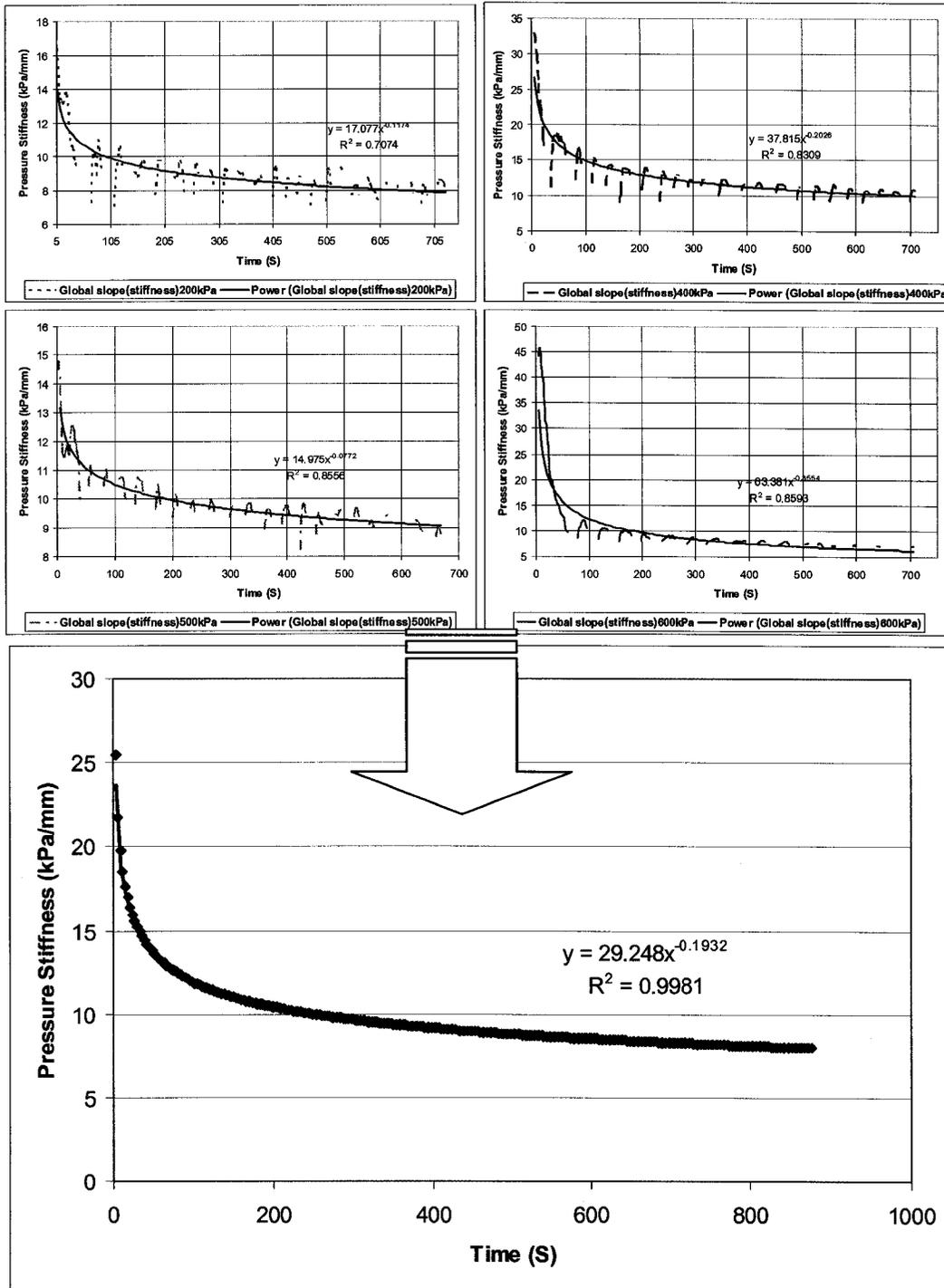
Figure 132: Curve fit method
