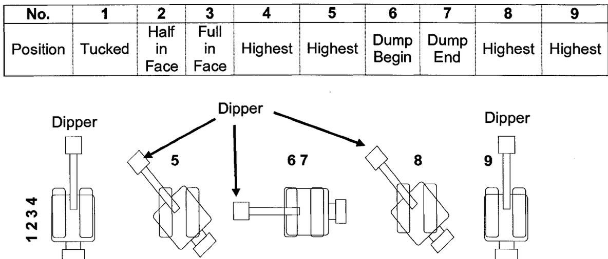
Figure 158: Different digging positions (after Joseph et al. 2003)
