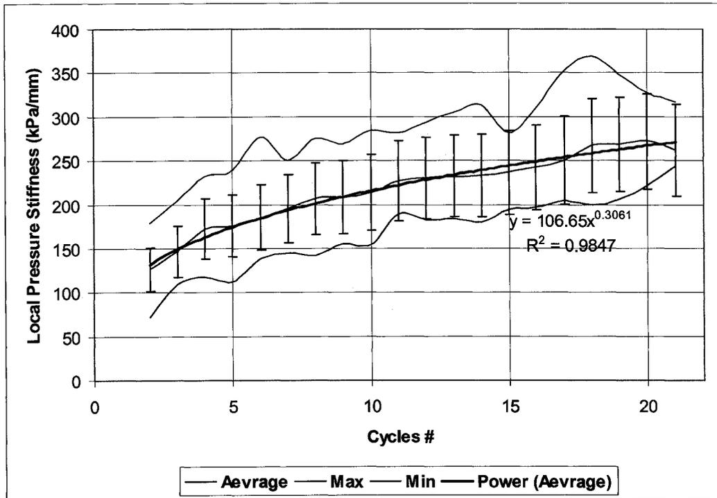
Figure 146: Average of values of local pressure stiffness for 0-10 min. duration cycles
