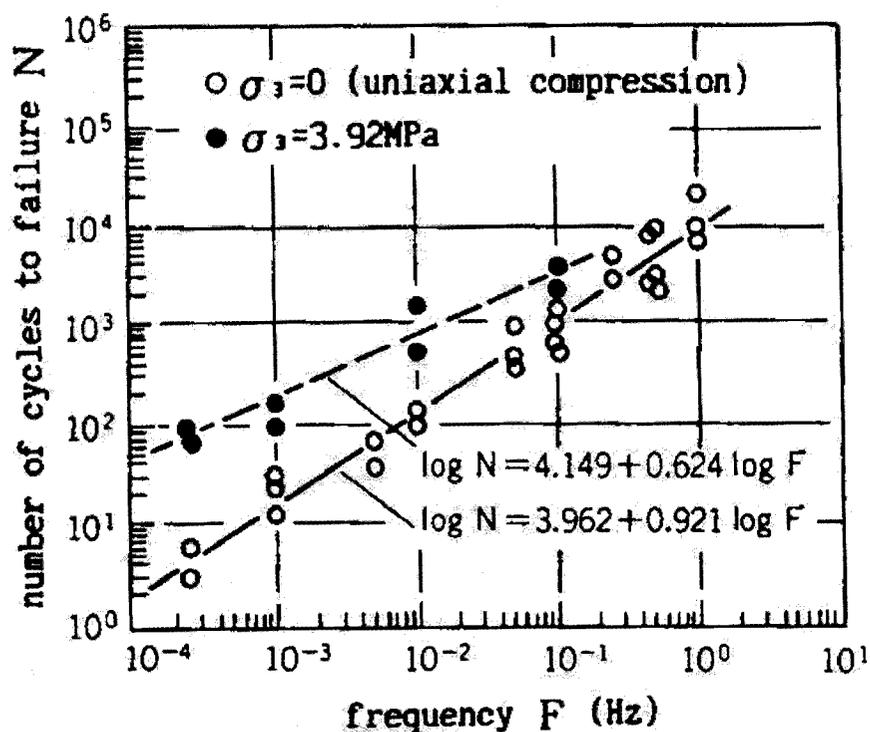
Figure 64: Number of cycles to failure  $N$  versus frequency  $F$ , at constant applied stress (after Ishizuka 1990)
