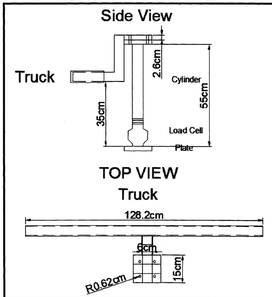
Figure 87: Cyclic plate load apparatus
