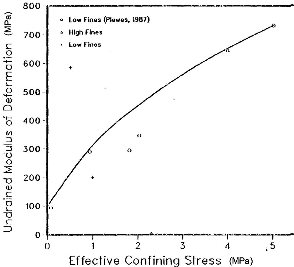
Figure 61: Tangent modulus of elasticity for undrained triaxial compression on oil sand (after Kosar 1989)
