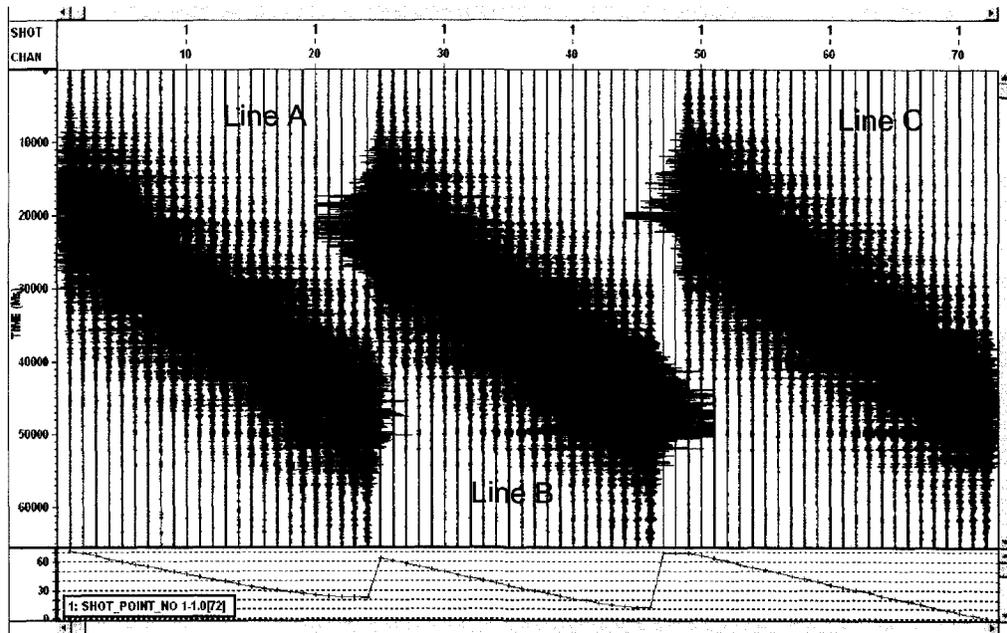
Figure 27: Passive data shot gather for a single run of truck
