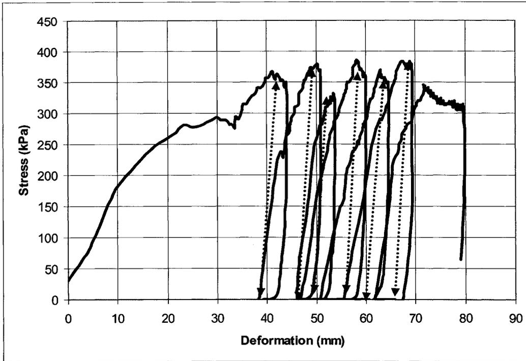
Figure 92: Stress-deformation curve for a cyclic test, showing unload-reload cycles
