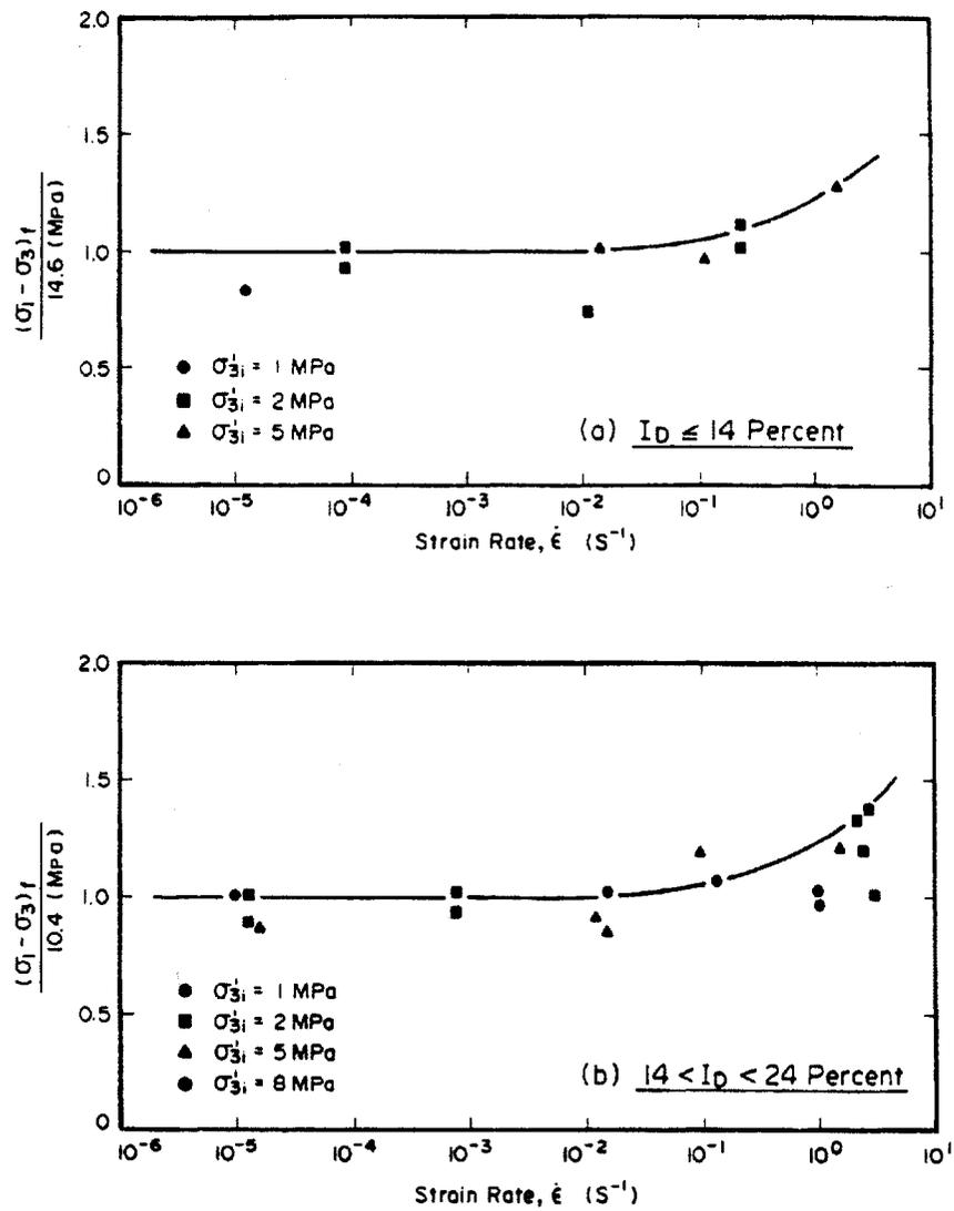
Figure 59: Effect of strain rate on ultimate strain undrained (after Plewes 1987)
