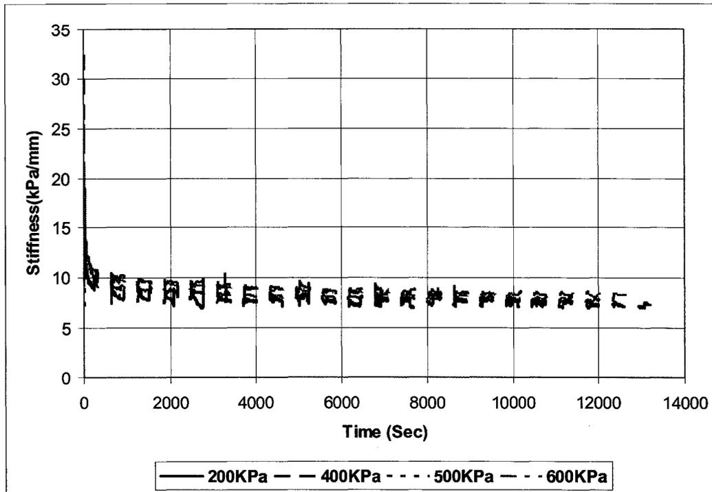
Figure 133: Pressure stiffness vs. time for 5-min. tests
