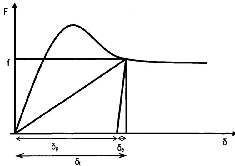
Figure 75: Total deformation in load-deformation curve
