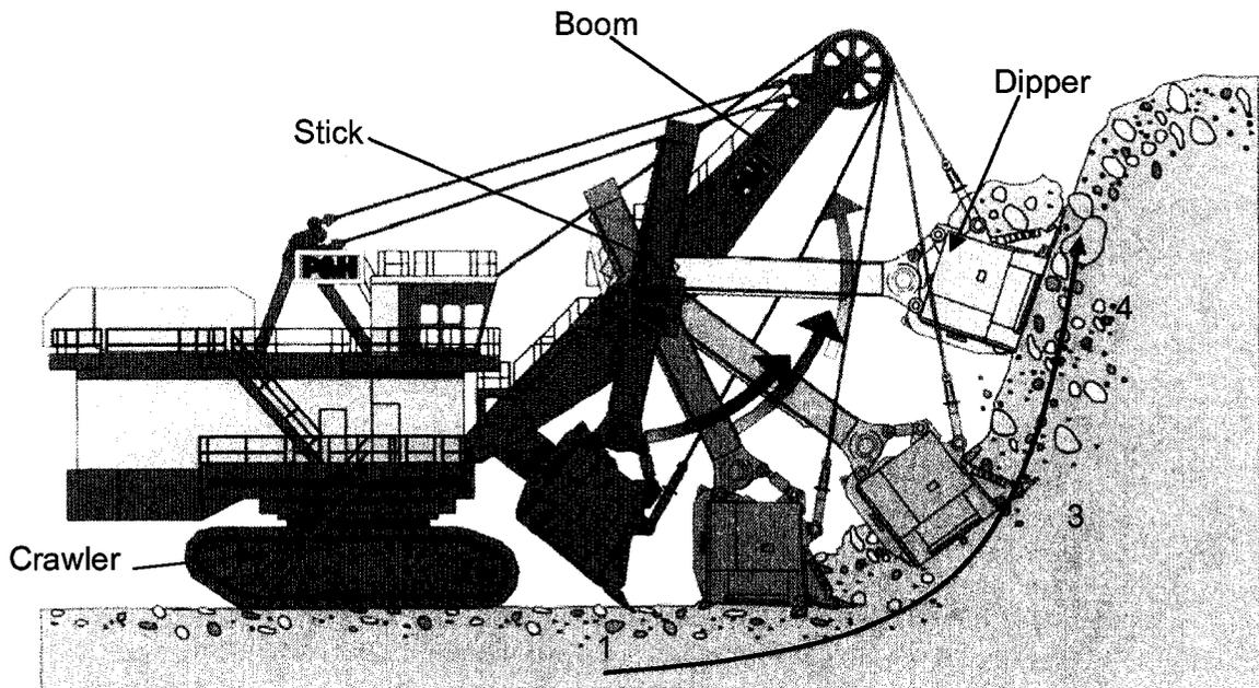
Figure 157: Different parts of the P&H 4100 BOSS shovel (after Harnischfeger 2001)
