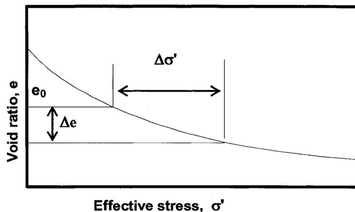
Figure 53: The coefficient of compressibility (after Craig 1996)
