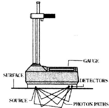
Figure 112: Two different methods for measuring density with a Troxler (after Evett 2000)
