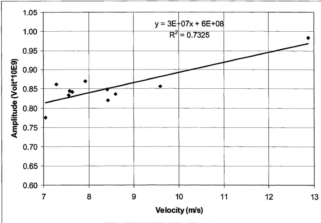
Figure 37: Sum of amplitude vs. truck velocity (loaded truck on day 1)
