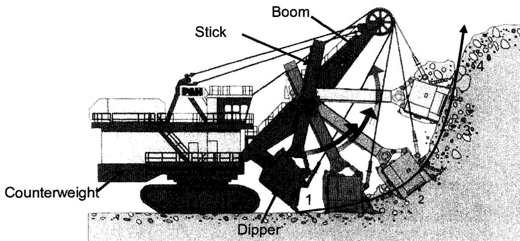
Figure 3: Excavating action (after Harnischfeger 2001)
