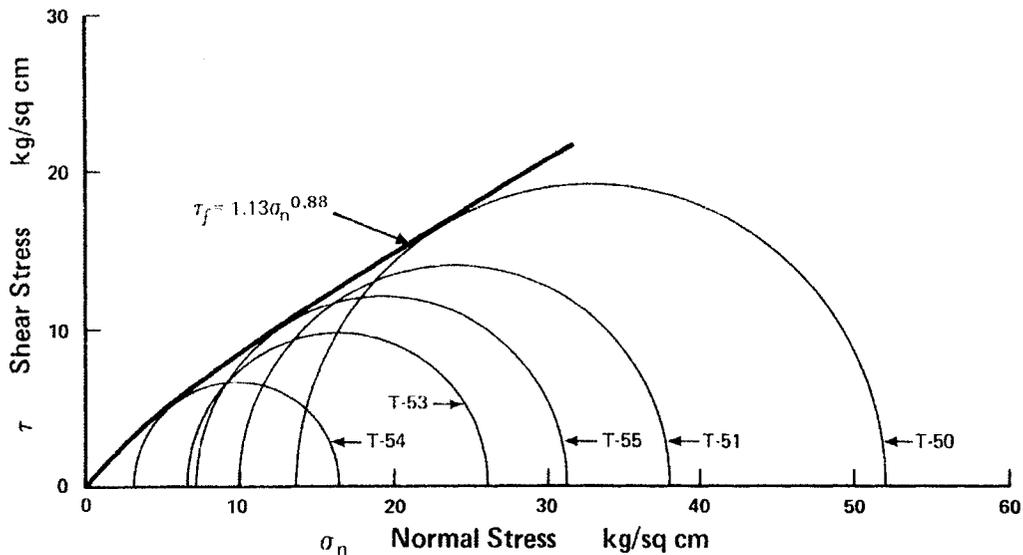
Figure 55: Failure envelope of re-compacted rich oil sand undrained triaxial tests (from Dusseault 1977)
