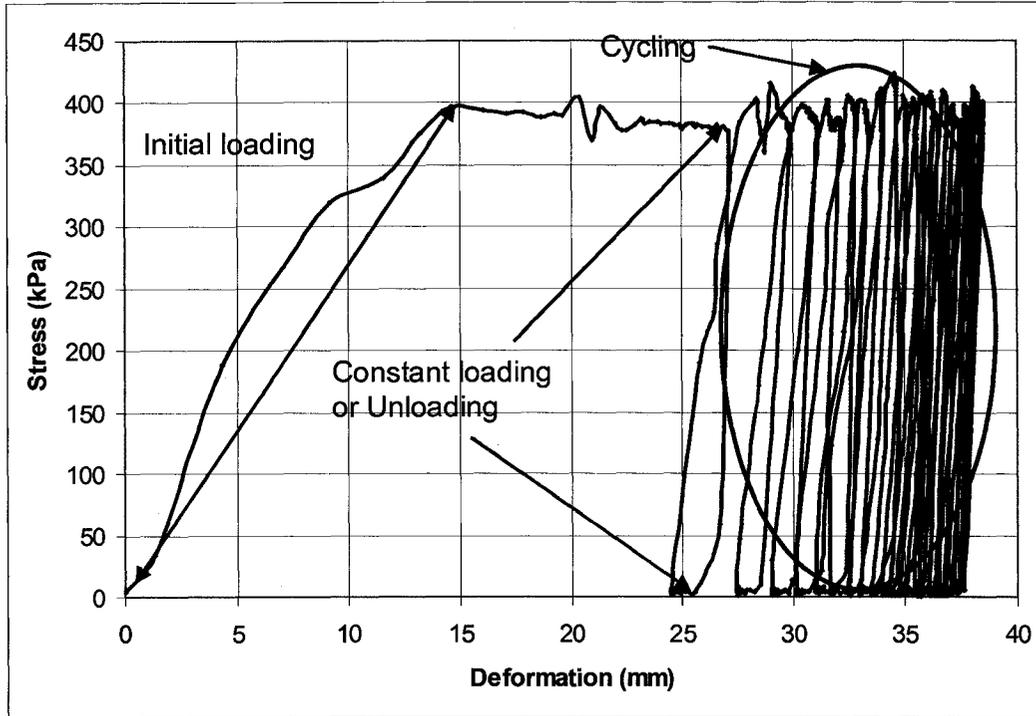
Figure 130: General stress-deformation curve for plate load test
