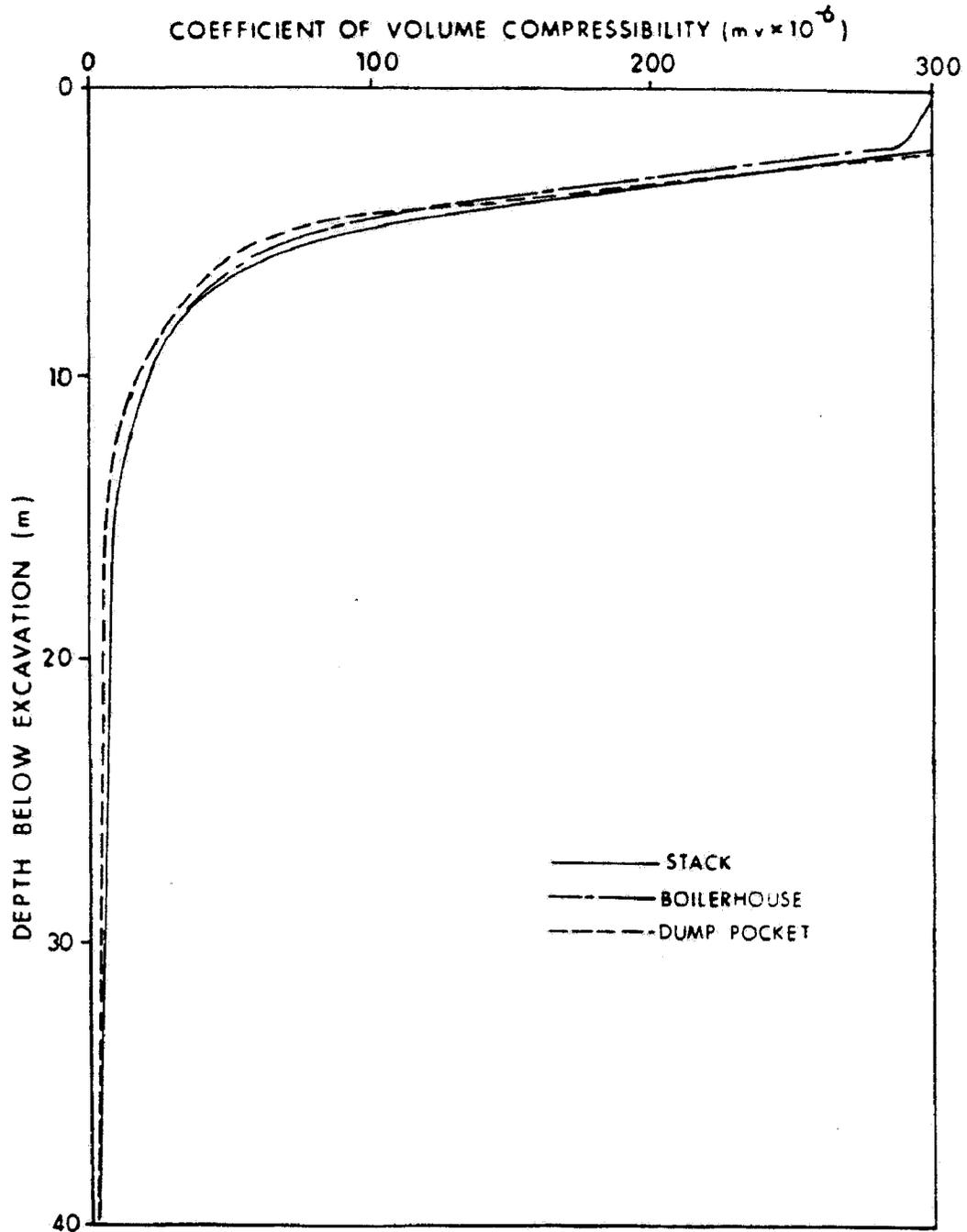
Figure 62: Disturbance of  $m_v$  with depth (after Griffin 1986)
