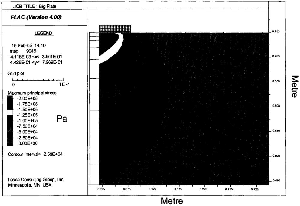
Figure 98: Vertical stress under large plate
