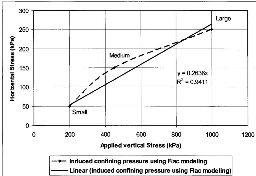
Figure 104: Induced confining pressure by FLAC modeling for different plate size
