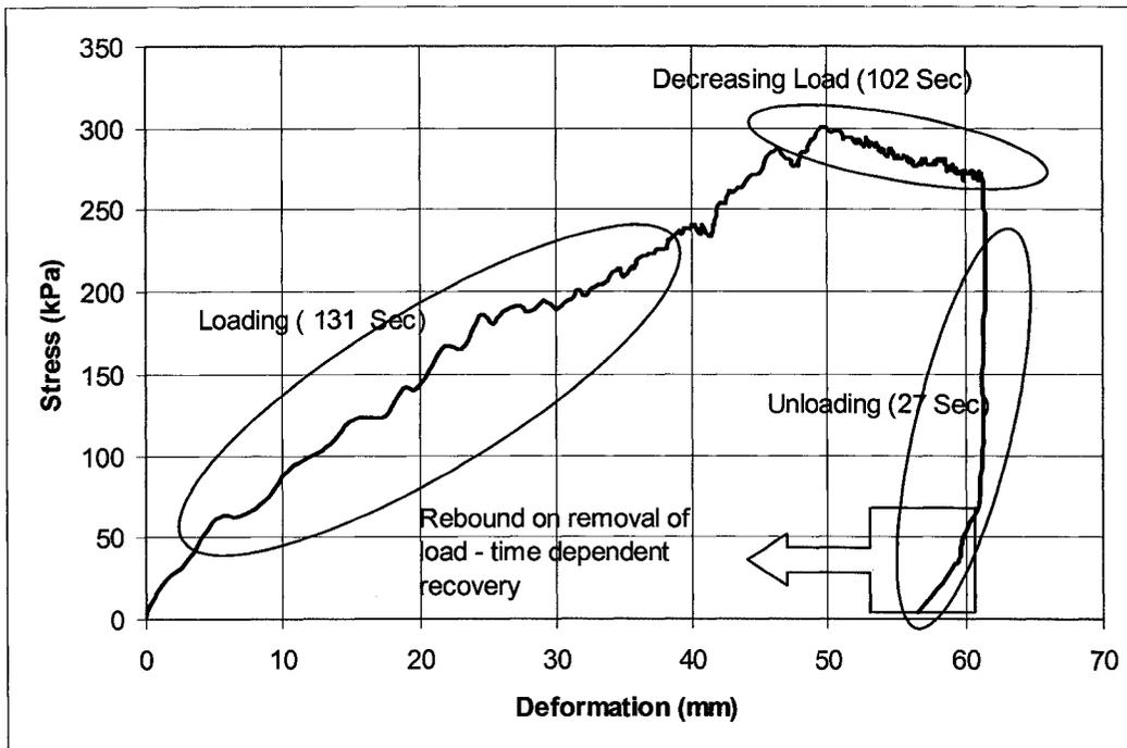
Figure 89: Stages of a cyclic plate load test
