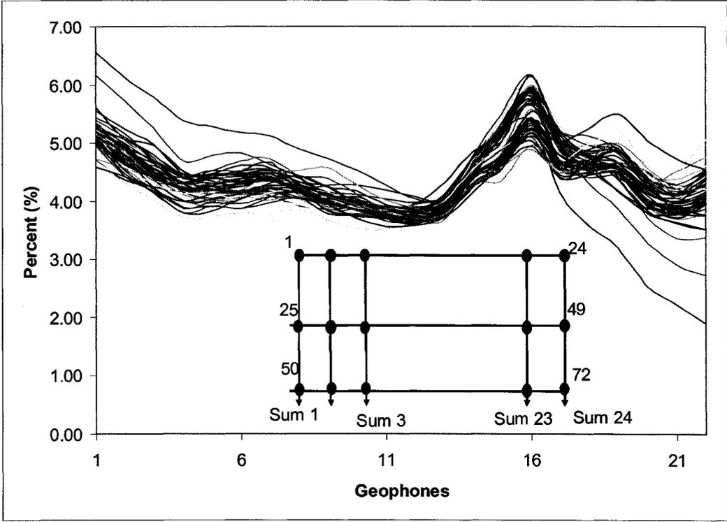
Figure 33: Comparing the amplitude normalization for different runs
