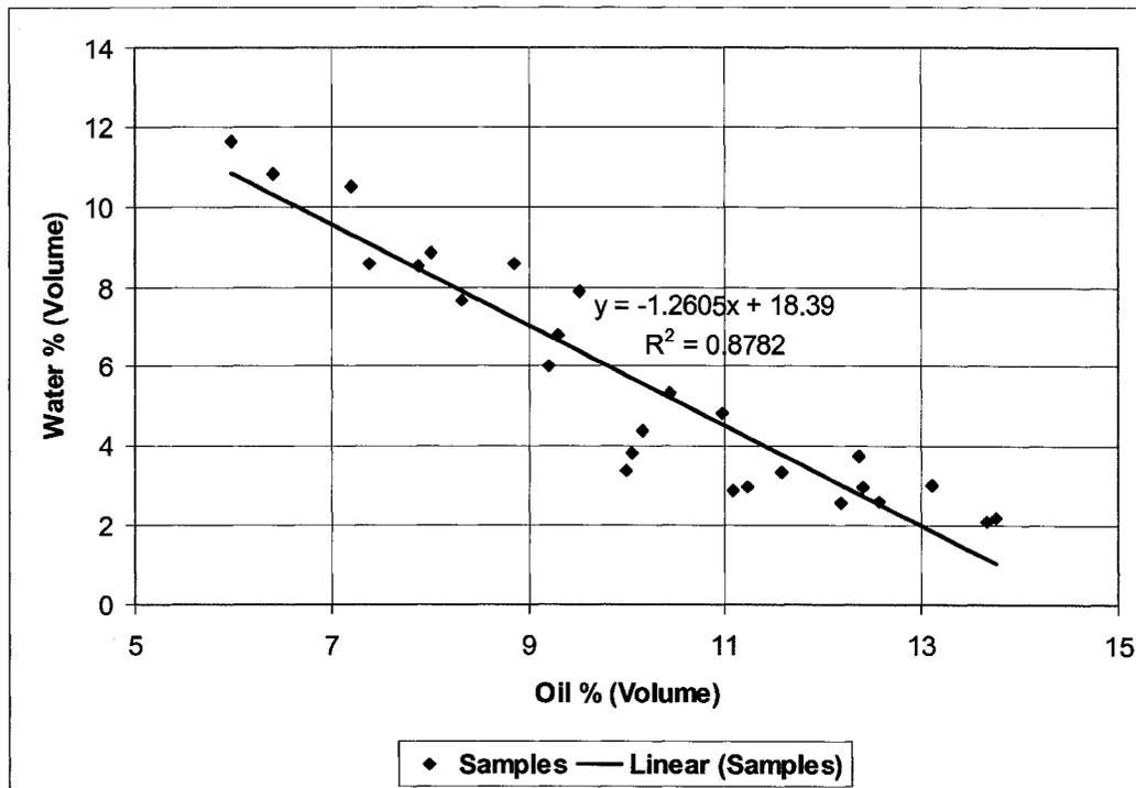
Figure 119: Relationship between oil and water content in oil sand pit
