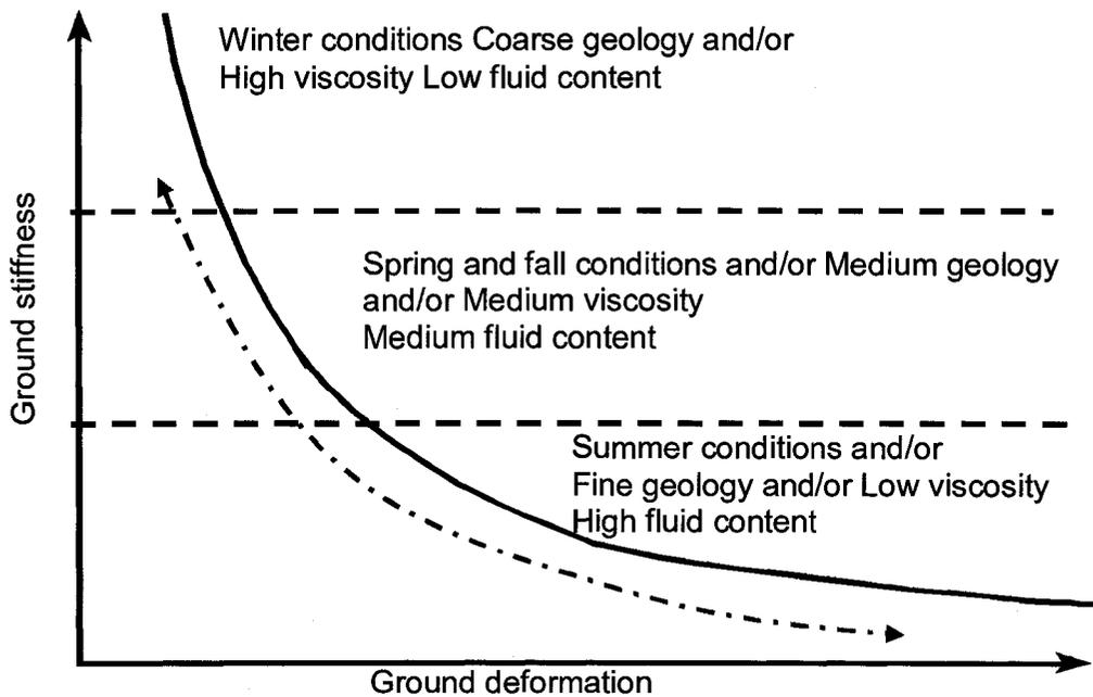
Figure 1: Stiffness of oil sand in different seasons (after Joseph et al. 2003)
