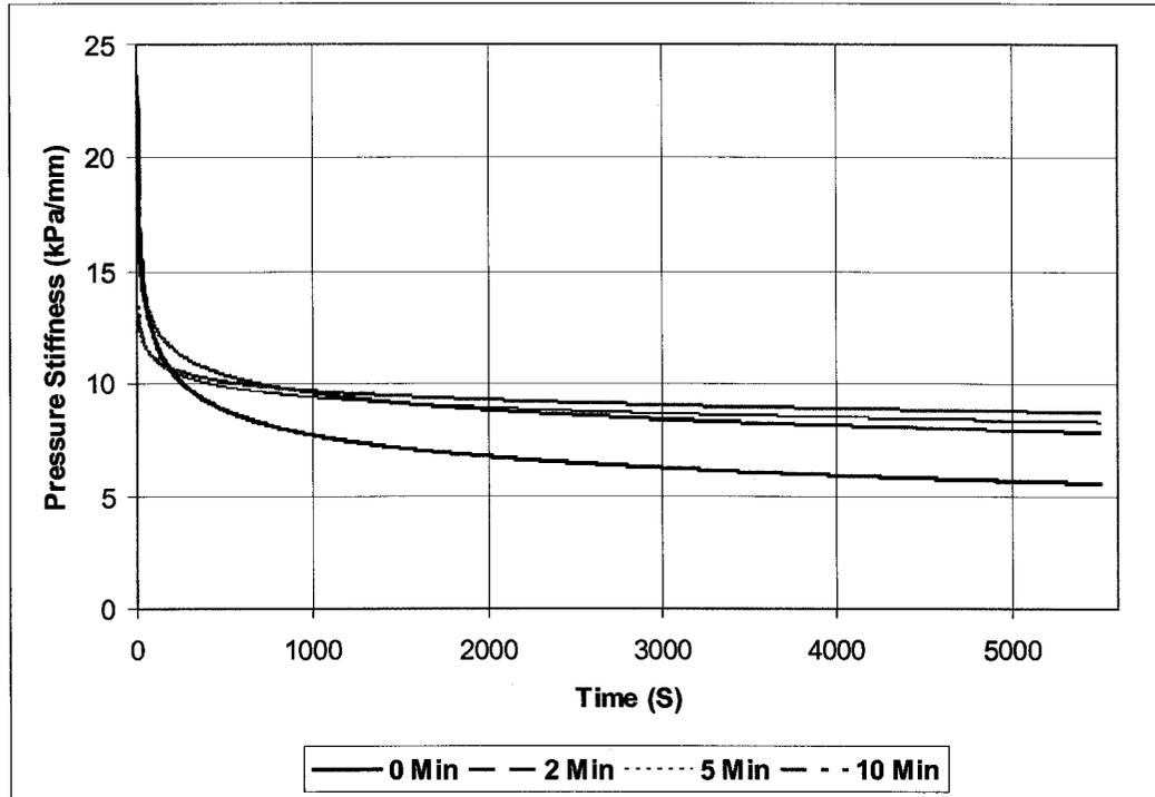
Figure 143: Pressure stiffness for different duration cycles based on averaging curve fit
