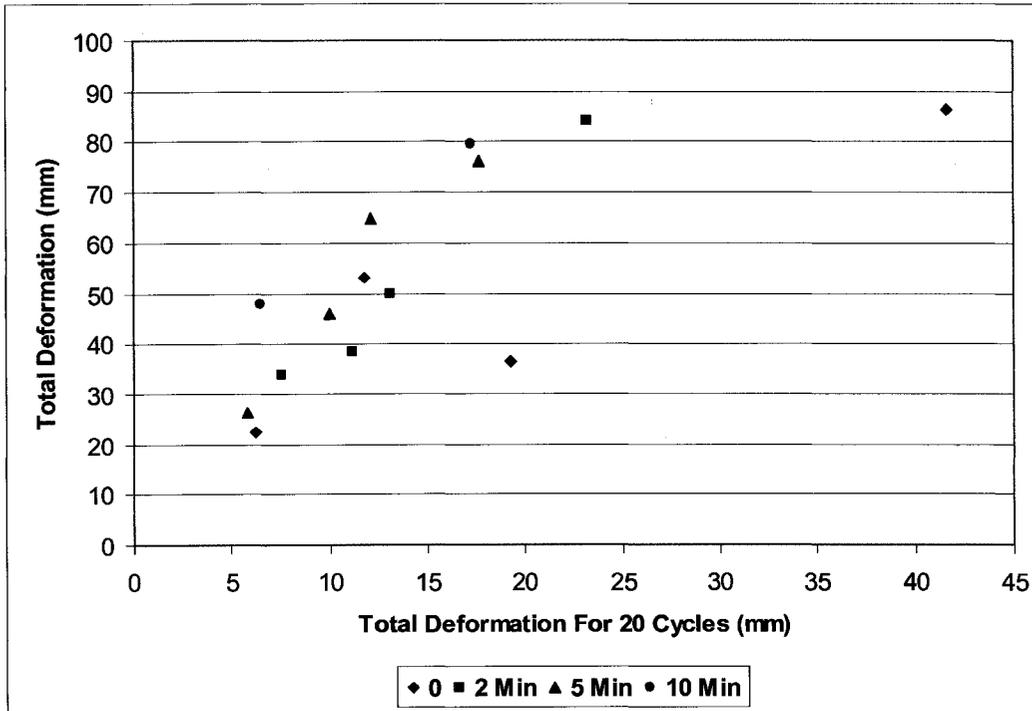
Figure 141: Total deformation versus deformation in 20 cycles for 0-10 min.
