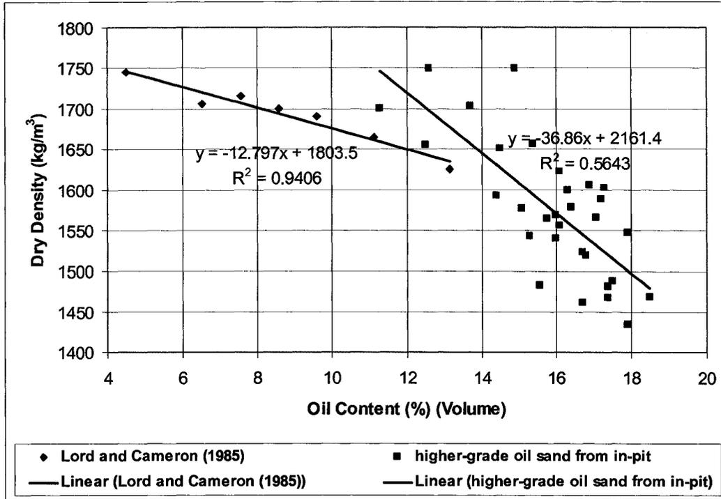
Figure 116: Analysis of compaction data by using results reported by Lord and Cameron (1985) and higher-grade oil sand from in-pit
