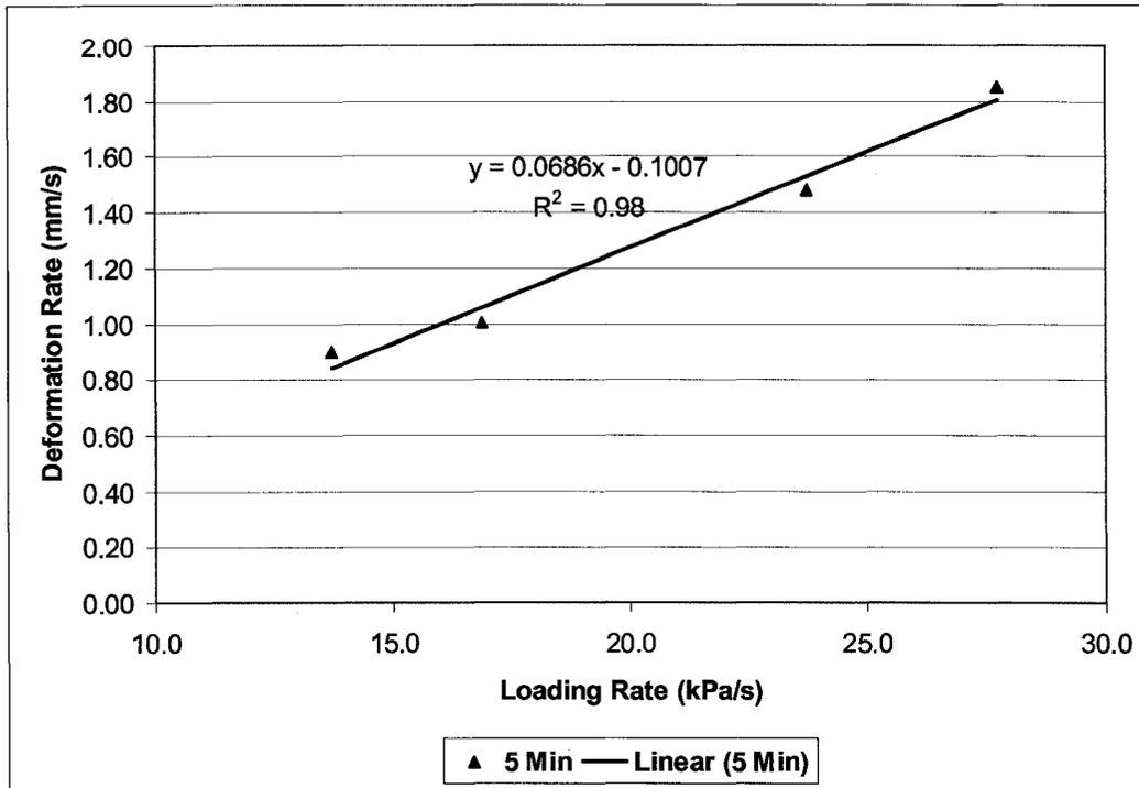
Figure 137: Loading rate and deformation rate for 5 Min test
