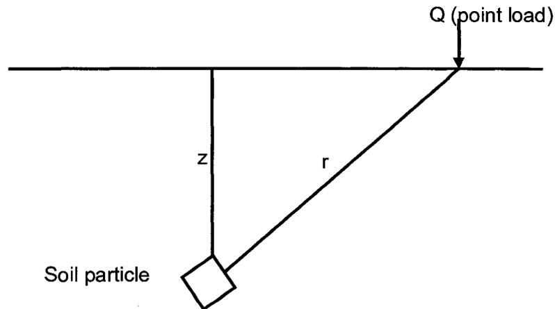
Figure 106: Load and distances from surface to soil particles
