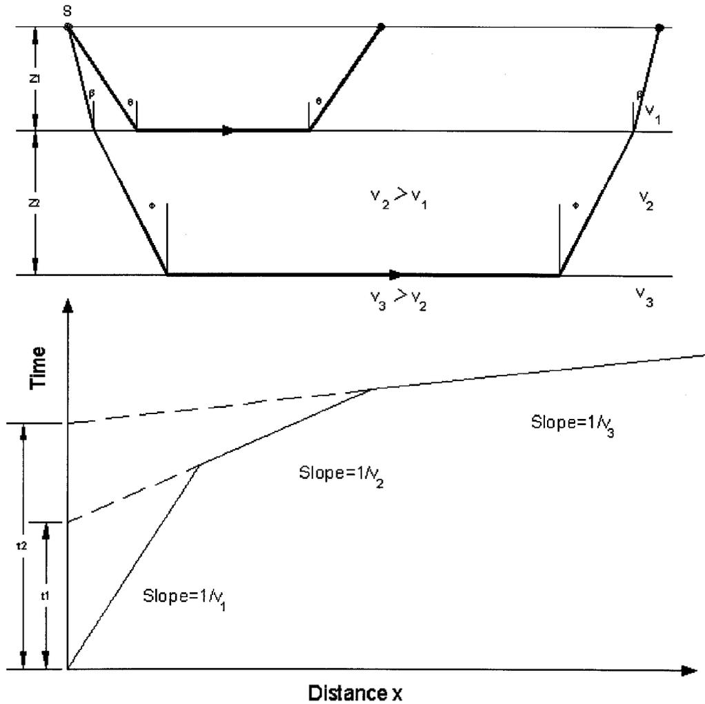
Figure 20: Refraction from two layers (after Tezkan 1998)
