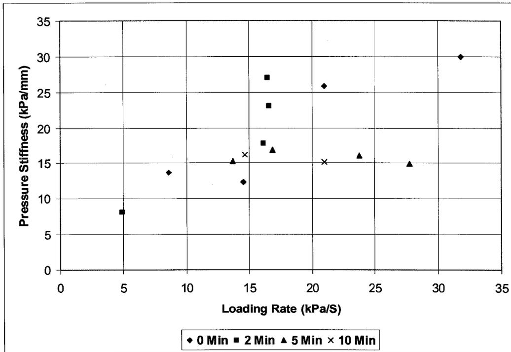
Figure 136: Loading rate vs. pressure stiffness for initial loading
