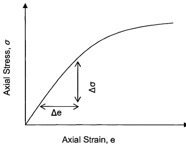
Figure 54: Modulus of deformation (after Craig 1996)
