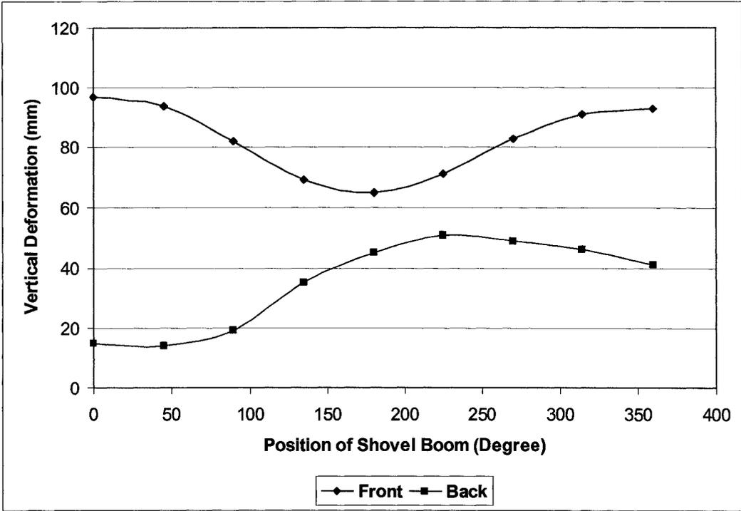
Figure 172: Changing the absolute deformation value during the static loading test
