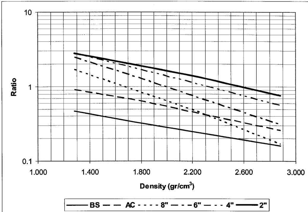
Figure 113: Density calibration curve for MC-1 densitometer
