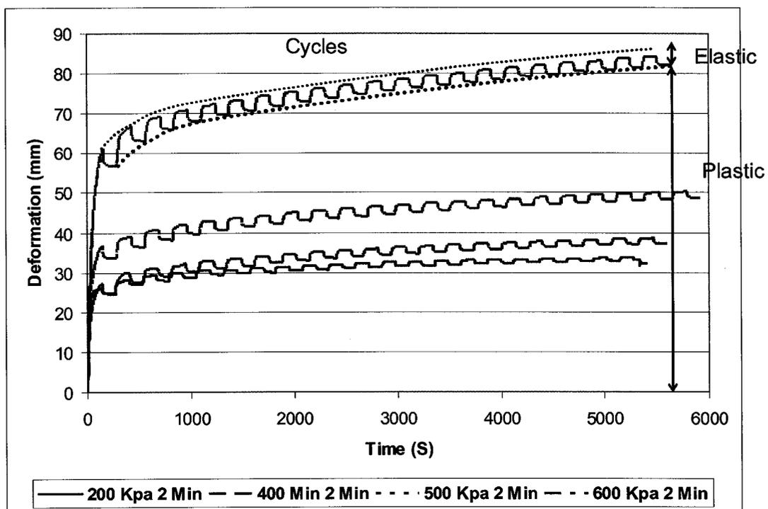
Figure 139: Time deformation curve for loading and unloading at different stresses for 2 min duration test
