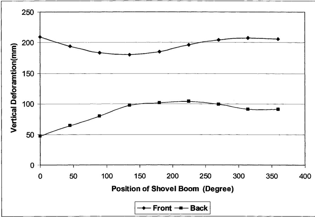
Figure 173: Changing the absolute deformation value during the static loading test (end of day)
