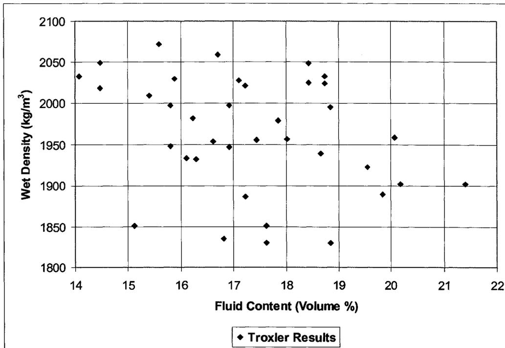
Figure 117: Troxler wet bulk density results vs. fluid content
