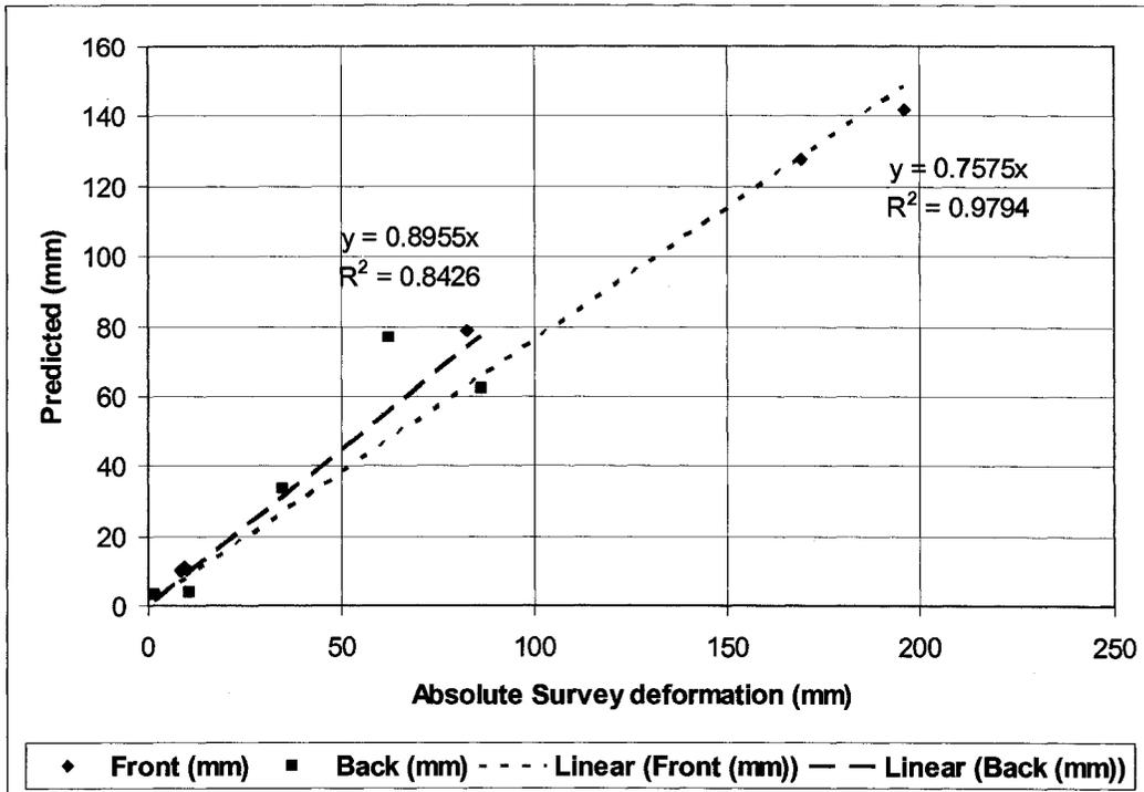
Figure 170: Absolute deformation from survey and prediction deformation
