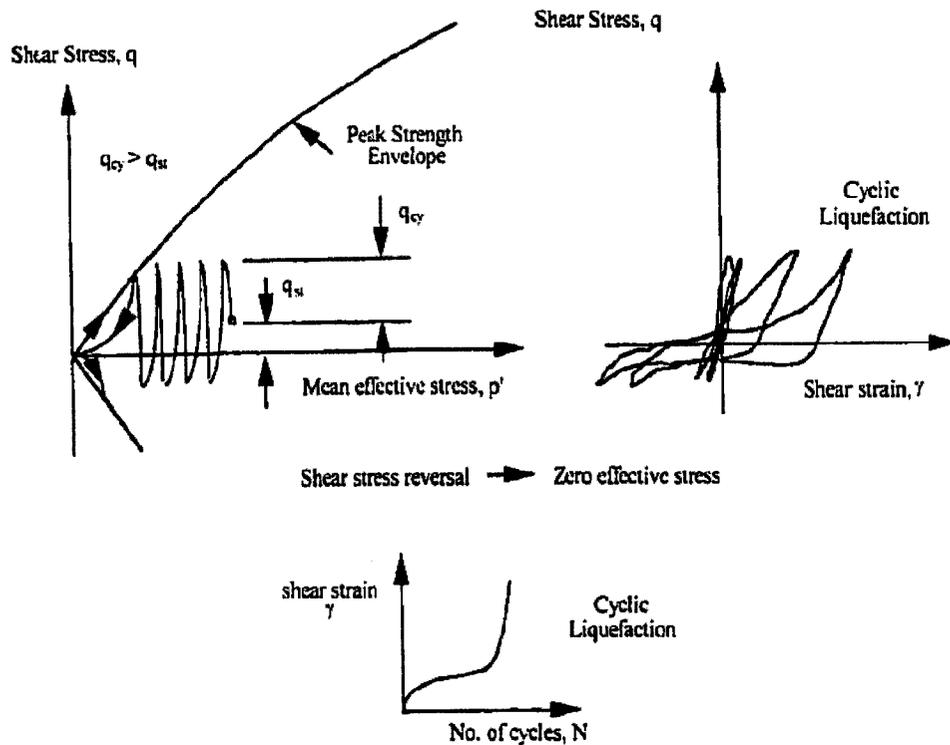
Figure 69: Schematic illustration of cyclic liquefaction (after Grozic, 1999)
