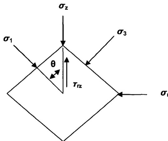
Figure 105: Principal, horizontal and vertical stresses on an element
