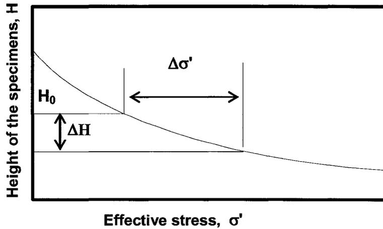
Figure 52: The coefficient of volume compressibility (after Craig 1996)
