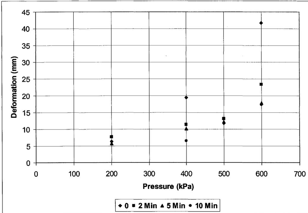
Figure 140: Total deformation at different pressure during 20 cycles
