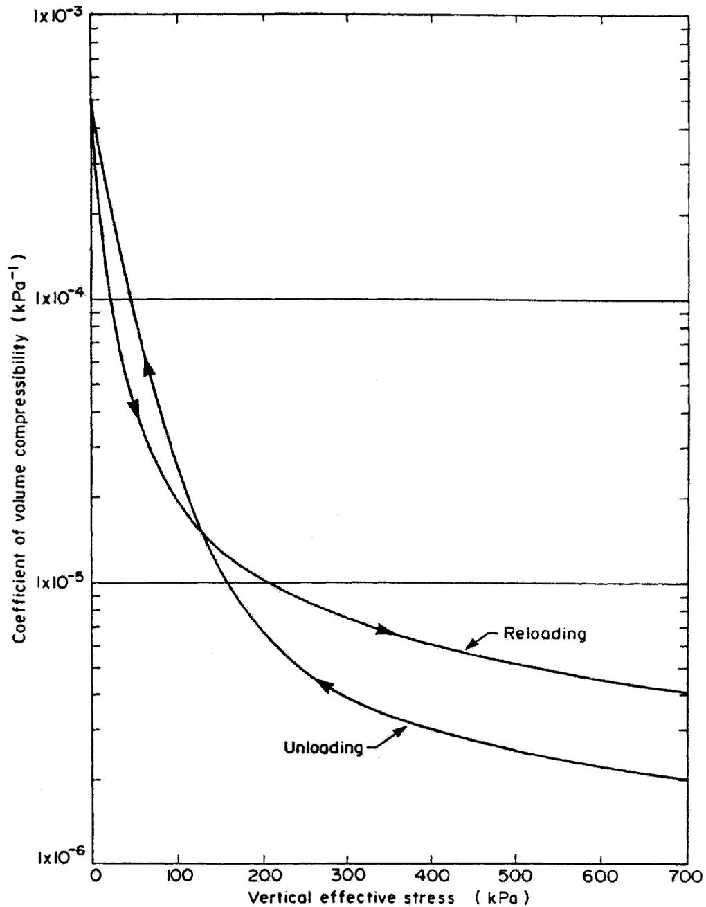
Figure 63: Compressibility of oil sand at different vertical effective stress (after Griffin 1986)
