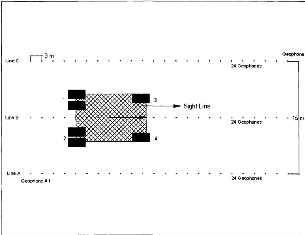
Figure 26: Test set-up for passive winter data acquisition
