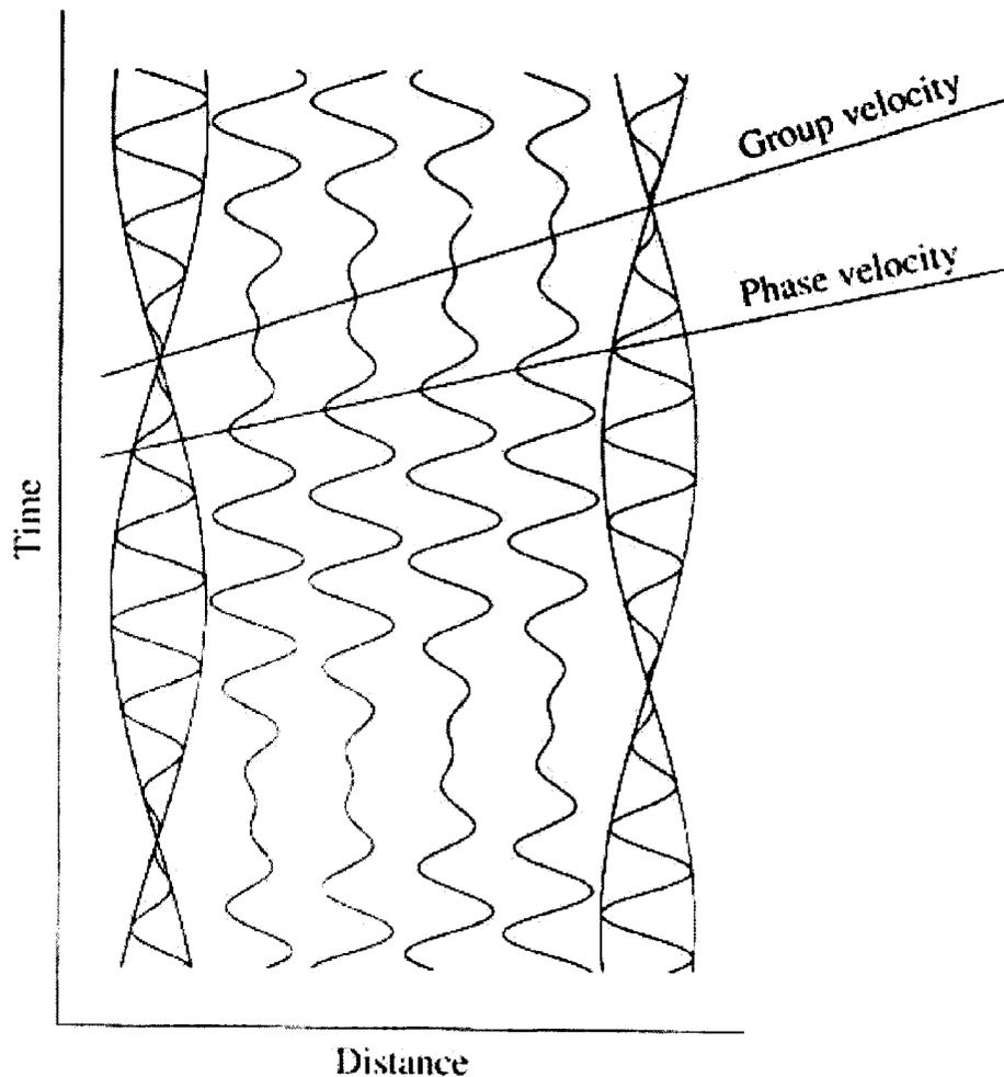
Figure 46: Phase and group velocity (from Shearer 1999)
