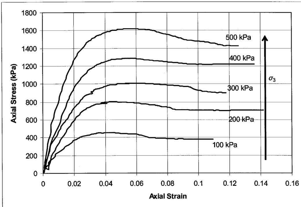
Figure 79: Stress-strain curve for 11% bitumen
