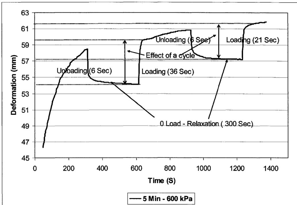
Figure 153: Effect of two cycles on the deformation for 600 kPa and 5 Min test
