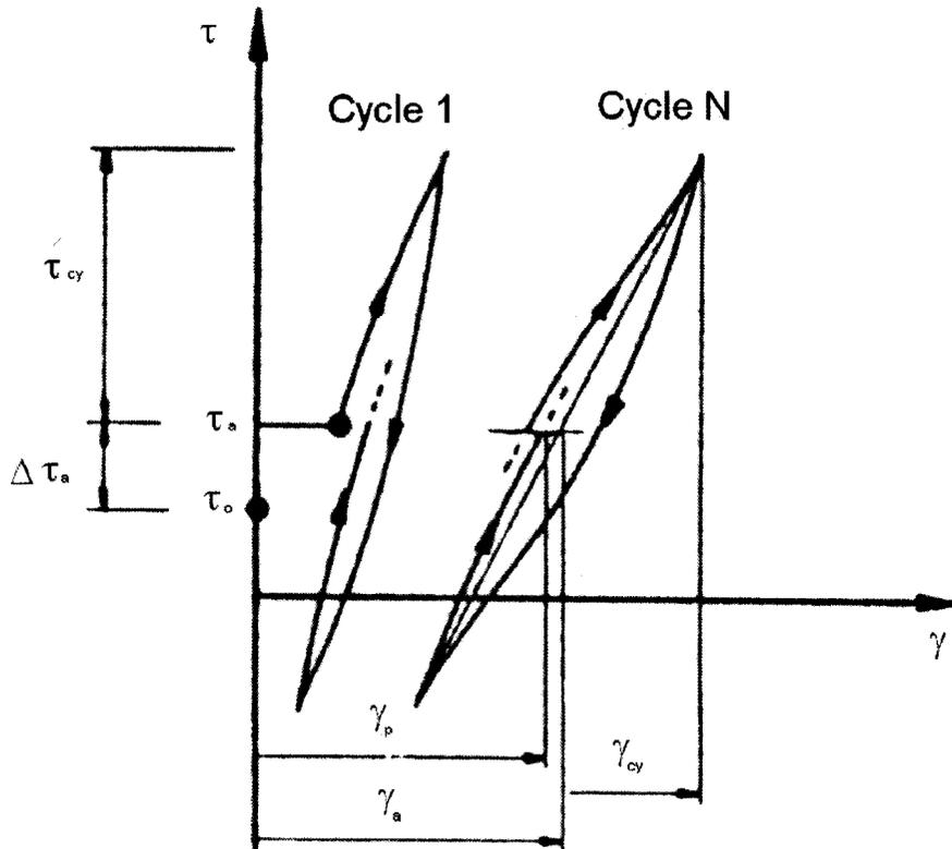
Figure 65: Shear stress and strain behaviour during cyclic loading (after Anderson, 1988)
