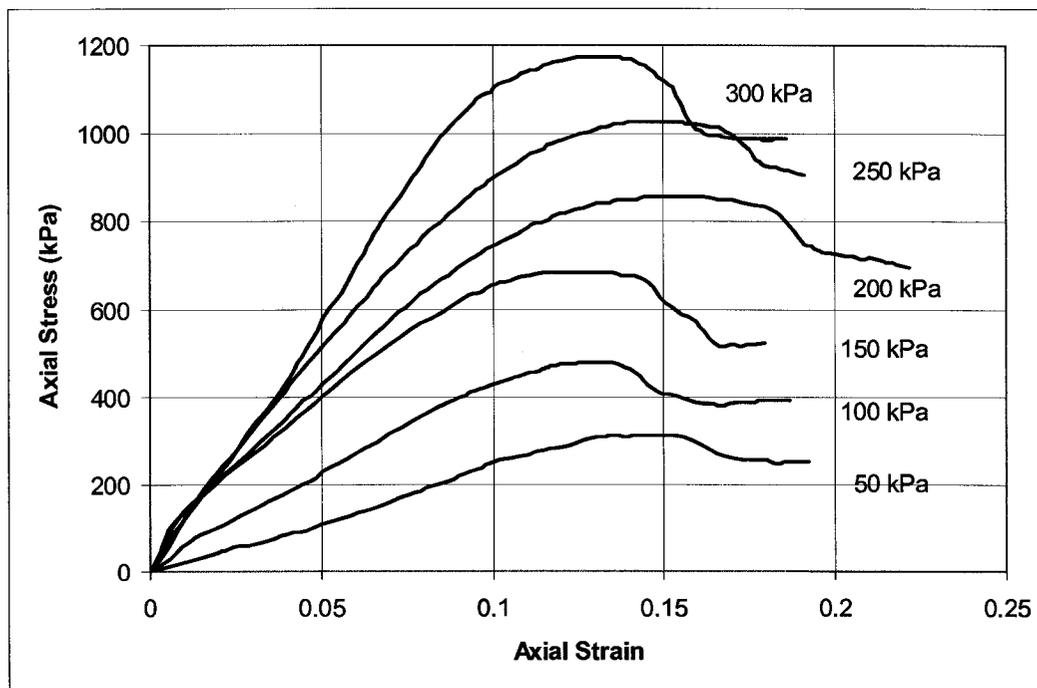
Figure 77: Stress- strain curve for 8% bitumen at room temperature
