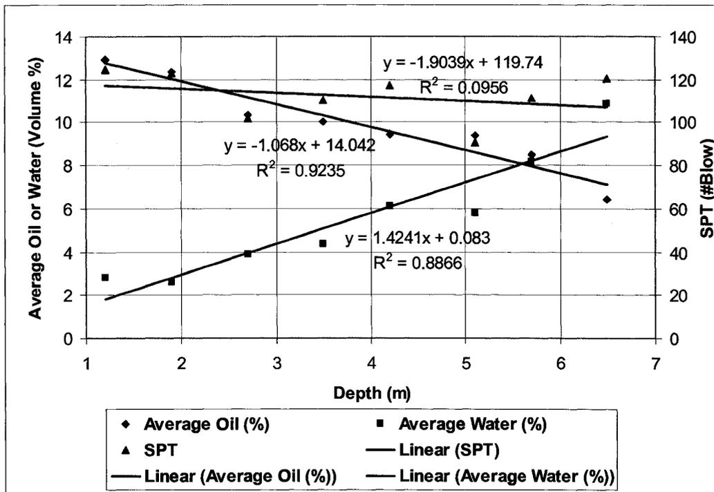
Figure 115: Data from a 7 m profile measuring SPT blow count and fluid content (Joseph, 2001)
