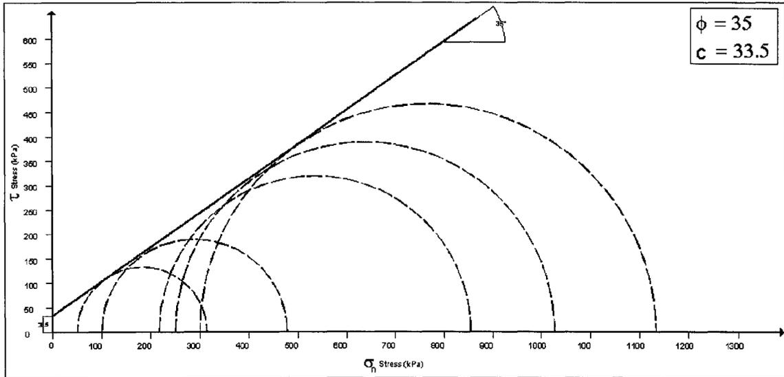
Figure 85: Mohr-Coulomb envelope for 8% oil sand
