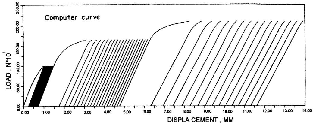
Figure 68: Cyclic plate 50mm bearing test (after Butterfield 1980)
