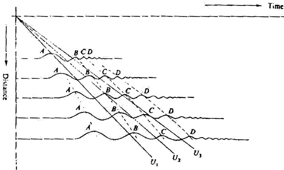
Figure 47: Dispersion of waveform (from Shearer 1999)
