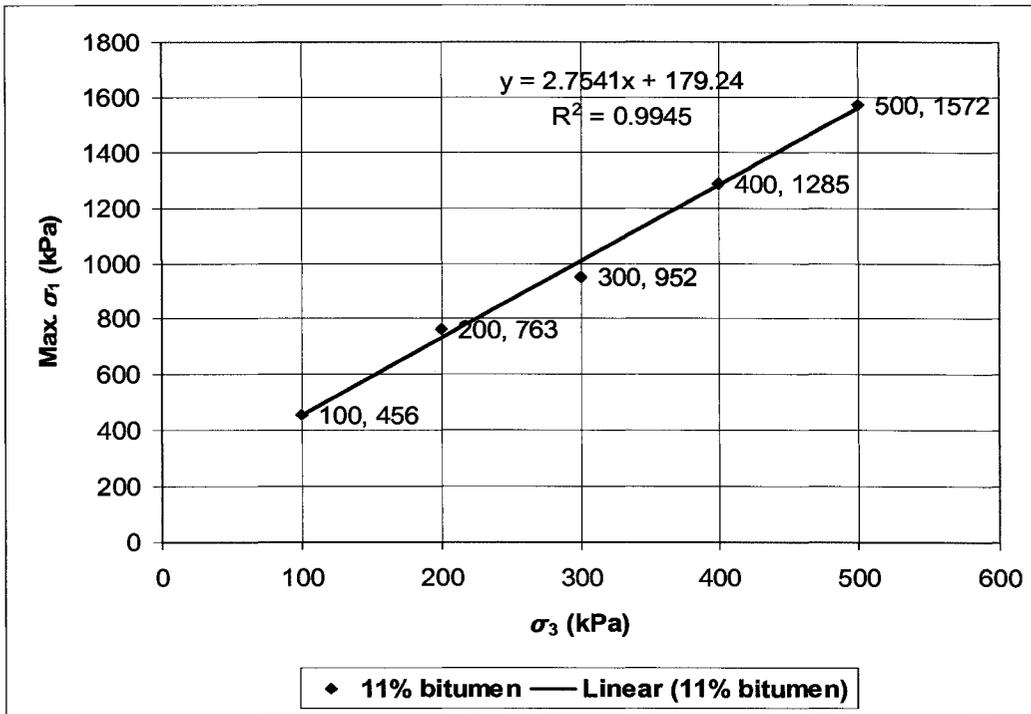
Figure 80: Linear relationship for 11 % bitumen between  $\sigma_1$  and  $\sigma_3$
