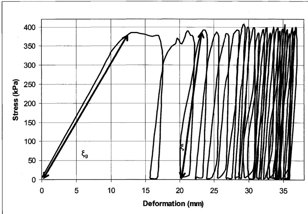
Figure 129: Global and local slope (stiffness)
