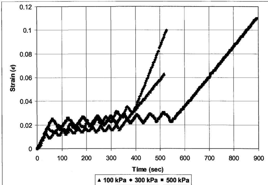
Figure 84: Time - Strain curve for triaxial cyclic loading
