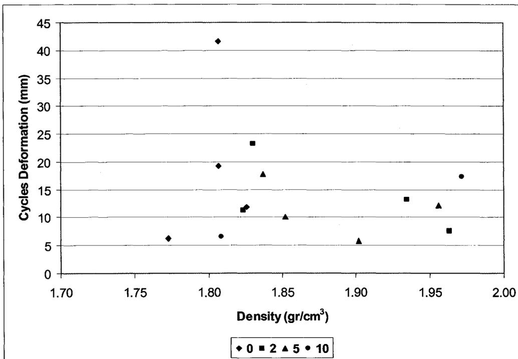
Figure 147: Initial density vs. total cyclic deformation
