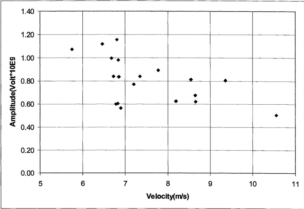
Figure 43: Loaded truck velocity vs. sum of geophones amplitude for day 3
