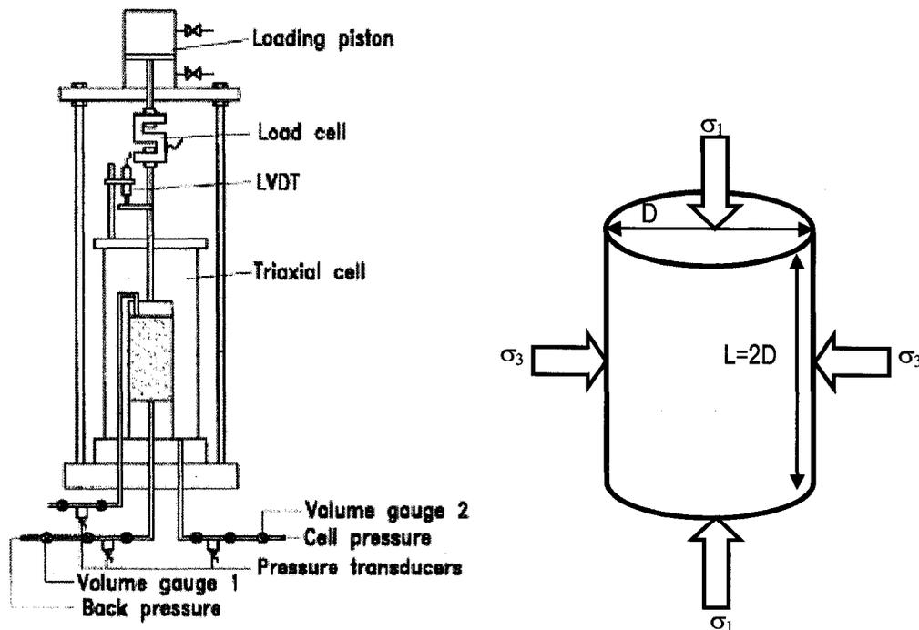
Figure 76: Schematic of triaxial test and principal stresses
