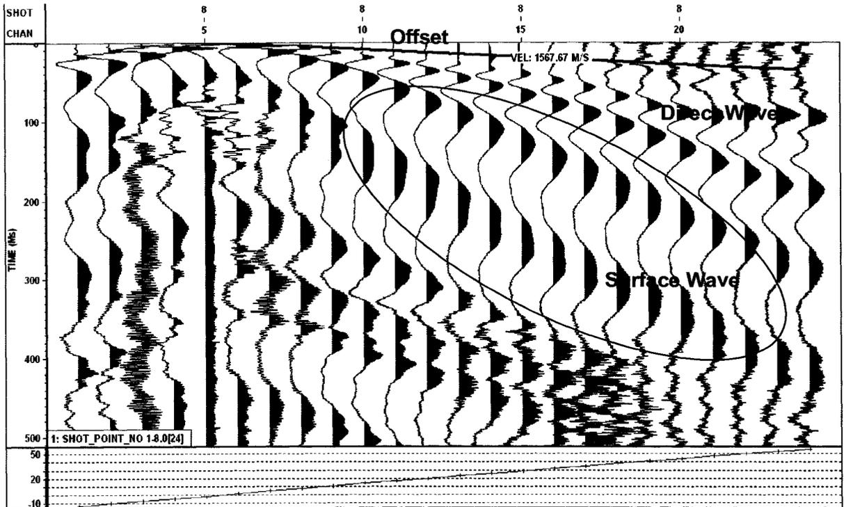
Figure 25: Winter surface and refraction data
