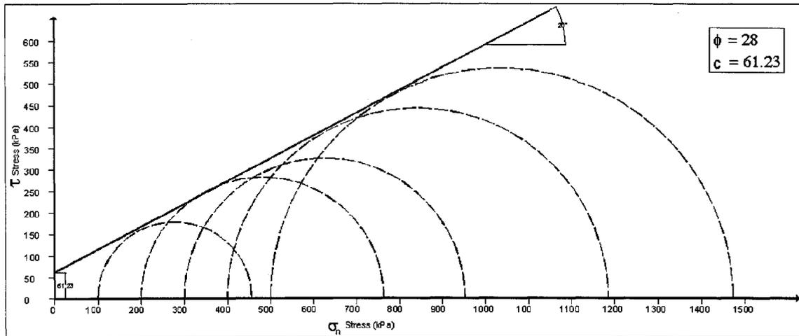
Figure 86: Mohr-Coulomb envelope for 11% oil sand
