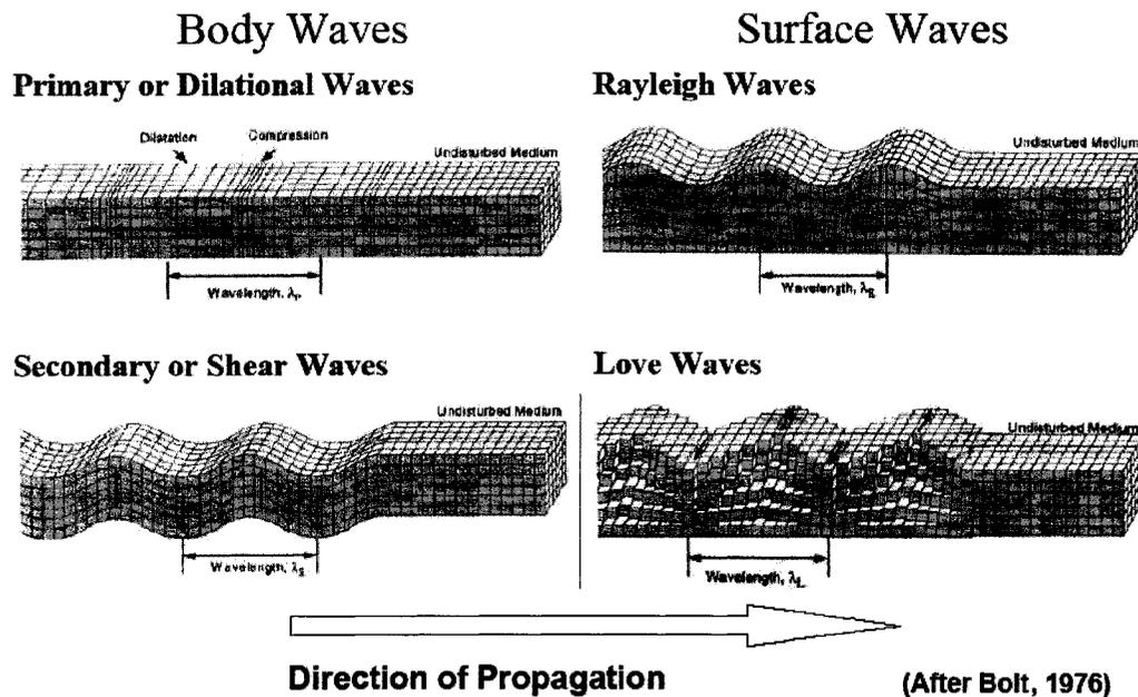
Figure 45: Particle motion of P, S, Love and Rayleigh waves (from Shearer 1999)
