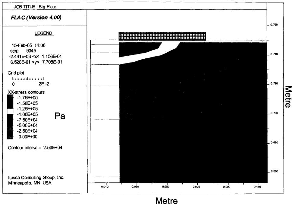
Figure 99: Horizontal stress under large plate
