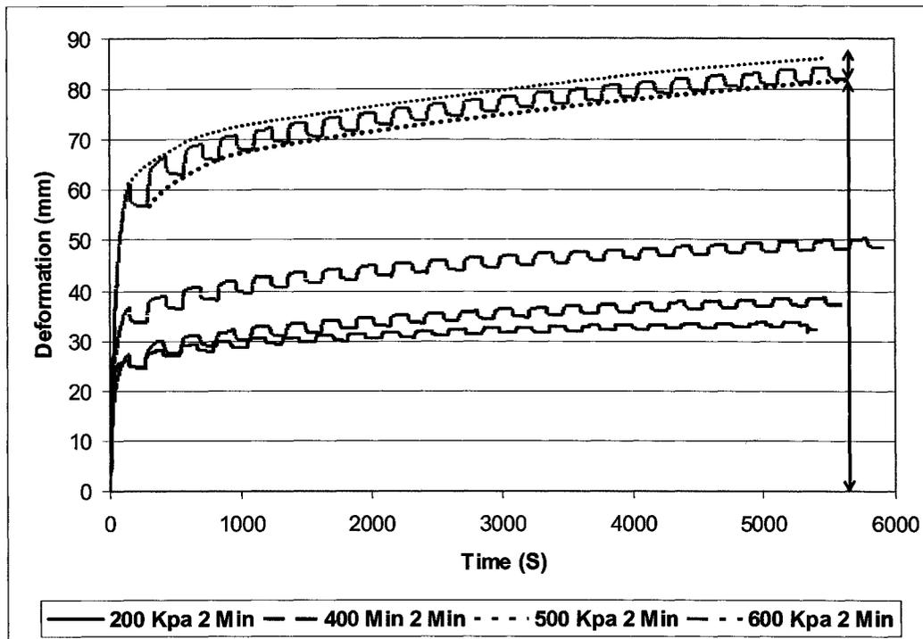
Figure 126: Time deformation results at different stresses for 2-min. duration
