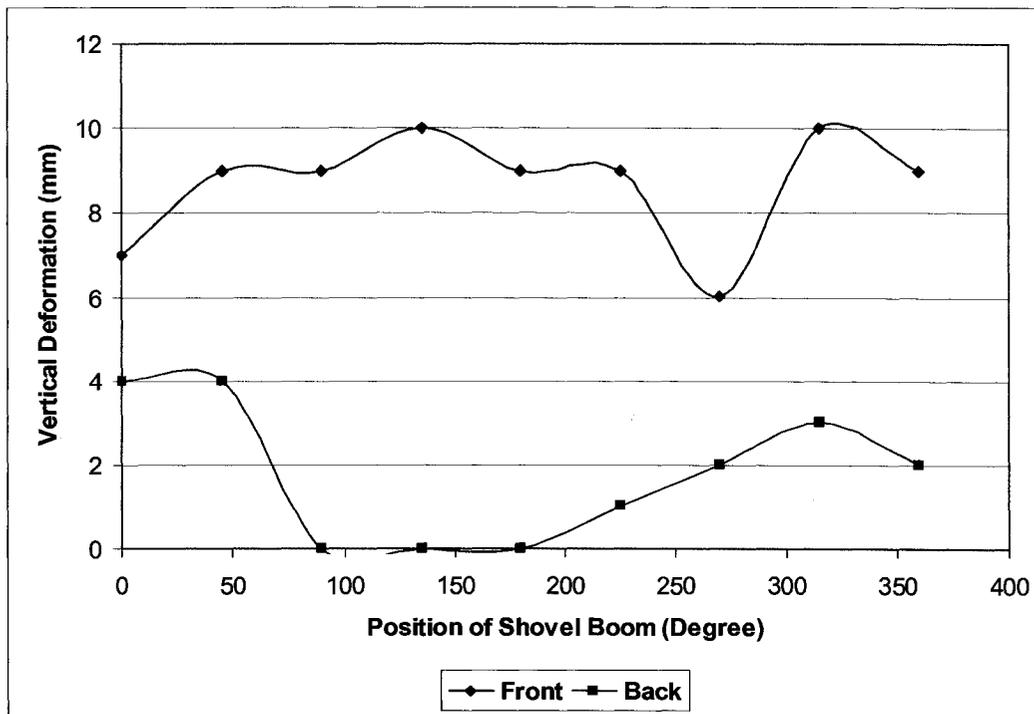
Figure 171: Changing the absolute deformation value during empty-shovel's rotation
