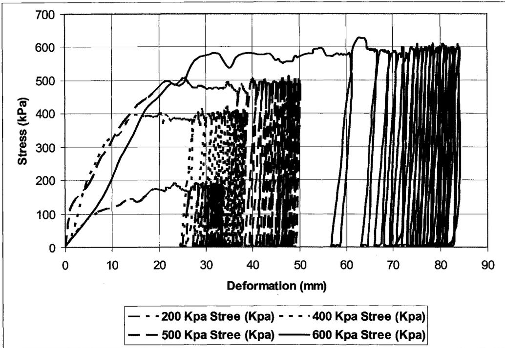
Figure 125: Plate load test results at different stresses for 2-min. loading time
