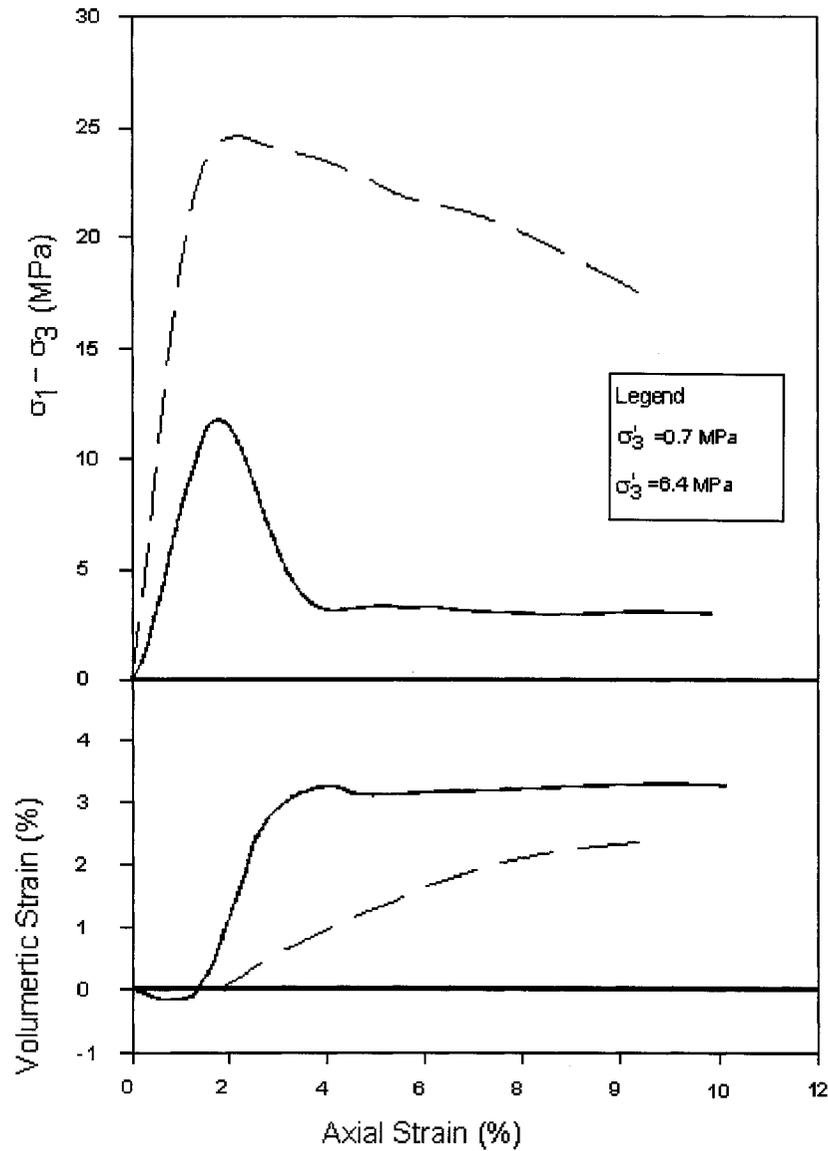
Figure 56: Typical drained stress strain curve for oil sand (from Plewes 1987)
