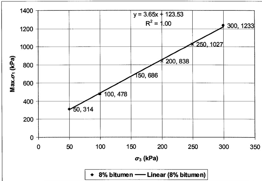
Figure 78: Linear relationship between  $\sigma_1$  and  $\sigma_3$
