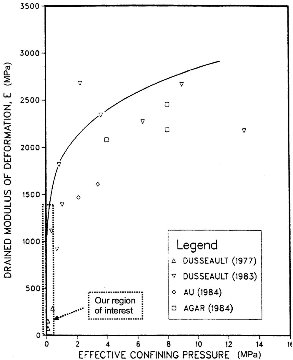
Figure 57: Deformation modulus for oil sand in drained triaxial testing (after Plewes 1987)
