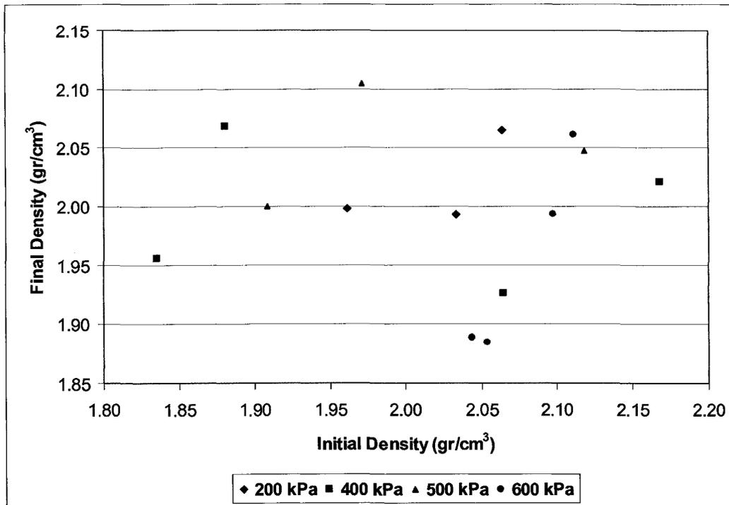
Figure 148: Initial density vs. final density
