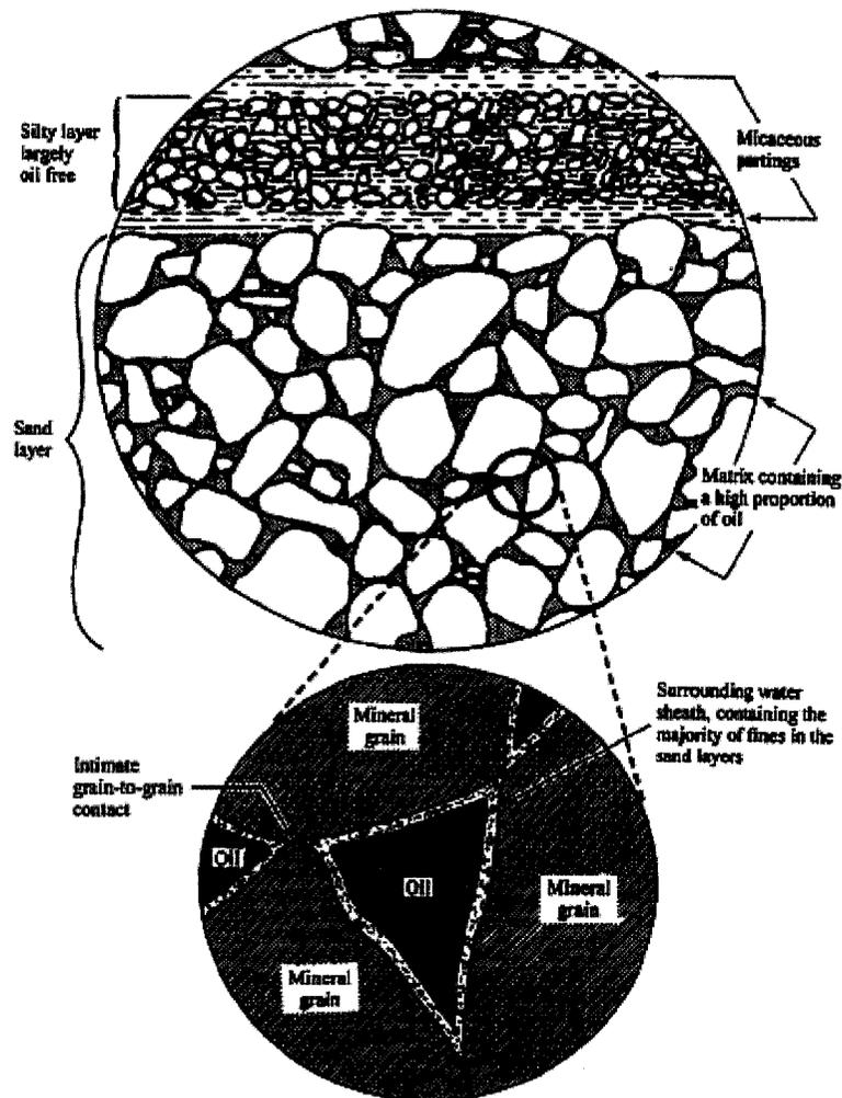
Figure 16: In situ structure of oil sands (from Dusseault 1977 & Grant 1980)
