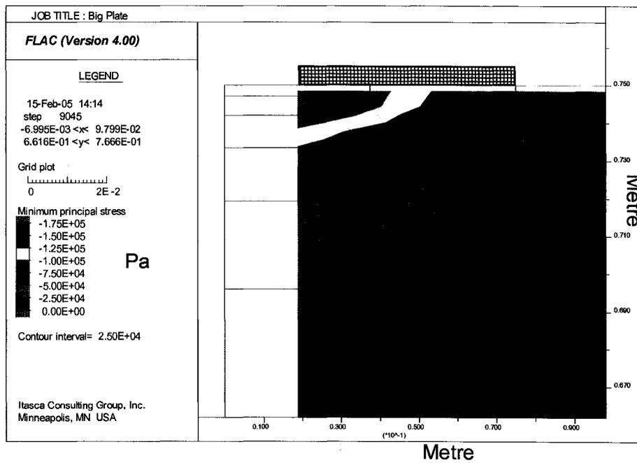
Figure 101: Confining pressure  $\sigma_3$  under large plate
