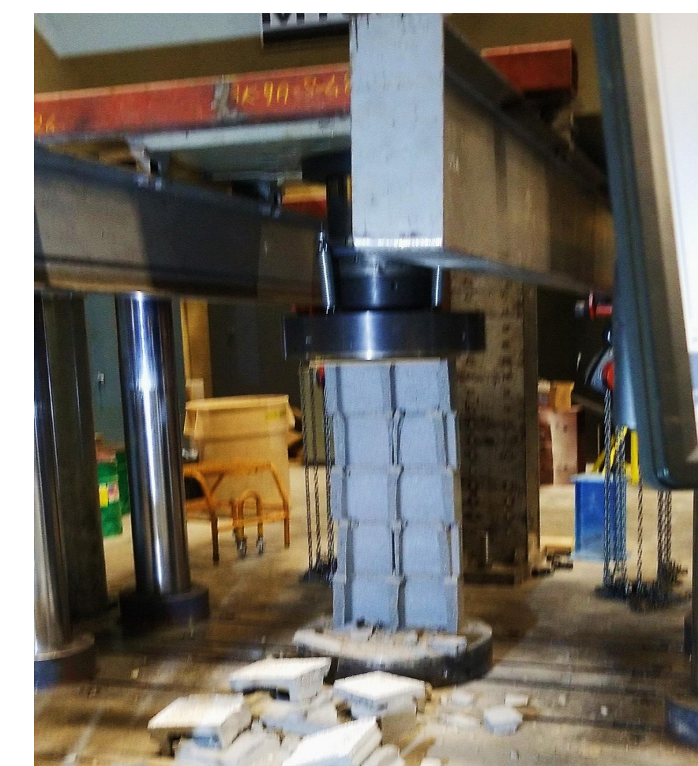
Figure 6. UngROUTED masonry wall cracked completely in half
