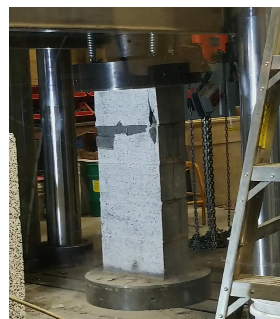
Figure 5. Grouted masonry prism cracked after experiencing intense lateral loads
