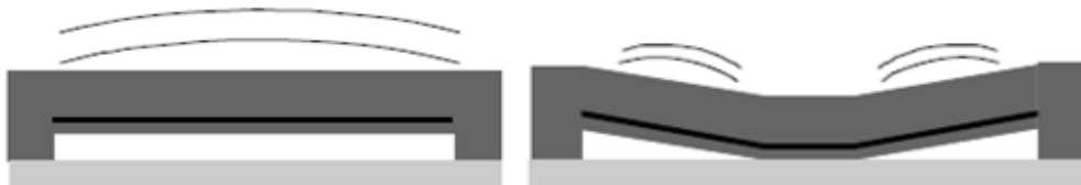
Figure 4.5: Operation of a CMUT in pre-collapse mode on the left, and collapse mode on the right [48] © 2009 IEEE
