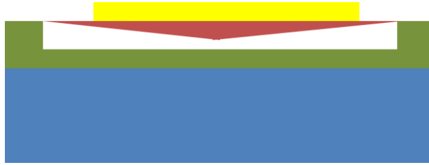
Figure 4.8: Diagram depicting the consequence of poor etch selectivity during sacrificial layer etch
