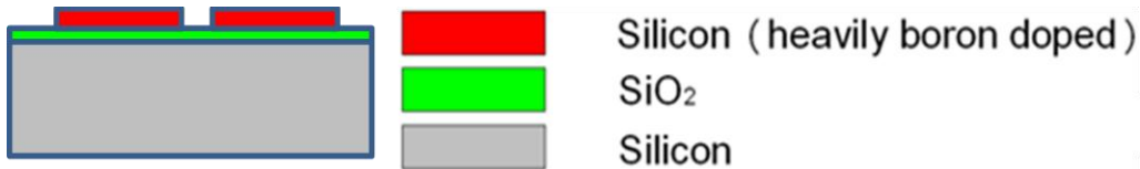
Figure 4.10: SOI wafer with trenches etched into silicon device layer. The silicon device layer is heavily doped to act as a bottom electrode
