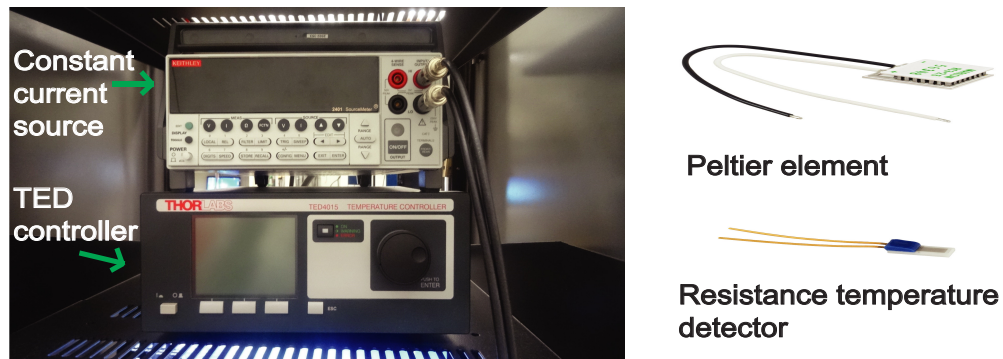
Figure 4.4: Left-top is the constant current source (Keithley-2401) and bottom one is thermoelectric temperature controller. Right top is the Peltier element and bottom one is the resistance temperature detector (PT-1000). The figures of Peltier element and resistance temperature detector are taken from thorlabs website.
