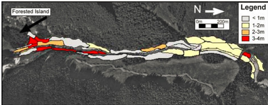
Figure 7-27: Thickness of deposition along the path of ZRRA from the forested island to the start of the canyon (Boulton et al. 2006)
