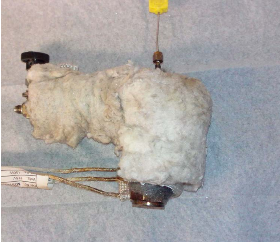
Figure 5.3: Wrapping the insulation material over the heating tape.
