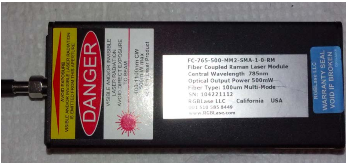
Figure 4.9: Top view of the fiber coupled 785nm Raman Laser Module from RGBLase LLC.
