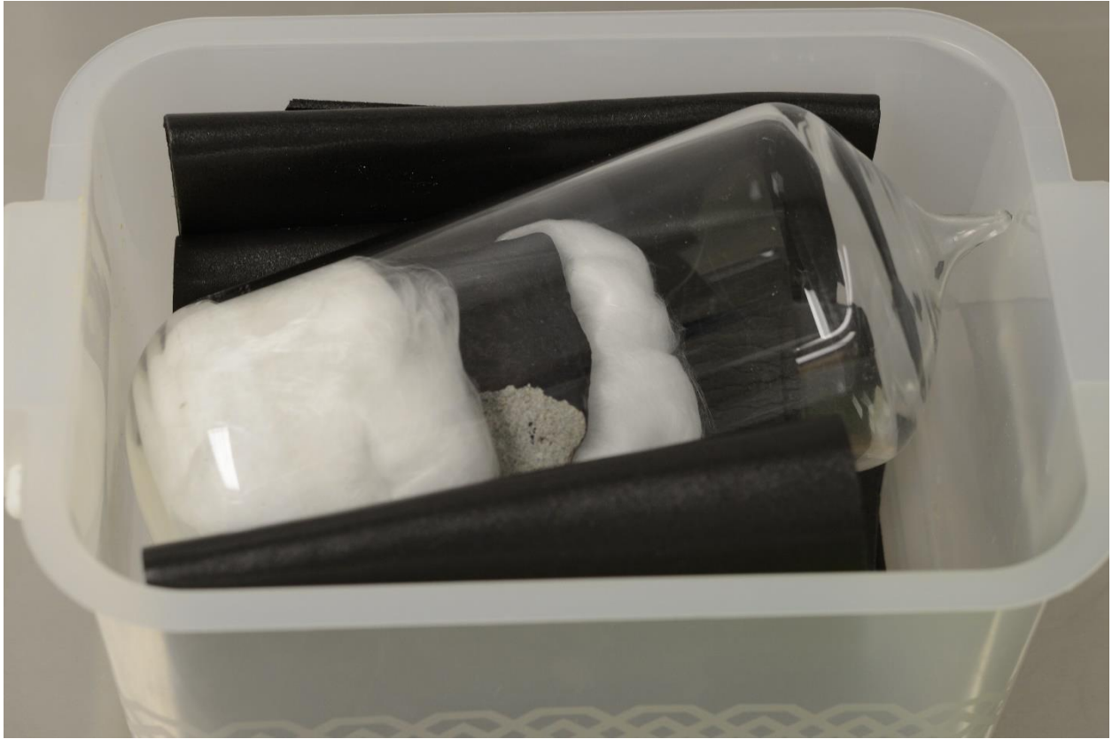
Figure 4.4. Photograph of MET4270/B-195 in the glass capsule with quartz wool cushioning.
