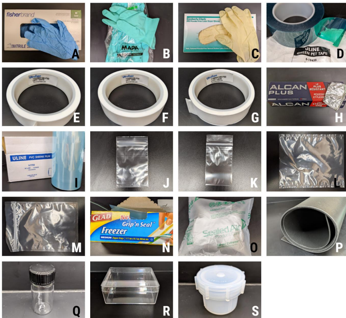
Figure 4.1. Curation materials that were swabbed with DCM. Materials included (a) Fisher nitrile gloves, (b) MAPA nitrile gloves, (c) Kimberly Clark co-polymer gloves, (d) Uline green PET tape, (e) UltraTape cleanroom tape #1153, (f) UltraTape cleanroom tape #1154, (g) UltraTape cleanroom tape #1160, (h) Alcan aluminum foil, (i) Uline PVC shrink film, (j) Shippers Supply reclosable bags, (k) Uline reclosable bags, (l) Benchmark Products Precision Clean II, (m) Benchmark Products Precision ZipClean Pouches, (n) Glad freezer bags, (o) Sealed Air air pillows, (p) Sekisui Voltek Inc Volara film, (q) Fisher Scientific glass vials, (r) Cargille Inc. plastic boxes, and (s) Savillelex PFA jar.
