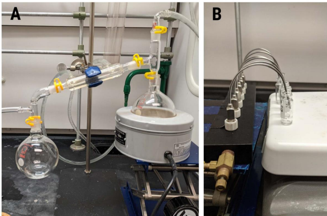
Figure 3.4. Setup of distilling calcium hydride (A) and evaporating down the derivatized hot water extracts (B) under a constant stream of N_{2(g)} to minimize moisture in the experiment.
