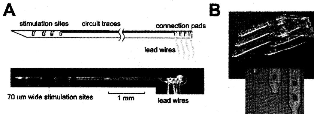
Figure 2.12: *Alternative designs for ISMS electrodes.*
