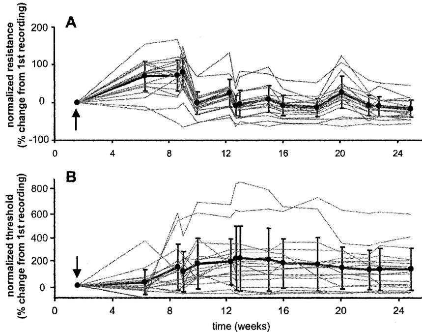
Figure 2.4: *Microwire resistances and motor thresholds measured periodically throughout a 6 month ISMS implant in a cat with spinal cord injury.*
