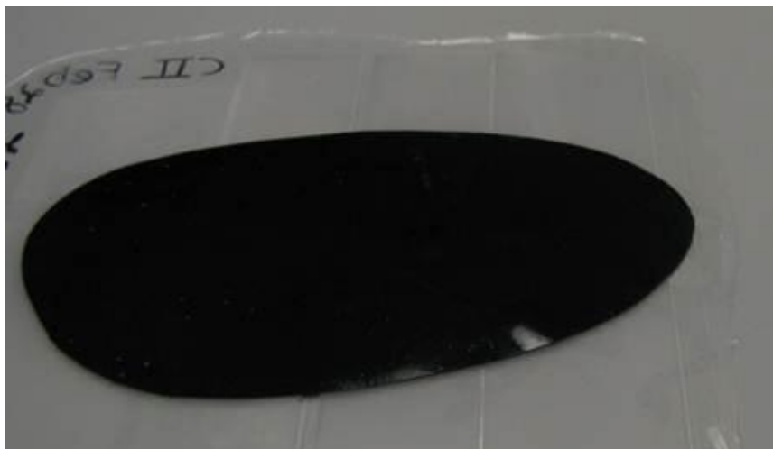
Figure 33: Result of laminating the viscous polymer/nanoparticle composite. A smooth, even backing layer is produced with fully formed adhesive structures.
