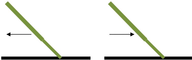
Figure 16: ST1060, 537.2 kPa, first pull (left) is towards acute angle of spatula. Second pull (right) is away from acute angle of spatula.
