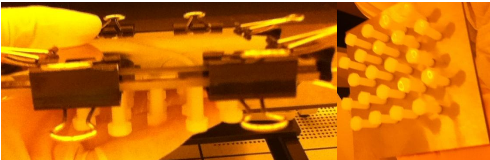
Figure 11: Adjustable screw apparatus for increasing mask contact. The screw array (right) is being used to apply pressure at strategic points of poor contact between the mask and substrate (left). Each screw can be individually turned to apply upwards pressure while the eight bull dog clips squeeze the mask, substrate, and screw apparatus together. The rigid glass mask remains stationary while the more flexible PMMA substrate conforms to flatten against it when being assisted by one or multiple screws.
