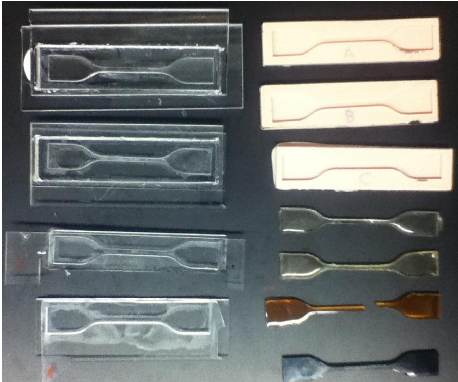
Figure 36: Various molds and casts for the dog bone test specimens. Upper left shows two PMMA positive molds, upper right shows the resulting TC-5045 silicone rubber negative molds, Lower right shows various dog bone specimen, lower left shows two negative PMMA molds. The PMMA molds were made using a laser engraver with scrap Acrylic, and thus the outer edges are slightly irregular.
