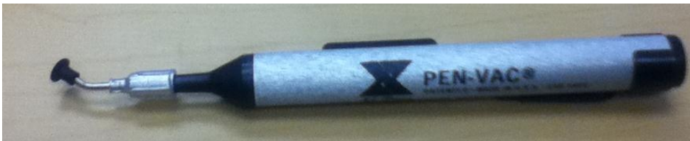
Figure 1: Vacuum pen for manual die manipulation. A lever on the side depresses a spring, and when the spring regains its shape air is pulled in through a hole in the rubber tip, creating a negative vacuum.
