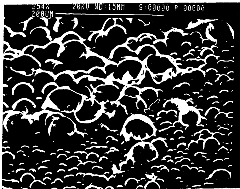
Figure 4.6 SEM Photo of Bubble Formation due to Excessive Anneal Temperature
