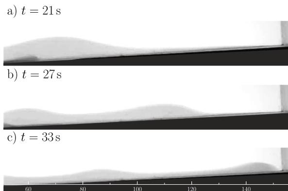
FIG. 6. Close-up snapshots of the subcritical gravity current experiment shown in Figure 5 focusing on the shoaling interfacial disturbance at times (a)  $t = 21$  s, (b)  $t = 27$  s, and (c)  $t = 33$  s. The field-of-view shows a portion of the tank far from the lock; the scale below panel c indicates the horizontal position from the lock-gate with distances measured in cm.
