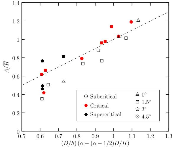
FIG. 12. Scaled interfacial disturbance amplitude vs the semi-empirical prediction (12) developed by Tan *et al.*<sup>19</sup> The dashed line uses  $\alpha = 0.67$  in (12) rather than  $\alpha = 0.87$ , the value suggested in this earlier study. Measurement errors are approximately equal to the size of the symbols.
