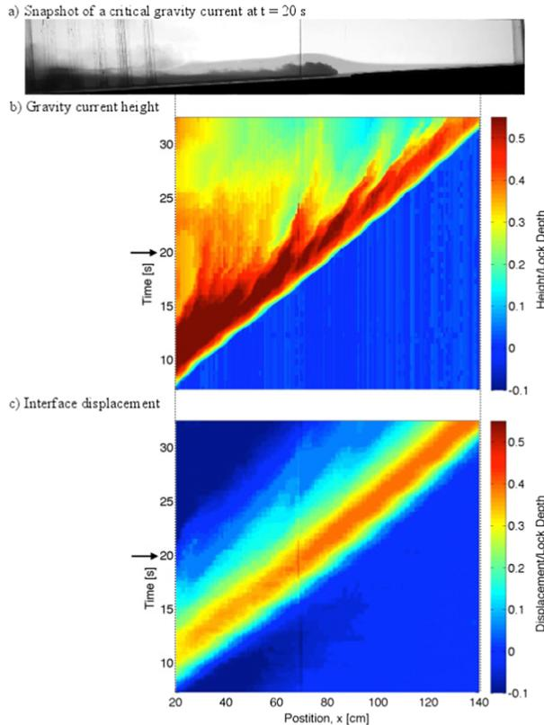
FIG. 4. As in Figure 2 but showing an example of a critical flow with  $D/H = 0.33$ ,  $s = 0.052$  ( $\theta = 3^\circ$ ),  $\rho_0 = 1.0083$  g/cm<sup>3</sup>,  $\rho_1 = 1.0017$  g/cm<sup>3</sup>, and  $S = 0.34$ .
