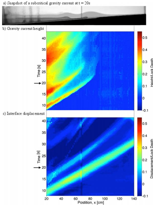
FIG. 5. As in figure 2 but showing an example of a subcritical flow with  $D/H = 0.33$ ,  $s = 0.052$  ( $\theta = 3^\circ$ ),  $\rho_0 = 1.014 \text{ g/cm}^3$ ,  $\rho_1 = 1.008 \text{ g/cm}^3$ , and  $S = 0.62$ .
