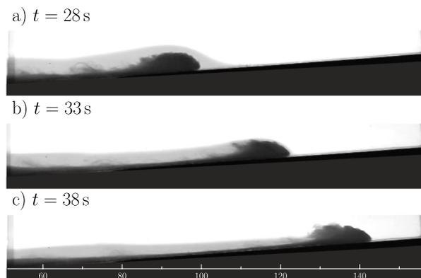
FIG. 3. Close-up snapshots of the supercritical gravity current shown in Figure 2 at times (a)  $t = 28$  s, (b) 33 s, and (c) 38 s. The field-of-view shows a portion of the tank far from the lock; the scale below panel (c) indicates the horizontal position from the lock-gate with distances measured in cm.
