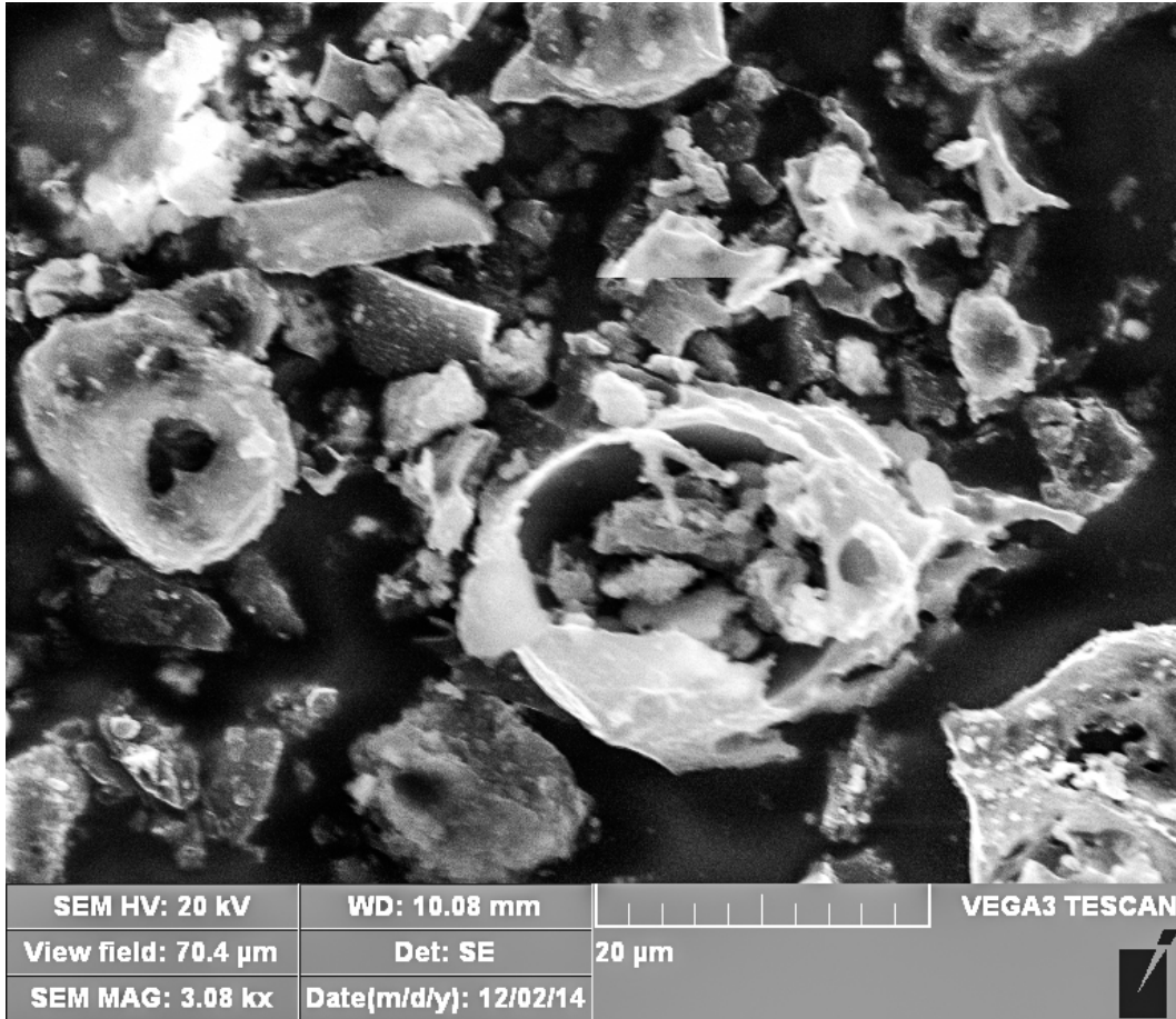
Figure 6.11: Raw coal char after combustion in an Entrained Flow reactor
