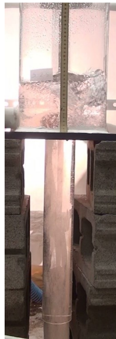
Fig A1.14 Different flow regimes in Series C2-1b (discharge ratio: 2) Two inlets at a horizontal plane (angle: 90), d_i=52 mm, S= 5 and 12 mm, d_o=76 mm
