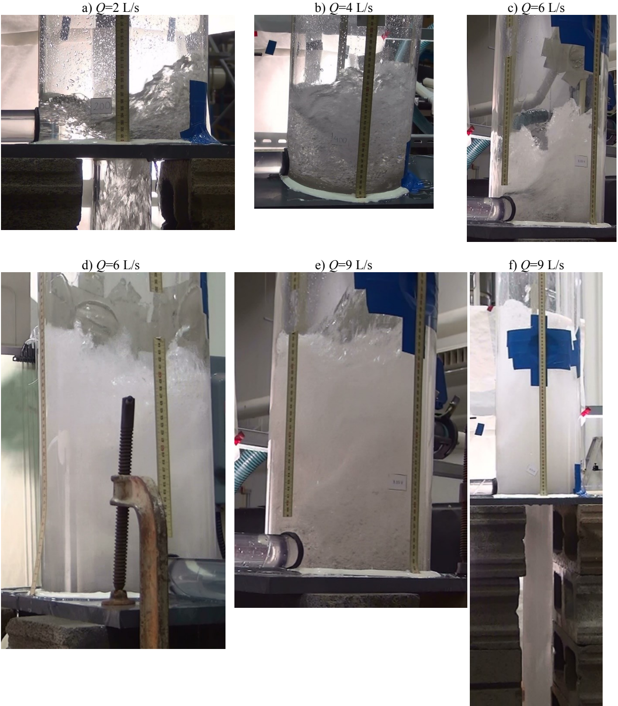
Fig A1.4 Different flow regimes in Series A2-1(One Inlet with d_i=4 mm and S= 8 mm, d_o=76 mm)
