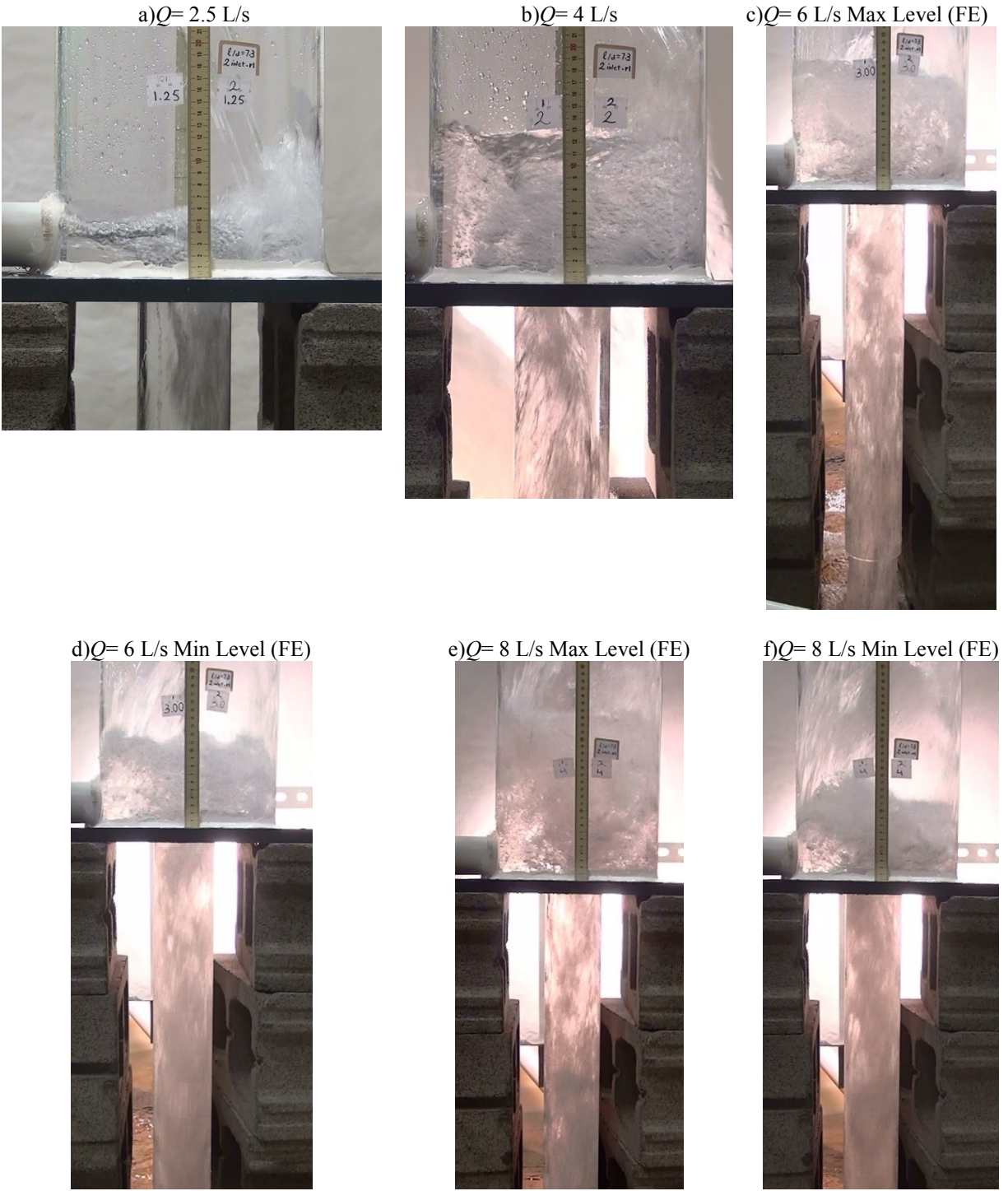
Fig A1.16 Different flow regimes in Series C2-2, (Series with two inlets at different horizontal planes with d_i=52 mm, S=12 & 389 mm, d_o=76 mm)
