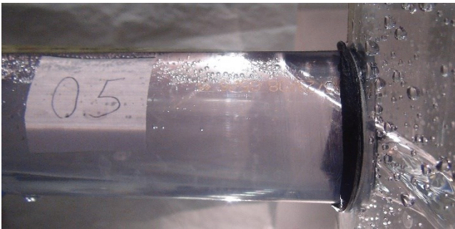
Fig A1.2 Comparing several cavity formation inside inlet in Series A1-2
