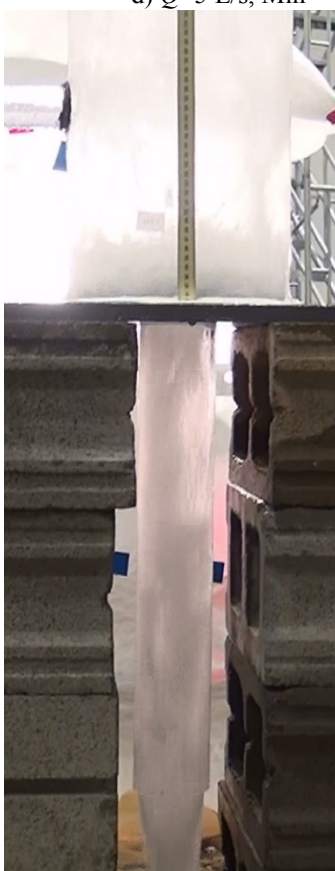
Fig A1.6 Different flow regimes in Series A2-3 (One Inlet with d_i=4 mm and S= 207 mm, d_o=76 mm)
