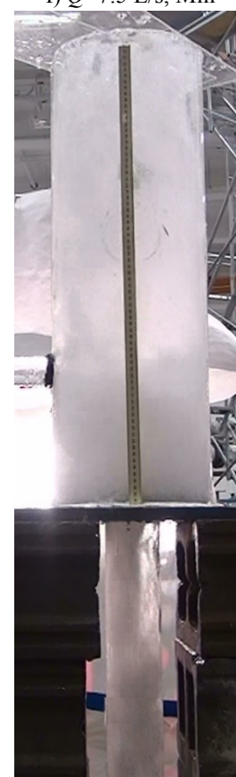
Fig A1.6 Different flow regimes in Series A2-3 (One Inlet with d_i=4 mm and S= 207 mm, d_o=76 mm)
