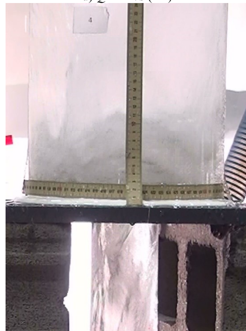
Fig A1.1 Different flow regimes in Series A1-2 (One inlet with d_i=4 mm and S=401 mm, d_o=76 mm)
