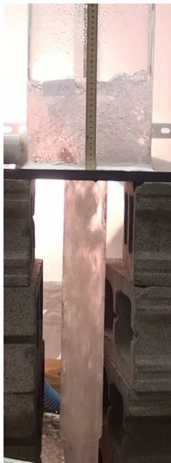
Fig A1.14 Different flow regimes in Series C2-1b (discharge ratio: 2) Two inlets at a horizontal plane (angle: 90), d_i=52 mm, S= 5 and 12 mm, d_o=76 mm
