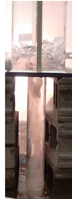
Fig A1.14 Different flow regimes in Series C2-1b (discharge ratio: 2) Two inlets at a horizontal plane (angle: 90), d_i=52 mm, S= 5 and 12 mm, d_o=76 mm
