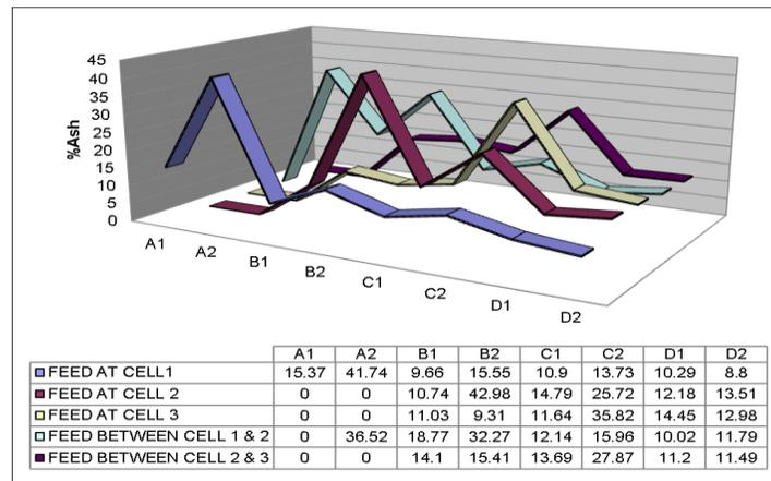
**Figure 14. Effect of Feed Location on Continuous mode Separator**
