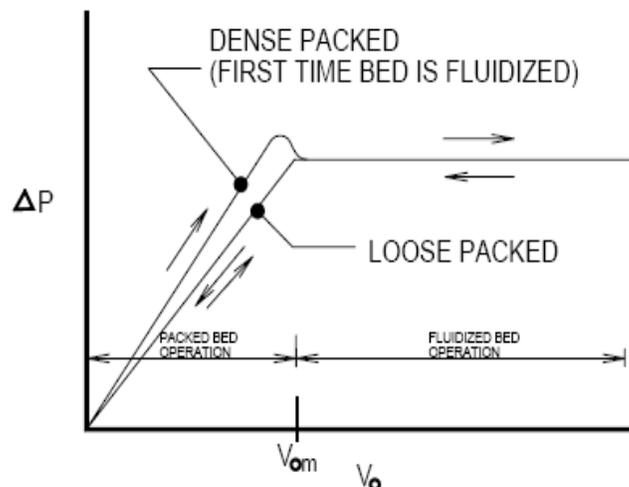
**Figure 4. Standard patterns of solids fluidisation (Chase, 2004)**
