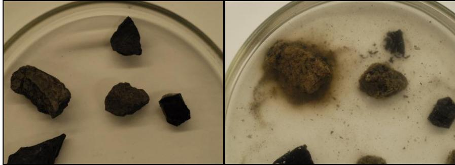
**Figure 2. Sliming of Alberta sub-bituminous coal (Dave et al, 2010)**
