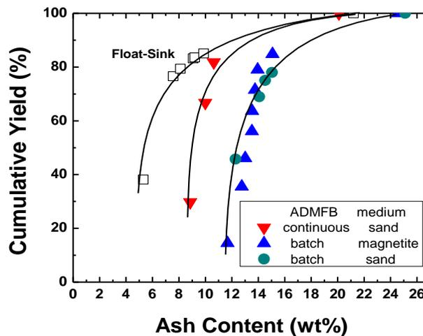
**Figure 20.** Effect of types of medium on ADMFB separators operated at batch mode on Separation performance (1 minute Fluidisation stratification). (Dave et al, 2010)
