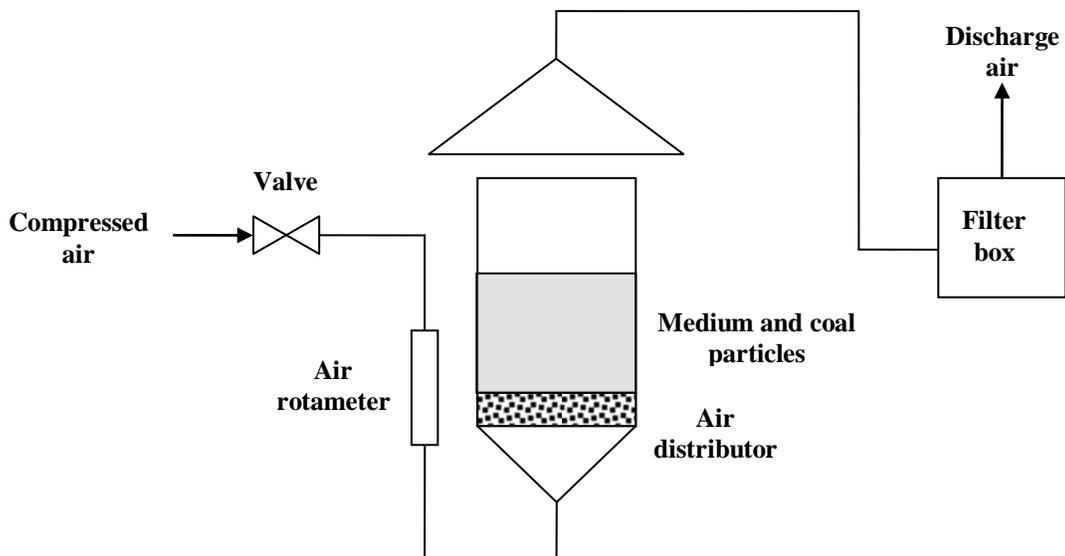
**Figure 8.** Schematics for the Batch mode Air Dense Medium Fluidised Separator (Zheng et al, 2007)
