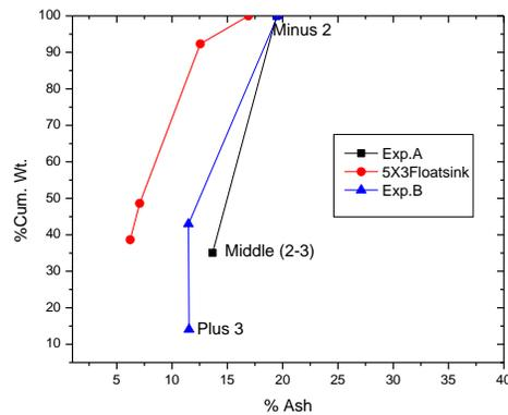
**Figure 11. Effect of Discharge flow on Continuous Mode ADMFB Separator**
