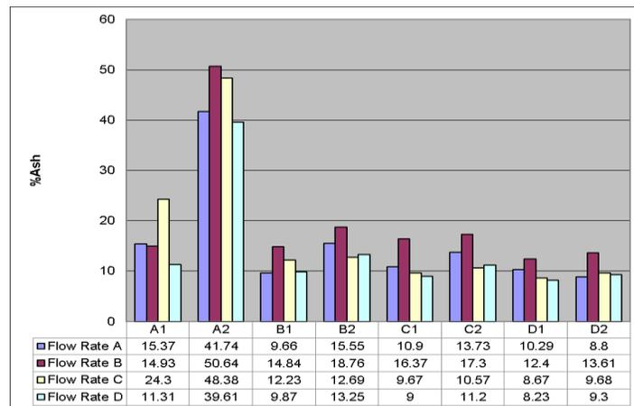
**Figure 15. Effect of Flow rate on Continuous mode Separator**
