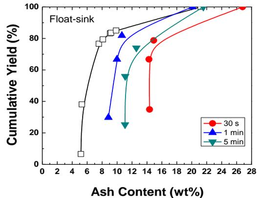
**Figure 21. Effect of Fluidisation time on Laboratory continuous ADMFB separator operated at Batch mode (Dave et al, 2010)**
