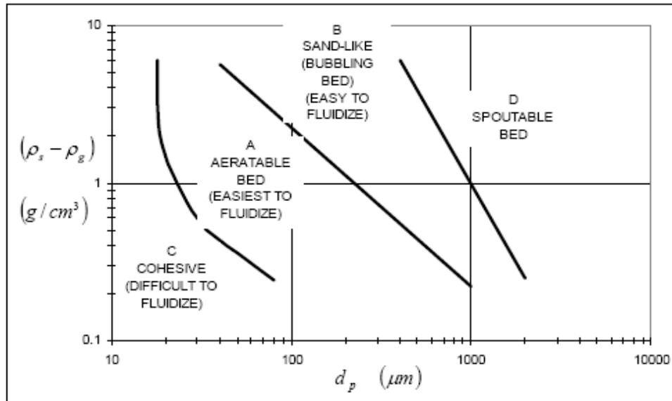
**Figure 6. Types of Gas Fluidisation (Geldart, 1973)**
