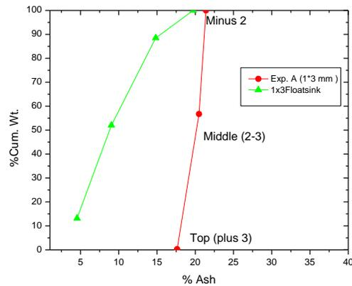
**Figure 12. Effect of size on Continuous mode ADMFB Separator**
