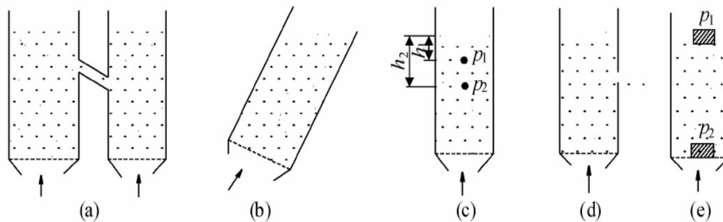
**Figure 5. Liquid-like behavior of gas-solid bed after fluidisation (Zhen-fu et al, 2007)**
