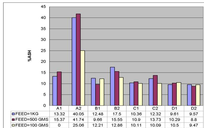
**Figure 16. Effect of Volume Loading on Continuous mode Separator**
