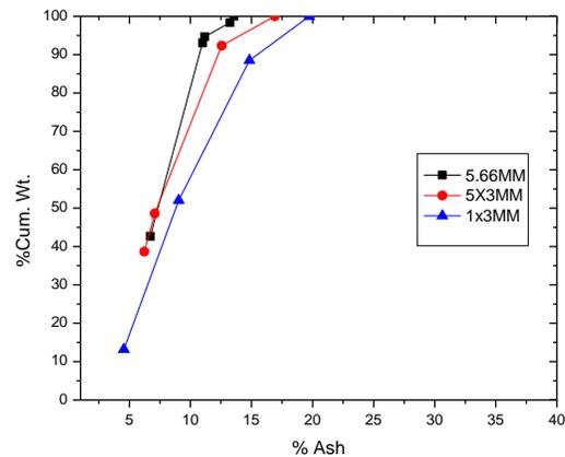
**Figure 10.** Float sink analysis for various size of Seam 2 coal
