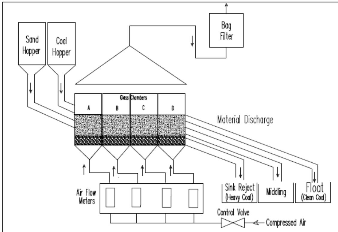
**Figure 9. Schematics of the Continuous mode Air Dense Medium Fluidised Bed Separator (Dave et al, 2010)**
