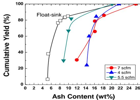
**Figure 22.** Effect of different air velocity on separation for continuous ADMFB separators operated at batch mode for single cell (Dave et al, 2010)
