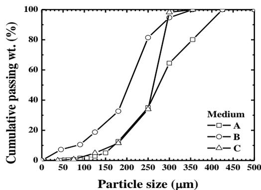
Figure 19. Size distribution for different mediums (Mak, 2007)
