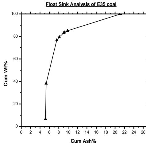
**Figure 18.** Float-Sink analysis of 1.0-5.66 mm E35 coal from Epcor
