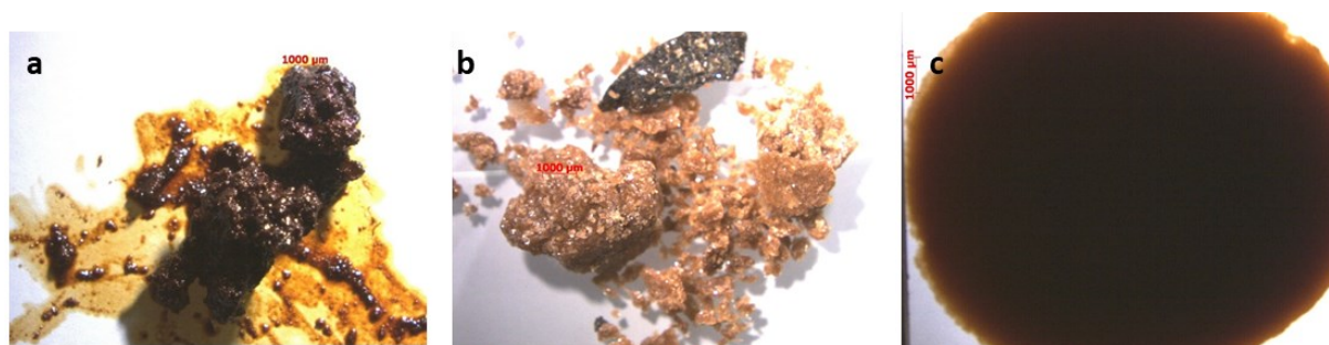
Figure 4.1. Pictures captured by Zeiss microscope for products of thermally cracked (a) indene, (b) indole and (c) benzofuran.
