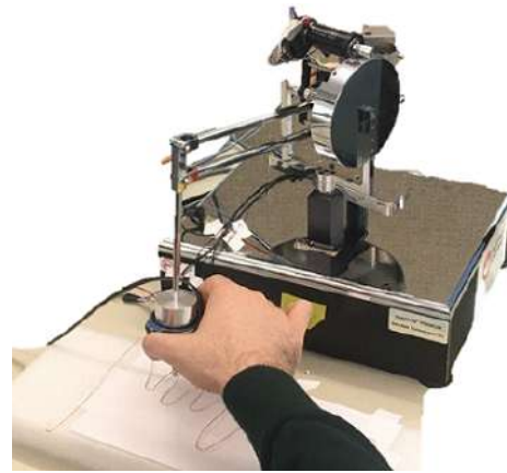
Fig. 7. Using Phantom Premium 1.5A Haptic Device in the squiggly line tracking task to test the generality of SkillNet and performance of the skill transfer algorithm in practice with different user data and another robotic platform.
